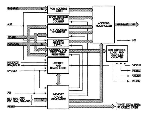
Figure 3-1. TMS34061 Internal Architecture Block Diagram
