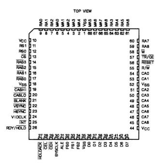
Figure 2-1. TMS34061 Pin Assignments and Signal Names
