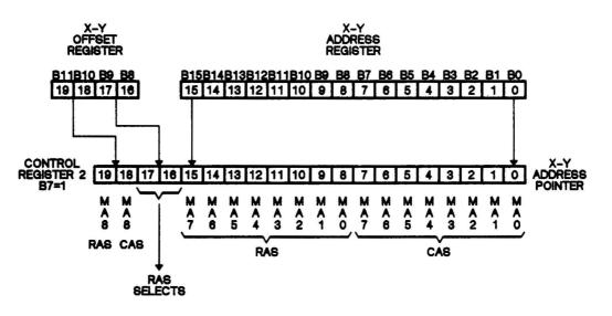
Figure 3-2. X-Y Address Pointer Register Construction
