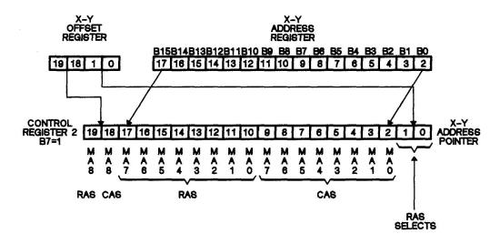
Figure 3-3. X-Y Address Pointer Register Output
