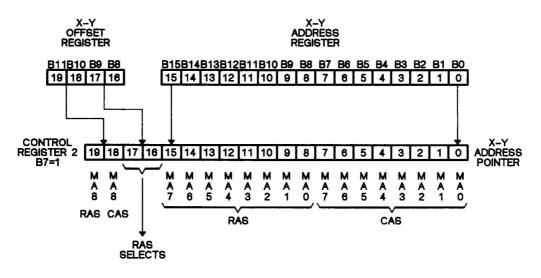
Figure 4-8. X-Y Address Pointer RAS Selects as MSBs
