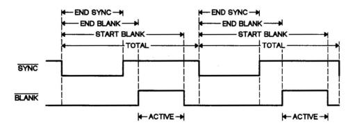
Figure 8-2. Horizontal and Vertical Timing Information
