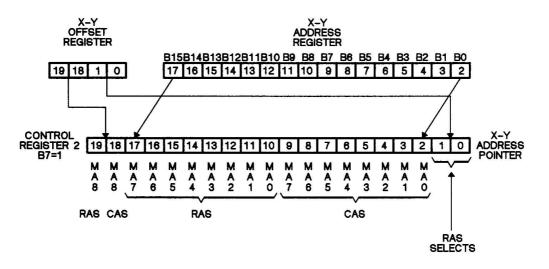
Figure 4-9. X-Y Address Pointer RAS Selects as LSBs
