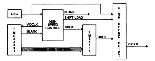
Figure 8-1. TMS34061 High Speed Logic
