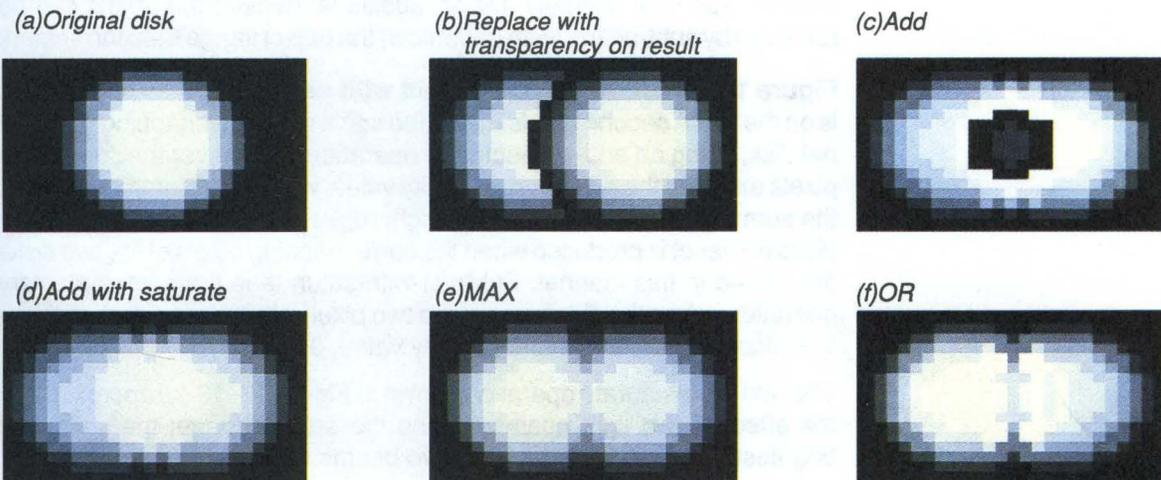
The gradual change in intensity at the edge of the disk in Figure 12–13 (a) is similar to the result produced by antialiasing techniques that reduce jagged-edge effects. A text font might be stored in antialiased form, for example, to give the text a smoother appearance. When two characters from the font table are
