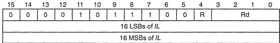
**Description** ANDNI bitwise-ANDs the 1s complement of a 32-bit immediate value with the contents of the destination register and then stores the result in the destination register. (The symbol *IL* in the syntax above represents a 32-bit immediate value.) ANDNI also uses this opcode.
