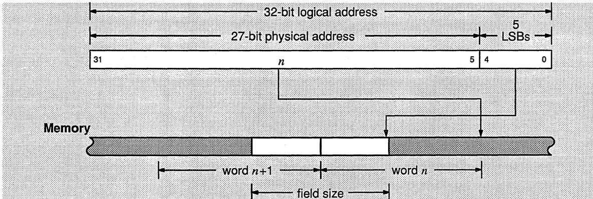
In Figure 3-5, word  $n$  is pointed to by a 27-bit physical address, output by the TMS34020 to memory. This 27-bit address corresponds to bits 5—31 of the field's 32-bit logical address. The 5 LSBs of the logical address point to the beginning of the field within word  $n$ .
