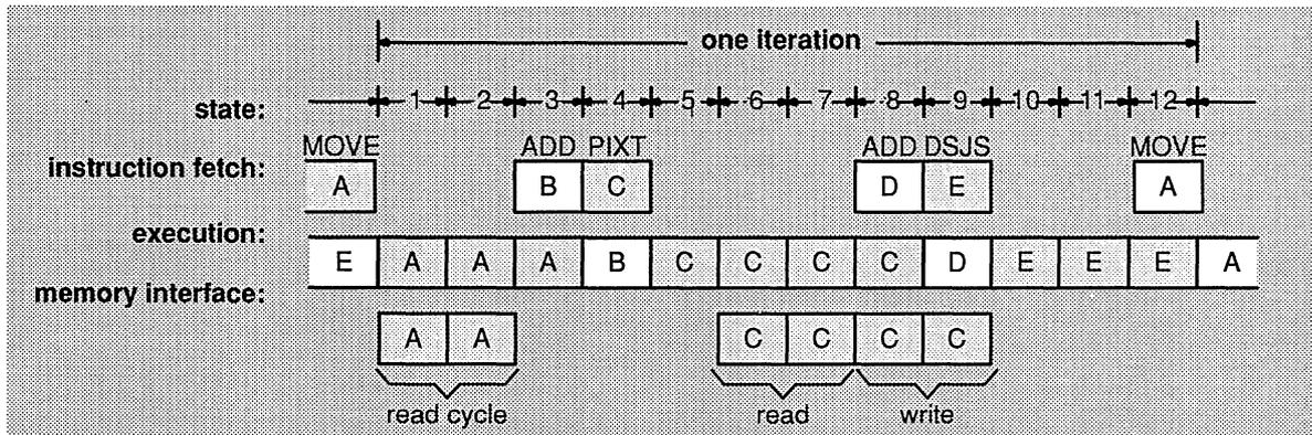
Figure 5–4 (a) shows the inner loop of a graphics routine; Figure 5–4 (b) represents execution of the code in (a). Figure 5–4 (b) shows three activities occurring in parallel:
