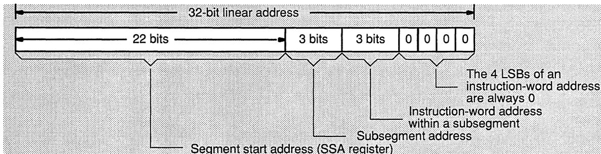
The 22 bits of the SSA register correspond to the 22 MSBs of the segment's memory address. These 22 MSBs are common to all 8 subsegments within a segment. The next three bits (bits 6–8) identify one of the 8 subsegments. Bits 4, 5, and 6 identify one of the 8 instruction words within a subsegment. The 4 LSBs are always 0s because instructions are aligned on word boundaries.
