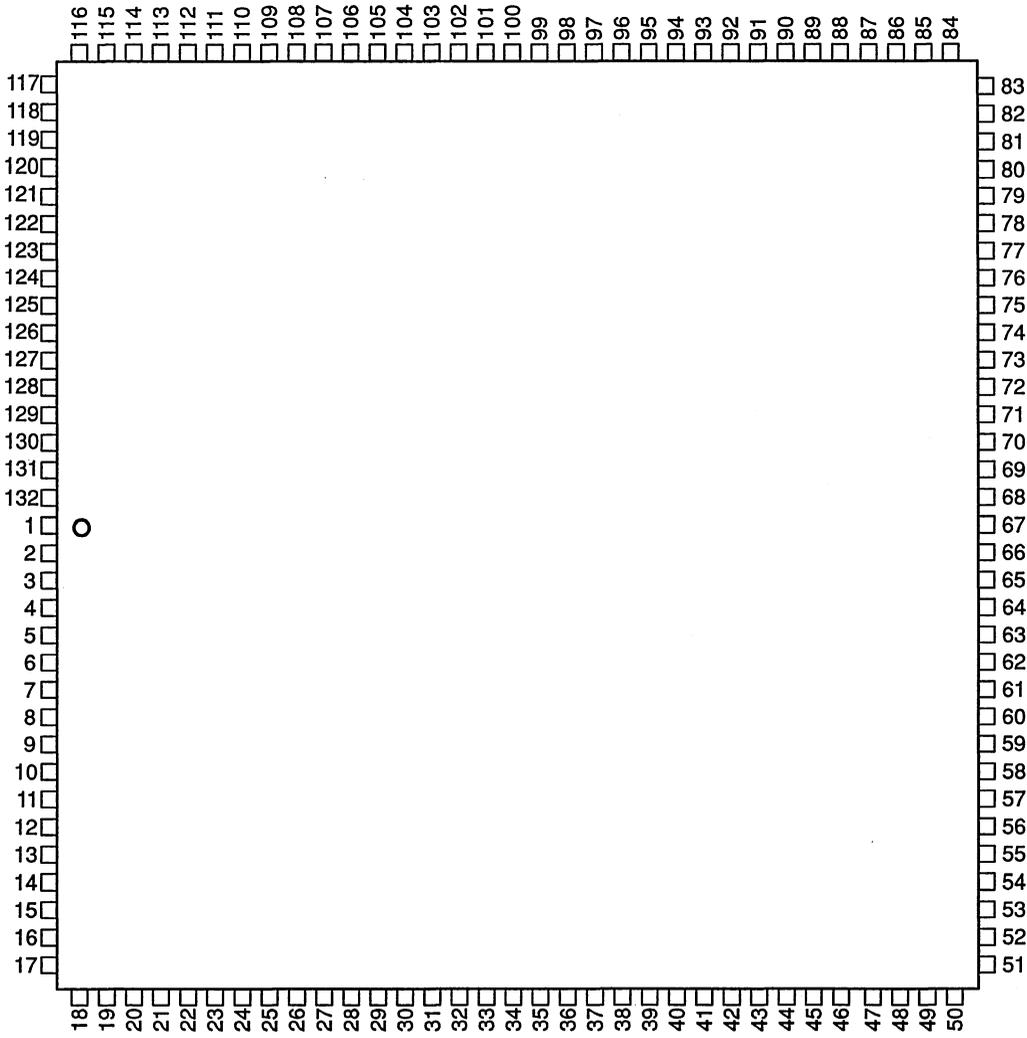
Table 2-3. Numerical List of TMS34020 Pin Assignments (132-Pin QFP)
