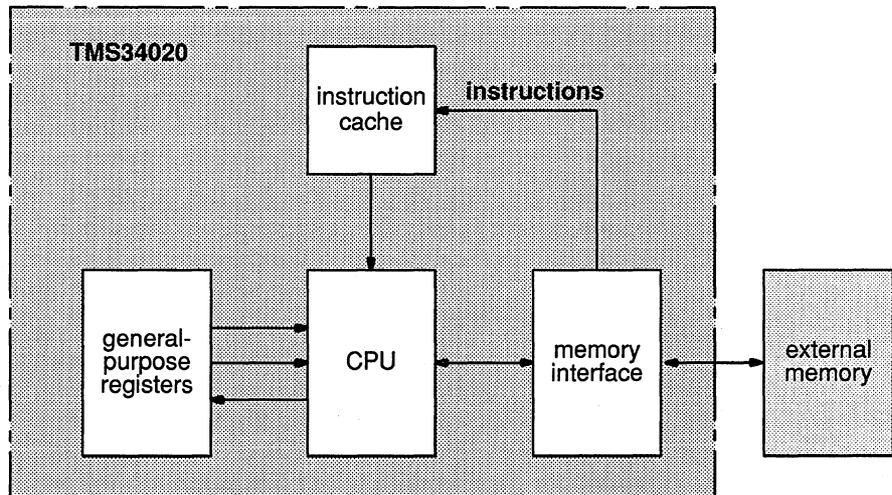
The TMS34020 can access each storage area independently of the other two. This allows the TMS34020 to perform the following actions in parallel during a pair of machine states:
