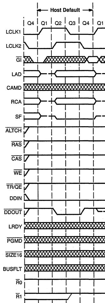
The address and status code output are normally of no significance, because  $\overline{\text{ALTCH}}$  and  $\overline{\text{RAS}}$  are not activated. The reason they are output at all is because
