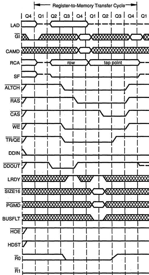
**Do not** use the video-capture feature with midline reloads. The register-to-memory cycle overwrites an entire VRAM row from the VRAM serial register. In the case of the first midline reload that follows the end of horizontal blanking, not all the bits in the serial register would need transferring—only those shifted in since the end of blanking.
