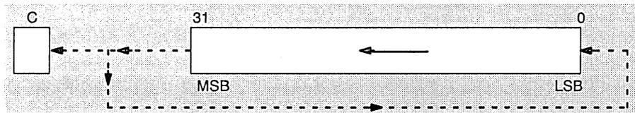
The assembler only accepts absolute expressions for the rotate count. If the specified rotation value is greater than 31, the assembler issues a warning and sets the constant to its 5 LSBs.
