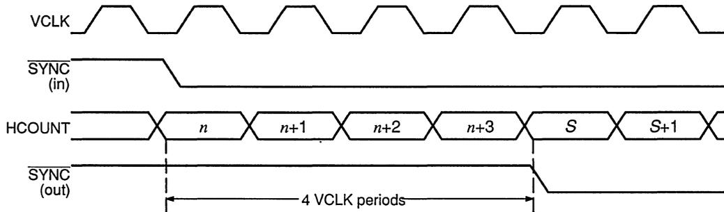
**Note:**  $S$  is the value contained in SETHCNT. 4-VCLK cycles after the falling edge on the input  $\overline{\text{SYNC}}$  pin occurs, HCOUNT is loaded with  $S$ , and the transition on the output  $\overline{\text{SYNC}}$  is caused to occur.
