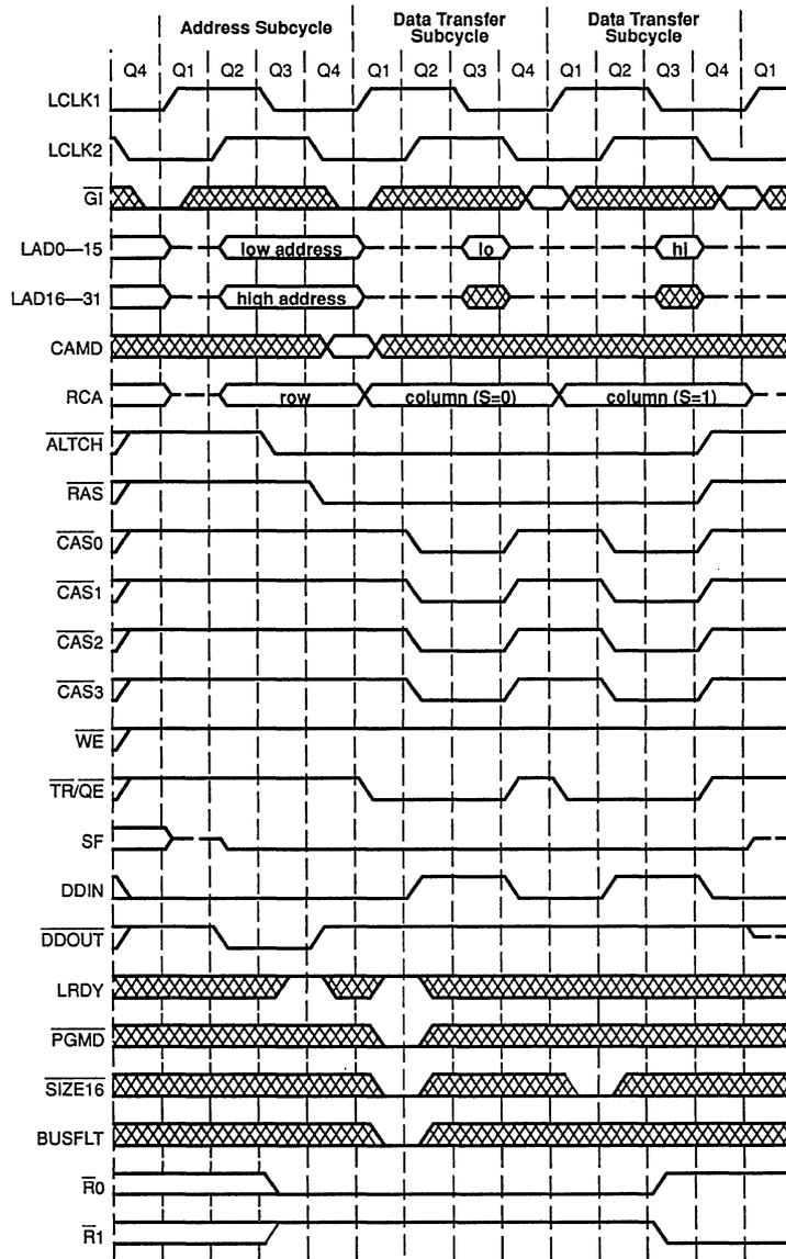
Figure 8–8. Dynamic Bus Sizing for a Write Cycle (Connection to LAD16—LAD31, Indicated by  $\overline{\text{SIZE16}}$  High During 2<sup>nd</sup> Data Cycle)
