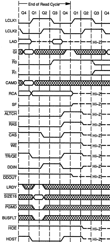
Figure 11-5 shows  $\overline{GI}$  being driven inactive just after the TMS34020 has started a sequence of page mode accesses. The TMS34020 breaks the sequence and issues the access-termination code. If  $\overline{GI}$  had remained active, this code would not have been generated until the sequence completed.
