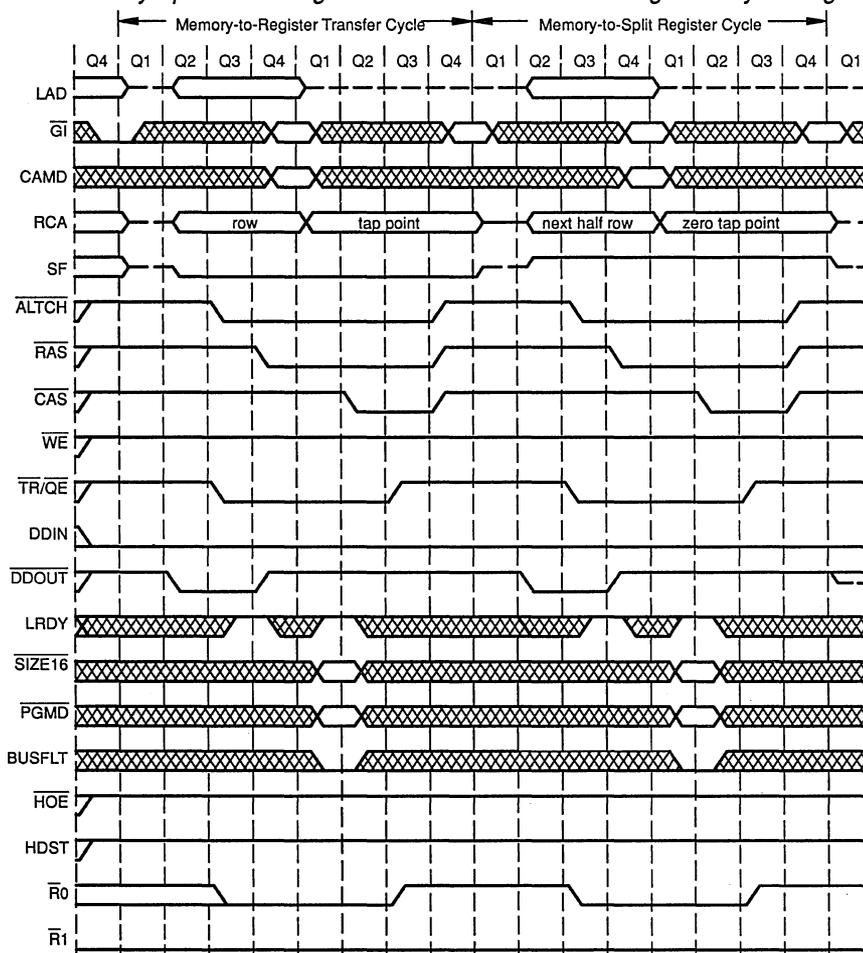
**Note:** During the second screen-refresh cycle, the MSB of the column address identifies which half of the serial register is reloaded. Remaining bits of the column address = 0 and represent the tap point. The row address output now addresses the memory row containing the next half row to be transferred to the split serial reg.
