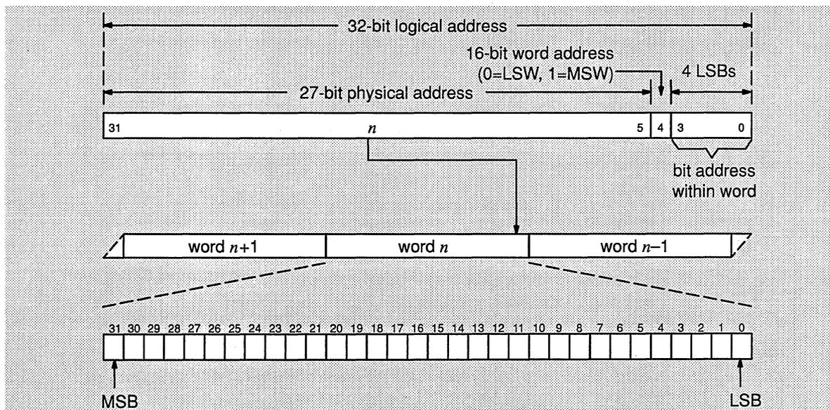
The TMS34020 communicates with memory over a 32-bit address/data bus (LAD0—LAD31) and always reads a complete long (32-bit) word from memory. Writes to memory may be 8-, 16-, 24-, or 32-bit values through the use of the TMS34020's  $\overline{\text{CAS}}$  (byte) strobes.
