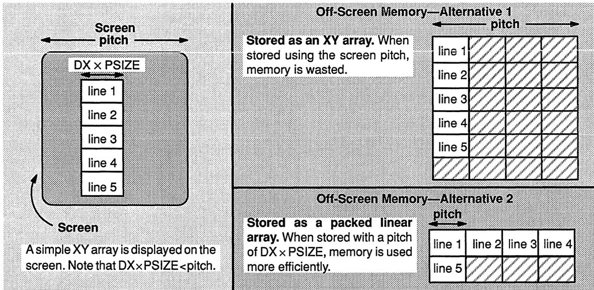
To store an XY array in packed linear form, use the PIXBLT XY, L instruction; to move a packed linear array onto a screen, use PIXBLT L,XY.
