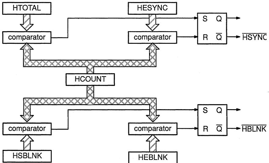
When HCOUNT = HSBLNK (shortly before the end of the horizontal scan), horizontal blanking begins. At this time, the video timing logic automatically schedules a screen-refresh memory cycle, preparing for the next displayed line.
