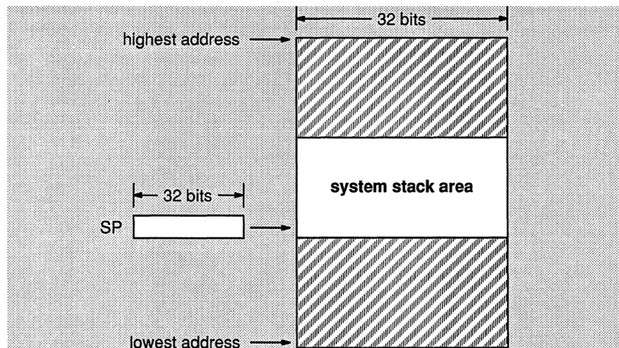
The SP points to the top of the stack; it contains the 32-bit address of the LSB (bit 0) of the value on top of the stack. The SP can contain any 32-bit address; however, stack operations execute more efficiently when the 5 LSBs of the SP
