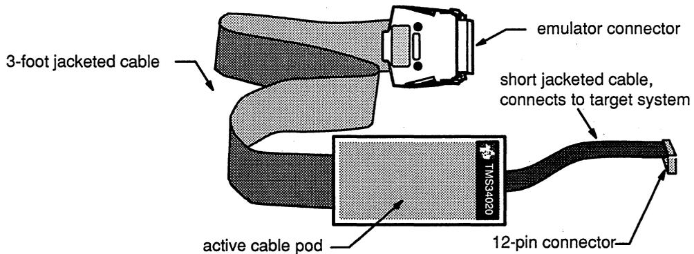
The overall cable length is approximately 3'10". Figure A-7 shows the mechanical dimensions for the target cable pod. The cable pod box is nonconductive plastic with 4 recessed metal screws.
