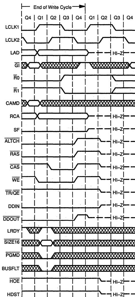
Figure 11-4 shows the TMS34020 outputting the access-termination code at the end of a (high priority) host read cycle. Note that  $\overline{GI}$  may be sampled at either level while the high-priority request code is being output. The TMS34020 cannot relinquish control of the local-memory interface until it completes the memory access (at which time it issues the access-termination code).
