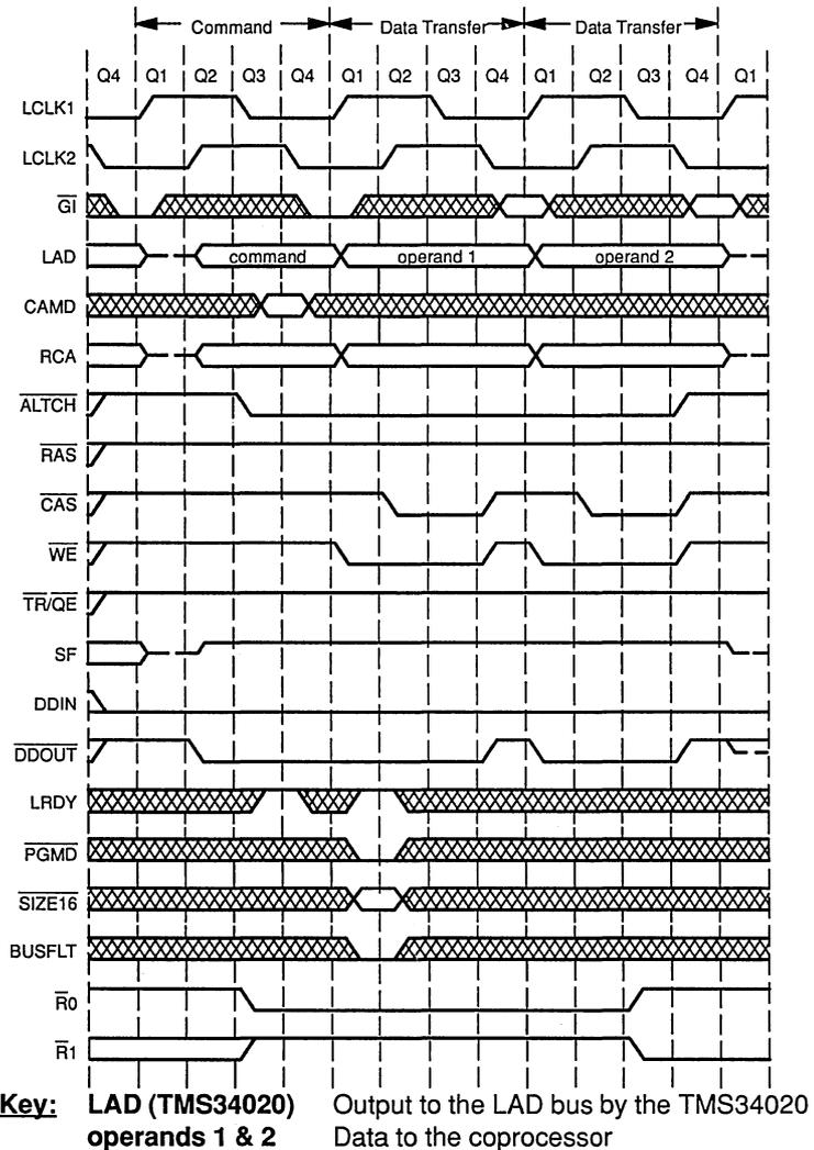
One or two 32-bit words may be transferred. If two words are transferred, the size bit determines whether the coprocessor should treat the words as two
