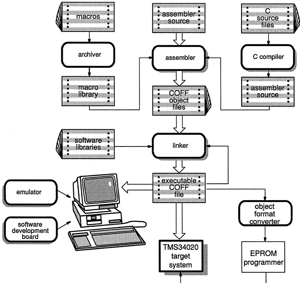
These tools use common object files format (COFF), which encourages modular programming. COFF allows you to divide your code into logical blocks, define your system's memory map, and then link code into specific memory areas. COFF also provides rich support for source-level debugging.
