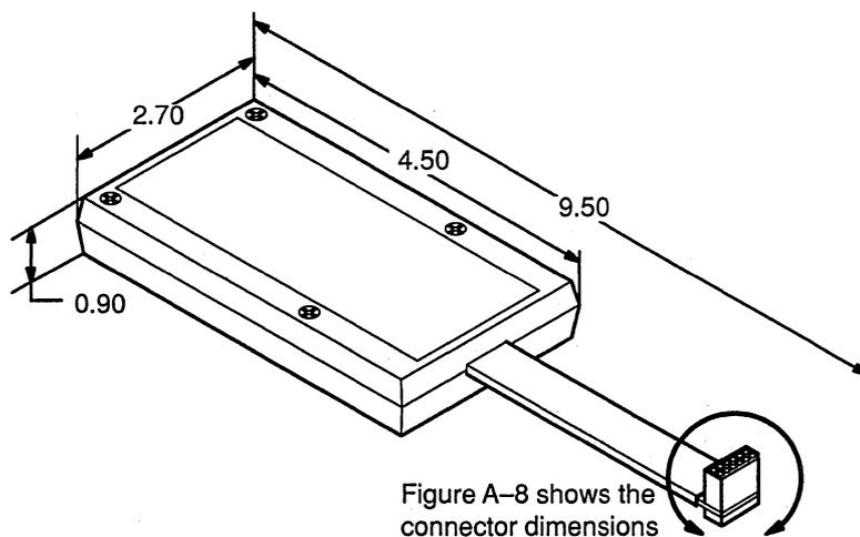
Figure A-8 shows the connector dimensions
