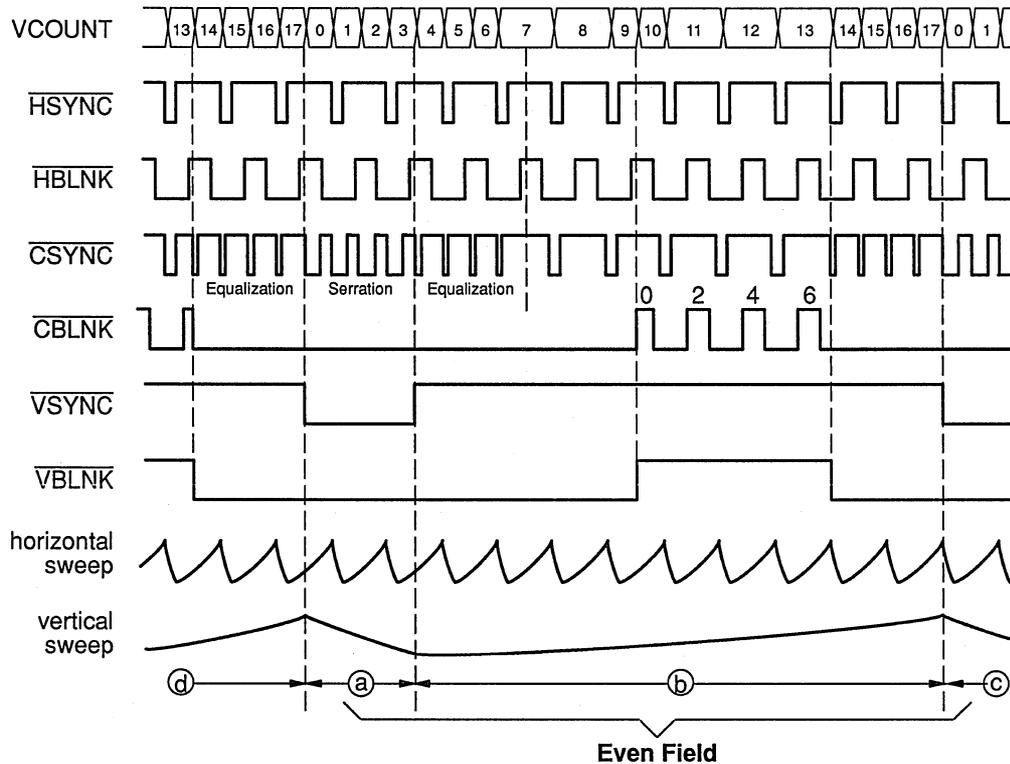
In Figure 9–15, VCOUNT is incremented twice per horizontal scan line during serration and equalization periods. This is the frequency at which equalization and serration pulses occur. Because VCOUNT increments every half line between the beginning of the first equalization period to the end of the second equalization period, you can specify the number of equalization and serration pulses required without being restricted to an integral number of lines.
