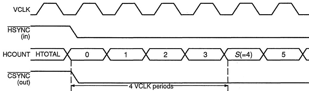
**Note:** If HTOTAL matches the external system and  $S=4$ , HTOTAL causes the output sync pin to transition in the same VCLK cycle as the input sync.
