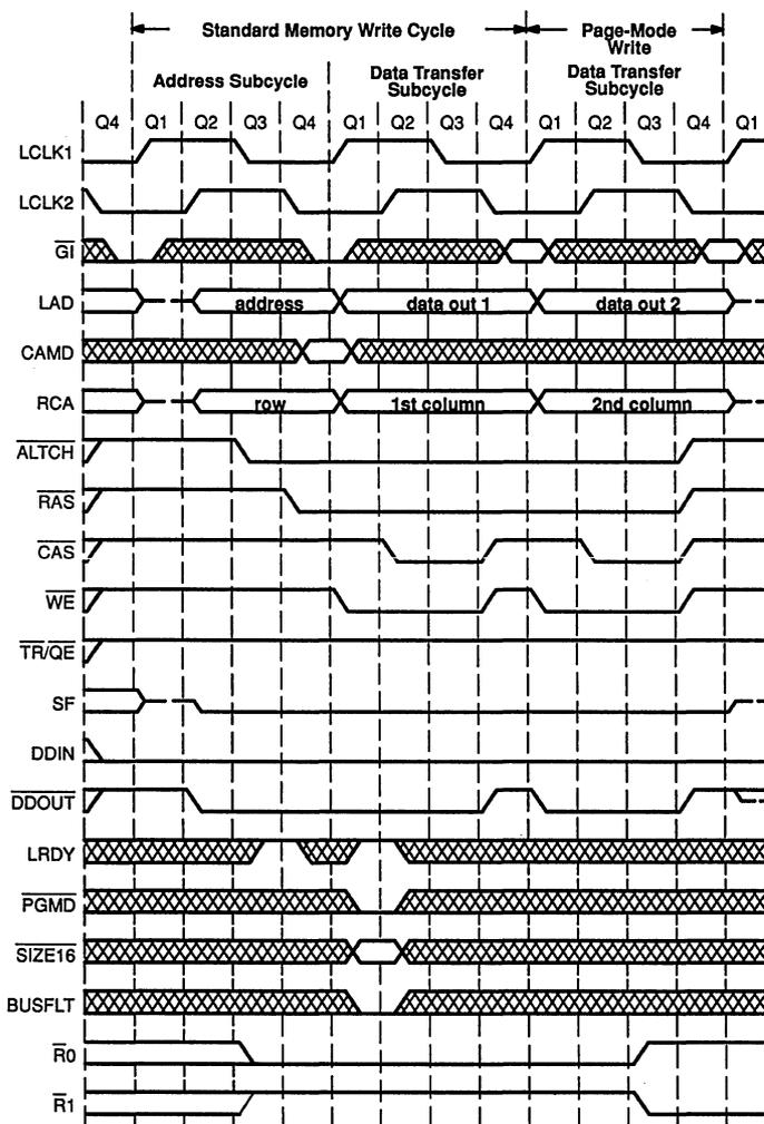
Note that when accessing a 32-bit memory, the TMS34020 does not sample  $\overline{\text{LRDY}}$ ,  $\overline{\text{PGMD}}$ , and  $\overline{\text{BUSFLT}}$  during subsequent page-mode cycles. The TMS34020 does not sample  $\overline{\text{SIZE16}}$  during the page-mode cycle, because the memory has responded that it supports 32-bit accesses. Section 8.9 (page 8-25) discusses dynamic bus sizing and  $\overline{\text{SIZE16}}$  in detail.
