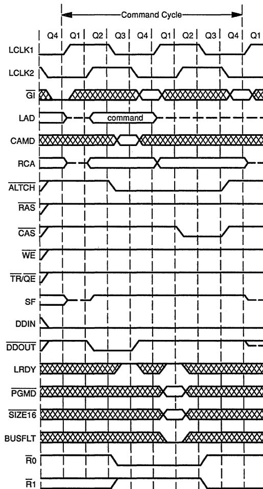
**Note:** Although the coprocessor command cycle never requires the use of page-mode cycles, you should still assert  $\overline{\text{PGMD}}$  at a valid level (high or low) at the time it is sampled by the TMS34020.
