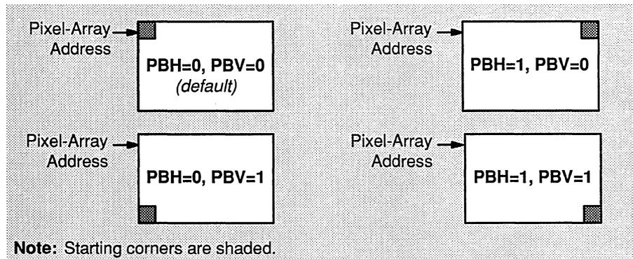
As Figure 12–3 shows, the PBV[CONTROL] and PBH[CONTROL] bits determine the starting corner for the PIXBLT. PBH controls horizontal movement; PBV controls vertical movement.
