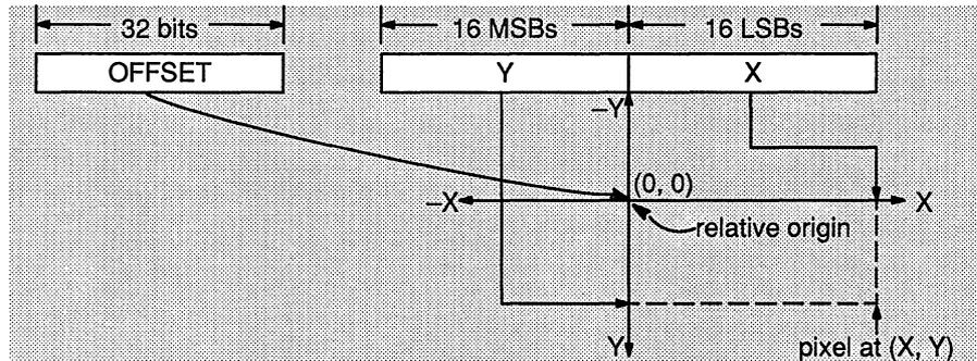
In Figure 3–13, a 32-bit general-purpose register contains an XY address. The X and Y components are treated as separate 16-bit signed integers. The X component is right-justified within the 16 LSBs of the register. The Y component is right-justified within the 16 MSBs of the register.
