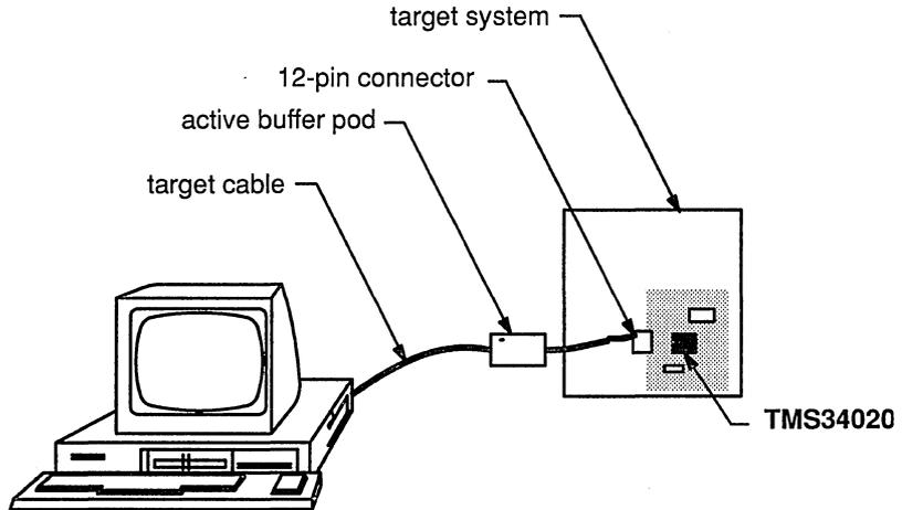
Figure A-2 shows how you connect the emulator and target cable to your target system.
