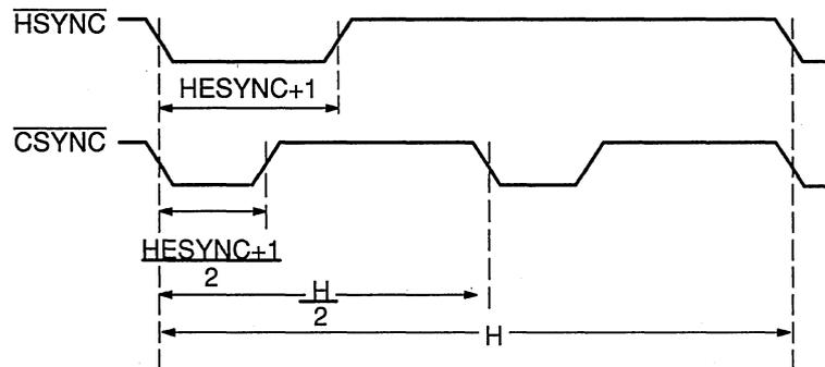
Broadcast-quality composite-video standards such as NTSC and PAL require that equalization pulses are exactly half the duration of horizontal-sync pulses. To achieve this, set  $HESYNC$  to an odd value.  $HCOUNT$  starts counting from 0, so an odd value in  $HESYNC$  means that horizontal sync is an even number of  $VCLK$  cycles in length, and therefore exactly divisible by 2. Similarly, set  $HTOTAL$  to an odd value so that  $HTOTAL/2$  is exactly the midpoint of each scan line.
