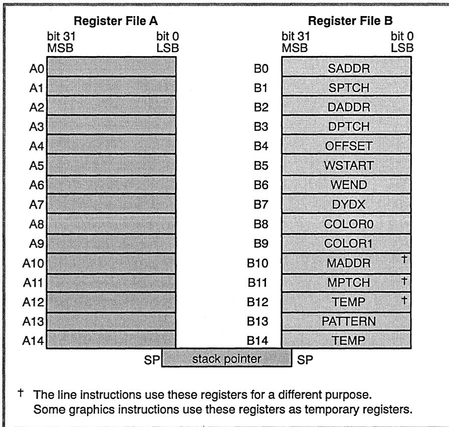
As Figure 4–4 shows, 15 of the general-purpose registers, A0–A14, form register file A. Register file B also consists of 15 general-purpose registers, B0–B14. Many of the TMS34020 instructions use these registers for storing and manipulating data.
