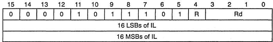
**Description**            This instruction bitwise-ORs a 32-bit immediate value with the contents of the destination register and stores the result in the destination register. (*IL* in the syntax represents the 32-bit value.)
