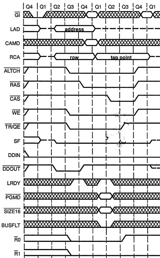
Although the TMS34020 ignores  $\overline{PGMD}$  and  $\overline{SIZE16}$  during this cycle, they should be held at valid levels as shown. Note that external logic must provide control of the VRAM  $\overline{SOE}$  pin.
