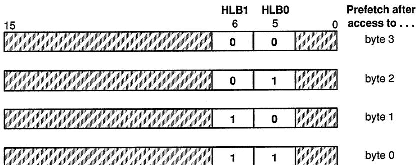
The HLB bits allow the host interface to accommodate all possible byte-ordering conventions and several different data-bus sizes.
