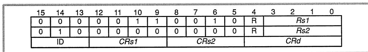
**Note:** This portion of the figure shows the ADD pseudo-op. ADD is a special form of the TMS34020 CMOVGC instruction. The coprocessor command and size portions of the CMOVGC instruction are hardcoded to specifically match the needs of the TMS34082's ADD instruction.
