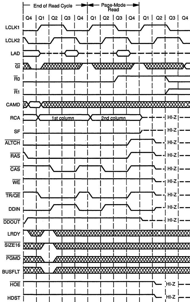
In Figure 11-6, the TMS34020 regains bus mastership as soon as its  $\overline{GI}$  pin is driven active low.  $\overline{R0}$  and  $\overline{R1}$  could be outputting any of the codes with the exception of the access-termination code.
