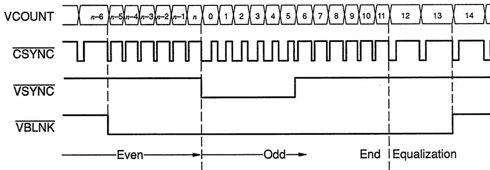
Figure 9-18. Vertical Blanking for NTSC and PAL Standards (Continued)
