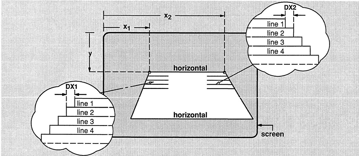
$x_1$  and  $x_2$  define the length and position of a horizontal line. TFILL draws a line, adjusts  $x_1$  and  $x_2$  by a specified amount, and increments  $y$  to point to the next position where a line could be drawn. Executing TFILL once draws only one line; to draw a trapezoid, you must call TFILL an appropriate number of times.
