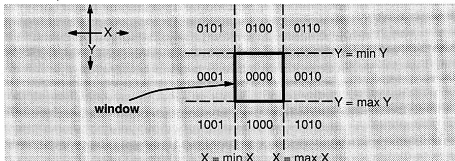
In this method, each region is assigned a 4-bit outcode. When an endpoint of a line falls within a particular region, it is assigned the outcode for that region. The outcodes determine the treatment of the lines.
