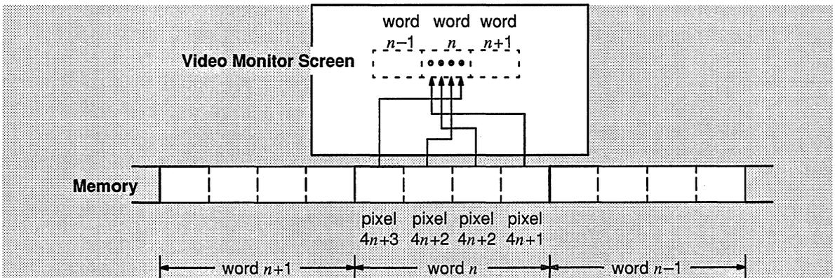
The TMS34020 allows you to identify a pixel in terms of its XY coordinates on the screen or in terms of the address of the logical pixel in memory. These 2 methods are called **XY addressing** and **linear addressing**, respectively.
