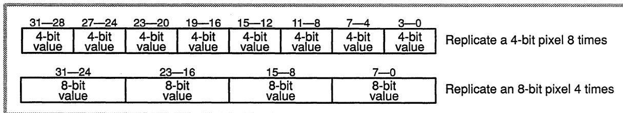
You can use the RPIX instruction to replicate the plane-mask value in a general-purpose register and then move the value into PMASK.
