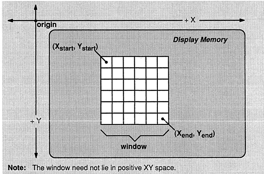
Figure 12–7 shows that a pixel with coordinates  $(X, Y)$  lies within the window if  $X_{start} \leq X \leq X_{end}$  and  $Y_{start} \leq Y \leq Y_{end}$ . If a pixel does not meet these conditions, it lies outside the window.
