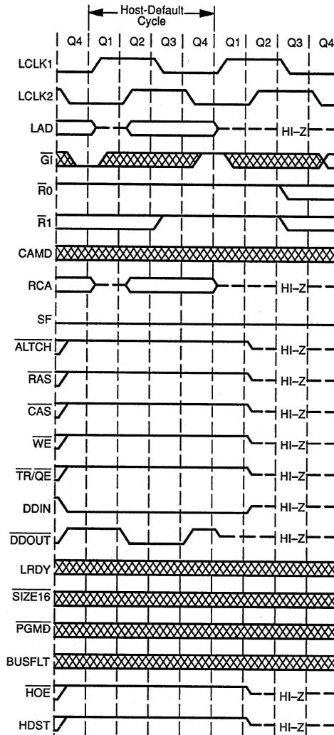
Figure 11-3 is identical to Figure 11-2 except that the TMS34020 is outputting the access-termination code at the end of a low-priority write cycle. Note that  $\overline{GI}$  may be sampled at either level while the low-priority request code is being output. The TMS34020 cannot relinquish control of the local-memory interface until it completes the memory access (at which time it issues the access-termination code).
