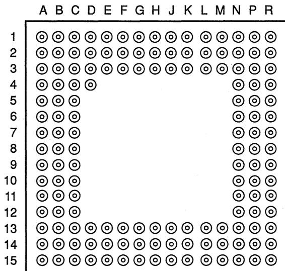
Table 2-1. Numerical List of TMS34020 Pin Assignments (145-Pin PGA)
