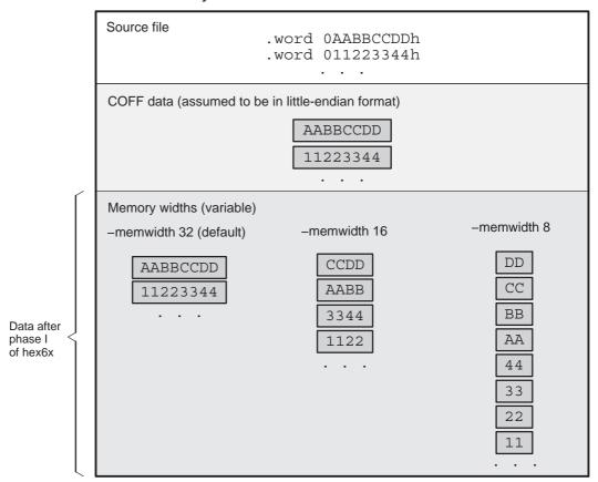
Figure 11–3. COFF Data and Memory Widths
