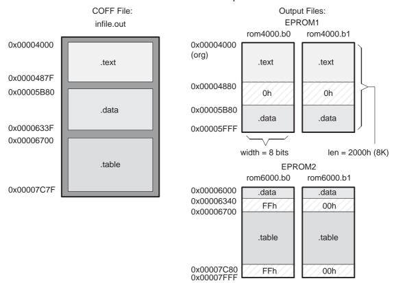
The map file (specified with the –map option) is advantageous when you use the ROMS directive with multiple ranges. The map file shows each range, its parameters, names of associated output files, and a list of contents (section names and fill values) broken down by address. Example 11–2 is a segment of the map file resulting from the example in Example 11–1.
