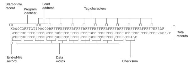
If any data fields appear before the first address, the first field is assigned address 0000h. Address fields may be expressed for any data byte, but none is required. The checksum field, which is preceded by the tag character 7, is the 2s complement of the sum of the 8-bit ASCII values of characters, beginning with the first tag character and ending with the checksum tag character (7 or 8). The end-of-file record is a colon (:).
