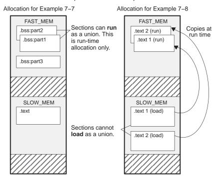
Figure 7–4. Memory Allocation Shown in Example 7–7 and Example 7–8
