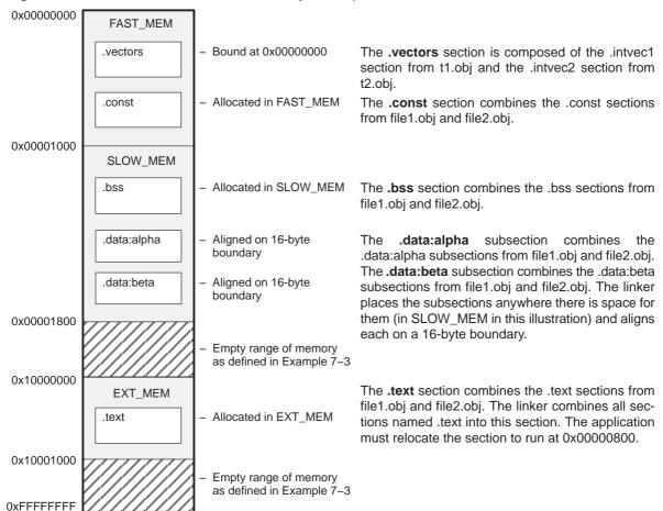
Figure 7–2. Section Allocation Defined by Example 7–4
