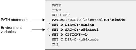
(a) Sample autoexec.bat file to use with the debugger and simulator
