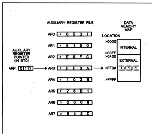
Figure 5. Example of indirect auxiliary register addressing.
