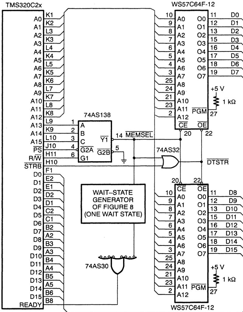
Figure 15. Interface Timing of the WS57C64F-12 to the TMS320C2x
