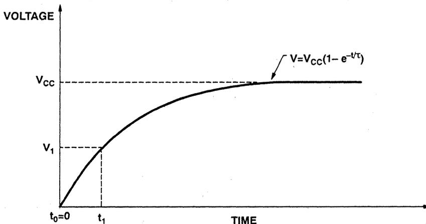
The duration of the low pulse on the reset pin is approximately  $t_1$ , which is the time it takes for the capacitor  $C_1$  to fully charge; i.e., 1.5 V. This is approximately the voltage at which the reset input switches from a logic level 0 to a logic level 1. The capacitor's voltage is given by
