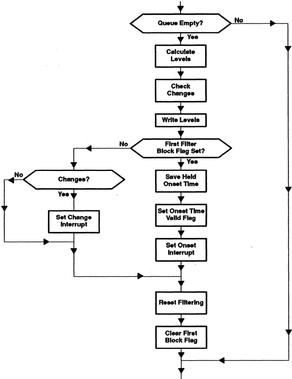
Figure 12. Tone Receiver Flow Chart—End of Filter Block
