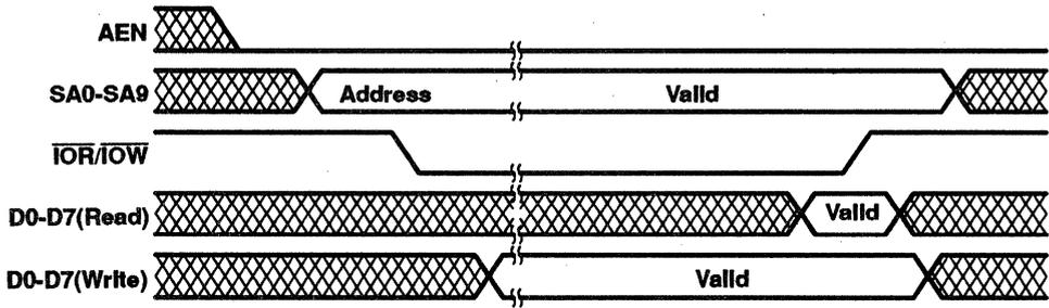
Figure 18. PC Bus Activity I/O Read or Write
