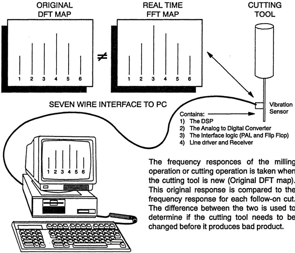
Within the PC is an interface board that has the TMS370C010 on it. The TMS370 holds the original map in EEPROM and compares it to each follow-on DFT map.
