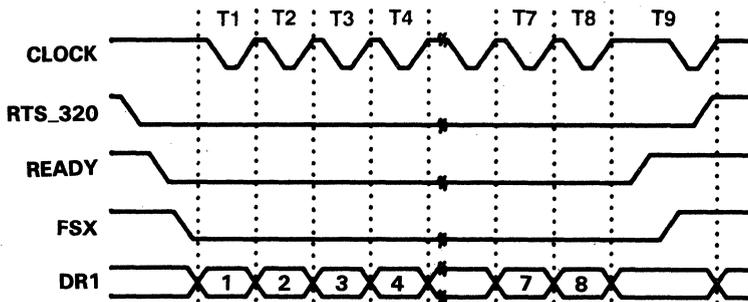
**Figure 9. Timing Diagram for TMS320C17/E17 to TMS370C010 Transmission**
