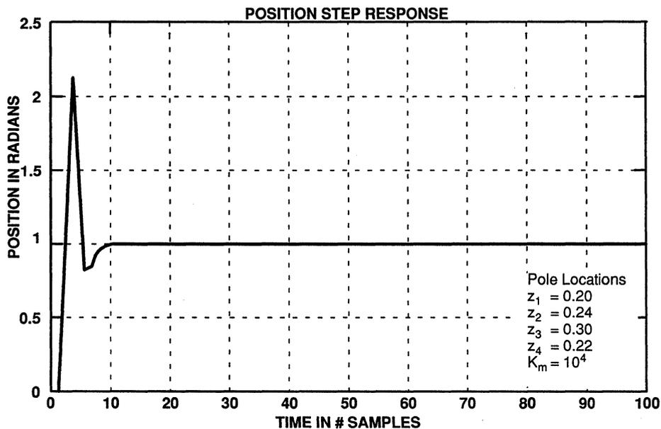
Figure 11. PID Controller Step Response for System's Third Pole Locations
