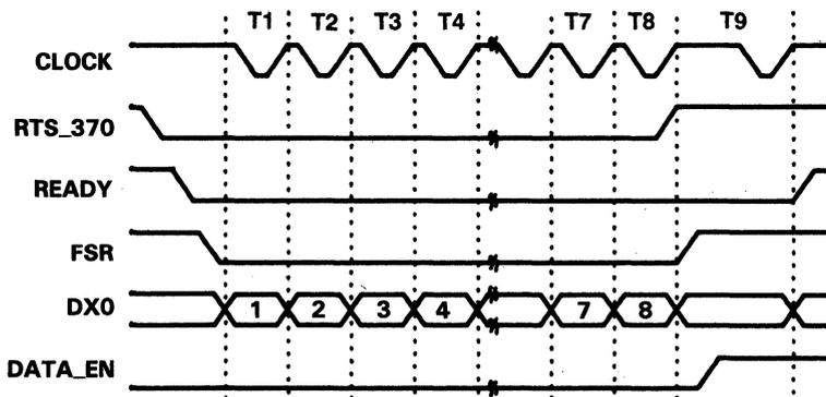
**Figure 8. Timing Diagram for TMS370C010 to TMS320C17/E17 Transmission**
