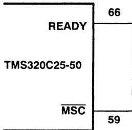
Similarly,  $\overline{MSC}$  and the  $\overline{PS}$ ,  $\overline{DS}$ , and  $\overline{IS}$  signals can be used to generate wait-state mixes such as that resulting from the circuit in Figure 3. With this circuit, all program space accesses are one wait-state accesses while all data space and I/O accesses occur at full speed.
