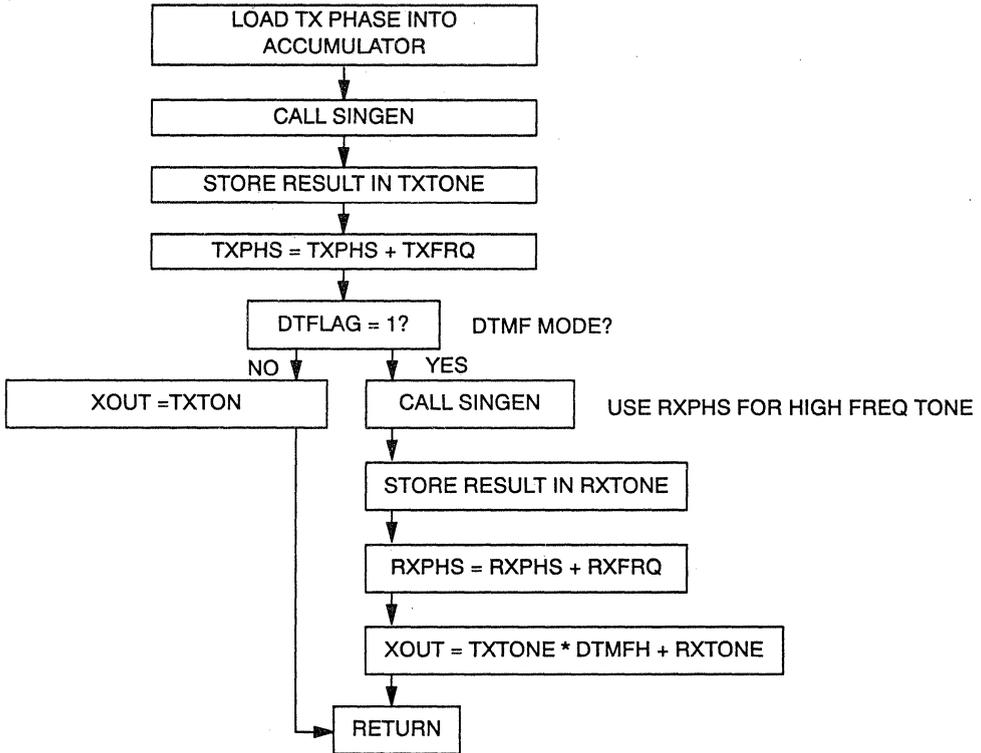
**Figure 6. Flowchart of Subroutine FSKTX**
