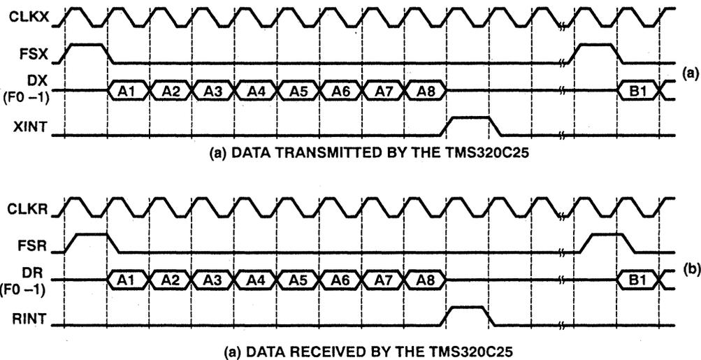
As indicated in Figure 29, both the transmit and receive operations are initiated by a framing pulse on the FSX and FSR pins of the TMS320C2x and the codec. The receive and transmit interrupts shown in Figure 29 occur only if they are enabled. Note that Figure 29 corresponds to the burst-mode serial port operation of the TMS320C2x.[1] Continuous-mode operation using framing pulses or without framing pulses is also available.
