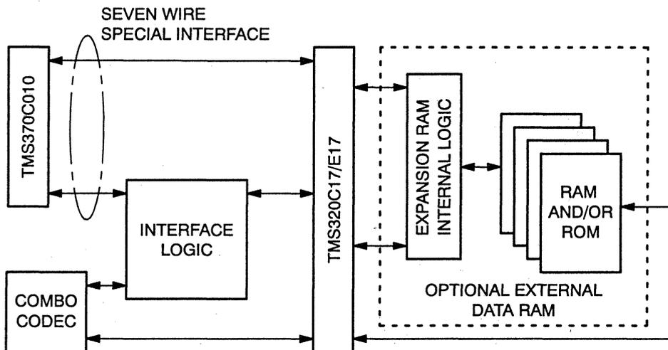
**Figure 1. Block Diagram of TMS320C17/E17/TMS370C010 System**
