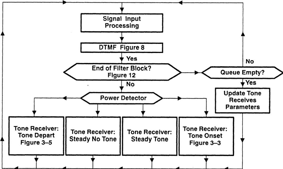
**Figure 4. Tone Detector Flow Chart - Top Level**
