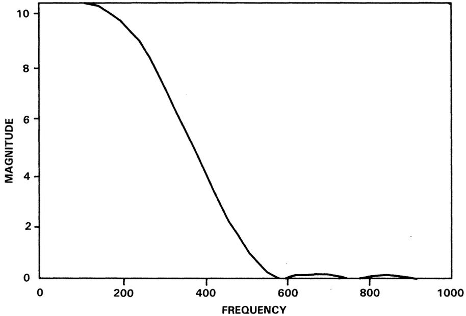
**Figure 13. Frequency Response Characteristics of Transmit Lowpass Filters**
