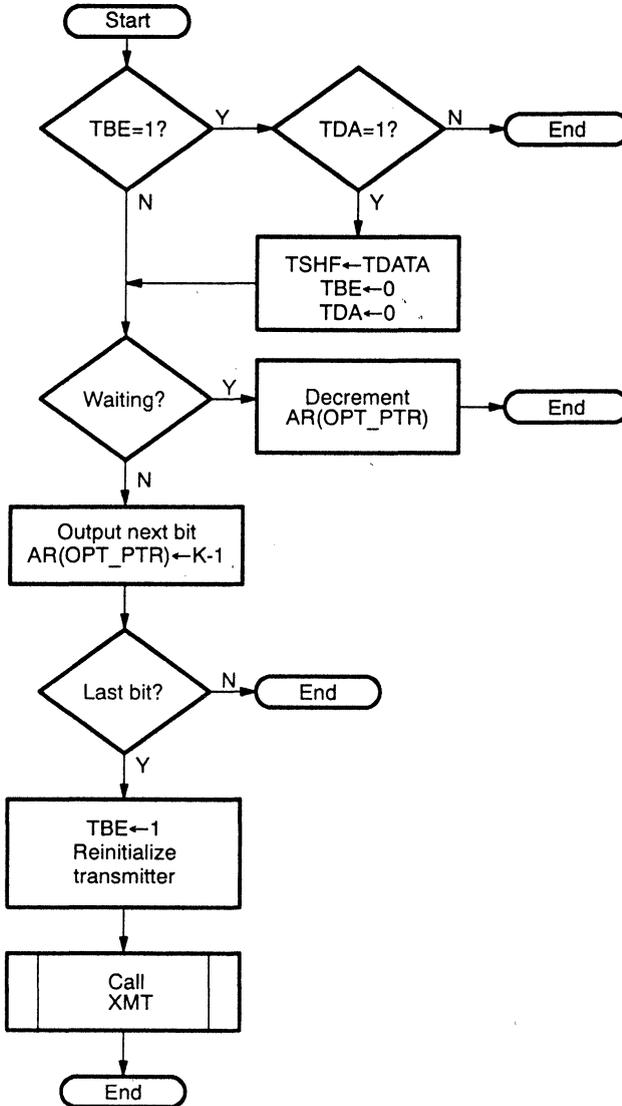
Figure 4. Transmitter Routine
