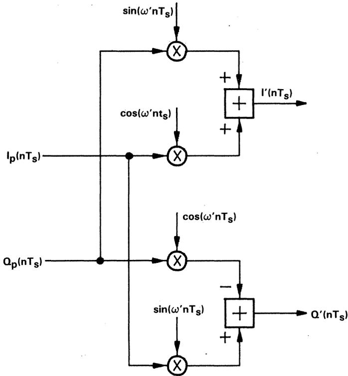
**Figure 6. Demodulator Structure**
