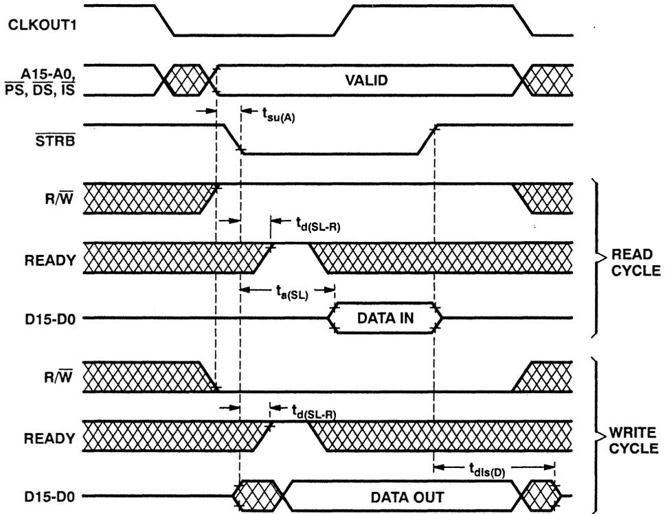
A timing requirement of special interest is the memory access time measured from the falling edge of  $\overline{\text{STRB}}$ . The specification of this requirement is jointly implied by the device  $t_{a(A)}$  and  $t_{\text{su(D)R}}$  specifications as shown in the following.
