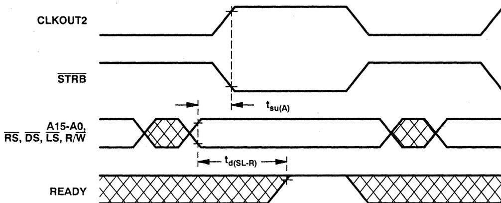
READY (see Figure 1) must be valid no later than  $t_{su(A)} + t_{d(SL-R)}$  after the address bus and interface control signals (except STRB) become valid. This evaluates to
