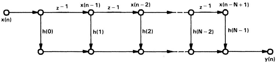
**Figure 14. Signal Flowgraph of the FIR Filter Structure**
