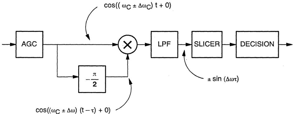
**Figure 8. FSK Demodulator**
