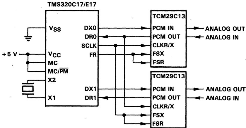
Figure 4. Simple TMS320C17/E17/CODEC Interface
