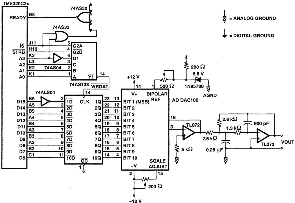
This design consists of three sections: the interface to the TMS320C2x, the D/A converter, and the smoothing filter. Each of these sections is considered separately.
