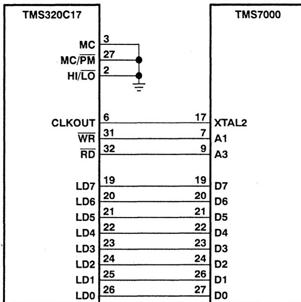
**Figure 25. TMS320C17 to 8-Bit Microcomputer (TMS7000) Interface**
