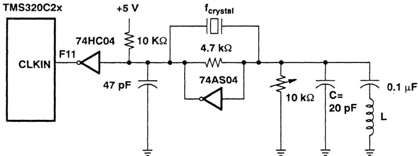
The 74AS04 inverter in Figure 26 provides the 180-degree phase shift that a parallel oscillator requires. The 4.7-kΩ resistor provides the negative feedback that keeps the oscillator in a stable
