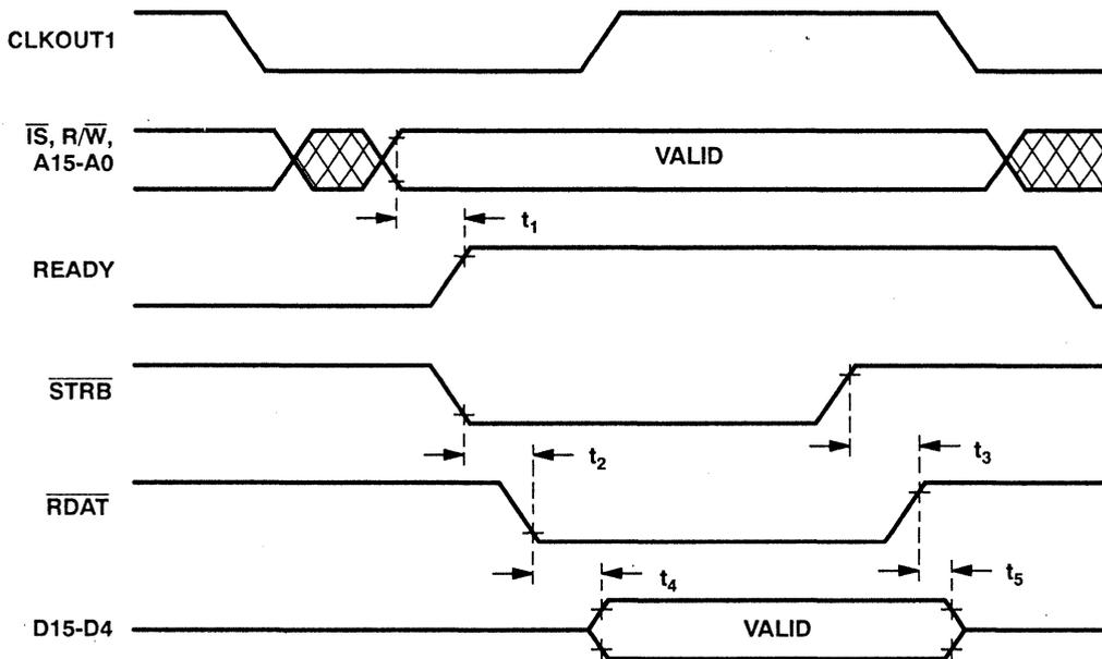
Time  $t_1$  in Figure 31 indicates the time from valid address to READY high. This is less than 10.8 ns, the maximum propagation delay through the READY generation logic. Therefore, the 18-ns READY timing requirement (at 40 MHz) is met.
