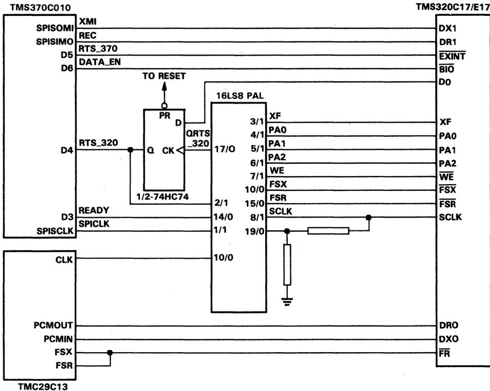
**Figure 11. Serial Interface with CODEC**
