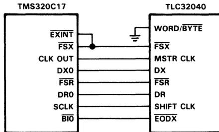
Figure 4-1. AIC Interface to TMS320C17
