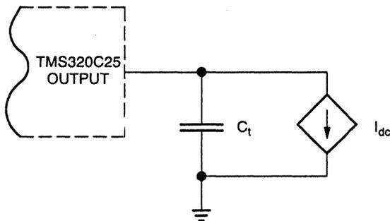
An equivalent load connected to each device output during the TMS320C25  $I_{CC}$  measurement is shown in Figure 5. Note that when the output is high, the device sources  $(V_{OH} - 2.15)/825 = 303 \mu\text{A}$  at  $V_{OH} = 2.4 \text{ V}$ . The device sinks  $(2.15 - V_{OL})/825 = 2.12 \text{ mA}$  at  $V_{OL} = 0.4 \text{ V}$  when the output is low. When the output is switching, the output buffer drives  $100 \text{ pF}$  of capacitance in addition to the resistor current.
