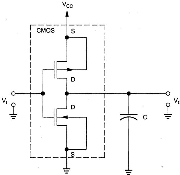
If the input voltage is fixed at a logic high or logic low level, one of the two inverter transistors will be non-conducting (off) while the other has a highly conductive channel (on). Under this condition, the supply current is equal to the negligibly small P-N junction leakage current through the off device.
