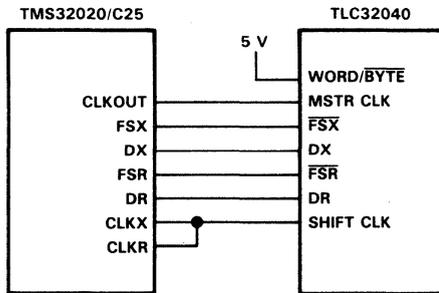
Figure 3-1. AIC Interface to TMS32020/C25
