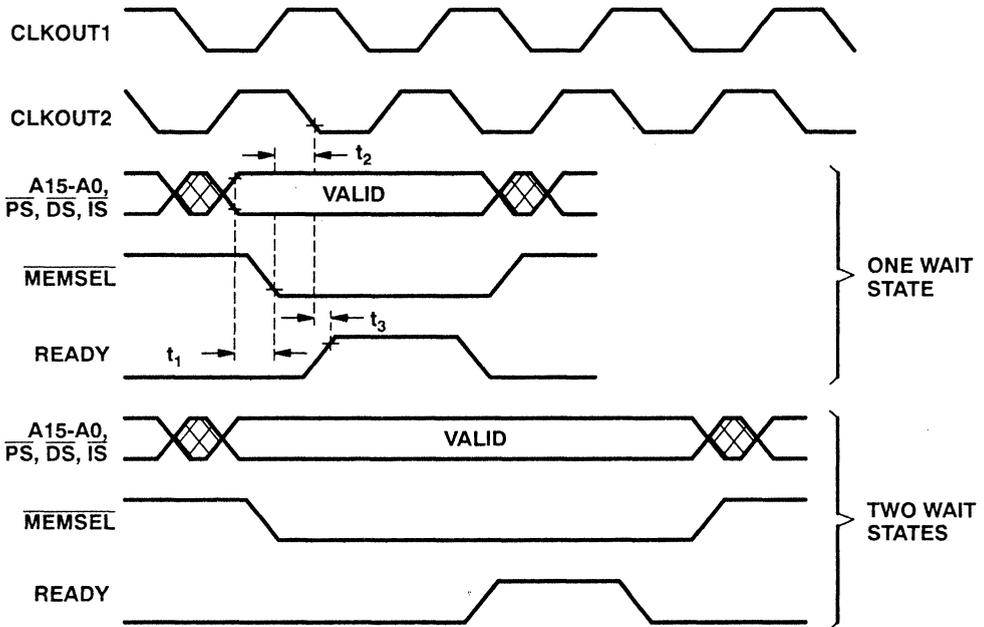
With this arrangement, READY is driven by a multiple-input NAND gate. This can be a standard gate such as a 74AS30 or can be part of the logic implemented by a high-speed programmable logic device. The output of this gate is low unless at least one of the inputs is low. The propagation delay of READY decode logic selecting zero wait-state devices in addition to the NAND delay
