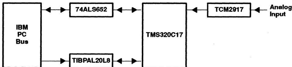
**Figure 6. PC Tone Detector Circuit Diagram—Block Level**
