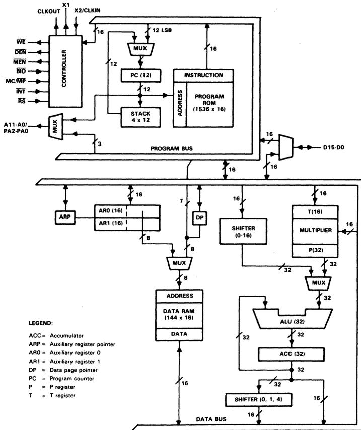
Fig. 4. TMS320C10 functional block diagram.
