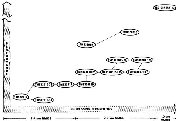
Fig. 1. The TMS320 family of digital signal processors.
