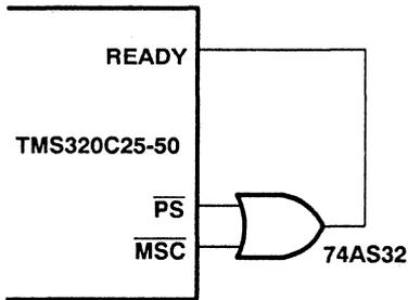
Applications having sufficiently simple address partitioning can make use of one or more levels of standard logic gates to generate READY. The circuit shown in Figure 4 has the following wait-state map:
