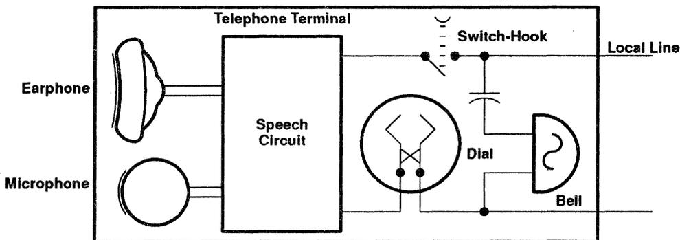
**Figure 1. Pulse Dialing Telephone**
