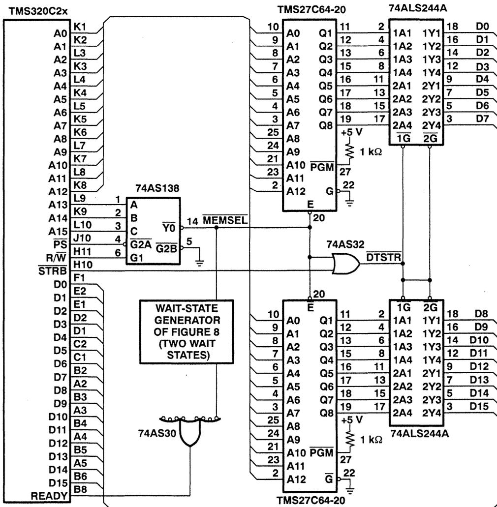
Figure 17. Interface Timing of the TMS27C64-20 to the TMS320C2x
