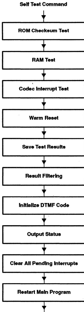
**Figure 14. Tone Receiver Flow Chart - Self Test**
