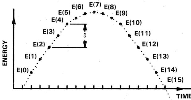
**Figure 20. Signal Energy Samples over a Baud**
