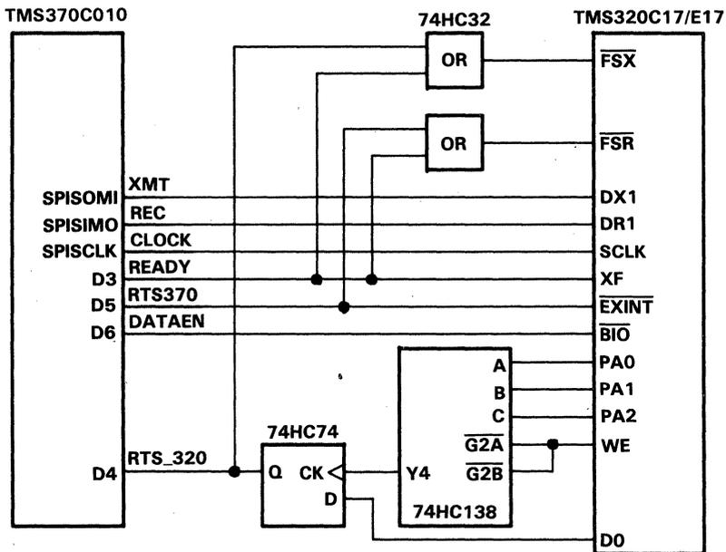
Figure 5. Stand-Alone TMS320C17/E17/TMS370 Serial Interface
