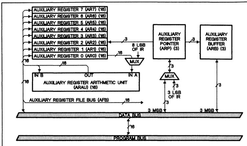
Figure 3. Auxiliary register file.
