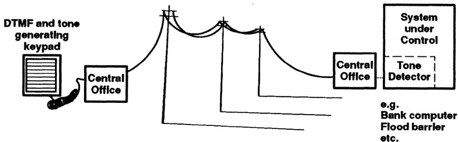
**Figure 23. Secure Remote Controller**
