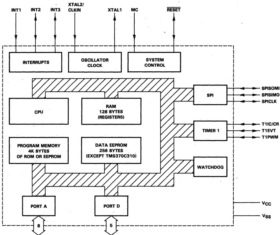
Figure 6. TMS370C010 Block Diagram
