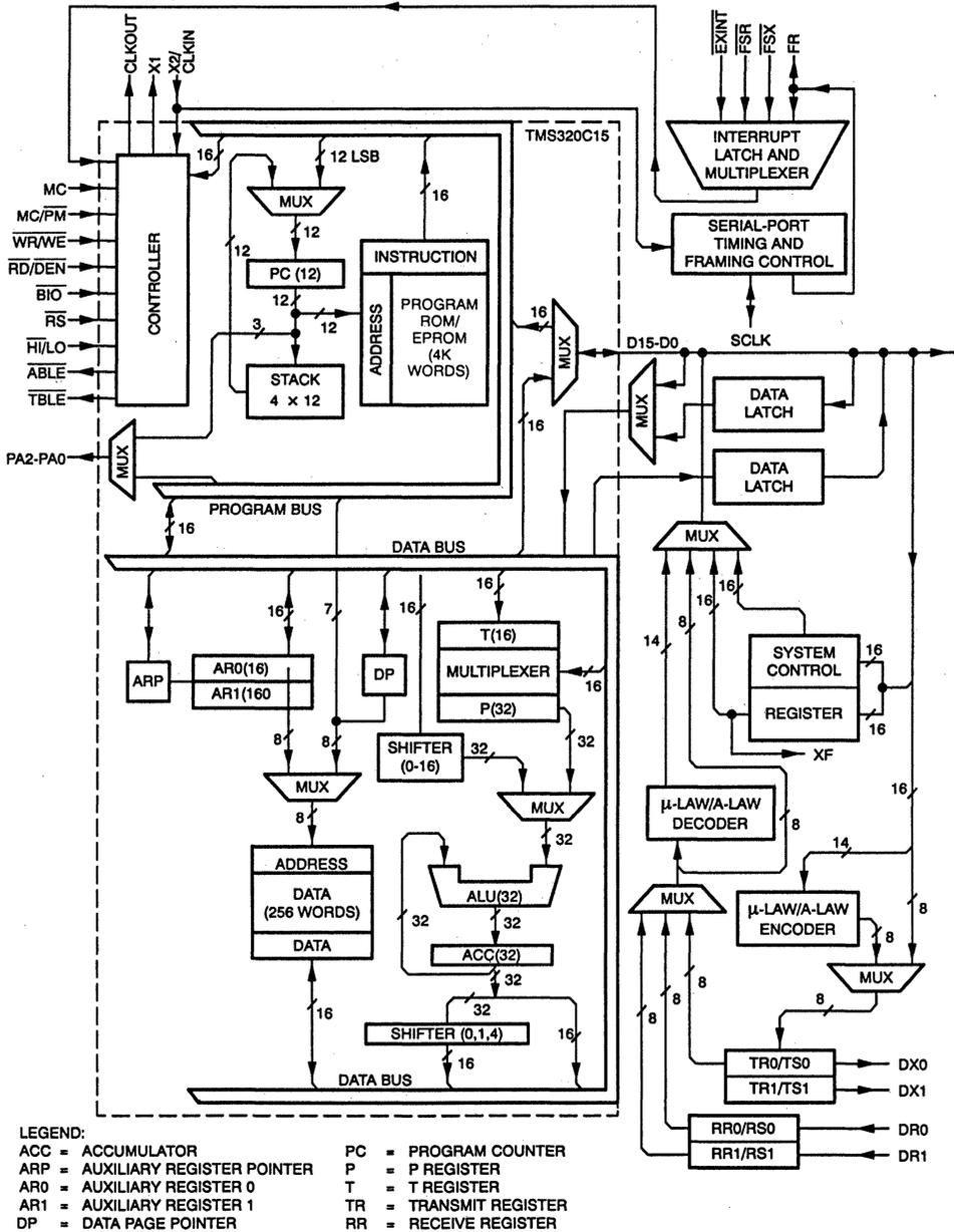
Figure 2. TMS320C17/E17 Block Diagram
