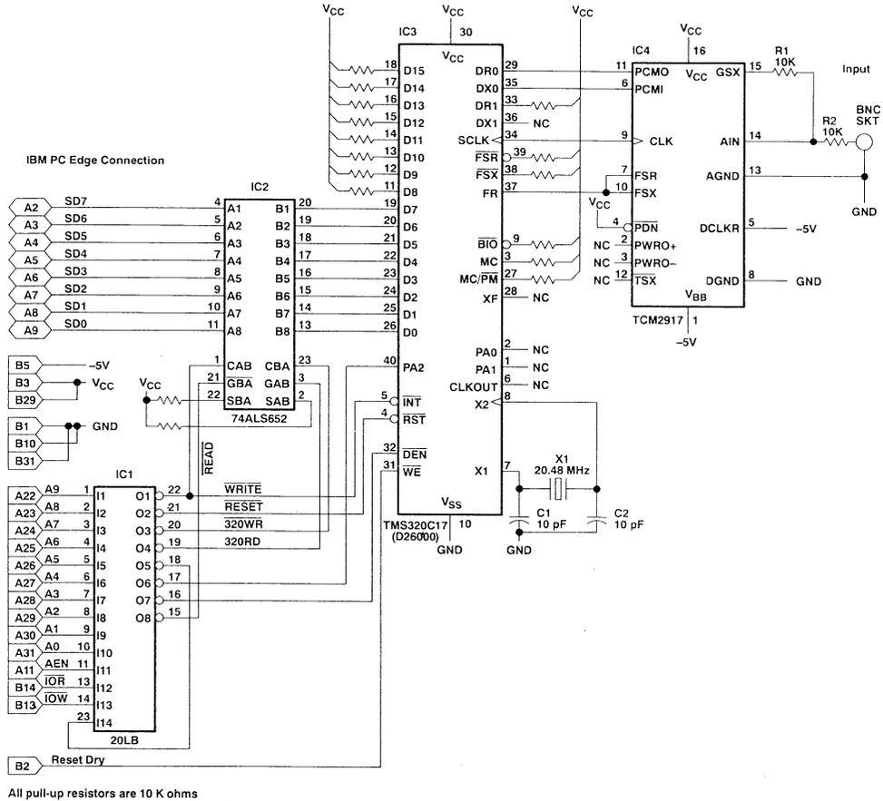
Figure 17. Tone Detector PC Application Circuit Diagram
