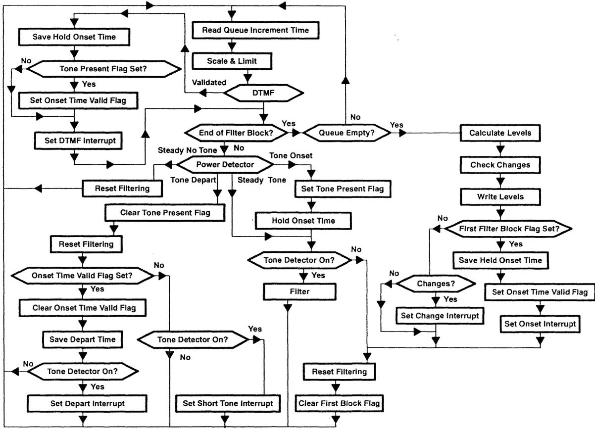
Figure 15. Tone Detector Flow Chart (Detailed)
