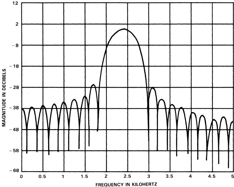
**Figure 15. Frequency Response of Receiver Bandpass Filters**
