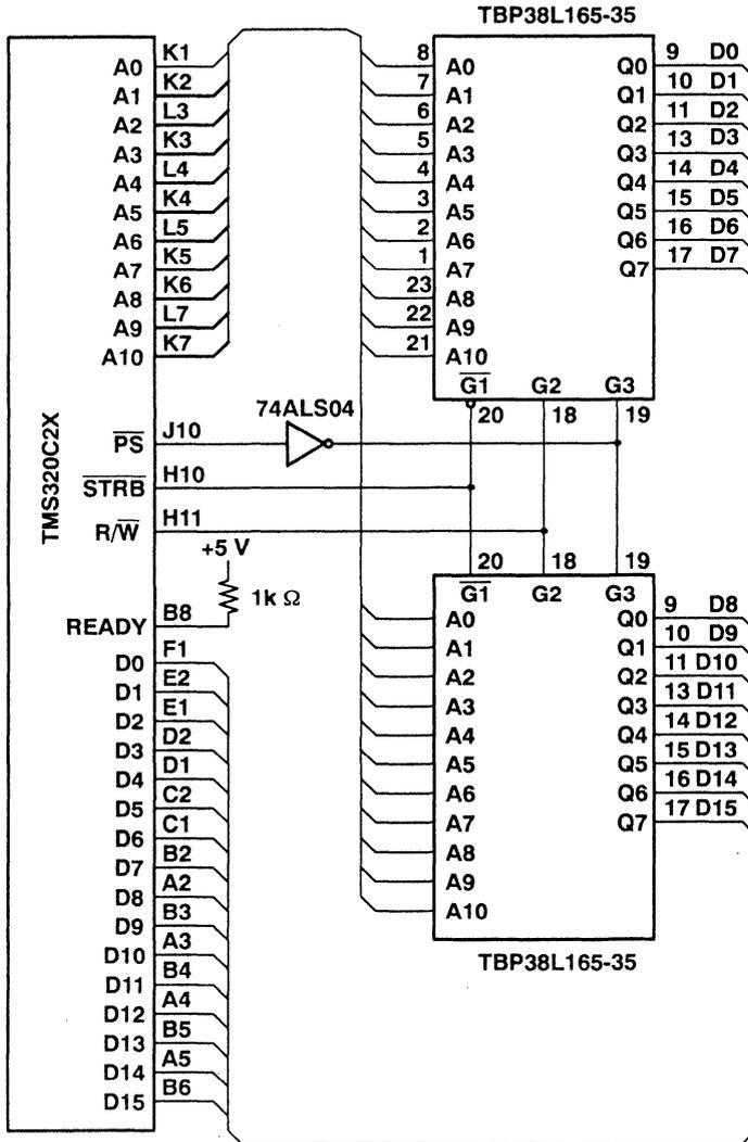
Figure 9. Interface Timing of the TBP38L165-35 to the TMS320C2x
