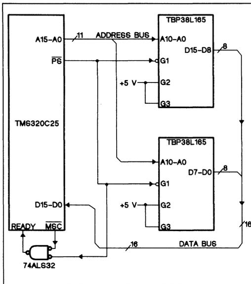
Figure 6. Minimal configuration for external program memory.
