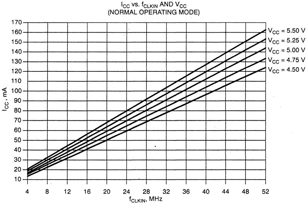
For a fixed value of supply voltage  $V_{CC0}$ ,  $I_{CC}$  increases linearly with the frequency of the CLKIN signal with a slope  $m$  given by
