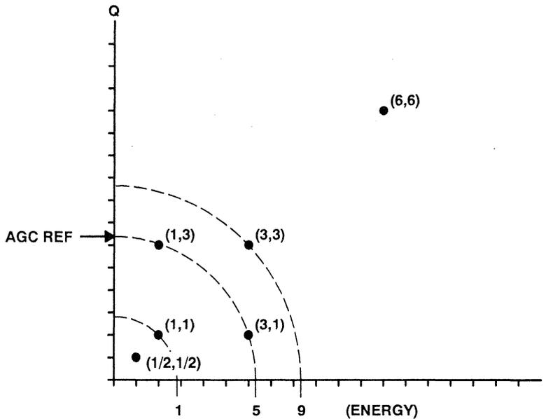
In Figure 3, constellation points (3,3) and (1,1) with respective energy contents of 9 and 1 lie outside the reference level of 5. A window function is then necessary so that the AGC does not treat these energy variations around the nominal energy as distortions induced by the communication channel.
