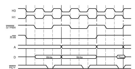
Figure 10–24. Write-Write-Read Sequence for STRBx Active
