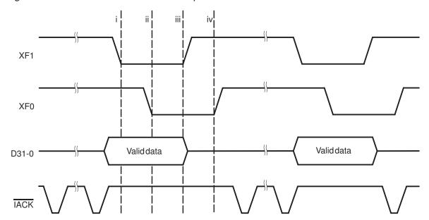
Figure 11-7. Handshake Data-Transfer Operation
