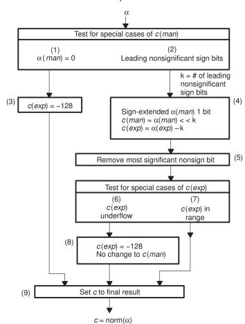
Figure 5–18. Flowchart for NORM Instruction Operation
