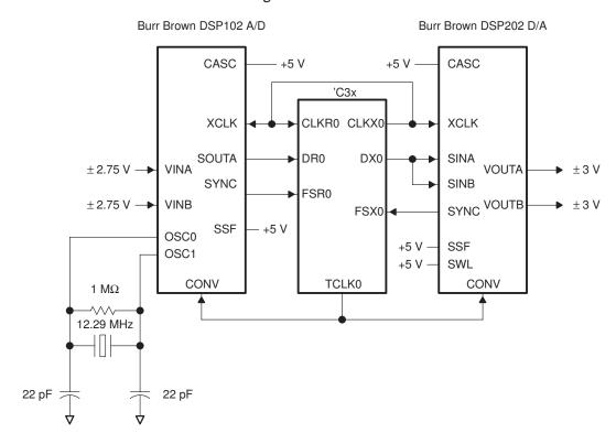
The DSP102 A/D is interfaced to the 'C3x serial-port receive side; the DSP202 D/A is interfaced to the transmit side. The A/Ds and D/As are hard-wired to run in cascade mode. In this mode, when the 'C3x initiates a convert command to the A/D via the TCLK0 pin, both analog inputs are converted into two 16-bit words, which are concatenated to form one 32-bit word.
