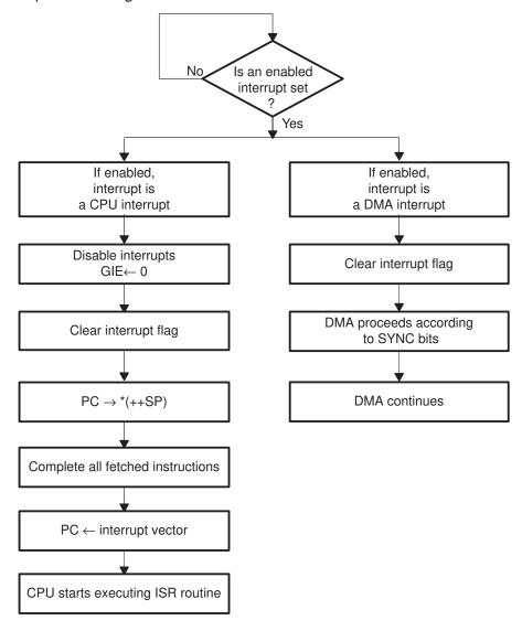
Figure 7-6. CPU Interrupt Processing
