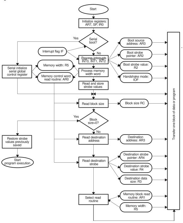
Figure C-1. Boot-Loader Flow Chart
