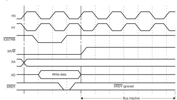
Figure 9–24. Inactive Bus States for IOSTRB
