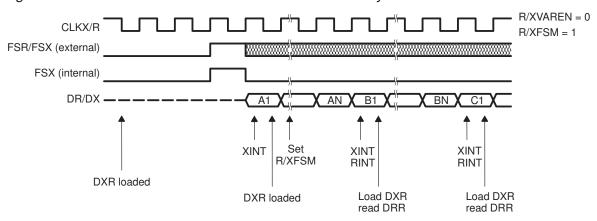
The timing of RINT and XINT and data transfers to and from DXR and DRR, respectively, are the same as in fixed data-rate standard mode with back-to-back frame syncs. This mode of operation also exhibits the same delay of 2.5 CLKX cycles after DXR is loaded before an internal FSX is generated. As in the case of continuous operation in fixed data-rate mode with frame sync, you must reload DXR no later than transmission of the N-3 bit.
