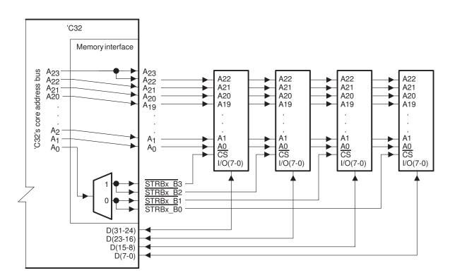
Figure 10–12. Functional Diagram for 16-Bit Data-Type Size and 32-Bit External-Memory Width
