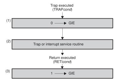
The **RETIcond** instruction manipulates the status flags as shown in block (3) in Figure 7–10. RETI*cond* provides a return from a trap or interrupt.
