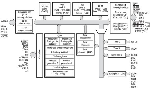
Figure 1–1. TMS320C3x Devices Block Diagram
