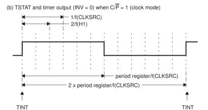
The timer signaling is determined by the frequency of the timer input clock and the period register. The following equations are valid with either an internal or an external timer clock:
