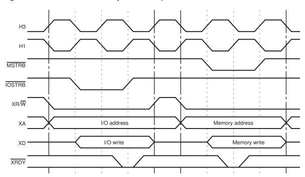
Figure 9–17. I/O Write and Memory Write for Expansion Bus
