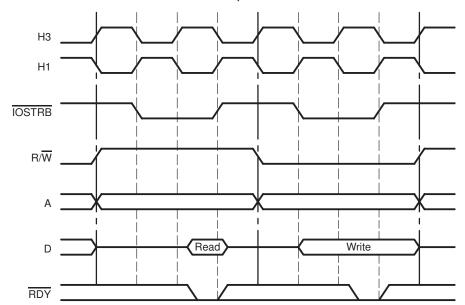
Figure 10–27. Zero Wait-State Read and Write Sequence for IOSTRB Active
