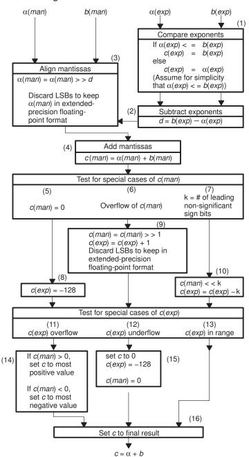
Figure 5-17. Flowchart for Floating-Point Addition
