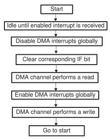
Figure 12-44. Mechanism for DMA Source Synchronization
