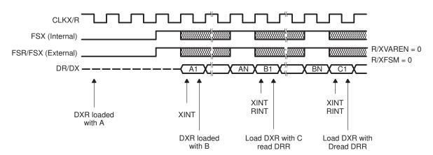
Figure 12–27. Fixed Standard Mode With Back-to-Back Frame Sync
