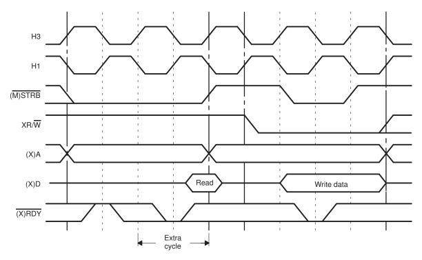
Figure 9–9 illustrates a write cycle with one wait state. Since initially  $\overline{(X)RDY}=1$ , the write cycle is extended.  $\overline{(M)STRB}$ ,  $\overline{(X)R/W}$ , and  $\overline{(X)A}$  are extended one cycle. The next time  $\overline{(X)RDY}$  is sampled, it is 0.
