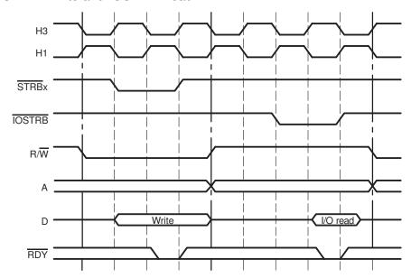
Figure 10–34 through Figure 10–37 show the transitions between  $\overline{\text{IOSTRB}}$  writes/reads and  $\overline{\text{STRBx}}$  writes/reads. In these transitions, the address changes on the rising edge of the H3 cycle.
