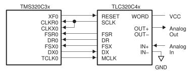
The 'C3x resets the AIC through the external pin XF0. It also generates the master clock for the AIC through the timer 0 output pin, TCLK0. (Precise selection of a sample rate may require the use of an external oscillator rather than the TCLK0 output to drive the AIC MCLK input.) In turn, the AIC generates the CLKR0 and CLKX0 shift clocks as well as the FSR0 and FSX0 frame synchronization signals.
