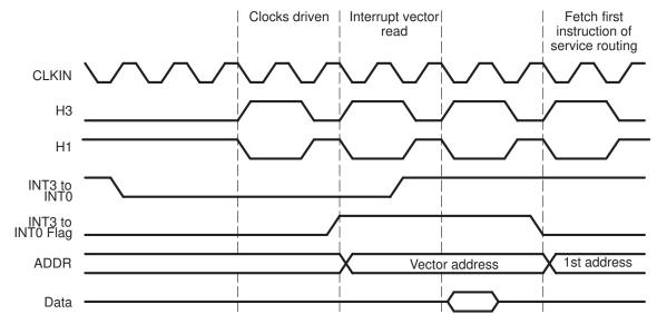
Figure 7–12. Interrupt Response Timing After IDLE2 Operation
