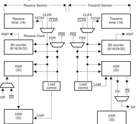
Figure 12-11. Serial Port Block Diagram
