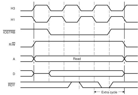
Figure 10–29. One Wait-State Write Sequence for IOSTRB Active
