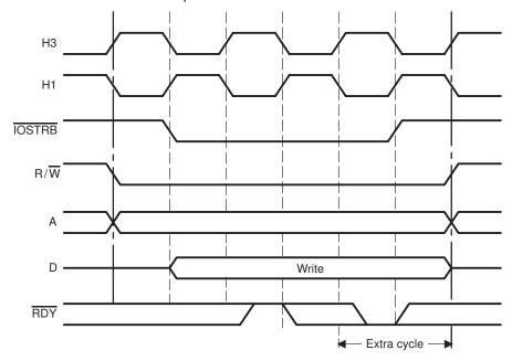
Figure 10–30 and Figure 10–31 illustrate the transitions between STRBx reads and IOSTRB writes and reads, respectively. In these transitions, the address changes on the falling edge of the H1 cycle.
