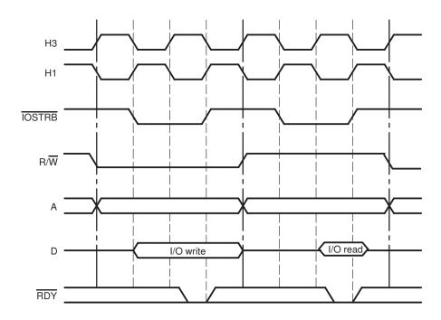
Figure 10–39. TOSTRB Write and Write
