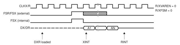
In receive operations, once a transfer is initiated, FSR is ignored until the last bit. For burst-mode transfers, FSR must be low during the last bit, or another transfer will be initiated. After a full word has been received and transferred to the DRR, an RINT is generated.
