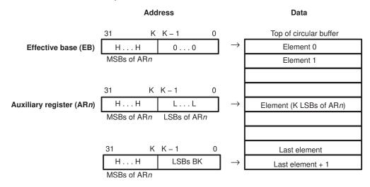
Example 6–24 shows circular addressing operation. Assuming that all ARs are four bits, let AR0 = 0000 and BK = 0110 (block size of 6). Example 6–24 shows a sequence of modifications and the resulting value of AR0. Example 6–24 also shows how the pointer steps through the circular queue with a variety of step sizes (both incrementing and decrementing).
