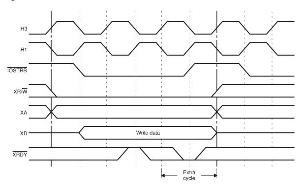
Figure 9–12. Write With One Wait State for  $\overline{IOSTRB} = 0$
