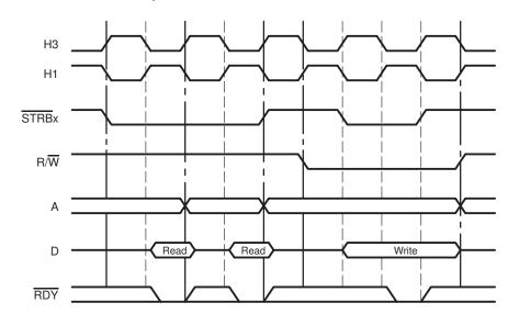
Figure 10–23. Read-Read-Write Sequence for STRBx Active
