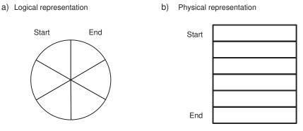
Figure 6-5. Logical and Physical Representation of Circular Buffer after Writing Three Values
