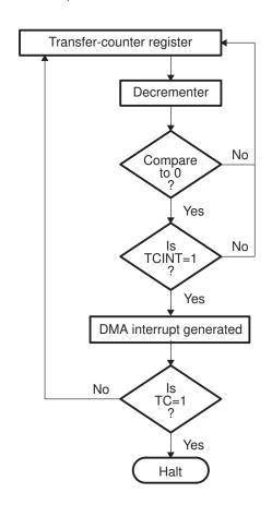
Figure 12–40. Transfer-Counter Operation
