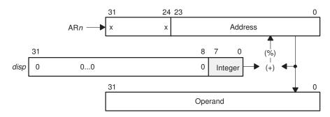
Example 6–10. Indirect Addressing With Postdisplacement Subtract and Circular Modify
