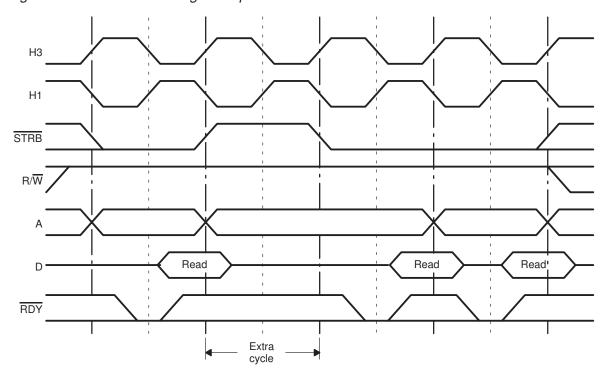
Figure 10-9. Bank-Switching Example
