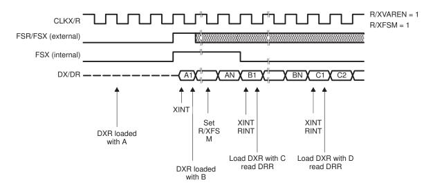
Figure 12–32. Variable Continuous Mode Without Frame Sync
