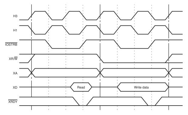
Figure 9–11 illustrates a read with one wait state when  $\overline{\text{IOSTRB}}$  is active, and Figure 9–12 illustrates a write with one wait state when  $\overline{\text{IOSTRB}}$  is active. For each wait state added,  $\overline{\text{IOSTRB}}$ , XR/ $\overline{\text{W}}$ , and XA are extended one clock cycle. Writes hold the data on the bus one additional cycle. The sampling of  $\overline{\text{XRDY}}$  is repeated each cycle.
