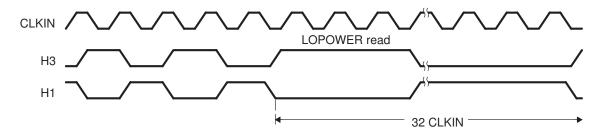
Figure 7-14. MAXSPEED Timing
