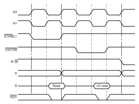
Figure 10–32 and Figure 10–33 illustrate the transitions between STRBx writes and IOSTRB writes and reads, respectively. In these transitions, the address changes on the falling edge of the H3 cycle.
