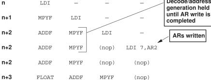
The case for reads of these groups is similar to the cases for writes. If an instruction must read a member of one of these groups, the use of that particular group by the decode for the following instruction is delayed until the read is complete. The registers are read at the start of the execute cycle and require only a one-cycle delay of the following decode. For four registers (IR0, IR1, BK, or DP), there is no delay. For all other registers, including the SP, the delay occurs.
