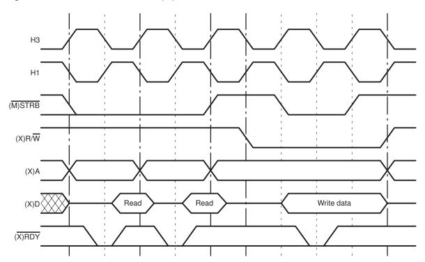
Figure 9–6. Read-Read-Write for  $(\overline{M})$ STRB = 0
