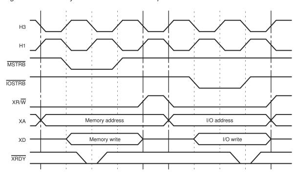
Figure 9–15. Memory Write and I/O Write for Expansion Bus
