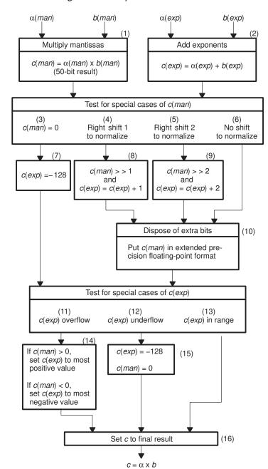
Figure 5-16. Flowchart for Floating-Point Multiplication
