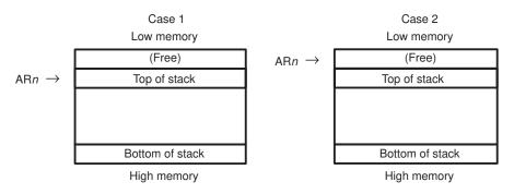
Stack growth from low-to-high memory can be implemented in two ways:
