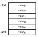
To implement a circular buffer in the 'C3x, the following criteria must be satisfied (more than one circular buffer can be implemented on the 'C3x as long as the size of the buffers are identical):
