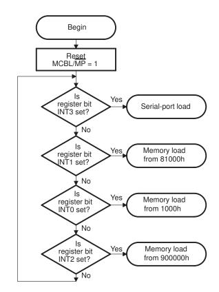
Figure 11-4.TMS320C32 Boot-Loader Mode-Selection Flowchart
