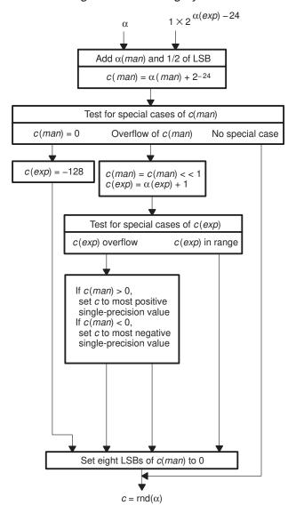
Figure 5–19. Flowchart for Floating-Point Rounding by the RND Instruction
