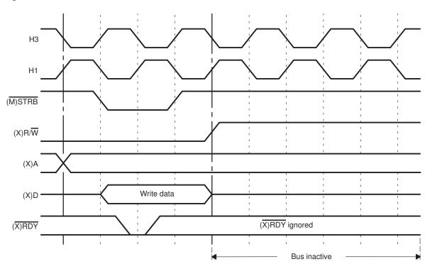
Figure 9–25. Inactive Bus States for  $\overline{STRB}$  and  $\overline{MSTRB}$
