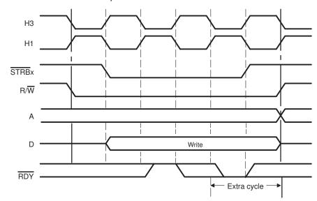
Figure 10–26. One Wait-State Write Sequence for STRBx Active
