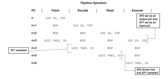
STFI and STII instructions drive the XF0 pin high during its execution phase. LDFI, LDII, and SIGI instructions sample the XF1 pin during its decode phase while driving the XF0 pin low during its read phase. Therefore, do not use an LDFI, LDII, or SIGI instruction immediately after an STFI or STII instruction (see Example 7–14).
