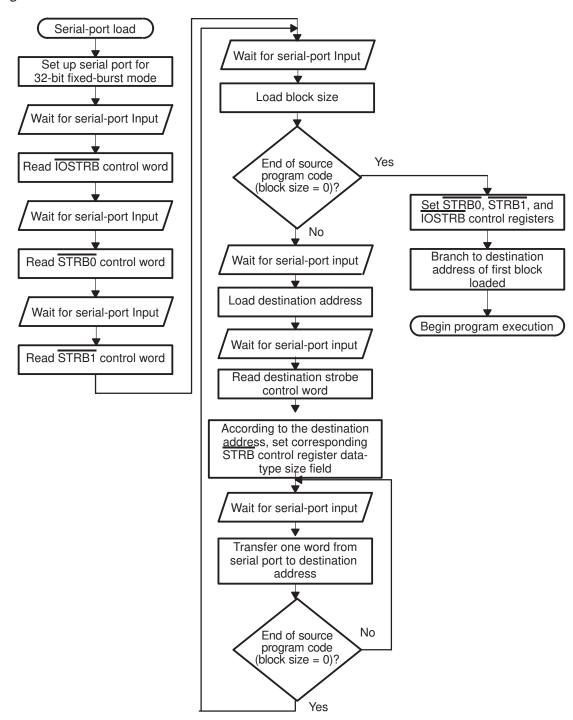
Figure 11-5.Boot-Loader Serial-Port Load Flowchart
