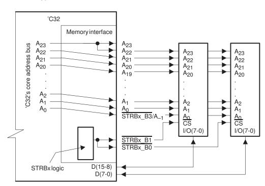
Figure 10–16. Functional Diagram for 16-Bit Data-Type Size and 16-Bit External-Memory Width
