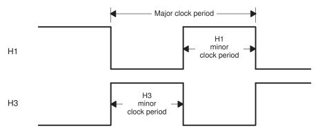
The precise operation of memory reads and writes can be defined according to these minor clock periods. The types of memory operations that can occur are program fetches, data loads and stores, and DMA accesses.
