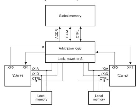
Figure 7-2. Multiple TMS320C3xs Sharing Global Memory
