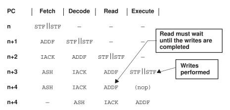
The final case involves an interlocked load (LDII or LDFI) instruction and XF1 = 1. Since the interlocked loads use the XF1 pin as an acknowledge that the read can complete, the loads might need to extend the read cycle, as shown in Example 8-10. A program refetch can occur.
