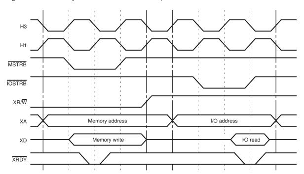
Figure 9–16. Memory Write and I/O Read for Expansion Bus
