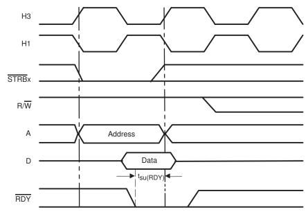
Do not change the  $\overline{RDY}$  signal during its setup time [ $^t$ su(RDY)].
