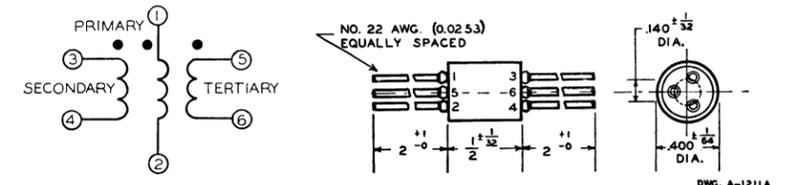
FIGURE 2—3-winding construction
