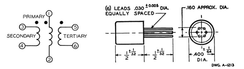
FIGURE 4—3-winding construction
