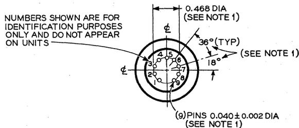
NOTE 1: TO MEET DIMENSIONAL REQUIREMENTS OF RETMA STANDARD (9) PIN MINIATURE TUBE BASE (E9-1)
