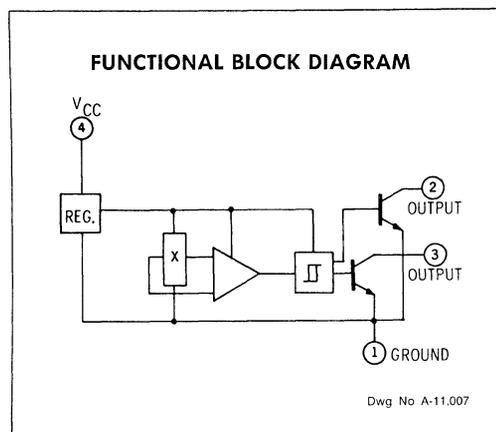
This device is supplied in a 4-pin single in-line molded package.
