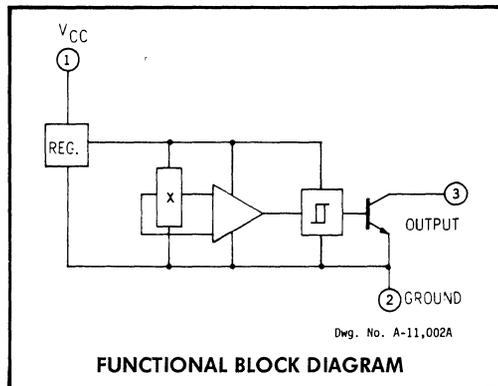
Type UGN-3076T/U is rated for operation over the temperature range of  $-20^{\circ}\text{C}$  to  $+85^{\circ}\text{C}$ . For applications in more severe environments, Type UGS-3076T/U has an operating temperature range of  $-55^{\circ}\text{C}$  to  $+125^{\circ}\text{C}$ . Both types work with supply voltages of 4.5 to 24 V.
