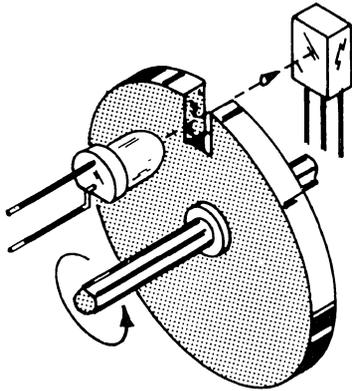
Figure 4. Shown is a commonly used speed-sensing assembly. The light field between the emitter-detector pair is interrupted by the rotating code wheel.
