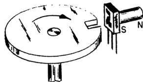
For reference only—an Alnico VIII permanent magnet, 0.212" (5.38 mm) in diameter and 0.187" (4.75 mm) long is approximately 800 gauss at the surface. A samarium cobalt permanent magnet, 0.100" (2.54 mm) square and 0.040" (1.02 mm) thick is approximately 1200 gauss at its surface.
