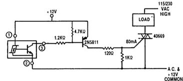
Figure 7. This circuit could be used to switch a 115 or 230 VAC load.
