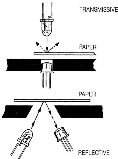
Figure 6. Sheet detector configurations using transmissive and reflective modes of operation are shown.
