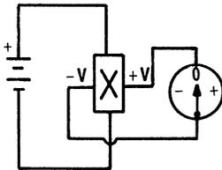
Figure 1. If no magnetic field is present, the voltage measured across the width of the semiconductor material of the Hall-effect sensor is zero.
