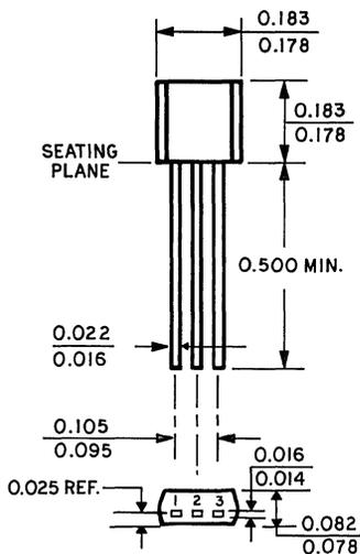
NOTE: Lead dimensions are controlled in the zone between 0.050" (0.13 mm) and 0.250" (6.35 mm) from the seating plane. Between 0.250" (6.35 mm) and 0.500" (12.7 mm) from the seating plane, a maximum lead diameter (diagonal dimension) of 0.021" (0.53 mm) is specified. Outside of these zones the lead dimensions are not controlled.
