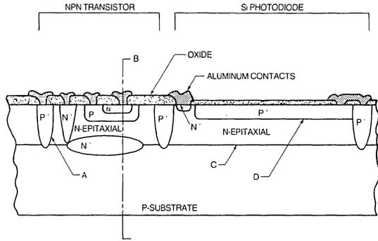
Figure 2. A cross section of a silicon IC shows a typical npn transistor and a photodiode (drawing is not to scale).
