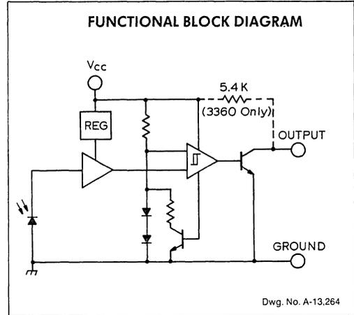
Series ULN-3330 and Series ULN-3360 switches turn ON as illumination of the photodiode falls below  $55 \mu\text{W}/\text{cm}^2$  at 880 nm. An internal latch provides hysteresis: The output turns OFF when illumination surpasses the turn-on threshold by approximately 12%.
