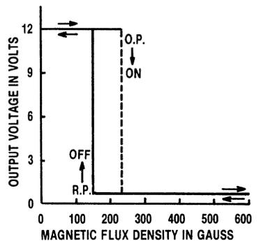
Figure 3. The transfer characteristic graph plots input on the horizontal axis vs output on the vertical axis. With no magnetic field present, the Hall-effect switch is off; as the field increases, the switch will turn on at a predesigned operating point. This particular device exhibits hysteresis of 90 gauss.
