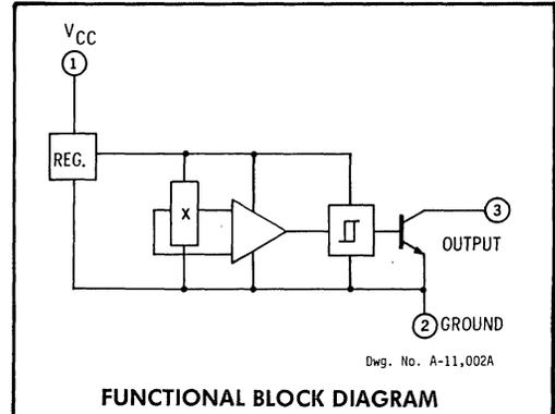
Type UGN-3075T/U is rated for operation over the temperature range of –20°C to +85°C. For applications in more severe environments, Type UGS-3075T/U has an operating temperature range of –55°C to +125°C. Both types work with supply voltages of 4.5 to 24 V.
