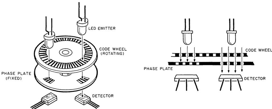
Figure 5a and b. This high-resolution rotary encoder shows the fixed phase plate along with the rotating code wheel. The two photodetectors are placed such that a light field on one device corresponds to a dark field on the other.
