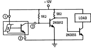
Figure 6. This circuit could be used if a load required a current of 4 A to switch.
