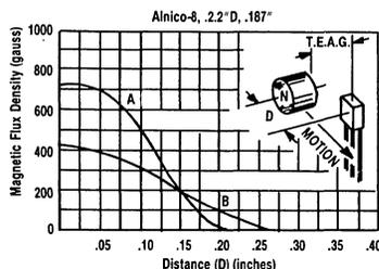
Figure 5. Hall devices must always switch on/off at the same point relative to the magnet. The effect of a change in flux density on switching distance is shown.
