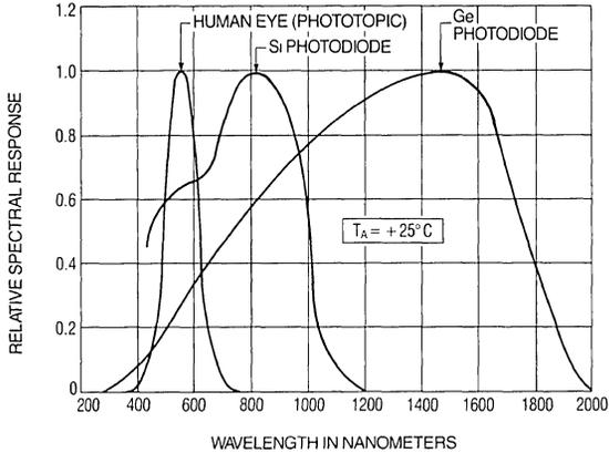
Figure 1. The CIE spectral response curve is overlaid on the spectral responsivity curves of silicon and germanium (1,3).
