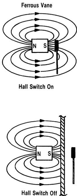
Figure 4. The ferromagnetic vane moves between the activating magnet and the Hall-effect switch shunting the flux field from the switch. These assemblies can be used for precision switching over large temperature ranges.
