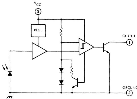
Figure 3. A functional block diagram of the Sprague ULN-3330 IC optical receiver is shown.
