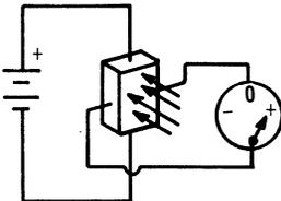
Figure 2. The output voltage of a Hall-effect sensor is directly proportional to the magnetic field present at right angles to the direction of current flow through the sensor.
