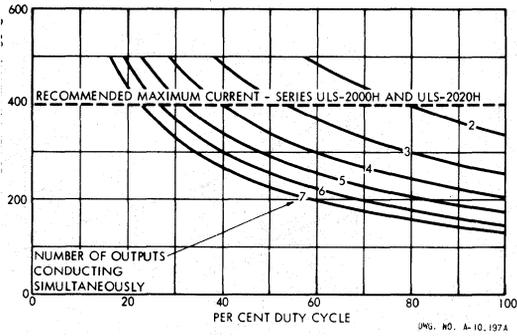
PEAK COLLECTOR CURRENT AS A FUNCTION OF DUTY CYCLE AND NUMBER OF OUTPUTS AT +50°C
