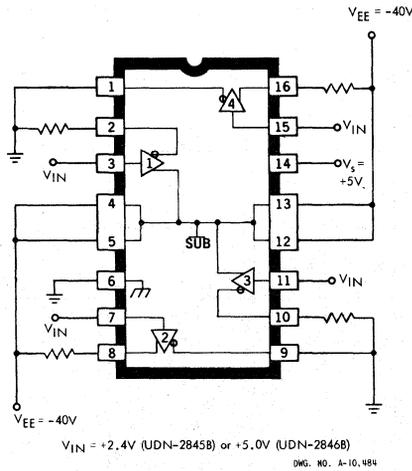
**TYPE UDN-2845B and UDN-2846B TEST CIRCUIT**
