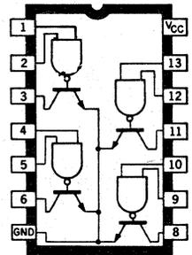
**Type UHP-402, UHP-402-1, and UHP-502 Quad 2-Input OR Power Drivers**
