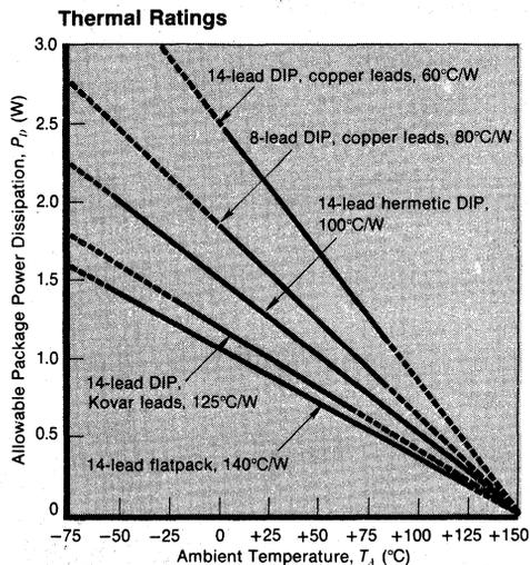
Typical thermal-resistance ratings for ICs in still air range from 60°C/W to 140°C/W. The slope of each curve on this graph is equal to the derating factor  $G_\theta$ , which is the reciprocal of thermal resistance  $R_\theta$ . For an ambient temperature of 50°C, a typical 14-lead flatpack with an  $R_\theta$  of 140°C/W can dissipate about 0.7 W. A typical DIP, however, with 14 copper-alloy leads can dissipate almost 1.7 W at 50°C.
