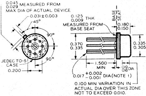
NOTE 1: THIS LEAD DIA APPLIES TO ZONE BETWEEN 0.050 AND 0.250 FROM BASE SEAT. IN ZONE BETWEEN 0.250 AND 1.500, A MAX OF 0.021 DIA IS HELD. OUTSIDE OF THESE ZONES, THE LEAD DIA IS NOT CONTROLLED.
