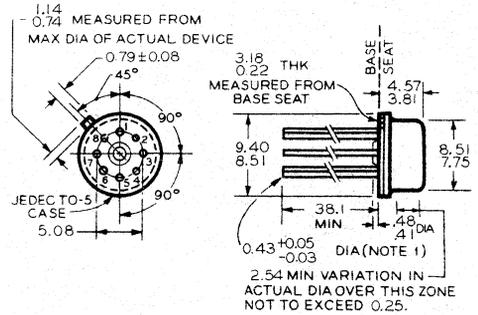
NOTE 1: THIS LEAD DIA APPLIES TO ZONE BETWEEN 1.27 AND 6.35 FROM BASE SEAT. IN ZONE BETWEEN 6.35 AND 38.1, A MAX OF 0.53 DIA IS HELD. OUTSIDE OF THESE ZONES, THE LEAD DIA IS NOT CONTROLLED.
