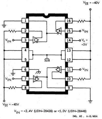
**TYPE UDN-2843B and UDN-2844B TEST CIRCUIT**
