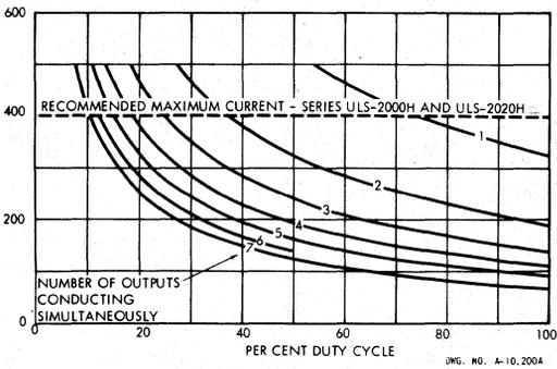
PEAK COLLECTOR CURRENT AS A FUNCTION OF DUTY CYCLE AND NUMBER OF OUTPUTS AT +100°C
