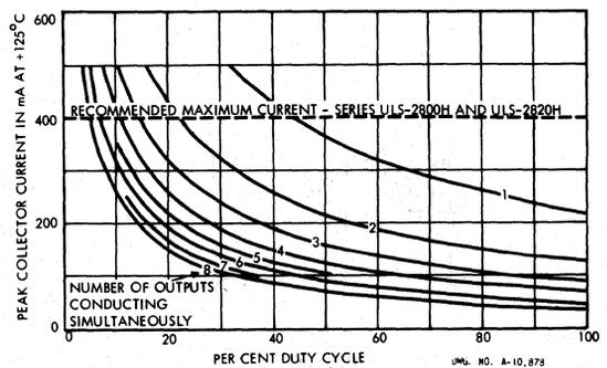
**PEAK COLLECTOR CURRENT AS A FUNCTION OF DUTY CYCLE AND NUMBER OF OUTPUTS AT +125°C**
