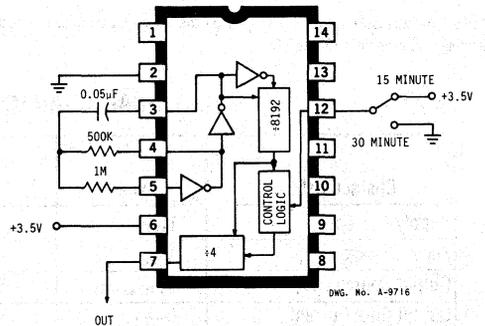
TYPICAL APPLICATION ( $f_{IN} \approx 18.2\text{Hz}$ )
