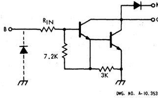
ULN-2064B }  $R_{IN} = 350\Omega$
