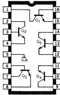
JEDEC style MO-001AC. The Type ULS-2083H is electrically identical to the ULN-2083A but is supplied in a hermetic dual in-line package for operation over the temperature range of -55°C to +125°C. This package conforms to the dimensional requirements of Military Specification MIL-M-38510 and can meet all of the applicable environmental requirements of Military Standard MIL-STD-883.
