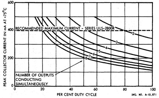
PEAK COLLECTOR CURRENT AS A FUNCTION OF DUTY CYCLE AND NUMBER OF OUTPUTS AT +75°C
