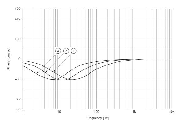
Fig. 5-26b. Servo LowBooster1 characteristics [FCS, TRK] (MCK = 128Fs)
