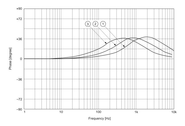
Fig. 5-26a. Servo HighBooster characteristics [FCS, TRK] (MCK = 128Fs)
