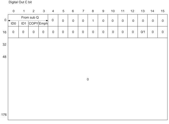
bits0 to 3 Sub-Q control bits that matched twice with CRCOK bit29 VPON: 1 X'tal: 0
