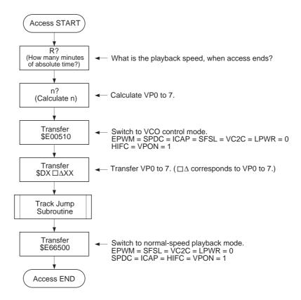
Fig. 3-3. Access Flow Chart Using VCO Control
