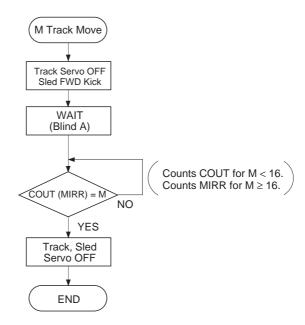
Fig. 4-13-(a). M-Track Move Flow Chart
