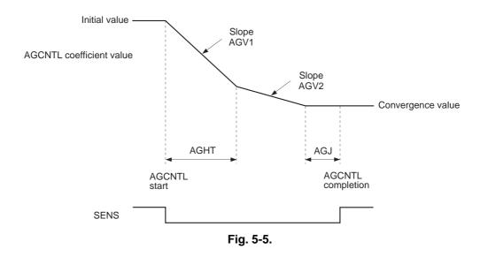
**Note)** Fig. 5-5 shows the case where the AGCNTL coefficient converges from the initial value to a smaller value.
