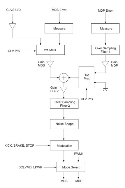
CLVS U/D: Up/down signal from CLVS servo
