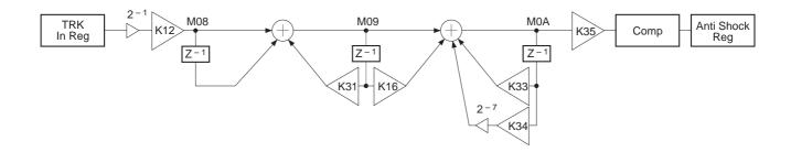
Note) Set the MSB bit of the K34 coefficient to 0.
