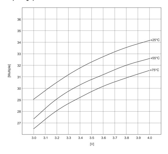
The Maximum Operating Speed graph shows the playback speed Vod (min.) at various temperatures. The playback conditions are that the high-speed VCO1 selects No.4 and VCO2 selects high speed in CAV-W
