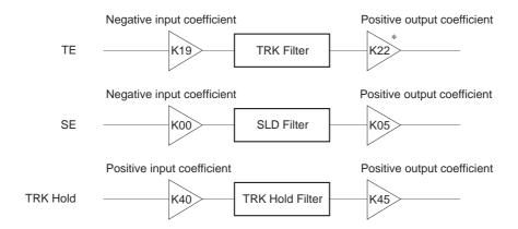
When SFID = 1, the TRK filter negative input coefficient is applied to the SLD filter, so the SLD input coefficient (K00) sign must be inverted. (For example, inverting the sign for coefficient K00: E0h results in 60h.) For the same reason, when THID = 1, the TRK hold input coefficient (K40) sign must be inverted.
