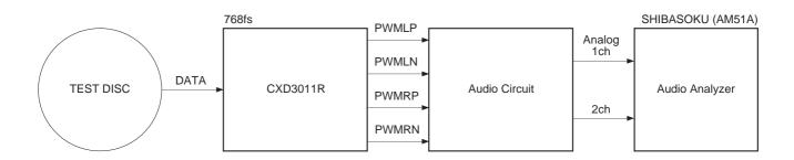
Block diagram of analog characteristics measurement
