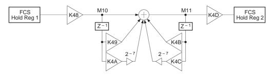
Note) Set the MSB bit of the K4A and K4C coefficients to 0.
