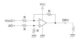
Fig. 5-23. Drive Circuit
