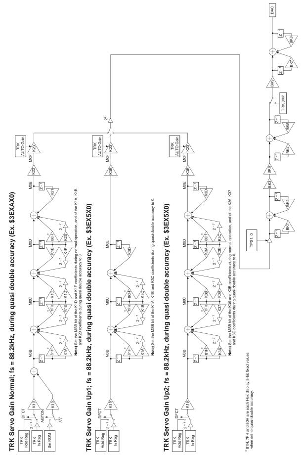
Note) Set SFJP (\$36) to 1 or TAOZ (\$34D) to 0 in order to boost the low frequency for the TRK Jump operation.
