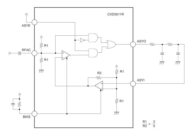
Fig. 4-16. Asymmetry Compensation Application Circuit
