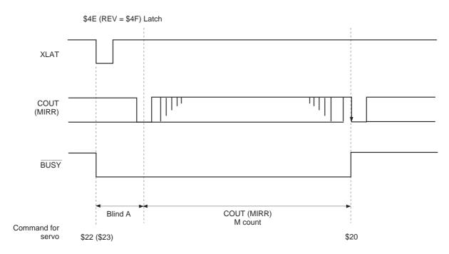
Fig. 4-13-(b). M-Track Move Timing Chart
