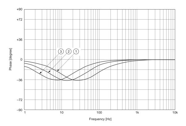
Fig. 5-26c. Servo LowBooster2 characteristics [FCS, TRK] (MCK = 128Fs)
