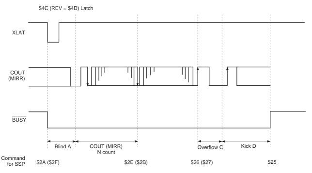
Fig. 4-11-(b). 2N-Track Jump Timing Chart
