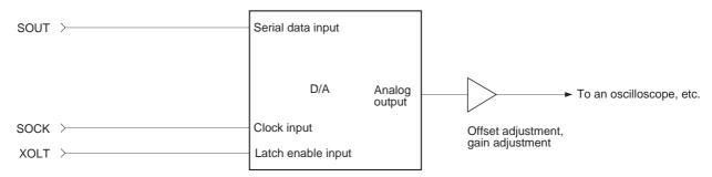
Waveforms can be monitored with an oscilloscope using a serial input-type D/A converter as shown above.
