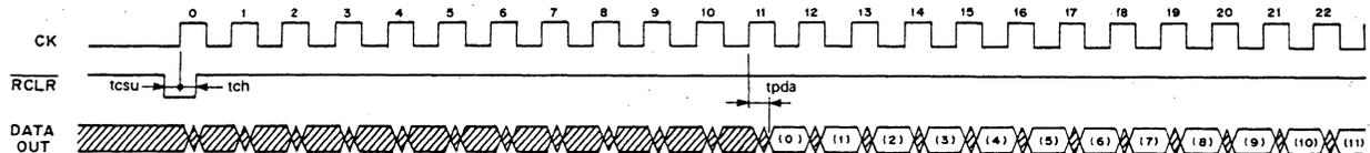
Fig. 7 The data read OUT timing
