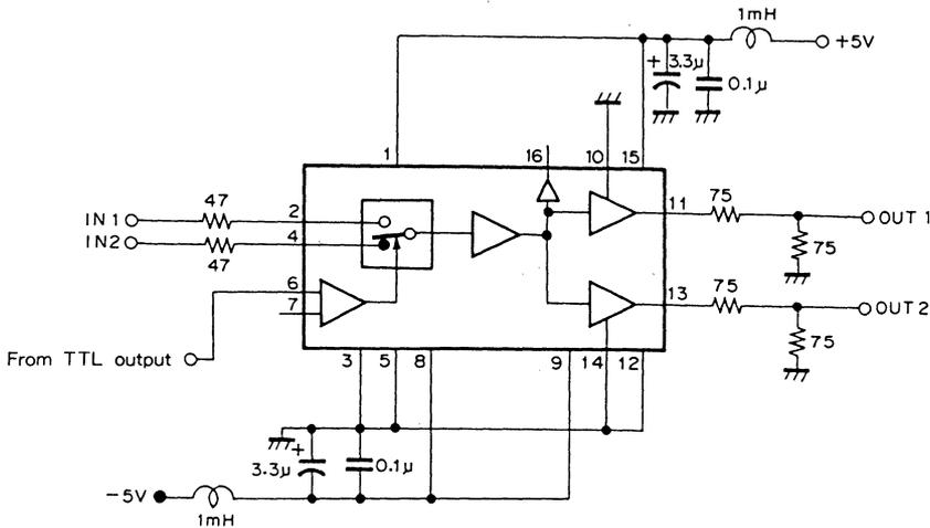
When the TTL output is low, the IN1 signal is output.
