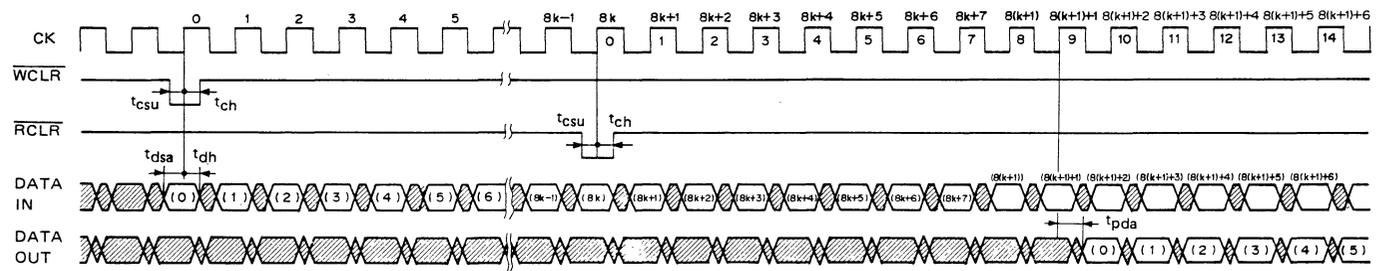
Fig. 8 The timing of data read out while writing in data
