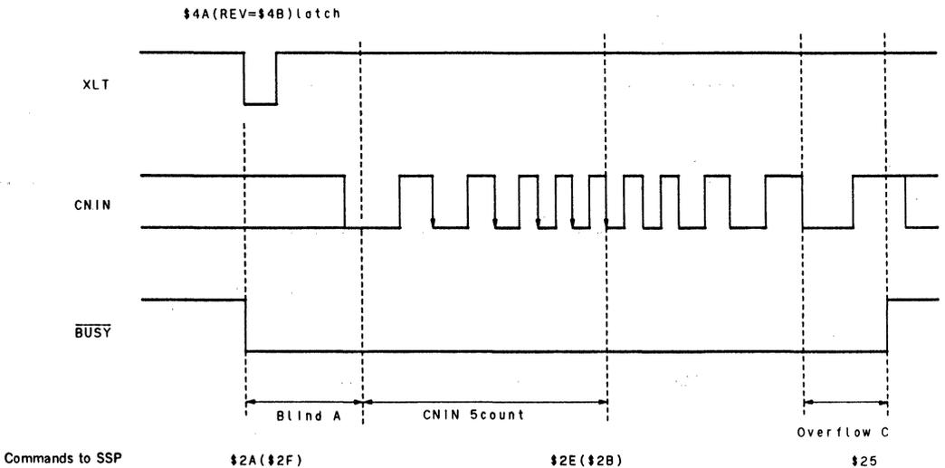
Figure 3-10 (b) Timing chart for 10-track jump
