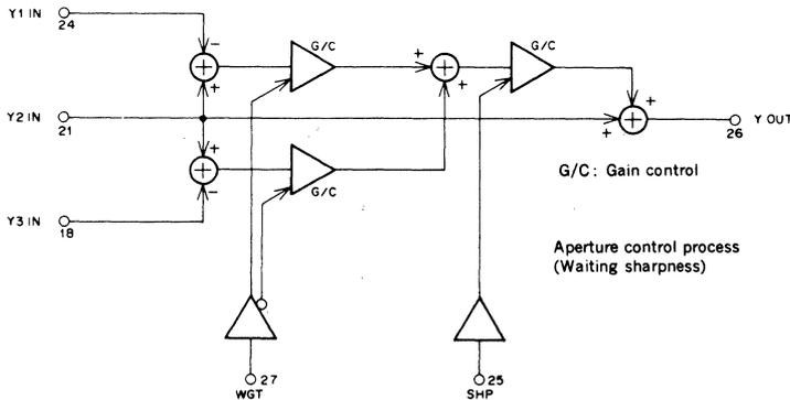
Aperture control process controls preshoot/overshoot ratio through WGT pin (Pin 27) and sharpness level through SHP pin (Pin 25) respectively. This control process is indicated on the above diagram.
