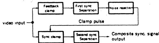
The video input signal passes through feedback clamp, first sync separation and after noise elimination, clamp pulse is formed. With this clamp pulse, the video input signal is sync clamped and the second sync separation performed.
