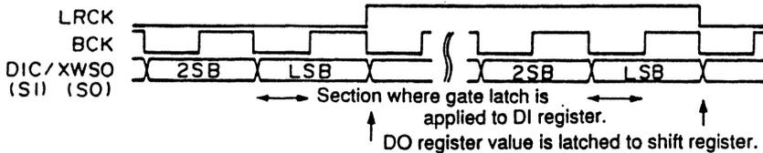
DI register value contained in the first half of 1LRCK calculating operations is the serial input data of the second half of the preceding LRCK. DI register value is similarly the serial input data of LRCK first half.
