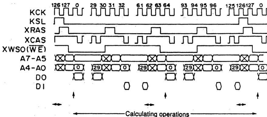
Should the data written last between cycle 0 to 62 in DO register be at CH1(n), data CH1(n-r) from the previous cycle 126 up to the present cycle 61 in DI register can perform read.
