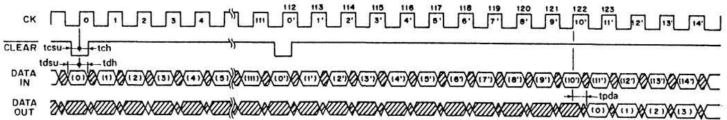
Fig. 4. Timing chart of 123 bits delay
