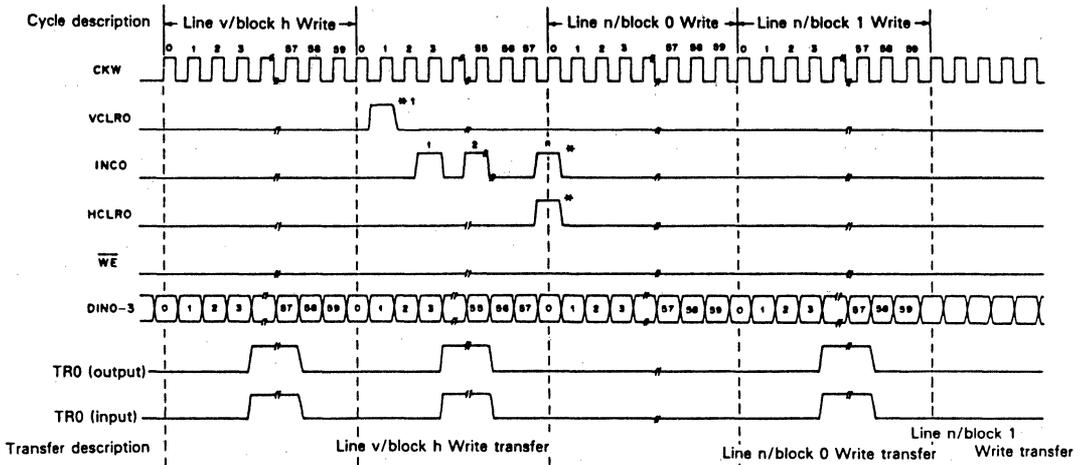
**\*Note)** When VCLRO enters after the 1st clock in the written block, followed by INCO n times, and then by HCLRO, the line address is reset, and incremented in the number equal to the number of times of INCO. Latch of the line address and reset of the block address are carried out.
