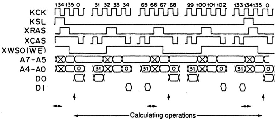
Should the data written last between cycle 0 to 66 in DO register be at CH1(n), data CH1(n-r) from the previous cycle 134 up to the present cycle 65 in DI register can perform read.
