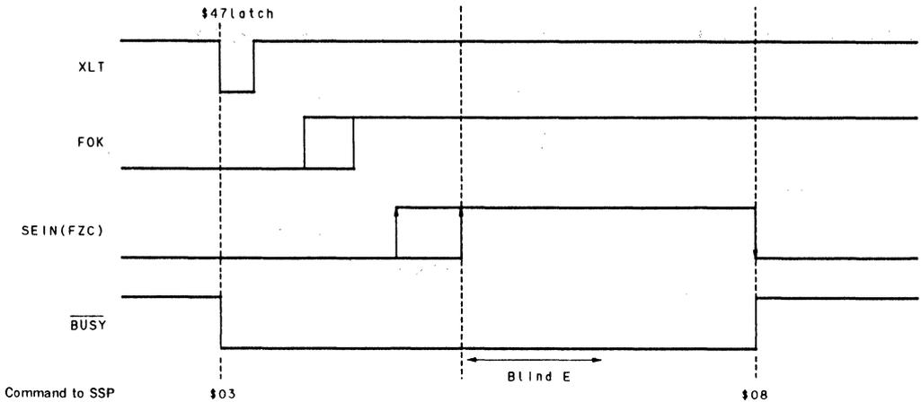
Figure 3-8 (b) Timing chart for auto focus operation
