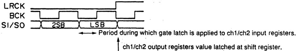
Serial I/O and I/O register are dependent on the timing with LRCK and BCK from the exterior. Also the only interrupt is executed between this LRCK and BCK on the Instructions.
