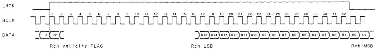
Fig. 2.1.1 (1) Digital In Timing Chart (C2PO don't care, no need for connection)
