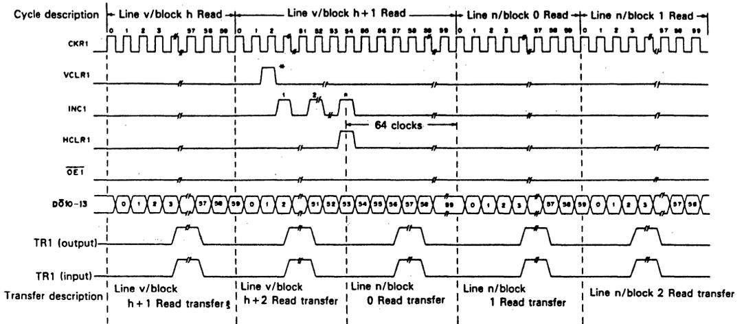
**\*Note)** When VCLR1 enters in one block, followed by INC1  $n$  times, and then followed by HCLR1 before clock 56 of the block, the line address is incremented in the number equal to the number of times of INC1 after reset, and line address latch and block address reset are carried out at the next clock.
