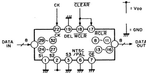
Fig. 3. Circuit of 123 bits delay
