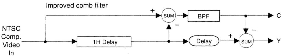
This can improve both cross color error and vertical resolution, but requires more components. Sony Digital comb filters can be recommended if the digital signal processor converting the digital Y, C data to RGB is available (See Application Note CAV04).
