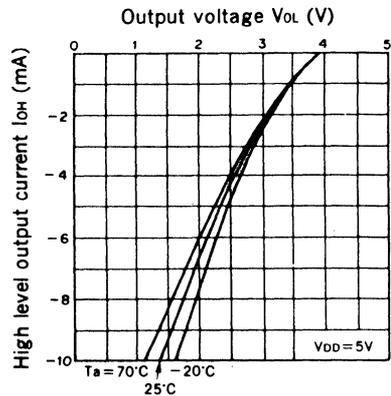
PD (Phase Comparator) pin Output Current Characteristics
