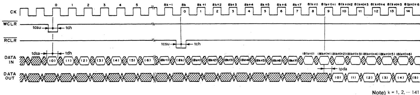
Fig. 8 The timing of data read out while writing in data (When S1="H", S2="L" and S3="L")
