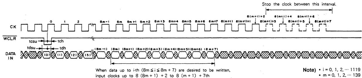
Fig. 6 The data write in timing when they are being held
