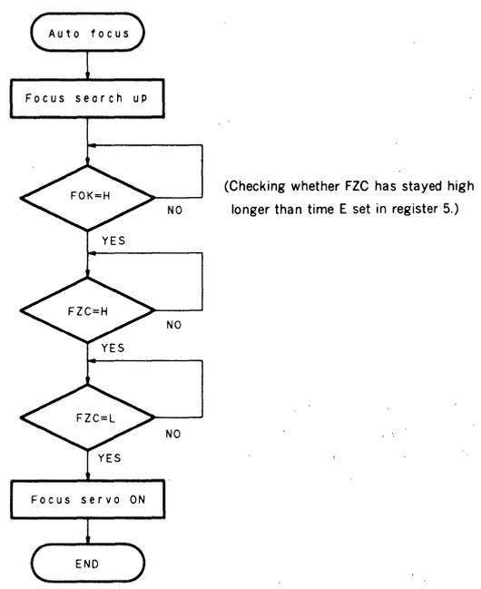
Figure 3-8 (a) Flowchart of auto focus operation
