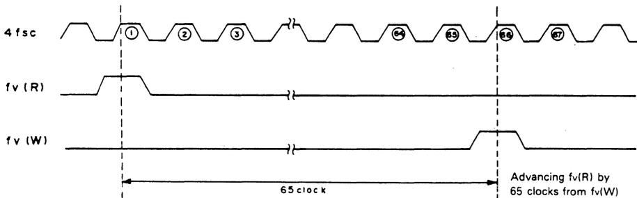
VRAM peripheral connection with 1 field delay
