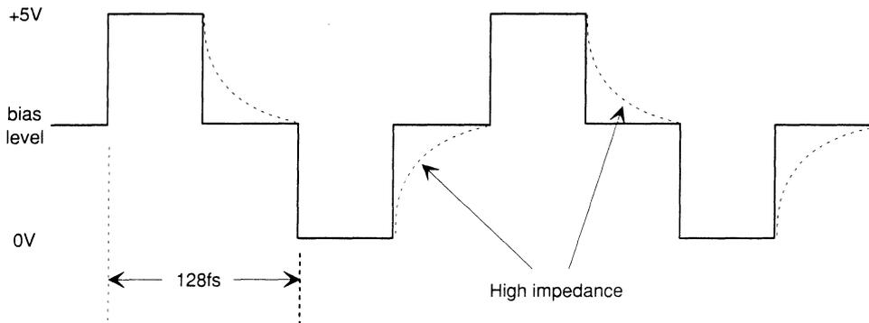
Filtering is necessary to eliminate 128fs component. Attenuation level for stop band frequency component is -45dB level. If it is necessary to increase this level, additional LPF is recommended to be used.
