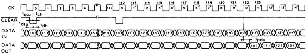
Fig. 4 Timing chart of 123 bits delay
