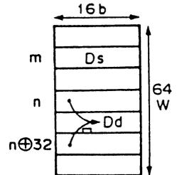
D-RAM address specification by users is a logical address and not a physical one. Inside the IC there is a 6 bit ring address counter that is incremented every I/O sampling. The logical address *addr* which is modulo added to this counter value DAC because the physical address.
