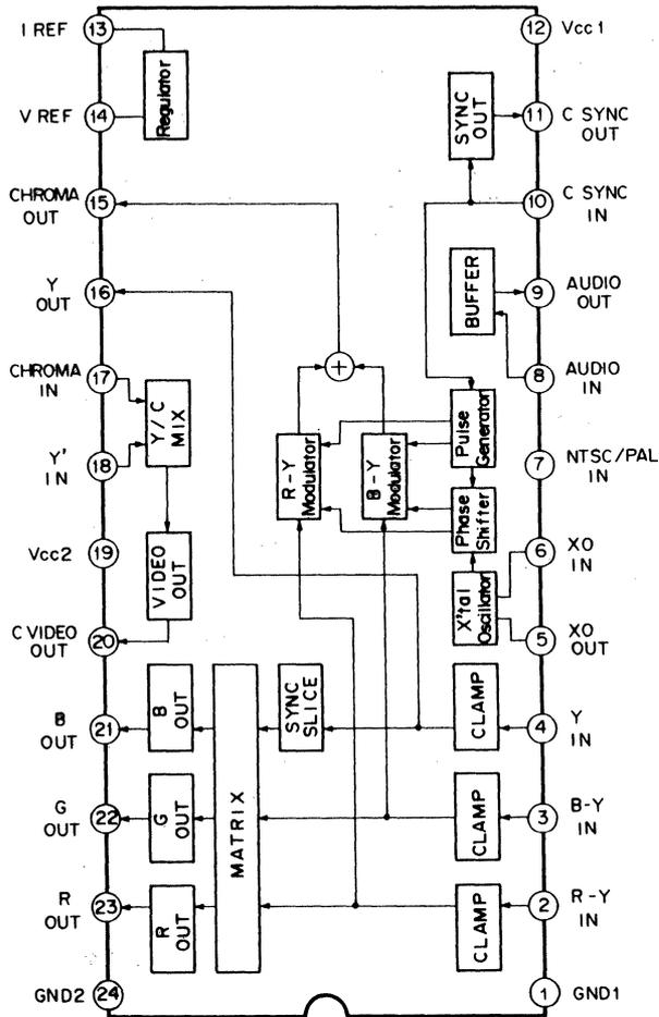
Pin Description and Equivalent Circuit
