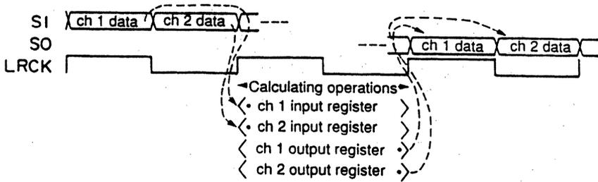
First, during 1LRCK period, ch1/ch2 serial data that is input from SI is latched at ch1/ch2 input register with the rising edge of the following LRCK. Also, during 1LRCK, if the results of the calculating operations are enclosed into ch1/ch2 output registers, those are latched by the shift register at the following rising edge of LRCK to be respectively output as serial data from SO.
