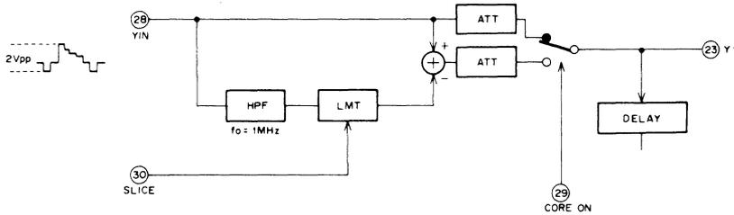
As shown in the above diagram, Y signal is passed through HPF, amplitude limitation is performed and the result subtracted from the original signal to execute Y signal coring.
