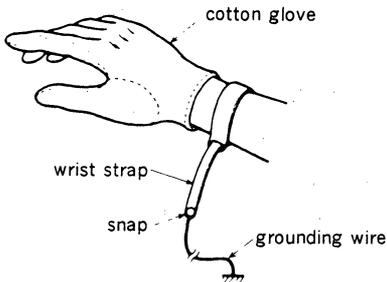
When using a copper wire for grounding, connect a 1MΩ resistance in series near the hand for safety.
