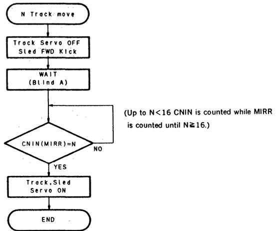
Figure 3-12 (a) Flowchart of N track move
