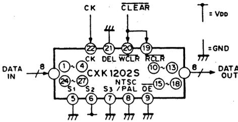
Fig. 3 Circuit of 123 bits delay
