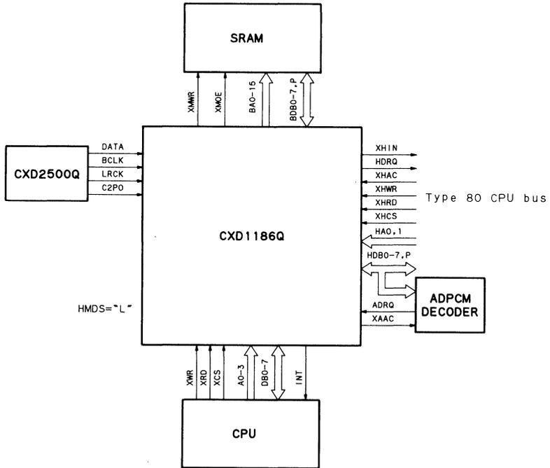
Fig. 4.2 CXD1186Q connection (Type80 CPU bus)
