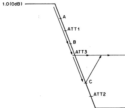
Fig.1 Transition from one attenuator value to another
