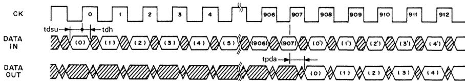
Fig. 2. Timing chart of 908 bits delay
