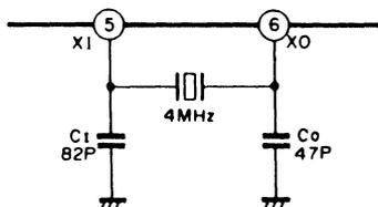
**[4-2] Reference signal generation by means of external clock**
