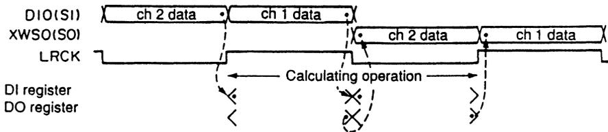
The detailed timing of delay I/O input/output register is as follows.
