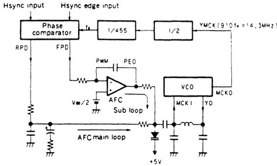
Input H sync, that edge and VCO ( $\approx 910f_H$ ) counted down to  $1/910$  are phase compared. There are 2 such error outputs: RPD: phase comparison output between all sync bottom line and the built-in H counter, and FPD: between sync rising edge and the built-in H counter. RPD output is a lag-lead filter and FPD output is an integrator. Both outputs are converted into DC error respectively.
