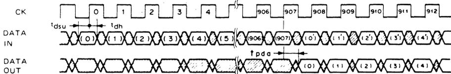
Fig. 2 Timing chart of 908 bits delay
