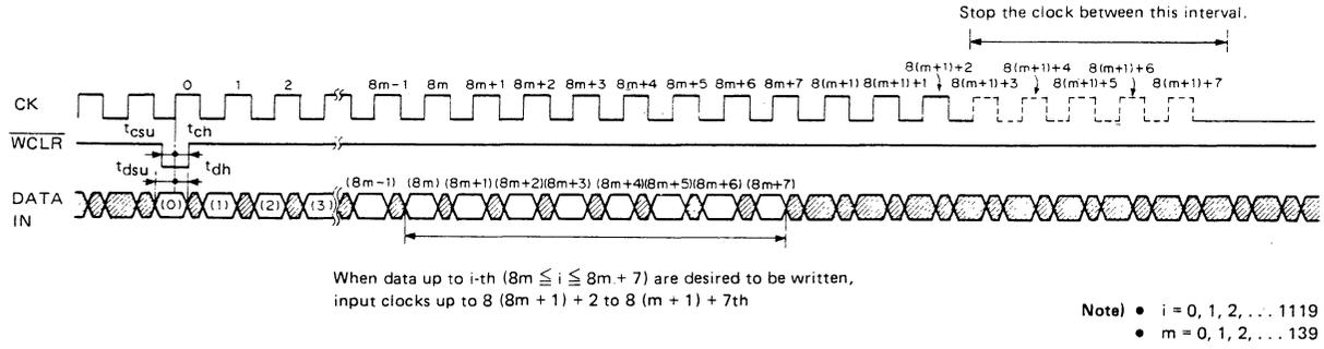
Fig. 6 The data write in timing when they are being held
