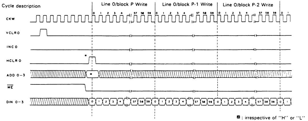
**\*Note)** The block address is latched by HCLRO in the case of address preset mode.
