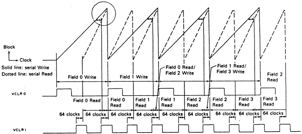
Note) Continuous input of CKW0 and CKR1.  $\overline{WE} = "L"$ ,  $\overline{OE} = "L"$
