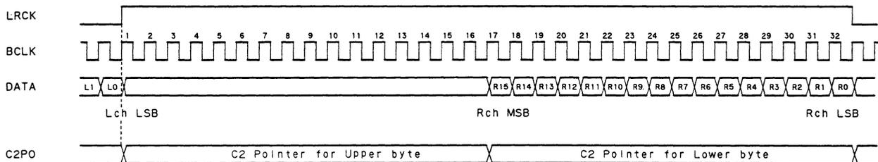
Fig. 2.1.1 (4) CXD2500Q, 64 bit slot mode, timing chart
