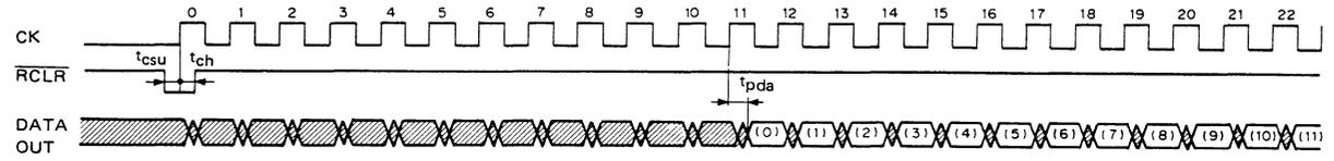
Fig. 7 The data read OUT timing
