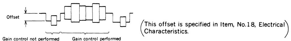
When the changing offset applies to the image chroma signal, the TV screen is adversely affected. Adjust Pin 9 (SET. P) voltage, controlling Pin 9 voltage so that it does not apply to the image.
