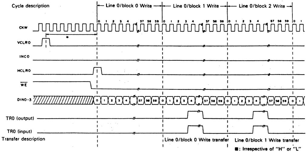
**\*Note)** In the case of initial cycle, it is necessary to enter VCLRO and HCLRO simultaneously, or to enter HCLRO before the first clock of the block next to that containing VCLRO.
