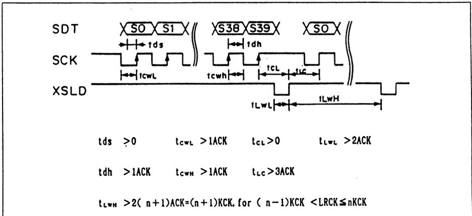
By applying the below conditions to XSLD the above  $t_{LWH}$  conditions can be prevented and the max. Transfer rate of 40 bit/LRCK realized.
