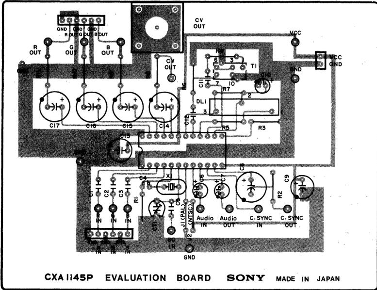
Parts arrangement diagram (parts side)
