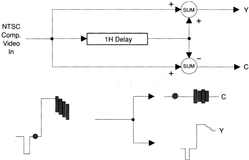
However, the low frequency components concentrated on harmonics of the sub carrier frequency will be combed away, and it will reduce the vertical resolution and decrease the sharpness of image in the vertical direction.
