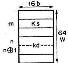
K-RAM address specify can be mentioned in the command that actually handles K-RAM. There are 2 types of K-RAM address specify absolute address specify and relative address specify.
