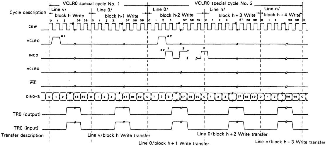
**Note)** \*1. VCLRO having entered after the 1st clock in the written block resets the line address, and is latched at the end of the block.
