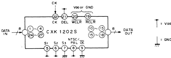
Fig. 1 Circuit of 908 bits delay
