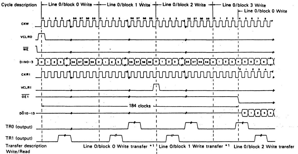
**Note) \*1.** In order to access new data, block Write transfer is conducted after Write of 60 bits, and readout is made after Read transfer of that block. A lag of more than 184 clocks is necessary for Read clock from Write clock.
