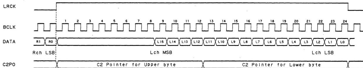
Fig. 2.1.1 (3) CXD2500Q, 48 bit slot mode, timing chart
