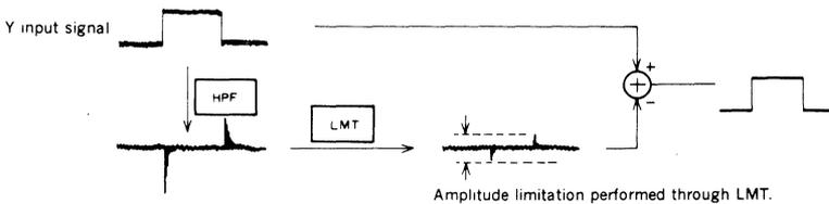
Cut off frequency of the HPF (high pass filter) used for coring stands at approx. 1MHz (Typ.). The amplitude limiting range of the limiter stands within 0 to 400mV (Typ.). Control is performed through Pin 30 (SLICE).
