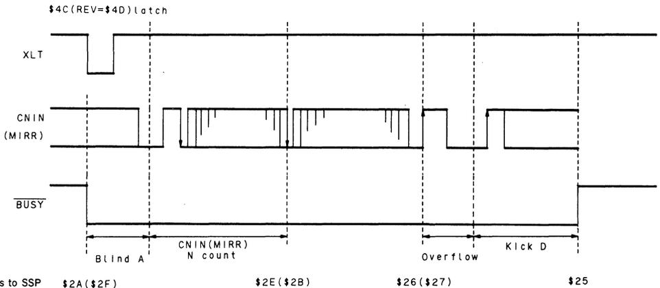
Figure 3-11 (b) Timing chart for 2N track jump
