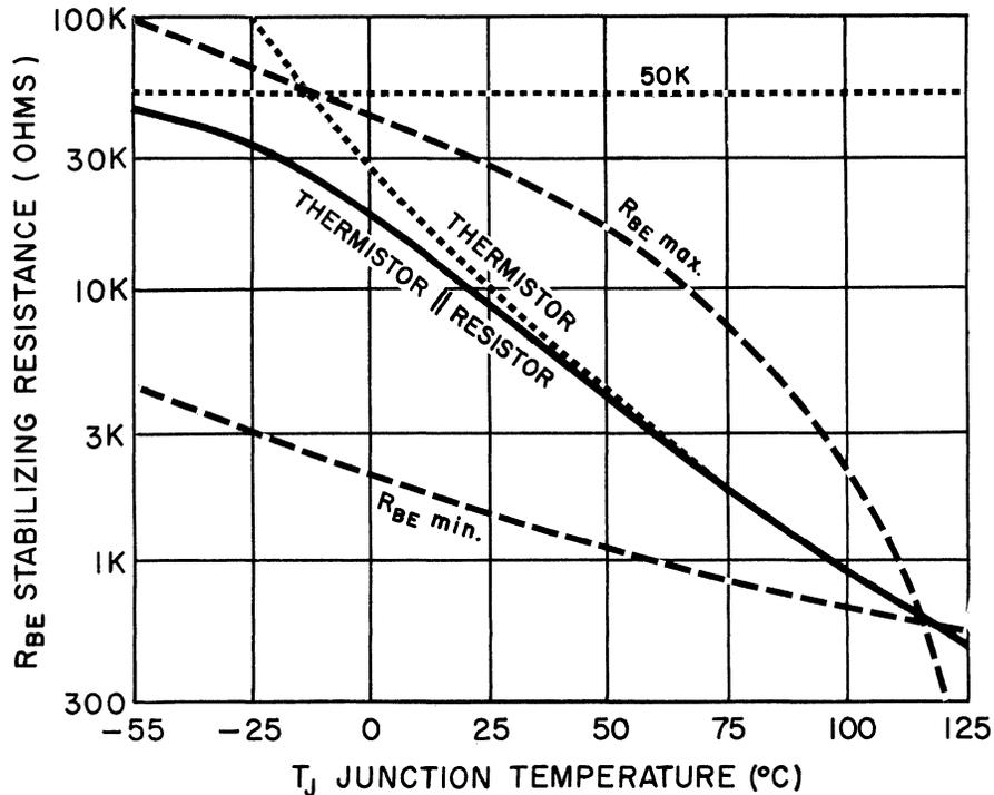
Fig. 6 Thermistor Bias Stabilization
