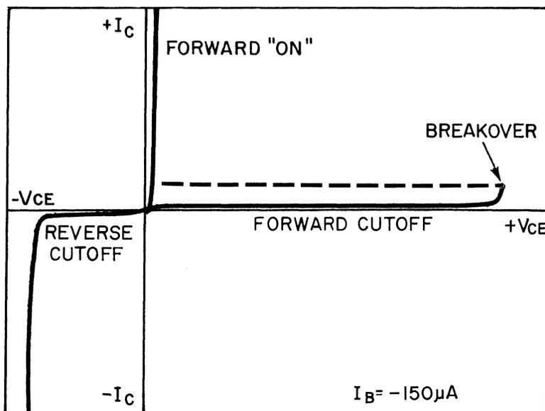
Fig. 4 Output Characteristic
