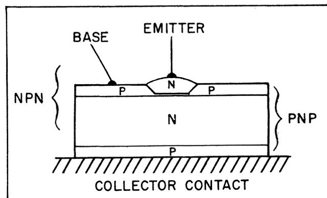
Fig. 1 Trigistor Construction
