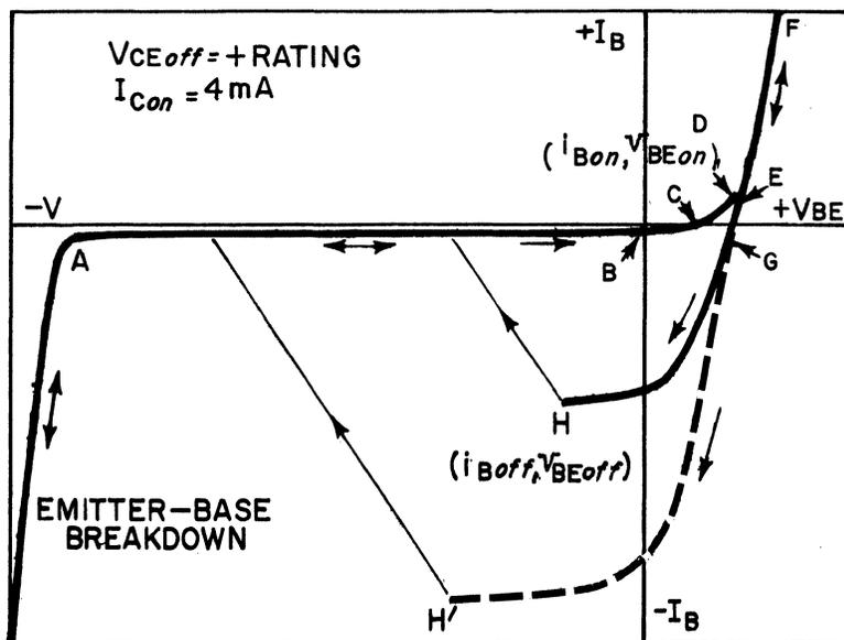
Fig. 5 Input Characteristic
