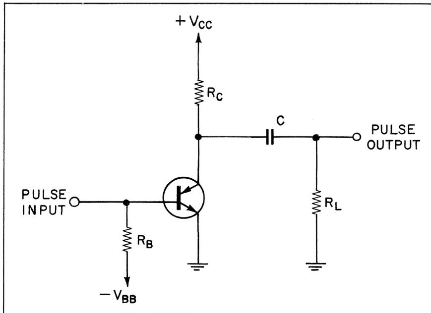
Fig. 7 Tristor Pulse Generator
