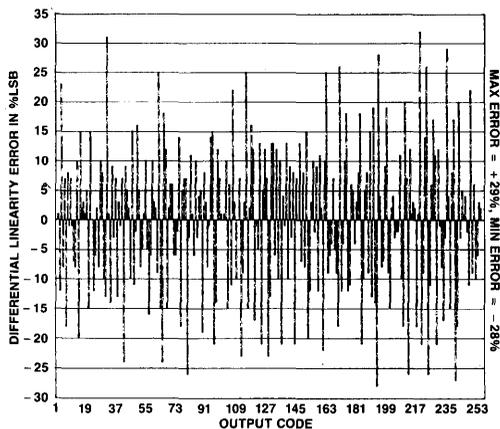
Figure 18. HS 168 Dynamic Differential Linearity Error
