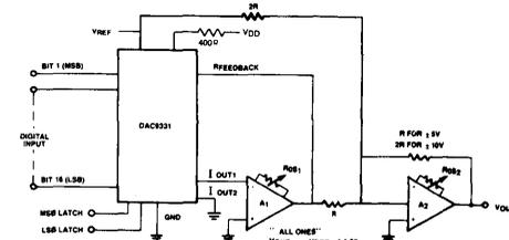
NOTE: To maintain specified DAC9331 linearity, external amplifiers (A1 and A2) must be zeroed. With a digital input of 10...0 and  $V_{REF}$  set to zero:
