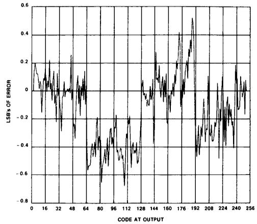
Graph 6. Dc Integral Linearity Error at  $F_{\text{Sample}} = 25 \text{ MHz}$
