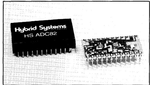
**Pin-to-Pin Compatibility** — The HS ADC82 is a superior replacement for the BURR-BROWN ADC82 AG. Reduced power consumption and a new packaging technique offer increased reliability and reduced cost.
