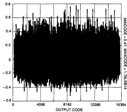
Figure 18. HS 9476 Dynamic Differential Linearity,  $F_{in} = 23.456\text{kHz}$ ,  $F_{sample} = 50\text{kHz}$
