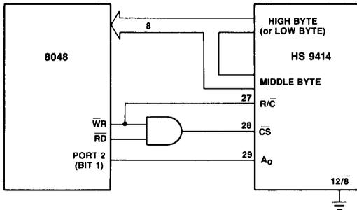
Figure 7. Interfacing the HS 9414 with a 8048  $\mu$ P.
