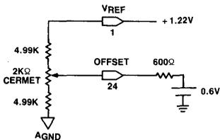
Figure 4. Bipolar Mode — Stable External Offset Adjustment
