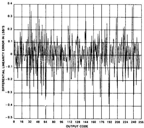
Graph 9. SP1072 Dynamic Diff<sub>ILIN</sub> Error at  $F_{\text{in}} = 6.103 \text{ kHz}$ ,  $F_s = 25 \text{ MHz}$
