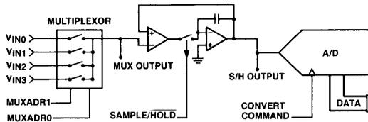
Figure 1A. Simple Sequential Four-Channel DAS
