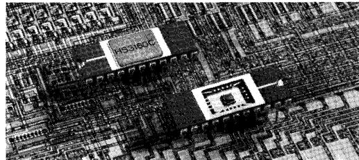
High resolution DAC's developed by Hybrid Systems include: DAC9331-16 (top) industry's first 0.0008% accurate Hybrid DAC and HS 3160 (bottom) 16-bit CMOS MDAC guaranteed monotonic to 14 bits (0.003%) from -25°C to +85°C.
