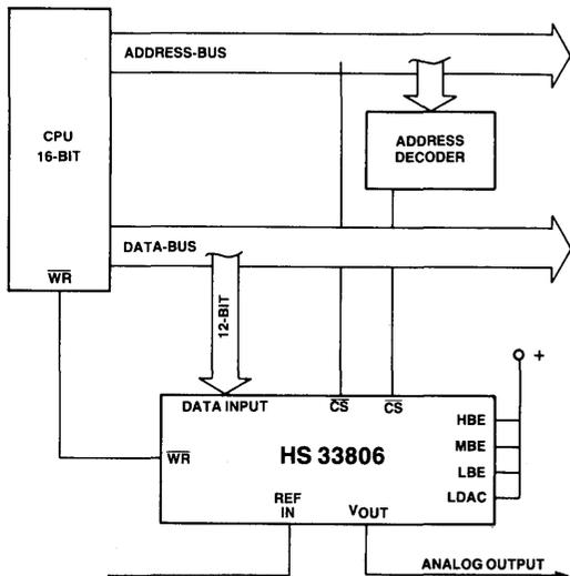
Interfacing the HS 33806 to a 16-Bit microprocessor is quite easy, because no multiplexing of the data inputs is necessary. An address decoder and the second chip-select input is used to select the DAC.
