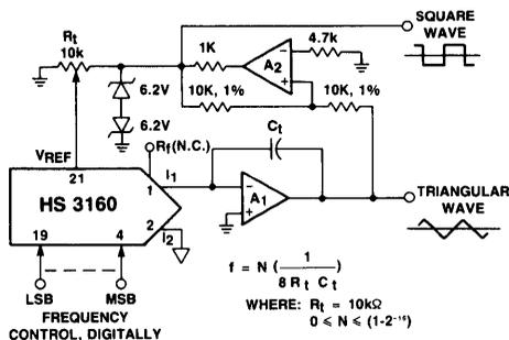
Figure 7. Programmable Function Generator
