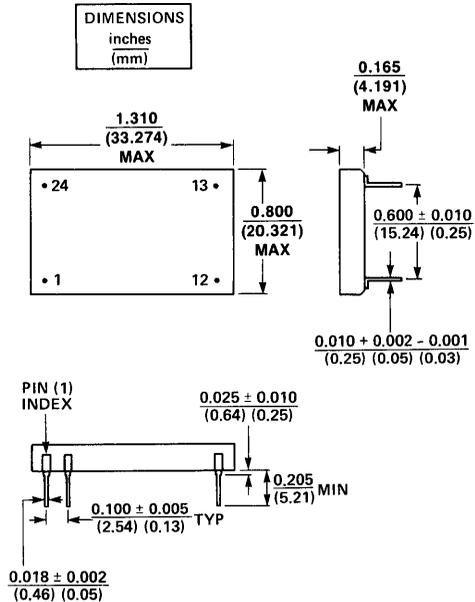
Pin 1 is marked by a dot on the top of the package.
