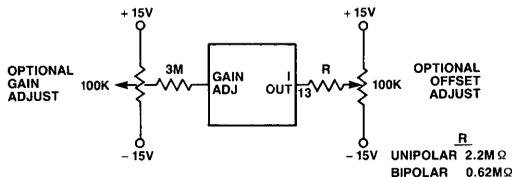
**Offset Adjustment:** Set the digital input code to 000...000 and adjust the offset trim potentiometer for zero output current (unipolar) or minus full scale output current (bipolar).
