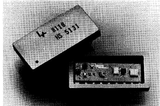
sion, laser-trimmed resistors for excellent long-term stability.
