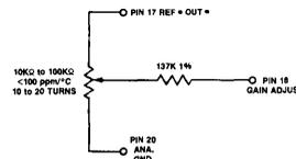
**GAIN ADJUST CIRCUIT MIN ADJUST RANGE =  $\pm 0.2\%$  FSR**
