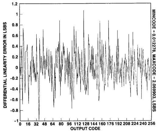
Graph 27. Dynamic DiffLin Error at  $F_{in} = 10-MHz$ ,  $F_s = 60$  MHz
