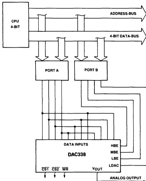
This figure shows how to operate the DAC338 with two 4-Bit ports. The chip-selects are tied to ground allowing continuous operation; they can be used for operating more DAC's at the same port. In the first step data should appear at the port A outputs; in the second step the control flags should appear on port B.
