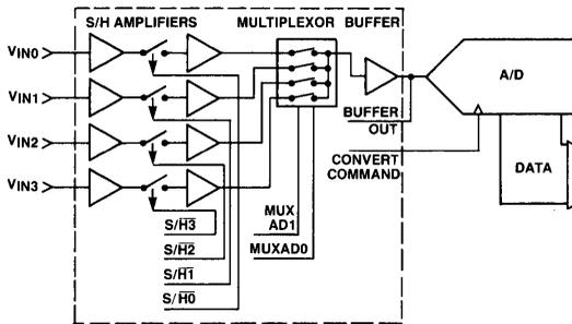
Figure 4A. Pipelined Acquisition DAS Using HS 9705
