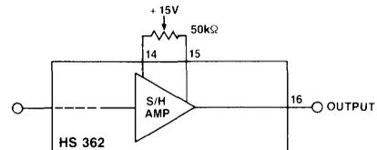
Figure 3. HS 362 Offset Voltage Adjustment
