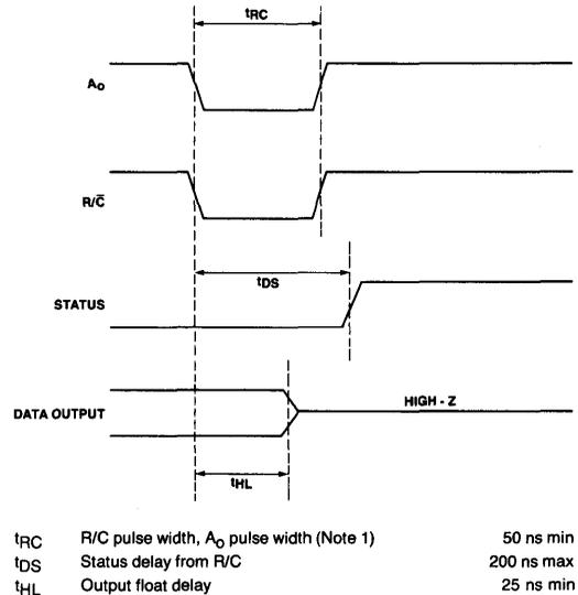
Figure 3. Timing Diagram to Start a 12-Bit Conversion
