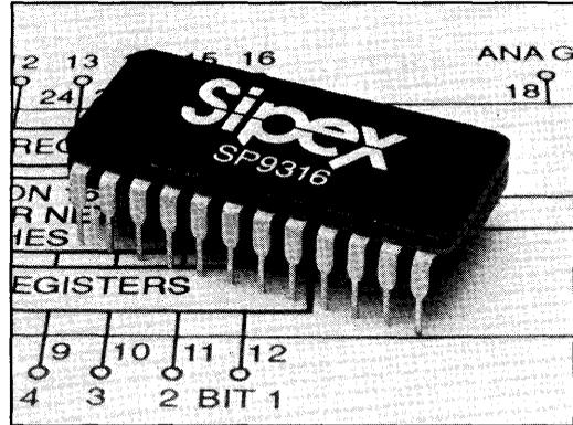
Packaged in a hermetic 24-pin ceramic or molded plastic. The SP9316 is specified for operation from 0°C to 70°C for commercial grades and -55°C to +125°C for military grades.
