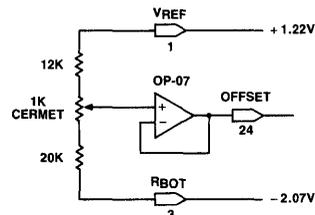
Figure 2. Unipolar Mode - Stable External Offset Adjustment
