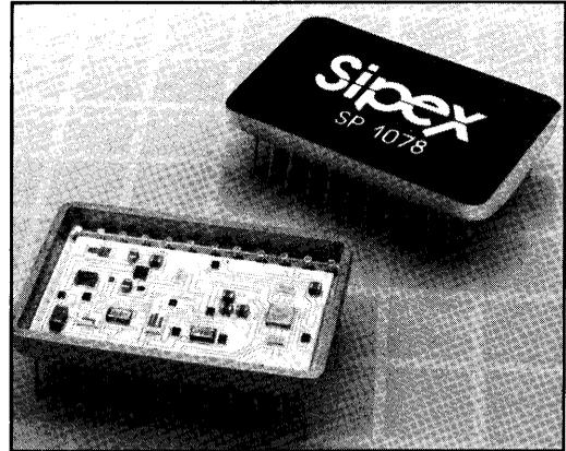
The combination of support circuitry and converter within one 24-pin package offers significant savings of board space. Other benefits include savings in component, assembly and design costs.
