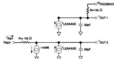
FIGURE 2: HS-7541A Equivalent Circuit (All Inputs Low)
