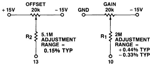
Values of  $R_1$  &  $R_2$  can be changed to increase or decrease the sensitivity of the adjustment. (This adjustment should not be greater than  $\pm 1\%$  around the nominal value for best performance.) Decreasing the  $R_1/R_2$  value increases the range of adjustment.
