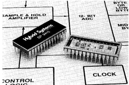
To take advantage of the 28-pin package the user must specify an input range of 0 to +10V,  $\pm 5V$  or  $\pm 10V$  when ordering. Four basic product grades are available; J and K models are specified over a temperature range of 0°C to +70°C while the S and T models are specified over an extended temperature range of -55°C to +125°C. Full screening to MIL-STD-883C is available.
