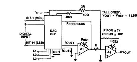
NOTE: TO MAINTAIN SPECIFIED LINEARITY, EXTERNAL AMPLIFIERS (A1 AND A2) MUST BE ZEROED, WITH A DIGITAL INPUT OF 10...0 AND VREF SET TO ZERO:
