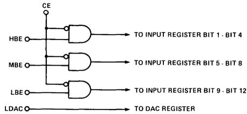
NOTE: The transfer from input register to DAC register can be performed without Enabling Chip.
