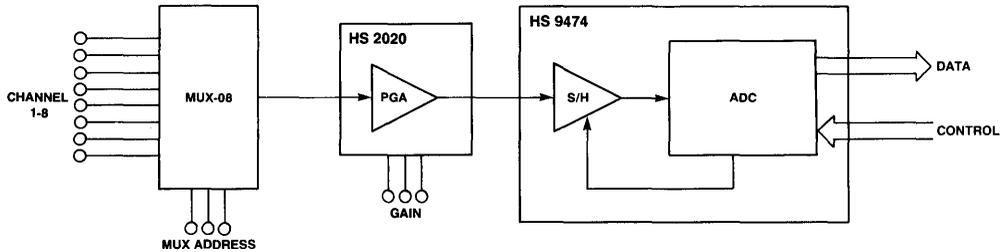
Figure 10. Data Acquisition System with Digitally Programmable Gain Amplifier
