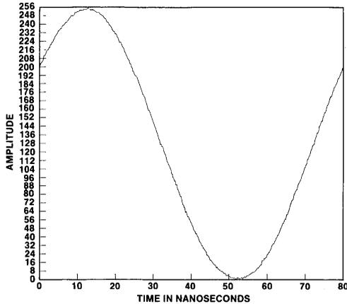
Graph 24. SP1078 Beat Frequency Test at  $F_{in} = 12.5+MHz$ ,  $F_s = 50$  MHz
