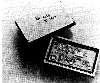
The HS 3860 includes an internal, precision reference supply, a fast output amplifier for minimum settling time, and input registers for easier microprocessor interface.
