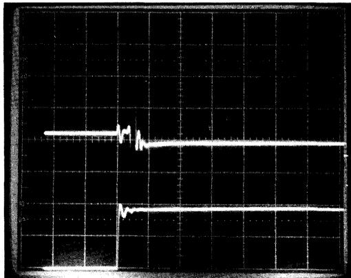
Figure 6. Sample-to-Hold Step (Top), HOLD Command (Bottom)
