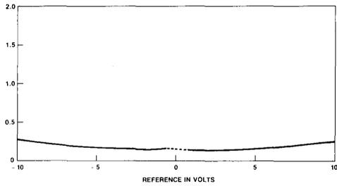
*Integral Linearity Error Vs. Reference Voltage
