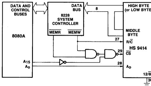
Figure 6. Interfacing the HS 9414 and 8080A  $\mu$ P
