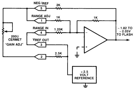
Figure 4. Gain Adjustment Circuit for 0 to 10% Gain Increase
