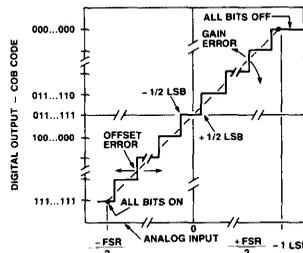
Figure 12. Ideal HS 9476 Transfer Characteristics (Bipolar Mode)
