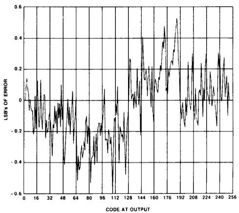
Graph 8. Dc Integral Linearity Error at  $F_{\text{Sample}} = 20 \text{ MHz}$
