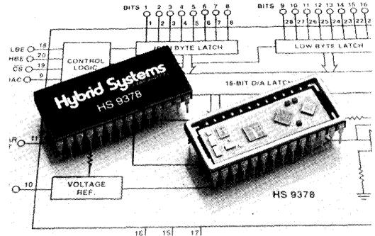
interface to 8- or 16-bit bus structures. The pinout of the HS9378 allows the user with an 8-bit bus to run only 8 traces directly underneath the hybrid to connect to the 16-bit input register.
