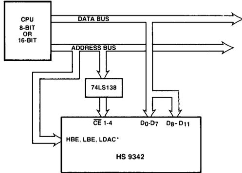
\*For 8-Bit Data Bus, HBE and LBE addressed separately as high byte and low byte.
