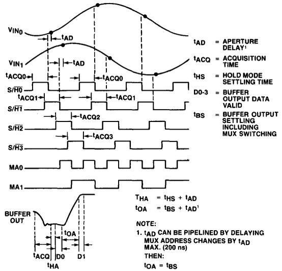
Figure 4. Pipelined Acquisition Sequential Sampling Using HS 9705.
