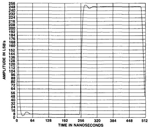
Figure 20. HS 1068 Beat Frequency Input Amplifier Settling Time
