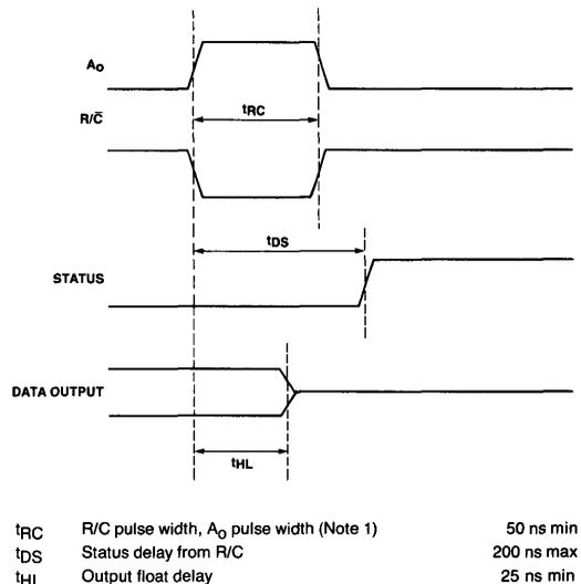
Figure 4. Timing Diagram to Start an 8-Bit Conversion
