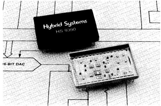
The HS9390 is packaged in a 32-pin metal triple DIP and is offered for commercial (0°C to +70°C) and military (-55°C to +125°C) applications with processing available in full compliance with MIL-STD-883C.
