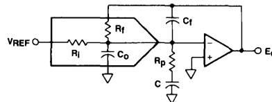
Figure 5 MDAC Equivalent Output Circuit
