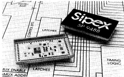
SP9488 is offered in a 62 pin hermetically sealed package. Temperature ranges available are 0 to 70°C for commercial versions and -55 to +125°C with MIL-STD-883 Rev C screening for military grades.
