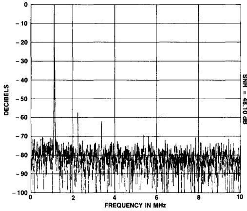
Figure 12. FFT of HS 1068,  $F_{IN}=1.123$  MHz,  $F_{SAMPLE}=20$  MHz
