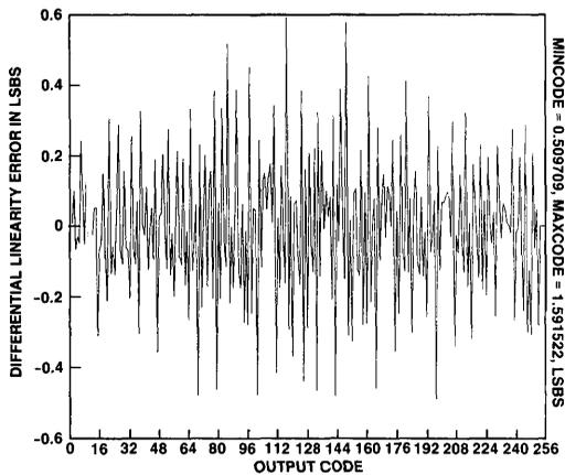
Graph 2. Dynamic DiffLin Error at  $F_{in} = 10$ -MHz,  $F_s = 20$  MHz
