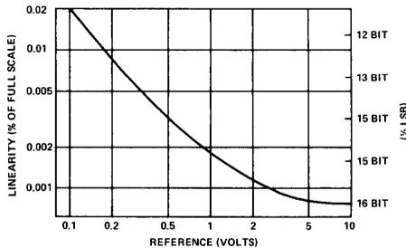
Figure 15 Linearity VS Reference Voltage, HS 3120 (top), DAC9331-16 (bottom)
