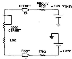
Figure 1. Unipolar Mode - External Offset Adjustment
