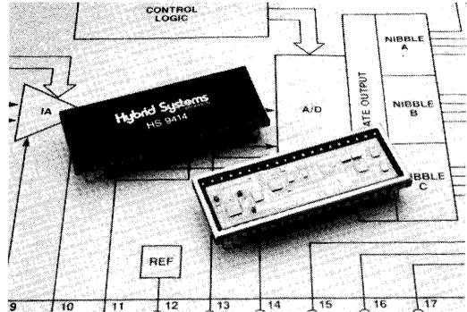
The HS9414 is offered in a ceramic package for commercial (0°C to +70°C) and military (-55°C to +125°C) applications with processing available in full compliance with MIL-STD-883C.
