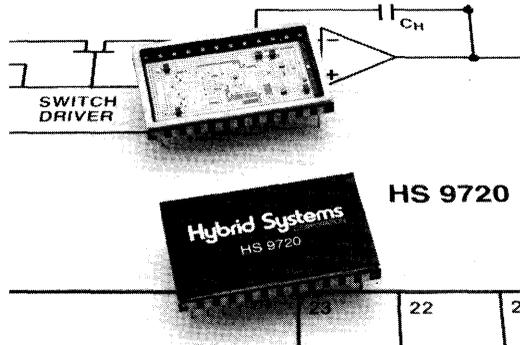
The HS9720 is packaged in a 24-pin DIP and is specified for operation from  $0^{\circ}\text{C}$  to  $+70^{\circ}\text{C}$  for commercial grades, and  $-55^{\circ}\text{C}$  to  $+125^{\circ}\text{C}$  for military grades. Full screening to MIL-STD-883C is available.
