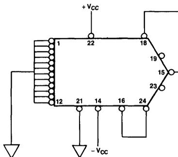
NOTE: Bypass each supply with a 1 $\mu$ F tantalum and a 0.01 $\mu$ F ceramic to Common.
