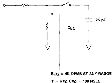
Figure 6. Equivalent HS 574A Input Circuit
