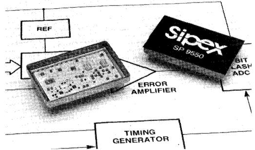
speed data acquisition systems. The SP9550 is ideal in all applications that require 12-bit performance at relatively high speed with moderately low power consumption.
