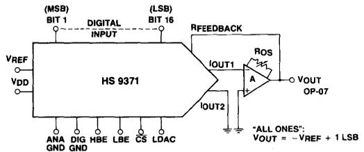
NOTE: To maintain specified HS 9371 linearity, the external amplifier (A) must be zeroed. Apply an ALL "ZEROS" digital input and adjust ROS for VOUT = 0 ± 1 mV.
