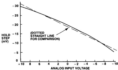
Figure 8. Hold Step vs. Input Voltage for Simplified Sample-and-Hold
