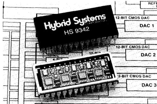
The HS9342 is packaged in a 28-pin DIP and is specified for operation from 0°C to 70°C for commercial grades and -55°C to +125°C for military grades. Full screening to MIL-STD-883C is available.
