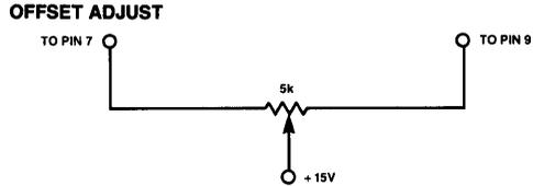
Connect the input (pin 13) to ground and adjust the output to read zero volt, while HS 346 is in sample mode (pin 1 at +5V).
