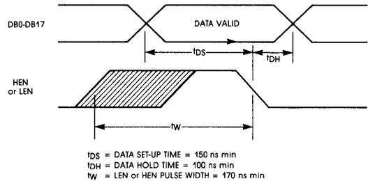
**Figure 6. SP9380 Timing Diagram**
