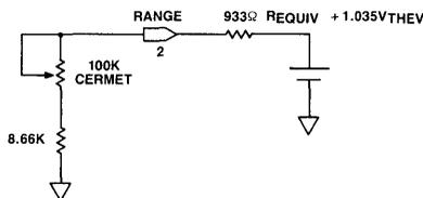
Figure 5. +1 to +10% External Gain Increase Circuit
