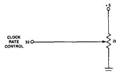
**ADJUSTMENT RANGE IS 50  $\mu\text{sec}$  to 200  $\mu\text{sec}$  at 16-BIT RESOLUTION**
