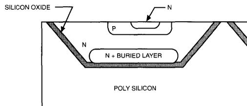
The process steps by which the DI islands are formed in the silicon substrate involves a combination of crystallographic preferential etching, oxidation, thick poly-silicon deposition and grinding and polishing.
