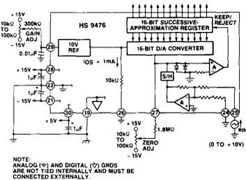
Figure 11a. Analog and Power Connections for Unipolar 0 to  $+10\text{V}$  Input Range
