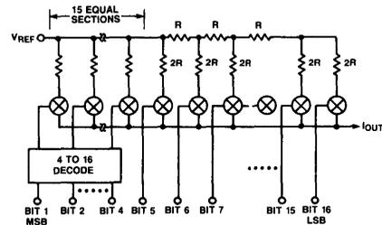
16-bit MDAC implemented by decoding top 4 MSB'S into 15 equal current sources followed by 12-bit R-2R DAC
