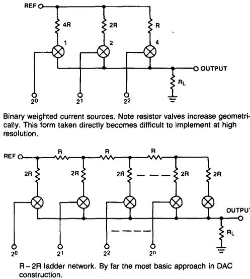
Figure 2 Binary Weighted DAC—Circuit Configuration
