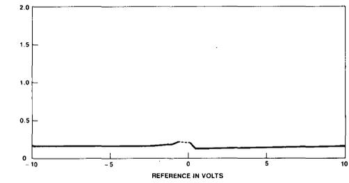
*Differential Linearity Error Vs. Reference Voltage
