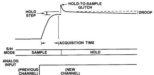
Figure 7b. Typical Sample-and-Hold Output Behavior
