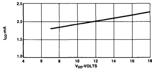
Power Supply Current vs. Voltage
