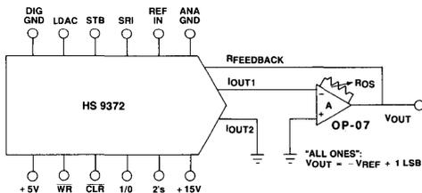
NOTE: To maintain specified HS 9372 linearity, the external amplifier (A) must be zeroed. This operation is easily performed without having to serially load an "all 0's" code; set  $\overline{CLR}$  and I/O to logic level "0" and adjust ROS for  $V_{OUT} = 0 \pm 1$  mV.
