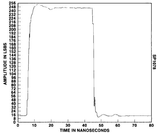
Graph 25. Beat Frequency Settling Time Test  $F_{in} = 12.5+MHz$ ,  $F_s = 50$  MHz
