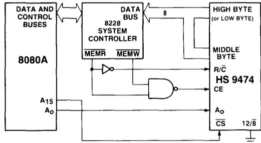
Figure 11A. Interfacing HS 9474 to 8080A  $\mu$ P (Top)
