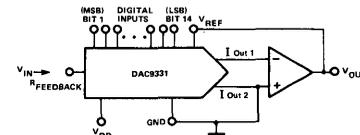
Via the above configuration, the DAC331 can be used to divide an analog signal by a digital code (i.e., for digitally controlled gain). The transfer function is given as
