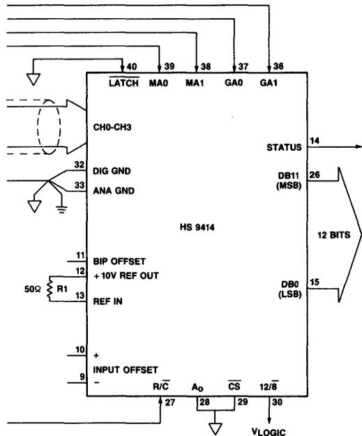
Figure 2c. No Trim Unipolar Connections
