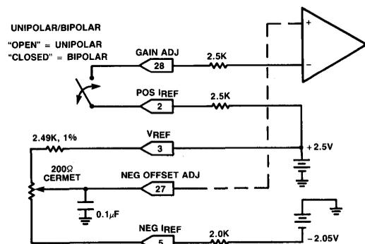
Figure 2. Unipolar/Bipolar Range Offset Adjustment Circuit
