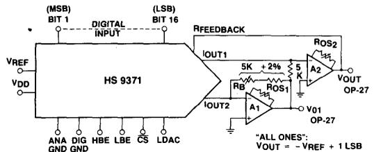
NOTE: To maintain specified HS 9371 linearity, external amplifiers (A1 and A2) must be zeroed. With a digital input of 10...0 and VREF set to zero:
