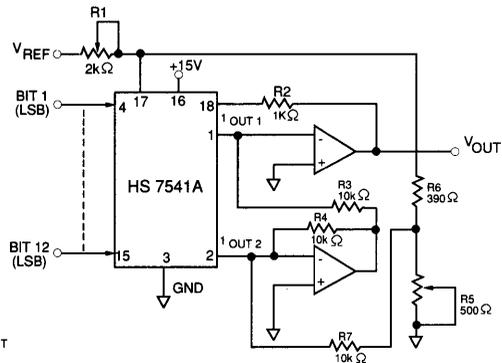
**FIGURE 5:** Bipolar Operation
