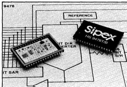
The HS9476 allows analog input ranges of  $\pm 5V$ ,  $\pm 10V$ , 0 to +10V, and 0 to +20V. Integral non-linearity is specified at  $\pm 0.003\%$  of FSR maximum, while no missing codes is guaranteed for the full operating temperature range. The HS9476 is available for operation over the commercial (0°C to 70°C) temperature range or -55°C to +125°C with full MIL-STD-883C screening.
