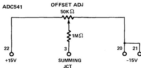
Unipolar: Apply a +½LSB analog input and set the potentiometer for a digital output that alternates between 000...0 and 000...1.
