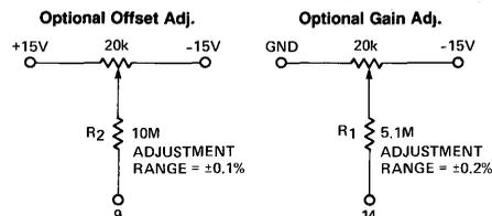
Values of  $R_1$  &  $R_2$  can be changed to increase or decrease the sensitivity of the adjustment. This adjustment should not be greater than  $\pm 1\%$  around the nominal value for best performance.
