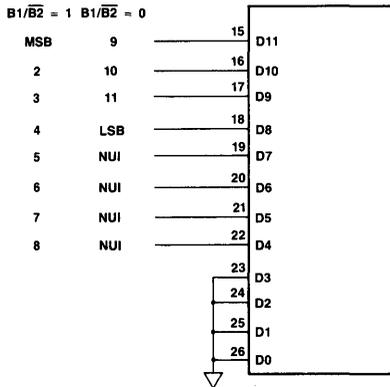
NUI = No Updated information. During the second load cycle, the information on pins 15 thru 18 will be loaded into the lower bits of the first register; information on pins 19 through 22 will not be recognized. Note: Upper 8 bits should be loaded first, then lower bits.
