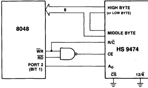
Figure 6. Interfacing the HS 9474 and a 8048  $\mu$ P
