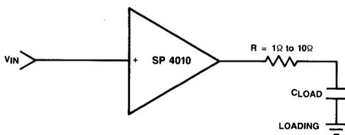
Figure 2. Capacitive Loading
