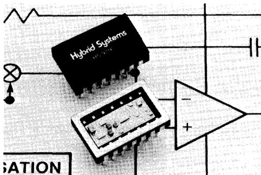
The HS9716/HS9714 comes complete with an internal hold capacitor and is available for use over the  $0^\circ\text{C}$  to  $70^\circ\text{C}$  temperature range and the  $-55^\circ\text{C}$  to  $+125^\circ\text{C}$  military temperature range. Full screening to MIL-STD-883C is available.
