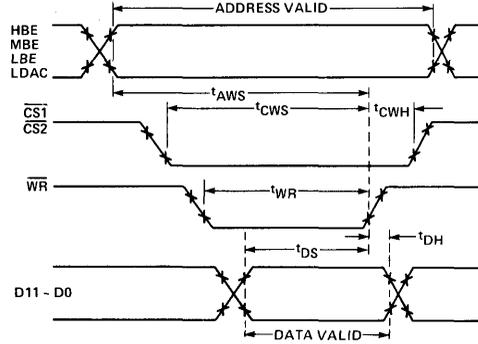
$t_{DS}$  : Data setup time, 250 nsec     $t_{CWS}$  : Chip select to write setup time, 300 nsec
