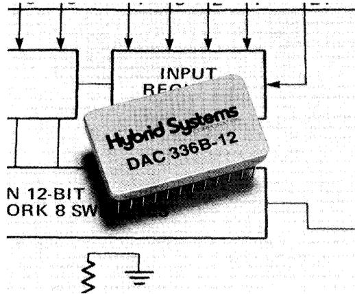
At the heart of the DAC336-12 is a laser-trimmed, low drift, thin-film nichrome network. The units accept TTL/DTL and 5V CMOS logic levels and deliver a minimum of 5 mA at  $\pm 10V$  out. Simple pin jumpering allows the user output choices of either  $\pm 10V$  or 0 to +10V.
