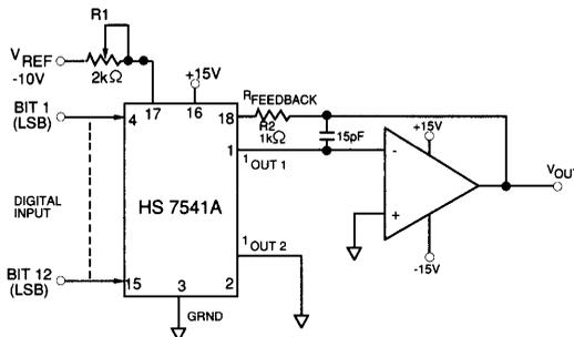
**FIGURE 4:** Unipolar Operation
