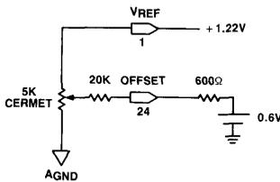
Figure 3. Bipolar Mode — External Offset Adjustment
