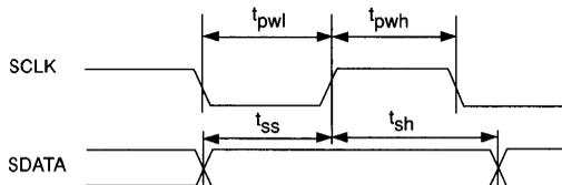
$$t_{pwl} = \text{pulse width low} = 2/f_{CLK} \text{ ns}$$
