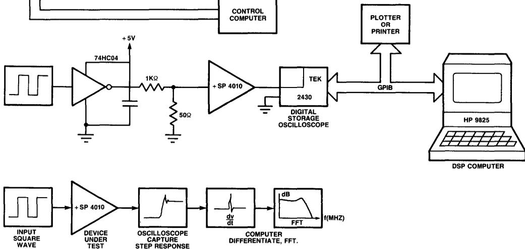
Figure 5. Frequency Response Test System
