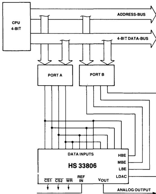
This figure shows how to operate the HS 33806 with two 4-Bit ports. The chip-selects are tied to ground allowing continuous operation; they can be used for operating more DAC's at the same port. In the first step data should appear at the port A outputs; in the second step the control flags should appear on port B.
