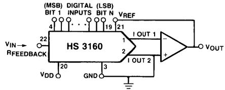
Via the above configuration, the HS 3160 can be used to divide an analog signal by a digital code (i.e. for digitally controlled gain). The transfer function is given as:
