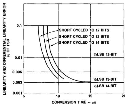
Figure 10. HS 9476 Nonlinearity Vs. Conversion Time
