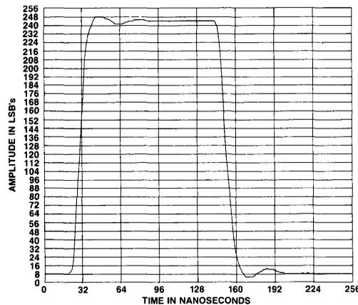
Figure 21. HS 1068 Beat Frequency Input Amplifier Settling Time
