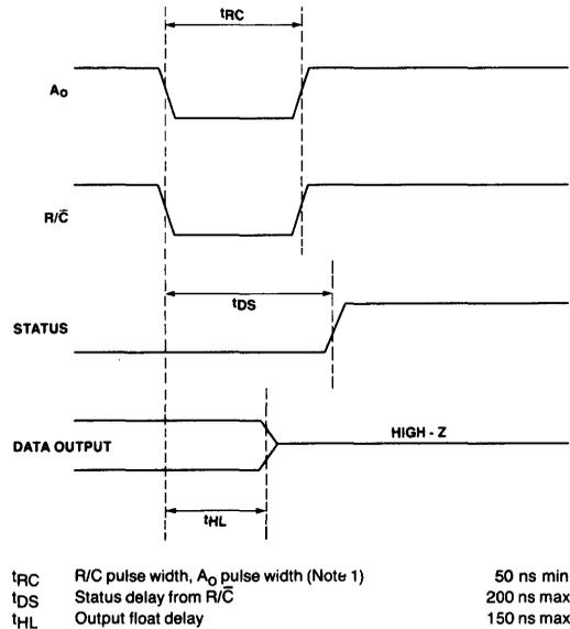
Figure 3. Timing Diagram to Start a 12-Bit Conversion
