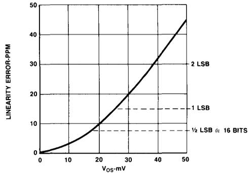
Additional Linearity Error vs. Output-Amplifier Offset-Voltage
