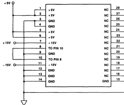
Figure 10. Burn-In Schematic
