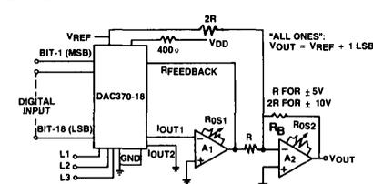
NOTE: TO MAINTAIN SPECIFIED LINEARITY, EXTERNAL AMPLIFIERS (A1 AND A2) MUST BE ZEROED, WITH A DIGITAL INPUT OF 10...10 AND  $V_{REF}$  SET TO ZERO:
