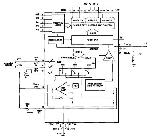
Figure 9. Bipolar Input Connections
