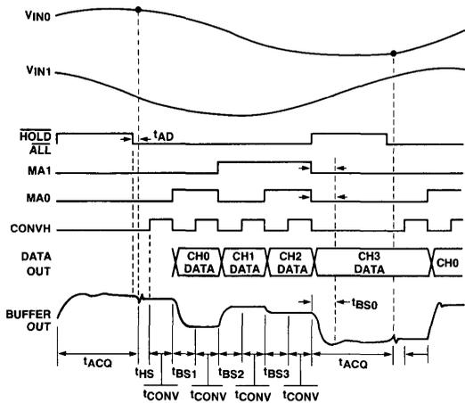
$t_{BS}$  = MUX SWITCHING AND OUTPUT BUFFER SETTLING TIME ASSUMING:  $t_{ACQ}$  = 7  $\mu$ s MAX
