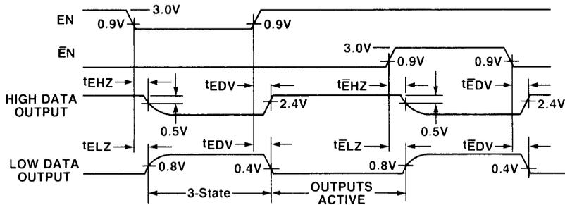
**TIMING CHARACTERISTICS** (T<sub>A</sub> = 25°C, V<sub>CC</sub> = +5.0V, V<sub>EE</sub> = 5.2V. See System Timing Diagram.)
