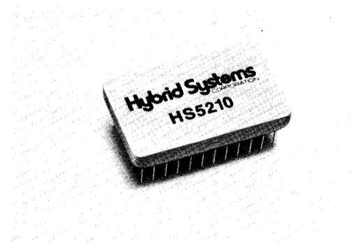
HS5210 Series ADCs are available in four input voltage ranges: 0 to  $-10$  volts (HS5210/13),  $\pm 5$  volts (HS5211/14),  $\pm 10$  volts (HS5212/15), and 0 to  $+10$  volts (HS5216). For each of these input ranges, the user has the option of specifying a model complete with an internal reference or for improved absolute accuracy, models which require an external reference.
