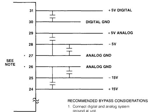
Note: \*Pin 26 & Pin 27 are internally connected.
