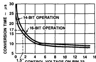
Figure 6. Conversion Time Vs. Clock Rate Control Voltage
