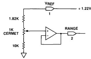
Figure 6. +8% to -1% External Gain Adjust Circuit
