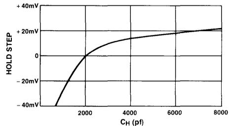
Figure 2. Typical Hold Step Vs. Hold Cap
