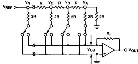
Figure 11 R-2R DAC with output amplifier
