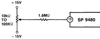
Figure 8. Offset Adjustment Circuit ( $\pm 0.4\%$  FSR)
