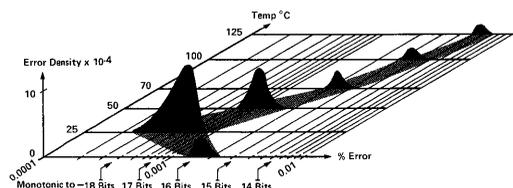
Differential Linearity is a measurement of the maximum deviation of any one LSB step change in the transfer function of the DAC377-18 from its ideal weight ( $38\mu\text{V}$ ). It is expressed in terms of the number of bits as well as the percent error.
