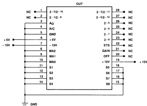
Figure 10. HS 9410 Burn-In Schematic
