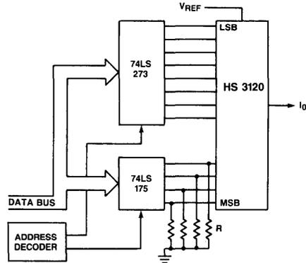
Figure 7 Clamp Resistors added to MSB Inputs
