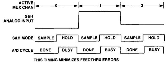
Figure 13. Changing Mux Channel During Hold Mode (and A/D Conversion) Invites Feedthru and Noise Errors
