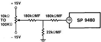
Figure 9. Low Tempco Offset Adjustment Circuit
