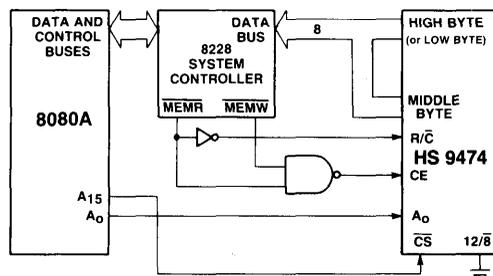
Figure 5. Interfacing the HS 9474 and 8080A  $\mu$ P
