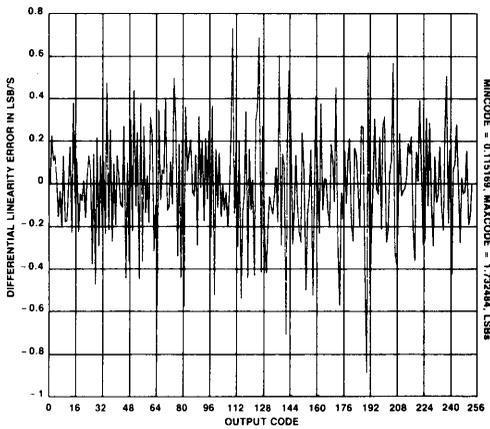
Graph 7. SP1072 Dynamic Diff<sub>ILIN</sub> Error at  $F_{\text{in}} = 5+ \text{ MHz}$ ,  $F_s = 25 \text{ MHz}$
