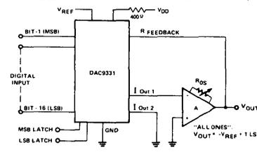
NOTE: To maintain specified DAC9331 linearity, the external amplifier (A) must be zeroed. Apply an ALL "ZEROS" digital input and adjust  $R_{OS}$  for  $V_{OUT} = 0 = 1mV$ .
