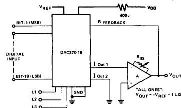
NOTE: To maintain specified linearity, the external amplifier (A) must be zeroed. Apply an ALL "ZEROS" digital input and adjust  $R_{OS}$  for  $V_{OUT} = 0 \pm 1mV$ .
