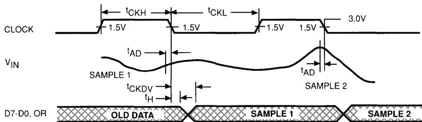
$t_{CKDV}$  and  $t_H$  measured at output levels of 0.8 and 2.4 volts.
