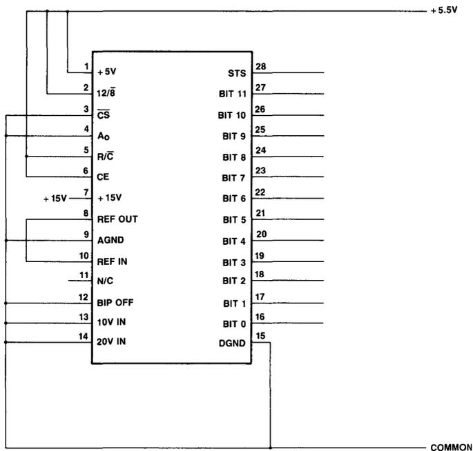
Figure 12. Burn-In Schematic
