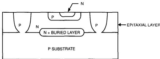
With a DI process, the reverse biased P-N junction is replaced by a high-quality, high field strength (Breakdown >800 Volts) silicon dioxide dielectric layer. Physically, this is realized by fabricating the circuit elements in individual silicon islands that are surrounded by silicon dioxide.
