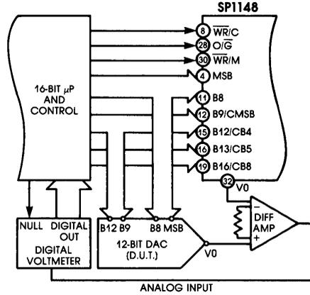
Figure 5. DAC Testing
