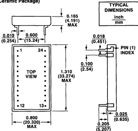
Pin 1 is marked by a dot on the top of the package.
