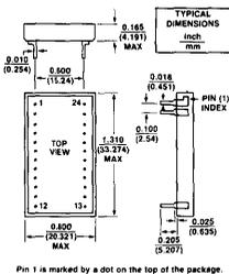
Pin 1 is marked by a dot on the top of the package.
