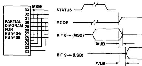
IVUB = TIME FOR UPPER BITS TO GO TO HIGH IMPEDANCE - 125ns
