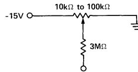
to PIN 14 (PIN 14 IS AT -6.4 VOLTS)
