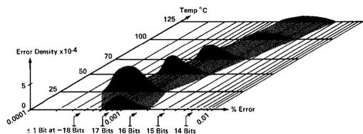
Integral Linearity is a measurement of the deviation of the DAC377-18 transfer function from a straight line through the end points. It is expressed in the number of bits as well as the percent error.
