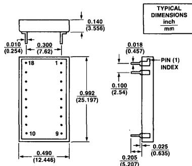
Pin 1 is marked by a dot on the top of the package.
