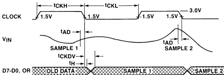
tCKDV and t<sub>H</sub> measured at output levels of 0.8 and 2.4 volts.
