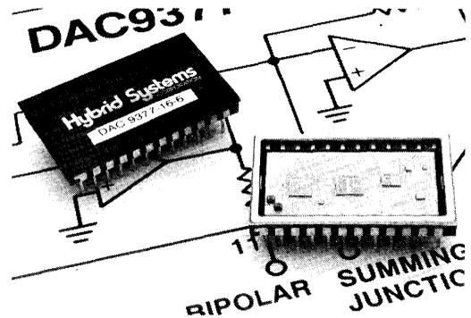
storage when latched, but is "transparent" when unlatched. The latch control is level-triggered for either static or dynamic operation.
