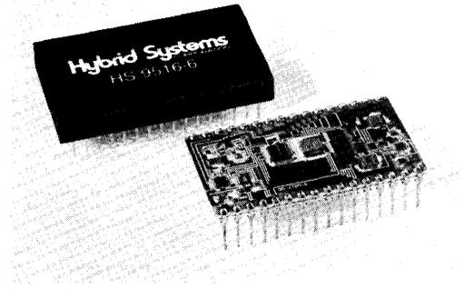
The HS9516 is available with 14-bit ( $\pm 0.003\%$  FSR), 15-bit ( $\pm 0.0015\%$  FSR) or 16-bit ( $\pm 0.0008\%$  FSR) non-linearity. The B versions are fully screened and tested to MIL-STD-883C and are packaged in a hermetic 32-pin DIP.
