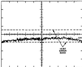
V = 200μV/DIV ( $V_{out} - V_{in}$ )
