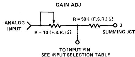
Unipolar & Bipolar: Apply a +(F.S. -3/2LSB) analog input and set the potentiometer for a digital output that alternates between 111...0 and 111...1.
