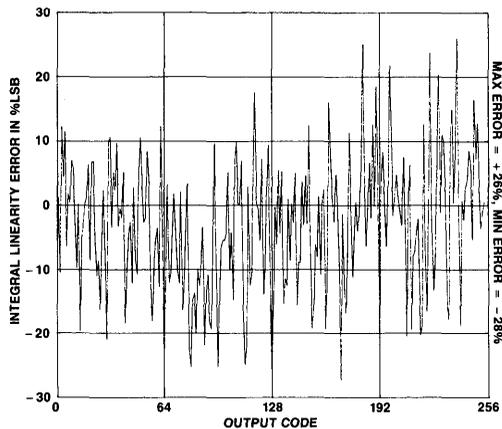
Figure 19. HS 168 Dynamic Integral Linearity Error
