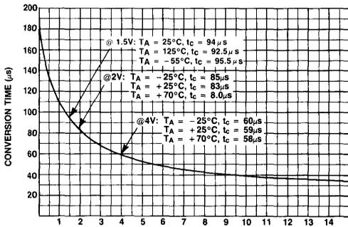
CONVERSION TIME VS. CONTROL VOLTAGE,  $T_A = +25^\circ\text{C}$
