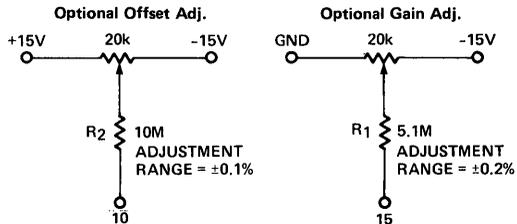
Values of R<sub>1</sub> & R<sub>2</sub> can be changed to increase or decrease the sensitivity of the adjustment. This adjustment should not be greater than ±1% around the nominal value for best performance.
