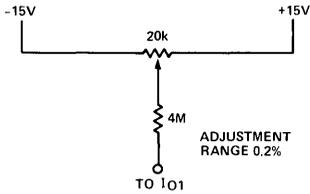
NOTE: External opamps have to be zeroed before the bipolar offset adjust circuit is connected.
