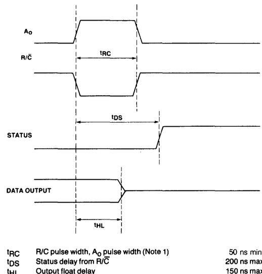
Figure 4. Timing Diagram to Start an 8-Bit Conversion
