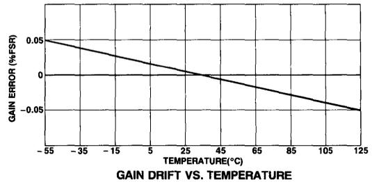
GAIN DRIFT VS. TEMPERATURE
