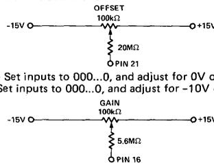
Unipolar - Set inputs to 000...0, and adjust for 0V output.
