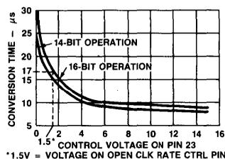
Figure 9. Conversion Time Vs. Clock Rate Control Voltage
