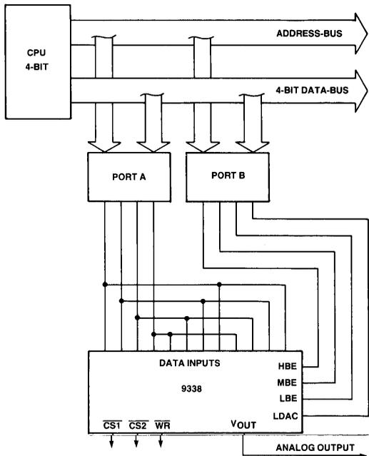
This figure shows how to operate the HS 9338 with two 4-Bit ports. The chip-selects are tied to ground allowing continuous operation; they can be used for operating more DAC's at the same port. In the first step data should appear at the port A outputs; in the second step the control flags should appear on port B.
