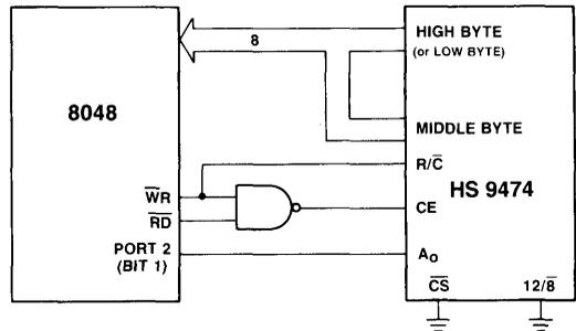
Figure 11B. Interfacing HS 9474 to 8048  $\mu$ P (Bottom)
