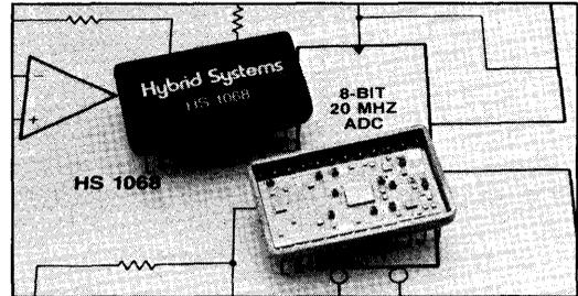
Designed to meet demanding military applications, the HS1068 is housed in a hermetic 24-pin DIP and operates with guaranteed performance over the full  $-55^{\circ}\text{C}$  to  $+125^{\circ}\text{C}$  case operating temperature range. Processing in compliance with MIL-STD-883C is available.
