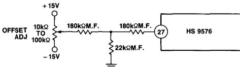
Figure 3. Low Tempco Adjustment Circuit
