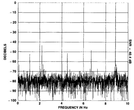
Figure 13. FFT of HS 1068,  $F_{IN}=8.9$  MHz,  $F_S=20$  MHz
