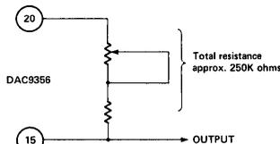
\*TC of external resistors must be between 0 and +50ppm/°C to maintain drift performance.
