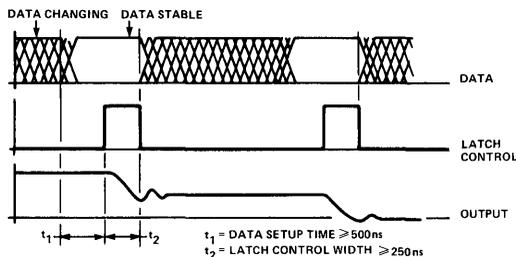
When loading the DAC from an 8-bit computer bus, optimum dynamic response will be obtained when the MSB segment is loaded first, followed by the LSB segments. This sequence allows the MSB's to settle while loading the LSB's. Note that this loading sequence is necessary only when the processor cycle time is longer than the DAC settling time. If the processor cycle time is shorter than the DAC settling time, the bits may be loaded in any sequence.
