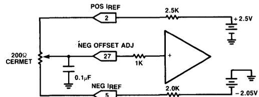
Figure 1. Simple Unipolar Range Offset Adjustment Circuit
