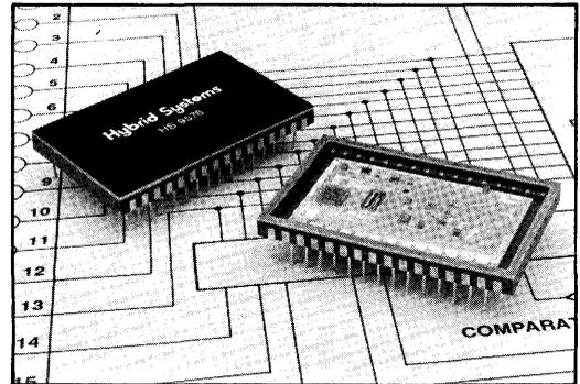
The HS9576 is a versatile building block for high-accuracy, high-speed systems. When used with the HS9716 sample (track)/hold, a high-speed acquisition system is formed which can digitize signals at a rate of 50,000 conversions per second. The HS9576 is available for operation over the commercial ( $0^\circ\text{C}$  to  $+70^\circ\text{C}$ ) temperature range or  $-55^\circ\text{C}$  to  $+125^\circ\text{C}$  with full MIL-STD-883C screening.
