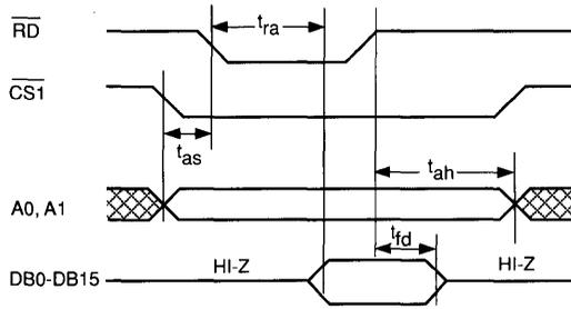
$t_{as}$  = address set-up time = 20 ns min.
