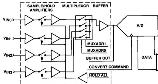
Figure 3A. Simultaneous Sampling DAS Using HS 9704
