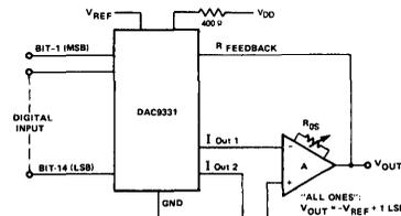
NOTE: To maintain specified DAC9331 linearity, the external amplifier (A) must be zeroed. Apply an ALL "ZEROS" digital input and adjust  $R_{OS}$  for  $V_{OUT} = 0 \pm 1mV$ .
