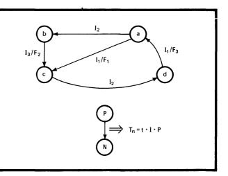
**5. State diagram.** Example of a state diagram (a) with four states— A, B, C, and D.  $I_1-I_3$  are jump conditions, which trigger output changes  $F_1-F_3$ . A state change (b) gives rise to transition term  $T_n$ , which is logical AND of clock t, input I, and present state P.
