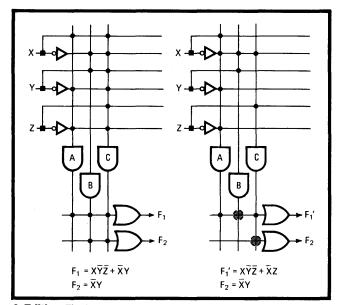
**3. Editing.** The logic array's programmable OR gates allow sharing of AND gates, as with gate B at left. The OR array also allows easy editing of logic statements when design changes are made; note how spare gate C at right was used to modify output  $F_1$  to  $F_1'$ .
