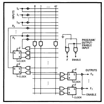
**6. Sequencer.** The field-programmable logic sequencer has 16 outputs, 48 AND gates, and 28 OR gates, plus 14 flip-flops that serve as state and output registers. Either an asynchronous preset input or an output-enable input is available as a programming option.
