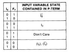
Note that 2 tests are required to uniquely determine the state of the input variable contained in the P-term.
