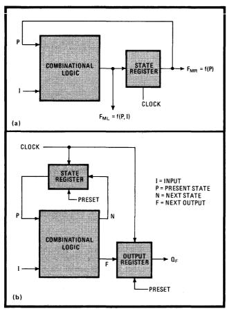
**4. State machine.** A state machine (a) takes either a Mealy or Moore form. The architecture of the field-programmable logic sequencer (b) is that of a self-contained Mealy machine, where the output is a function of both the present state and the present input.
