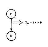
Figure 3: Typical state transition between any two states of Figure 2. The arrow connecting the two states gives rise to a transition term  $T_n$ . I is the jump condition.
