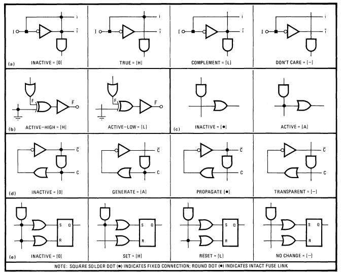
**1. New notation.** The many combinations of blown and unblown fuse links in the field-programmable logic family require new notation. The four possibilities for AND gates are shown in (a), while those for exclusive-OR outputs are in (b). The combinations for OR gates are in (c). The complement array in the logic sequencers is detailed in (d). Finally, OR gates controlling the flip-flops in sequencers are in (e).
