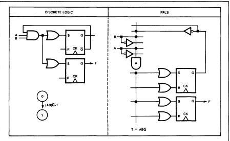
Figure 4: Typical state jump from state (0) to state (1), if inputs A=B="1". The jump also forces F="1", as required.
