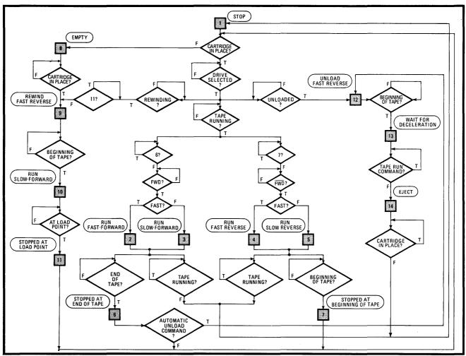
5. Goes with the flow. The first step in designing the controller is preparing a flow chart of the operation. The chart is much easier to understand than a state diagram or Mealy machine, yet provides all the information needed for programming the logic-sequencer chip.
