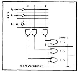
**1. Gate array.** The simplest device in Signetics' field-programmable logic is the gate array, capable of single-level logic. Any of 16 inputs can connect to nine NAND gates by true/complement buffers. Since outputs can be complemented to AND, manipulating De Morgan's theorem makes the device a universal logic element.
