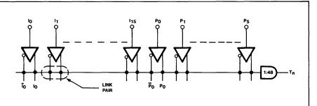
Figure 6: Typical AND gate coupled to (I) and (P) inputs. If at least one link *pair* remains intact,  $T_n$  is unconditionally forced Low.
