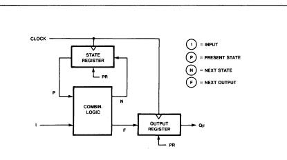
Figure 1: Basic architecture of 82S104/105 FPLS. I, P, N, and F are multi-line paths denoting groups of binary variables programmed by the user.
