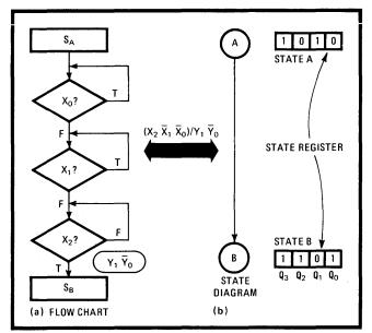
**6. Flow chart to state diagram.** Simple transition from state A to state B is shown in flow chart (a). Three inputs  $(X_0, X_1, X_2)$  and two outputs  $(Y_0, Y_1)$  are assumed. The contents of a four-bit state register show the transition from state A (1010<sub>2</sub>) to state B (1101<sub>2</sub>).
