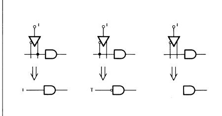
Figure 7: Choice of input polarity coupling to a typical AND gate. With both links open, (I) is logically Don't Care.
