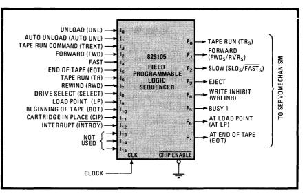
4. Tape controller. A field-programmable logic sequencer like this tape controller can perform extremely complex tasks. The 82S105 receives commands from an input/output bus or monitor, and provides all the necessary signals for driving the tapetransport servo-motor mechanism.
