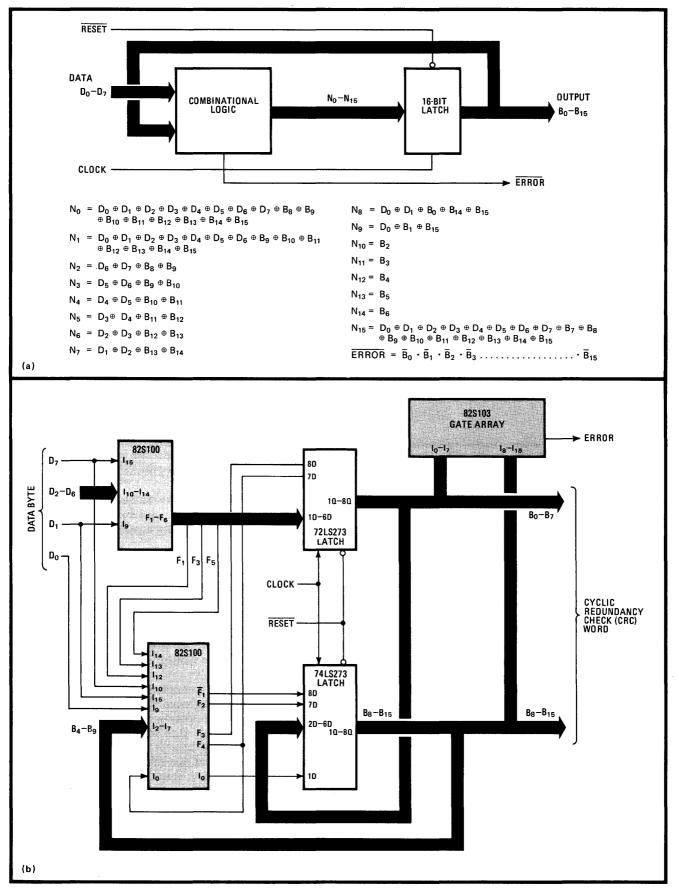
**3. Error-free.** The technique of using a cyclic redundancy check (CRC) word for error-free data transmission requires complex logic to generate the word (a). A pair of logic arrays, two latches, and a gate array (b) do the job, which usually requires a boardful of chips.
