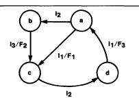
Figure 2: Typical state diagram.  $I_{1-3}$  are jump conditions which must be satisfied before any transitions take place.  $F_r$  are changes in output triggered by  $I_m$ , and stored in the Output Register. State transitions  $a \rightarrow b$  and  $c \rightarrow d$  involve no output change.
