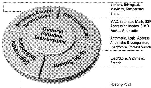
**Figure 1: TriCore: A Modular Instruction Set Architecture**
