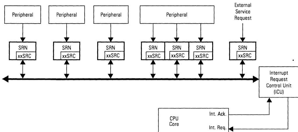
**Figure 38: Block Diagram of Interrupt System**
