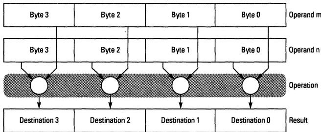
**Figure 53: Packed Byte Data Format**
