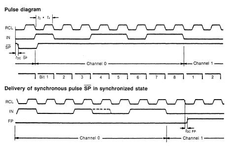
Delivery of fault pulse FP in the event of erroneous frame alignment signal
