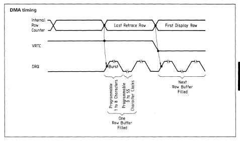
The DMA controller is typically initialized for the next frame at the end of the current frame.
