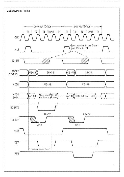
Status bits  $\overline{S0}$ ,  $\overline{S1}$ , and  $\overline{S2}$  are used by the bus controller, in maximum mode, to identify the type of bus transaction according to the following table:
