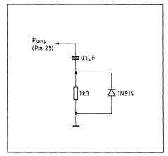
Since  $5^{1}/_{4}$ " Drives operate at exactly one-half the data rate (250 Kbytes/sec) the above capacitor should be doubled to 0.2 or 0.22  $\mu$ F.
