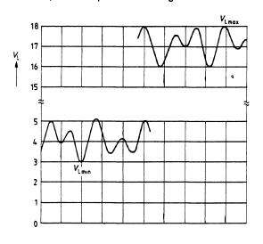
Minimal/maximal peak line voltage
