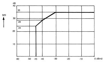
SIGNAL-TO-TOTAL DISTORTION Measured with sine-wave in the range 700-1100Hz, excluding submultiples of 8kHz
