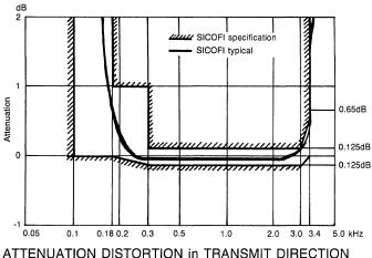
ATTENUATION DISTORTION in TRANSMIT DIRECTION Reference frequency is 1kHz Input signal level is φdBmφ
