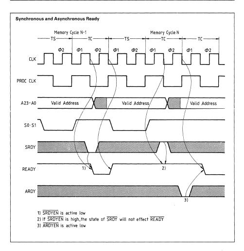
ARDY or ARDYEN must be HIGH at the end of TS. ARDY cannot be used to terminate a bus cycle with no wait states.
