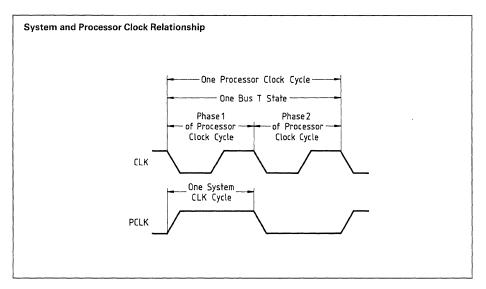
Six types of bus operations are supported: memory read, memory write, I/O read, I/O write, interrupt acknowledge, and halt/shutdown. Data can be transferred at a maximum rate of one word per two processor clock cycles.
