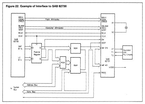
RAM or ROM may be selected either by addresses or by control signals. For pipeline register use positive edge triggered D-Flipflops (non-transparent latch) like SN 74374.
