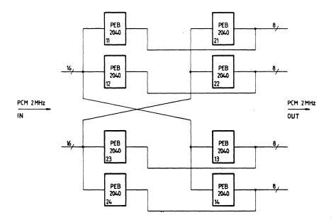
Memory time switch 32/32 for a non blocking 1022 channel switch using the tristate function.
