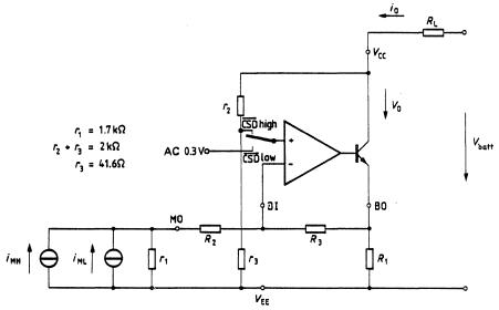
The internal feedback loop is normally closed ( $r_2$ ,  $r_3$ , positive input of output amplifier). If the current sink is disabled, the positiv input of the output amplifier is supported with a fixed voltage of about 0.3 V. This voltage is derived from the internal reference voltage.
