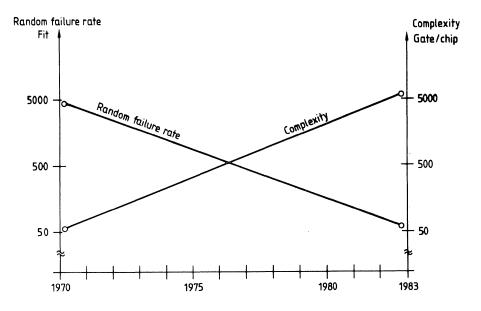
Figure 2 shows the general course of the failure rate for digital MOS ICs in fit for the years 1970 to 1983. The increasing complexity as regards gate functions/chip is also specified.
