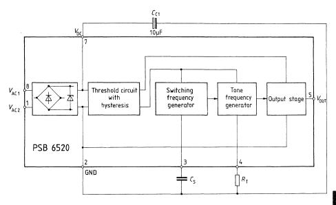
The IC contains an oscillator which generates a square wave voltage. The frequency of this voltage is periodically switched by a second oscillator back and forth between two basic values having a ratio of 1 : 1.38. The basic frequency  $f_{1T}$  is adjusted by the resistor  $R_T$  and the switching frequency  $f_s$  by the capacitor  $C_s$  (fig. 12 and 13).
