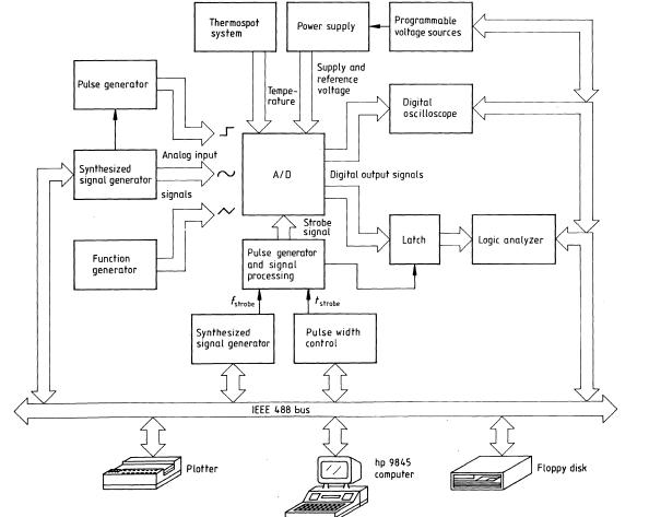
Computer supported test setup
