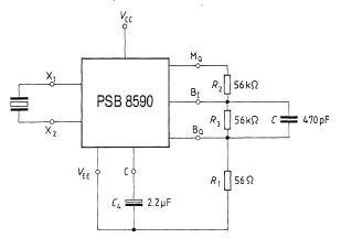
In order to keep the insertion loss for all the DTMF frequencies less than 0.2 dB the 3 dB cutoff frequency of the filter should be at least 6 kHz.
