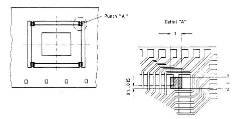
Lay down the punched MICROPACK onto an electrically conductive surface vacuum pickup. Coat the mounting points on the substrate with flux (with brush by hand).
