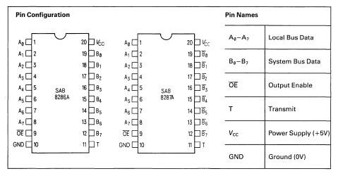
The SAB 8286A and SAB 8287A are 8-bit bipolar transceivers with 3-state outputs. The SAB 8287A inverts the input data at its outputs while the SAB 8286A does not. Thus, a wide variety of applications for buffering in microcomputer systems can be met. This device is fabricated in a fast bipolar ASBC (Advanced Standard Buried Collector) process of Siemens.
