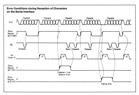
1) Character format for this example: 6 Data bits without Parity and one Stop bit
