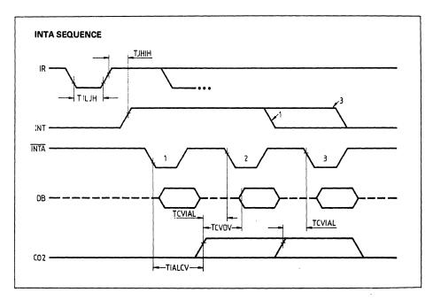
Notes: Interrupt output must remain HIGH at least until leading edge of first INTA. 1. Cycle 1 in SAB 8086/88 systems, the Data Bus is not active.
