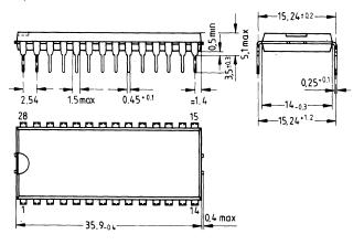
Plastic plug-in package 20 B 28 DIN 41866, 28 pins, DIP
