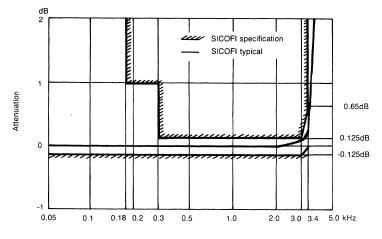
ATTENUATION DISTORTION in RECEIVE DIRECTION Reference frequency is 1kHz Input signal level is ødBmø
