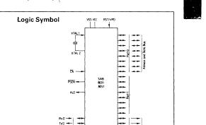
The SAB 8031/8051 is a stand-alone, high-performance single-chip computer fabricated in +5V advanced N-channel, silicon gate Siemens MYMOS technology and packaged in a 40-pin DIP. It provides the hardware features, architectural enhancements and new instructions that are necessary to make it a powerful and cost effective controller for applications requiring up to 64K bytes of program memory and/or up to 64K bytes of data storage.
