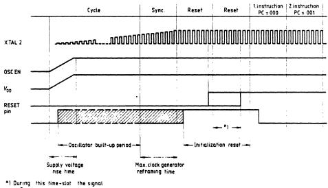
at Reset-pin can change to V<sub>DD</sub> without lengthening the Reset execution
