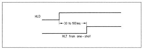
When both HLD and HLT are true, the SAB 279XA will then read from or write to the media. The "And" of HLD and HLT appears as status bit 5 in Type I status.
