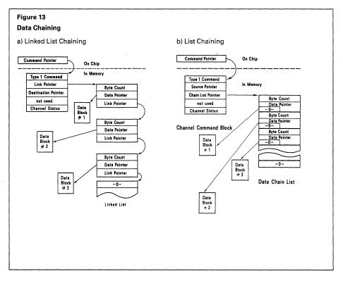
In the case of linked list chaining (see figure 13 a) each data block has a descriptor containing information on position of data block in memory, length of data block, and a pointer to the next description.
