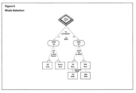
SAB 82258 can also operate in a remote or stand alone mode where it is not coupled directly to a processor. Figure 5 shows the way how SAB 82258 detects with which processor or in which mode it is operating. Figure 2 shows the logic pinning in the 286 mode – for operation with SAB 80286. Figure 3 shows the logic pinning in the 186 mode – for operation with SAB 80186/188 and SAB 8086/88, and Figure 4 shows the pinning when SAB 82258 is in the remote mode and not directly coupled to a processor.
