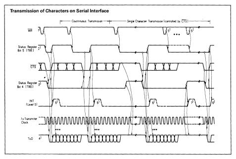
1) Load Transmitter buffer register
