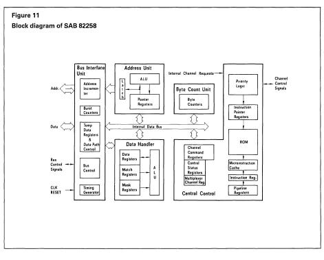
The ADMA supports two address spaces, memory space and I/O space, each with a maximum address range of 16 Mbytes. In addition, the maximum
