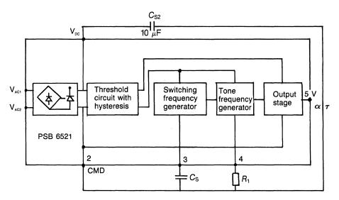
The IC contains an oscillator which generates a square wave voltage. The frequency of this voltage is periodically switched by a second oscillator back and forth between two basic values having a ratio of 1 : 1.25. The basci frequency  $f_{1\tau}$  is adjusted by the resistor  $R_{\tau}$  and the switching frequency  $f_s$  by the capacitor  $C_s$  (Figs. 12 and 13).
