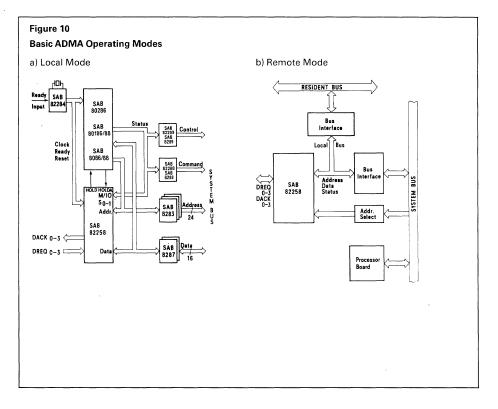
SAB 82258 has four independent DMA channels that can transfer up to 8 Mbytes/sec in the single cycle mode (2 clocks/transfer). In the 2 cycle transfer mode the maximum rate is 4 Mbytes/sec. Switching between channels induces no time penalty. Thus the overall maximum transfer rate of 8 Mbytes/sec is also valid for multiple channel operation.
