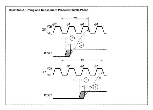
1) When RESET meets the setup time shown, the next CLK will start or repeat  $\emptyset$  2 of a processor cycle.
