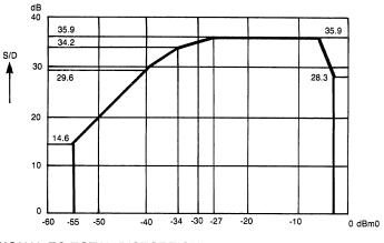
SIGNAL-TO-TOTAL DISTORTION Measured with noise signal
