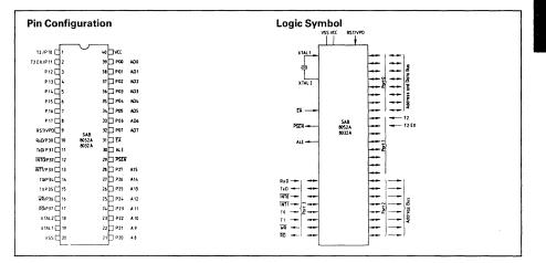
The SAB 8032A/8052A is a stand-alone, high-performance single-chip microcomputer fabricated in +5V advanced N-channel, silicon gate Siemens MYMOS technology, packaged in a 40-pin DIP. It is upward compatible with the SAB 8031A/8051A. It provides the hardware features, architectural enhancements, and instructions that are necessary to make it a powerful and cost effective controller for applications requiring up to 64 Kbytes of program memory and/or up to 64 Kbytes of data memory.
