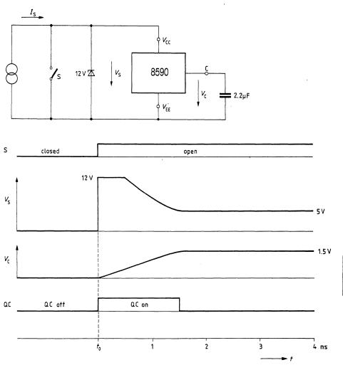
The control circuitry for the quick charging circuit has hysteresis with the following thresholds  $\label{eq:control}$
