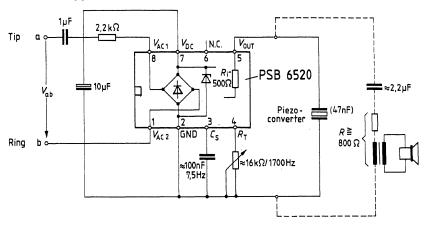
Fig. 3 PSB 6520 application circuit for telephone sets.
