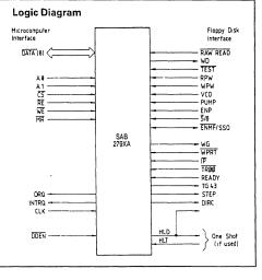
SAB 279XA is a floppy disk controller family of N-channel MOS LSI components designed to interface with SAB 8080/8051 family processors. Its flexibility and ease of use makes it an ideal floppy disk interface between conventional floppy disks and all computer systems. Software compatible with its predecessor, the SAB 179X, the device also contains a high performance PhaseLock-Loop Data Separator as well as Write Precompensation Logic.
