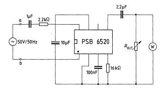
Fig. 7 Test circuit to determine output power for variable call voltage  $V_{\rm ab}$
