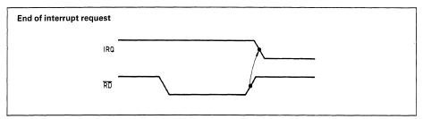
A reset command will also cause IRQ to go inactive, but this is not recommended during normal service.
