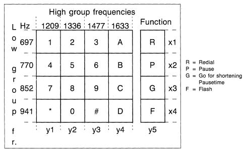
The position of the 4 Special-Keys is in the device mask-programmable.
