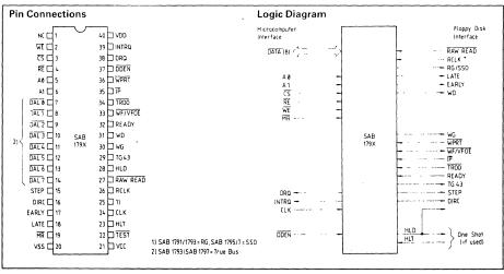
SAB 179X is a floppy disk controller family of N-channel MOS LSI components designed to interface with SAB 8080/8085/8086/8051 family processors. Its flexibility and ease of use makes it an ideal floppy disk interface between conventional floppy disks and all computer systems.
