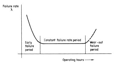
Reliability tests for ICs are usually destructive examinations. They are, therefore, carried out with samples. Most failure mechanisms can be accelerated by means of higher temperatures. Due to the temperature dependence of the failure mechanisms, it is possible to simulate a future operational behavior within a short time by applying high temperatures; this is called life test.
