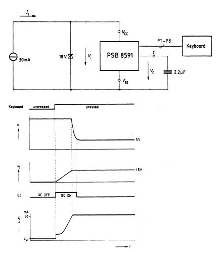
The control circuitry for the quick charging circuit has a hysteresis with the following thresholds:
