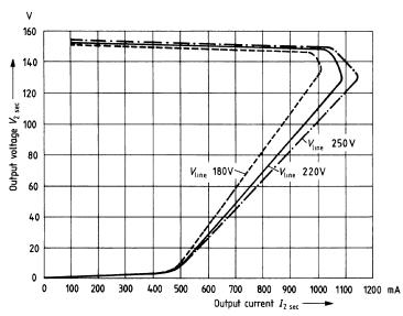
Load characteristic  $V_{2 \text{ sec}}$  versus output current  $I_{2 \text{ sec}}$
