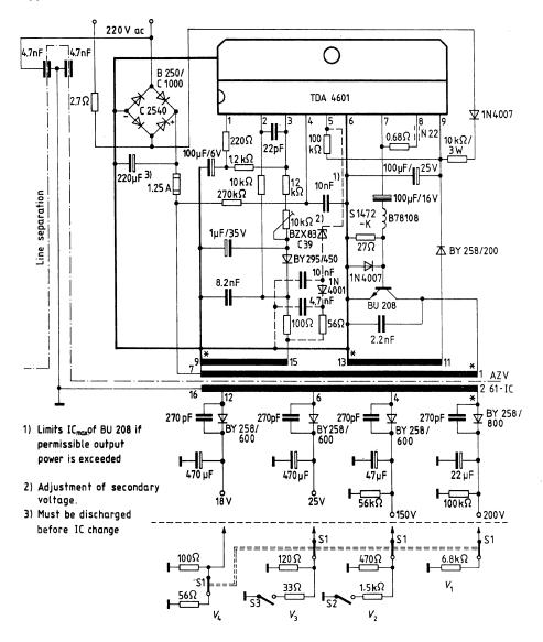
\_ \_\_ Protective circuit to prevent increase of secondary voltage when fault occurs
