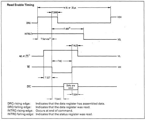
$^{11}$   $\overline{\text{CS}}$  may be permanently tied LOW if desired.
