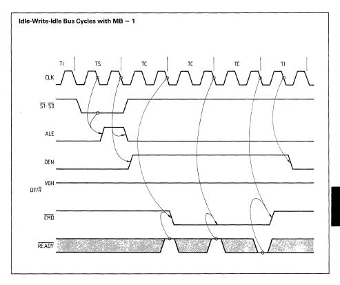
The MB control input affects the timing of the command and DEN outputs. These outputs are automatically delayed in Multipus mode to satisfy three requirements:
