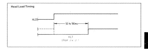
When both HLD and HLT are true, the SAB 179X will waits for HLT to be true. If h = 1 and V = 1, then read from or write to the media. The "and" of HLD and HLT appears as a status bit in Type I status. HLD and HLT appears as a status bit in Type I been issued, an internal 15 ms delay occurs
