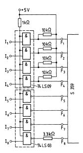
The inputs  $I_1$  to  $I_4$  control the frequencies of the lower frequency group  $f_1 - f_4$  and the inputs  $I_5$  to  $I_8$  control the frequencies of the higher frequency group. For the generation of a dual tone, one input of  $I_1$  to  $I_4$  of the lower group and one input of  $I_5$  to  $I_8$  of the higher group must have an H-level.
