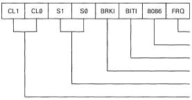
Timer Input Frequency Processor Type Select Source for Interrupt Level 1 Break-In Detect Enable Stop Bit Length Character Length
