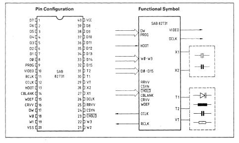
The SAB 82731 is a general purpose video interface, which generates a video signal output for the CRT monitor from parallel character and attribute information coming from the character generator and the CRT controller. The SAB 82731 together with minimal hardware, comprises a complete video interface system for the CRT controller and the CRT monitor. The device is fabricated in a fast bipolar ASBC (Advanced Standard Buried Collector) process of Siemens.
