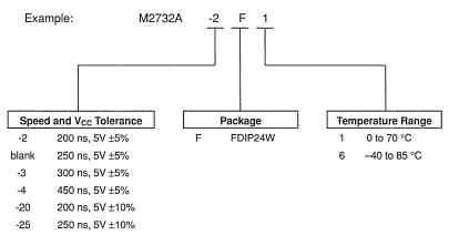
For a list of available options (Speed,  $V_{CC}$  Tolerance, Package, etc...) refer to the current Memory Shortform catalogue.
