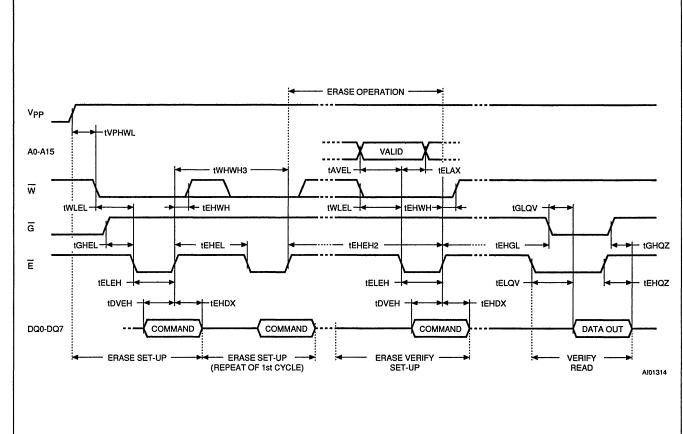
Figure ö Erase Set-up and Erase Verify Commands Waveforms, m Controlled
