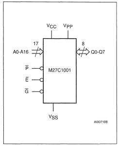
Figure 2A. DIP Pin Connections
