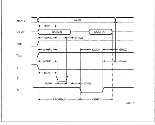
Figure 6. Programming and Verify Modes AC Waveforms
