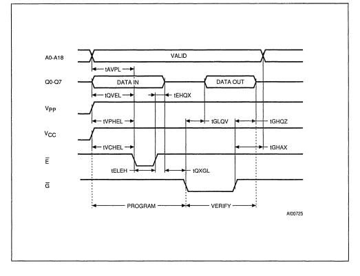
Figure 6. Programming and Verify Modes AC Waveforms
