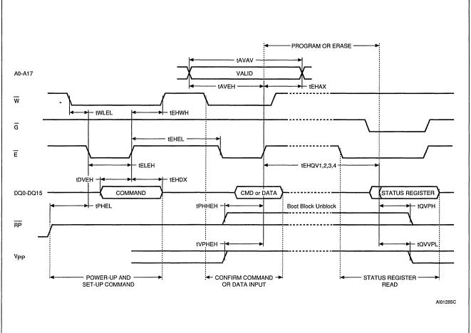
Figure 7 Program & Erase AC Waveforms, m Controlled
