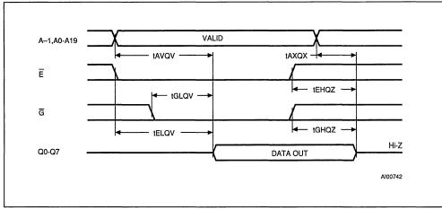
Figure 4. Byte-Wide Read Mode AC Waveforms
