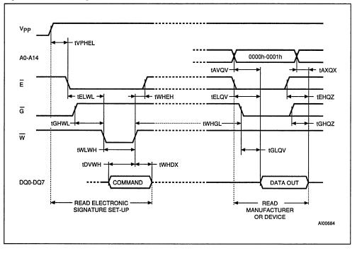
Figure 7. Electronic Signature Command Waveforms
