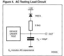
Note: For 55ns class: input pulse voltages are 0V to 3V, input output test points are at 1.5V, CL is 30 pF.
