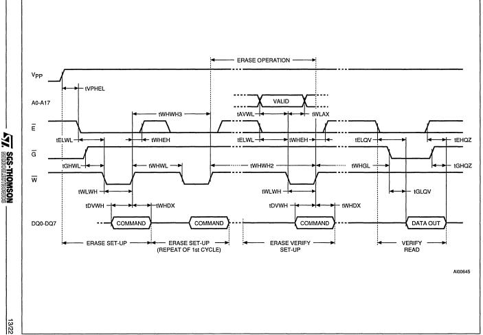
Figure 8. Erase Set-up and Erase Verify Commands Waveforms,  $\overline{\mathbf{W}}$ Controlled
