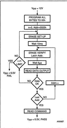
Figure 12. Erasing Flowchart
