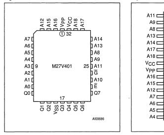
Figure 2B. TSOP Pin Connections
