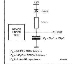
Figure 4. AC Testing Load Circuit
