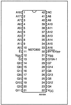
Figure 2B. SO Pin Connections
