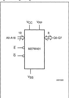
Figure 2A. LCC Pin Connections
