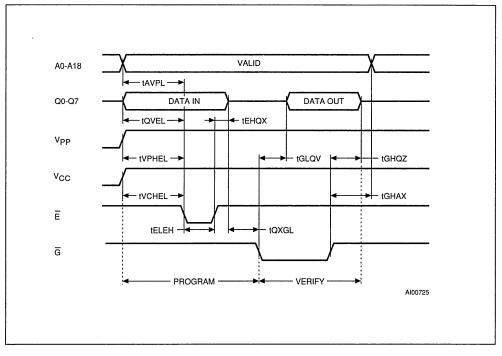
Figure 6. Programming and Verify Modes AC Waveforms
