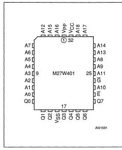
Figure 2B. TSOP Pin Connections
