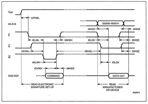
Figure 7. Electronic Signature Command Waveforms
