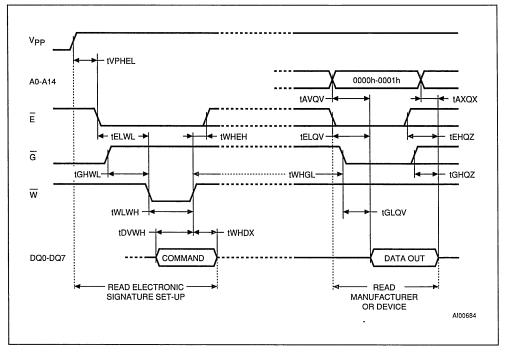
Figure 7. Electronic Signature Command Waveforms
