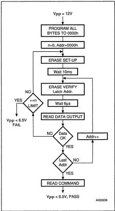
Figure 12. Erasing Flowchart
