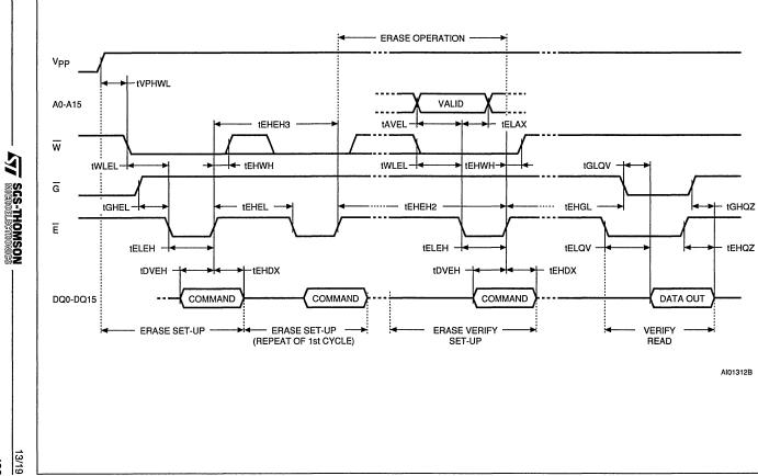
Figure . Ģ Erase Set-up and Erase Verify Commands Waveforms, m Controlled
