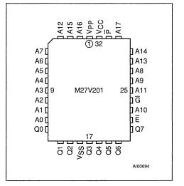
Figure 2A. LCC Pin Connections
