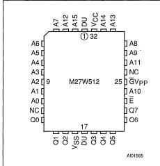
Figure 2A. LCC Pin Connections
