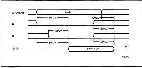
Figure 4. Byte-Wide Read Mode AC Waveforms
