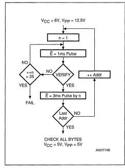
Figure 8. Fast Programming Flowchart
