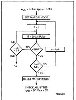
for reliability. Before starting the programming the internal MARGIN MODE circuit is set in order to guarantee that each cell is programmed with enough margin.
