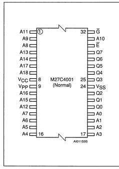
Figure 2B. LCC Pin Connections
