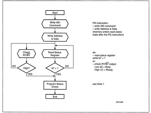
Note: 1. Status check of b7 can be made after each byte programming or after a sequence.
