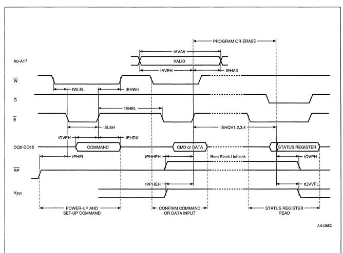
Figure 9. Program & Erase AC Waveforms, E Controlled
