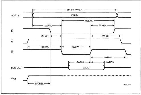
Figure 7. Write AC Waveforms, W Controlled
