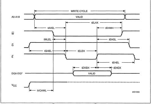
Figure 8. Write AC Waveforms, E Controlled
