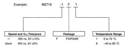
For a list of available options (Speed,  $V_{CC}$  Tolerance, Package, etc...) refer to the current Memory Shortform catalogue.
