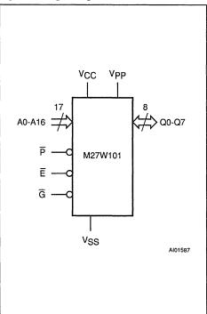
Figure 2A. LCC Pin Connections
