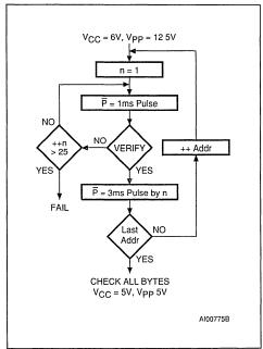
continually monitored to determine when it has been successfully programmed. A flowchart of the M27128A Fast Programming Algorithm is shown on the last page. The Fast Programming Algorithm utilizes two different pulse types: initial and overprogram.
