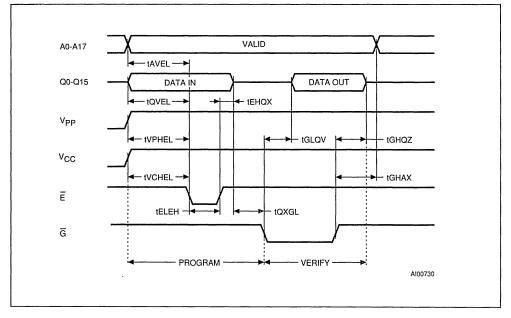
Figure 6. Programming and Verify Modes AC Waveforms
