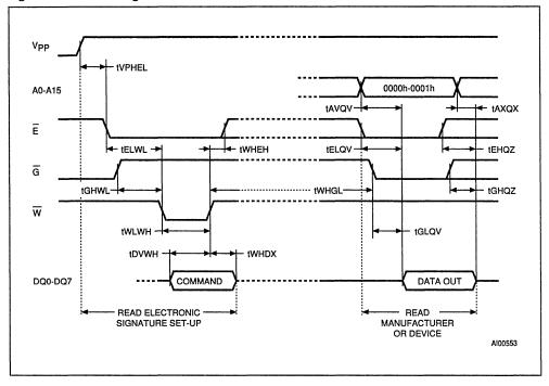
Figure 7. Electronic Signature Command Waveforms
