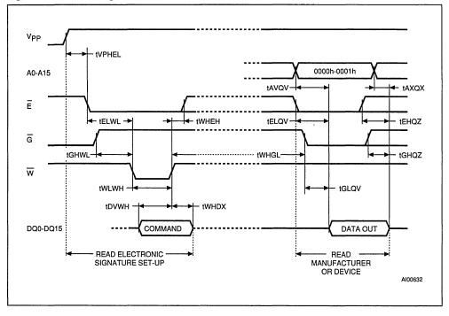
Figure 7. Electronic Signature Command Waveforms
