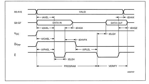
Figure 7. Programming and Verify Modes AC Waveforms
