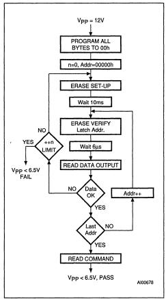
Figure 12. Erasing Flowchart
