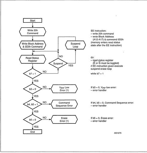
Note: 1. If VPP Low or Erase Error is found, the Status Register must be cleared (CLRS instruction) before further P/E.C. operations.
