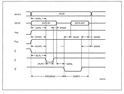
Figure 6. Programming and Verify Modes AC Waveforms
