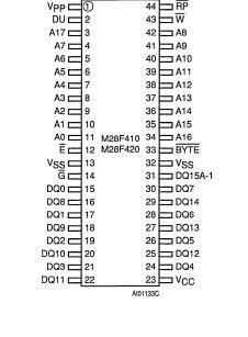
Figure 2B. SO Pin Connections
