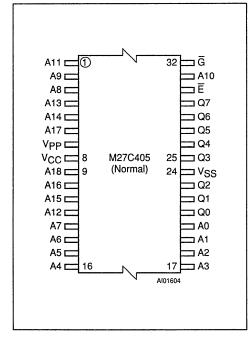
Figure 2B. LCC Pin Connections
