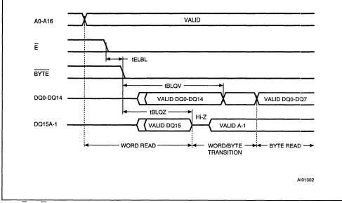
Note:  $\overline{G}$  Low,  $\overline{W}$  = High, other timings as Read Mode AC waveforms.
