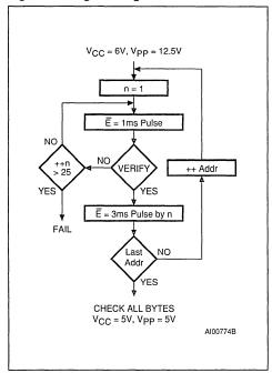
to a particular M27256 location), before a correct verify occurs. Up to 25 one-millisecond pulses per byte are provided for before the over program pulse is applied. The entire sequence of program pulses and byte verifications is performed at  $V_{CC} = 6V$  and  $V_{PP} = 12.5V$ .
