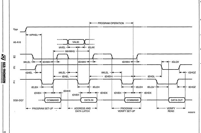
Figure 11. Program Set-up and Program Verify Commands Waveforms, m Controlled
