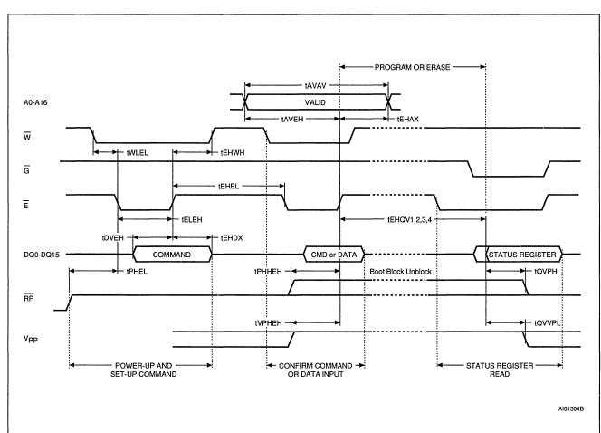
Figure 9. Program & Erase AC Waveforms, m Controlled
