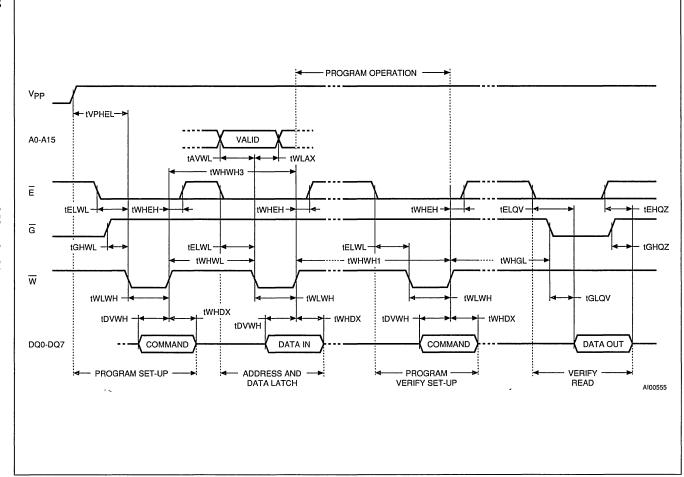
Figure 10. Program Set-up and Program Verify Commands Waveforms,  $\overline{W}$  Controlled
