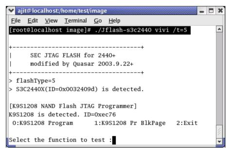
Figure 5-2 selecting function to test Jflash-s3c2440
