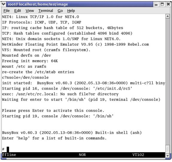
Figure 4-7 Booting Target Board
