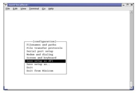
Figure 4-5 saving Minicom Setup
