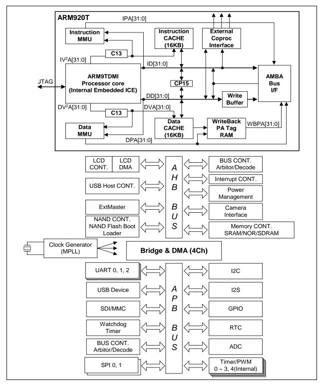
Figure 1-1 S3C2440X Block Diagram
