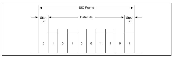
Figure 11-4. Serial I/O Frame Timing Diagram (Normal UART)
