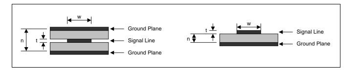
Transmission line capacitance, Inductance, Z0 and TPD can be calculated with PCB size and material dielectric constant.
