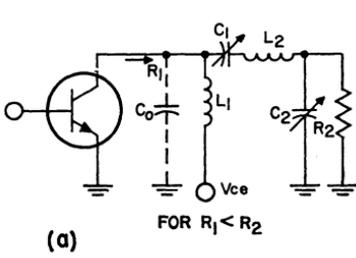
(1)  $X_{C1} = Q_L R_1$     (2)  $X_{C2} = \frac{R_2}{\sqrt{\frac{R_2(Q_L^2 + 1)}{R_1 Q_L^2} - 1}}$
