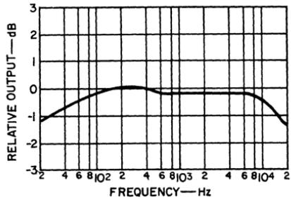
Figure 457. Relative response of the bridge audio amplifier.
