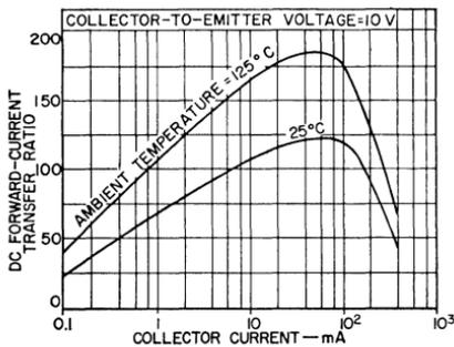
Figure 156. Typical dc forward-current transfer ratio ( $h_{FE}$ ) as a function of collector current for the 2N3053 silicon power transistor.
