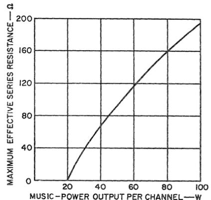
Figure 440. Maximum effective series resistance as a function of music power output.
