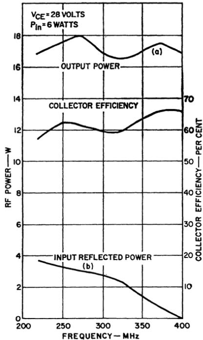
Figure 371. RF power output, input reflected power, and collector efficiency of the RCA 2N5016 transistor as functions of frequency.
