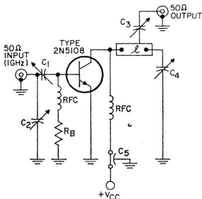
$C_1, C_2, C_3, C_4$  = Variable capacitor, 0.3 to 3.5 pF, Johanson piston type or equiv.
