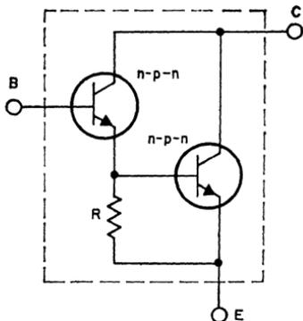
Figure 427. Darlington connection of n-p-n driver transistor to n-p-n output transistor.
