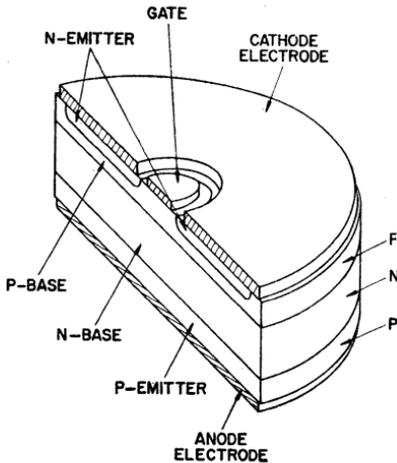
Figure 36. Cross-section of a typical SCR pellet.
