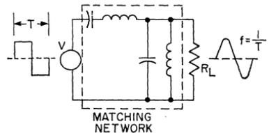
Figure 465. Use of a transducer and resonant matching network to convert a square-wave input to a sinusoidal output. Reactive component of transducer is used as the shunt inductor or capacitor of the matching network depending upon whether a magnetostrictive or electrostrictive type of transducer is used.
