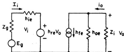
Figure 124. Terminated h-parameter equivalent circuit for a transistor used in a common-emitter configuration.
