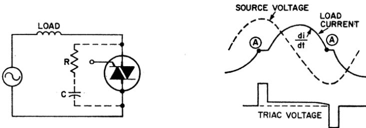
Figure 65. Simplified diagram and voltage and current waveforms for operation of a triac in a circuit that has an inductive load and a lagging-current power factor.
