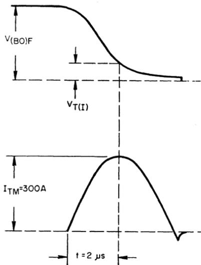
Figure 51. Initial ON-state voltage and current waveforms for the 2N3873 SCR.
