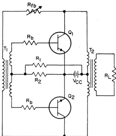
Figure 211. Two-transistor, two-transformer push-pull inverter that uses a resistive voltage-divider network to provide starting bias.
