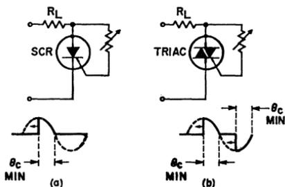
Figure 256. Degree of control over conduction angles when ac resistive network is used to trigger SCR's and triacs.
