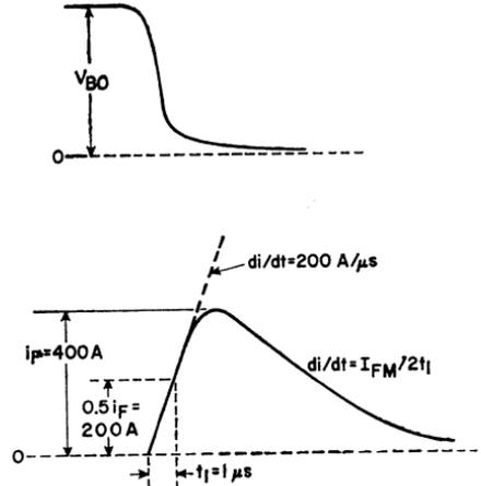
Figure 44. Voltage and current waveforms used to determine  $di/dt$  rating of the RCA-2N3873 SCR.
