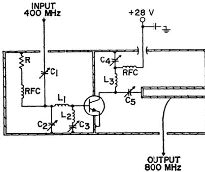
Figure 400. 400-to-800-MHz common-emitter transistor frequency multiplier.
