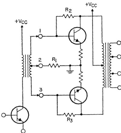
Figure 419. Class AB, push-pull, transformer-coupled audio output stage.
