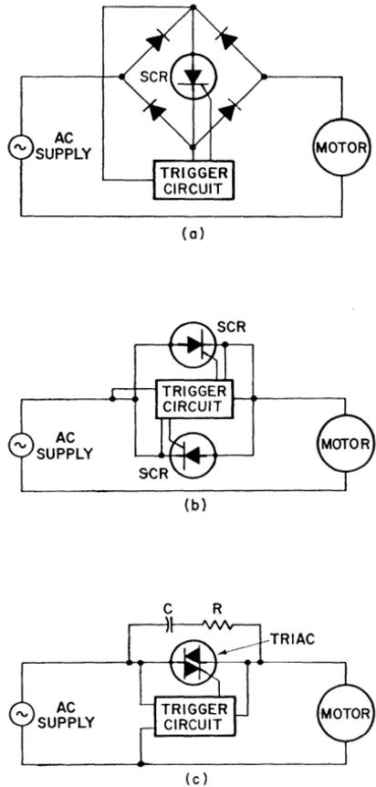
Figure 278. Full-wave thyristor motor control circuits: (a) Use of full-wave bridge rectifier to enable full-wave motor control by a single SCR; (b) Use of inverse parallel SCR's to provide full-wave motor control; (c) Use of triac to provide full-wave motor control.
