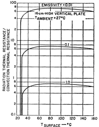
Figure 92. Ratio of radiation thermal resistance to convection thermal resistance as a function of heat sink surface temperature for various surface emissivities. (Reprinted from **Control Engineering**, October 1967.)
