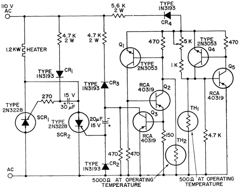
Figure 287. Full-wave zero-switching SCR heater control circuit.
