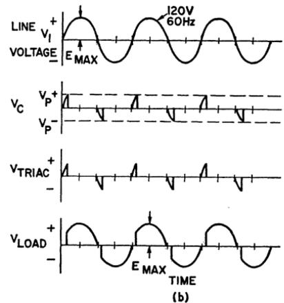
Figure 260. Voltage waveforms for circuit shown in Fig. 258: (a) thyristor in blocking state; (b) when thyristor is triggered at controlled intervals by triggering-device circuit.
