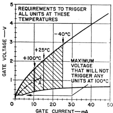
Figure 55. Gate-characteristics curves for a typical RCA SCR.
