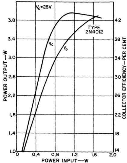
Figure 401. Output power and collector efficiency as a function of input power for the 400-to-800-MHz frequency doubler.
