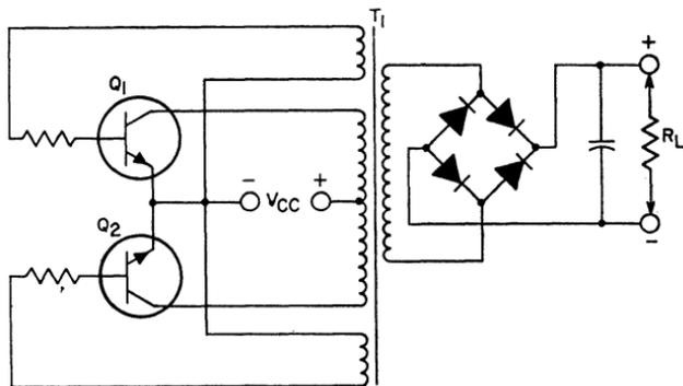
Figure 200. Basic circuit configuration of a single-transformer push-pull switching converter.
