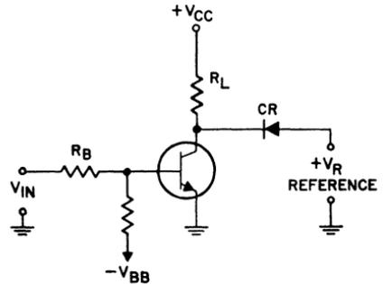
Figure 162. "Collector-catcher" circuit.
