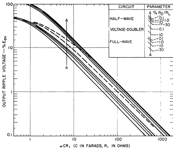
Figure 197. RMS ripple voltage in capacitor-input circuits.
