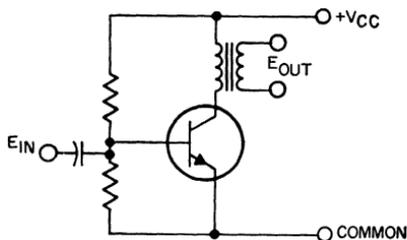
Figure 411. Basic class A, transformer-coupled amplifier.
