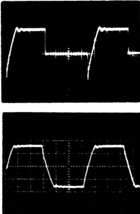
Figure 219. Typical operating waveforms for SCR inverter shown in Fig. 218.
