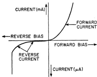
Figure 8. Voltage-current characteristic for a p-n junction.
