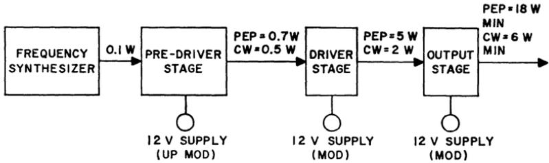
Figure 341. Block diagram of transmitter designed to deliver a minimum of 6 watts of rf power at 85-per-cent modulation for operation from a 12-volt airplane battery without converters.
