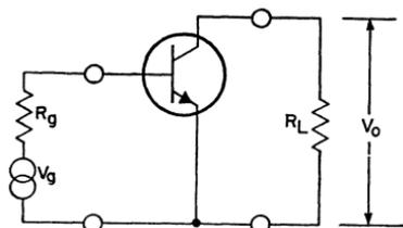
Figure 347. Common-emitter transistor amplifier.
