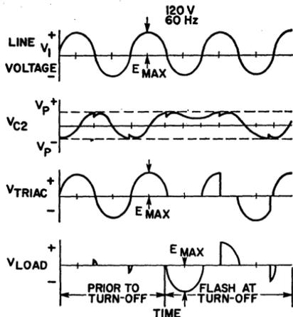
Figure 295. Waveforms during flash-at-turn-off condition in a double-time-constant phase-control circuit.
