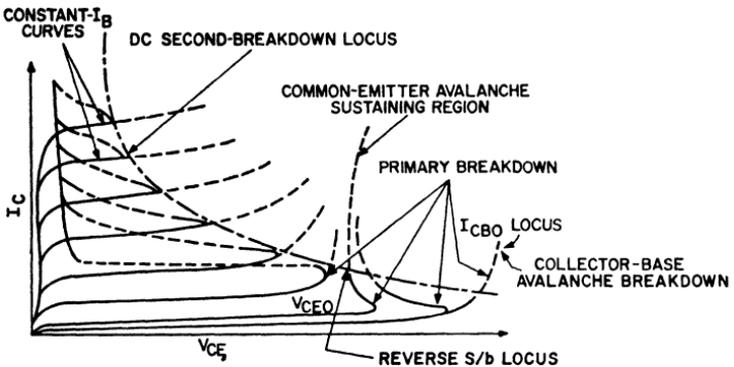
Figure 96. Transistor collector characteristics.
