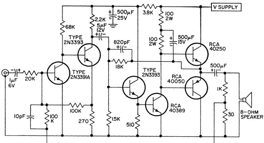
Figure 438. Class B complementary-symmetry power amplifier.
