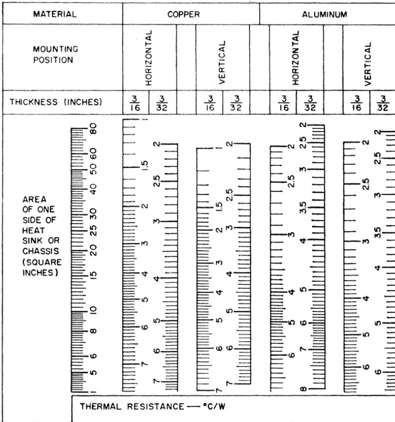
INSTRUCTION FOR USE: SELECT THE HEAT-SINK AREA AT LEFT AND DRAW A HORIZONTAL LINE ACROSS THE CHART FROM THIS VALUE. READ THE VALUE OF MAXIMUM THERMAL RESISTANCE DEPENDING ON THE THICKNESS OF THE MATERIAL, TYPE OF MATERIAL, AND MOUNTING POSITION. Figure 93. Thermal resistance as a function of heat-sink dimensions. (Nomograph reprinted from *Electronic Design*, August 16, 1961.)
