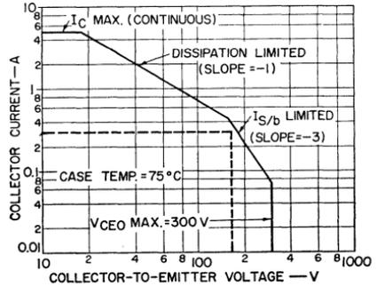
Figure 233. Safe-area curve for the RCA 2N5240 transistor. Dashed-line rectangle indicates that transistor operates within ratings in the 100-volt current-limiting (0.3 ampere) series-regulated power supply.
