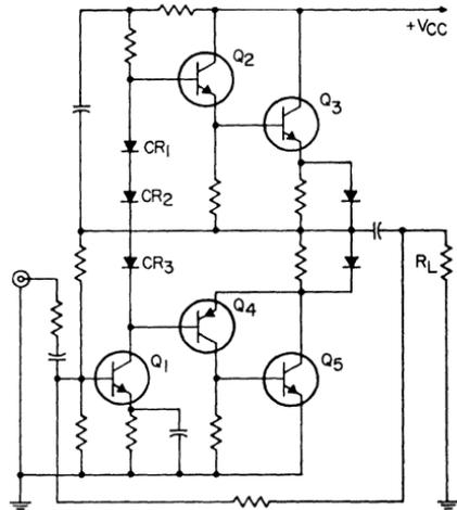
Figure 441. Quasi-complementary amplifier that incorporates two stabilization networks.
