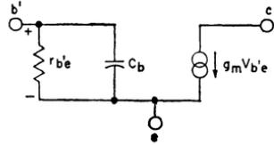
Figure 126. Elementary small-signal transistor equivalent circuit.
