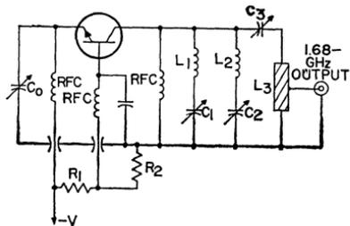
Figure 410. Oscillator-quadrupler circuit.
