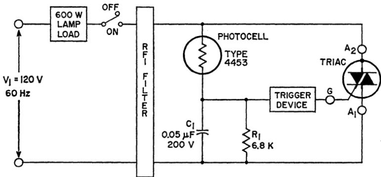
Figure 293. Photocell-operated on-off lamp control that energizes lamp load when photocell is illuminated.
