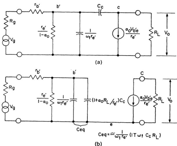
Figure 348. Equivalent circuits for common-emitter amplifier shown in Fig. 347: (a) without parasitic elements; (b) simplified equivalent circuit.
