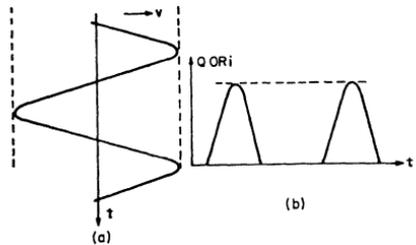
Figure 395. (a) Sinusoidal voltage developed by the amplifier section of an overlay transistor to drive the nonlinear collector-to-base capacitance; (b) distorted charge, or current, waveform produced by the nonlinear collector-to-base capacitance of an overlay transistor in the generation of harmonic power.
