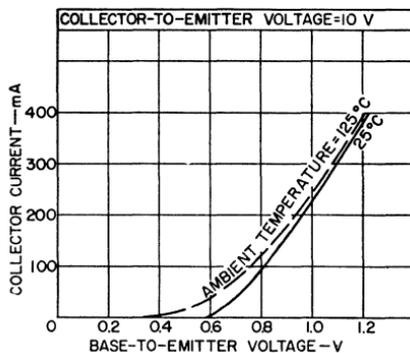
Figure 157. Typical transfer characteristics for the 2N3053 silicon power transistor.
