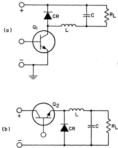
Figure 243. Basic transistor switching arrangements: (a) filter elements and load impedance in collector circuit of switching transistor; (b) filter elements and load impedance in emitter circuit of switching transistor.
