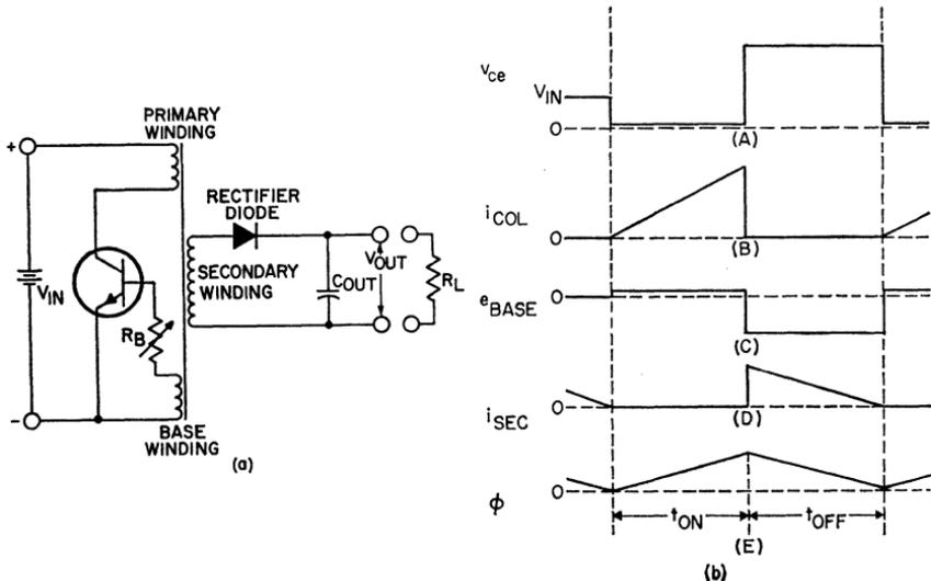
Figure 204. Ringing-choke converter: (a) Schematic diagram; (b) Typical operating waveforms in a ringing-choke converter—(A) primary voltage; (B) primary current; (C) base-to-emitter voltage; (D) secondary current; (E) magnetic flux in transformer core.
