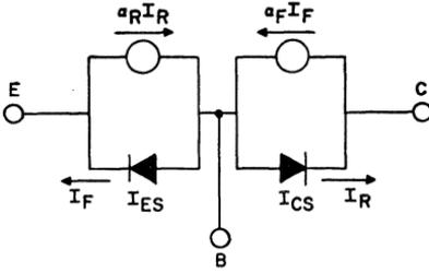
Figure 153. Ebers-Moll model of an n-p-n transistor controlled by diode currents.
