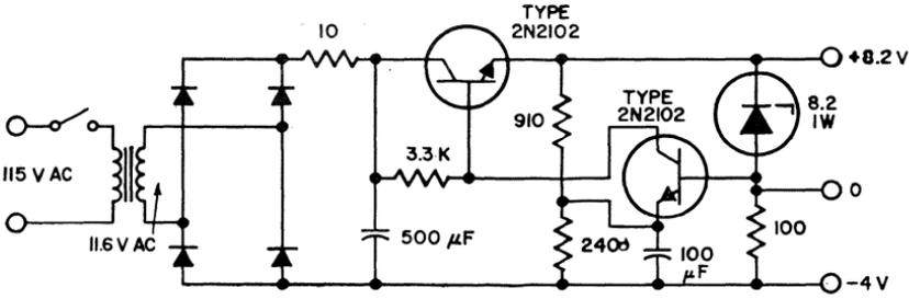
Figure 235. Schematic diagram of reference voltage supply for regulated power supply shown in Fig. 234.
