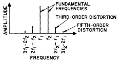
Figure 330. Frequency spectrum showing the frequency relationship of some distortion products to two test signals  $f_1$  and  $f_2$ .
