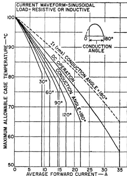
Figure 40. Current rating chart for the RCA-2N3873 SCR.
