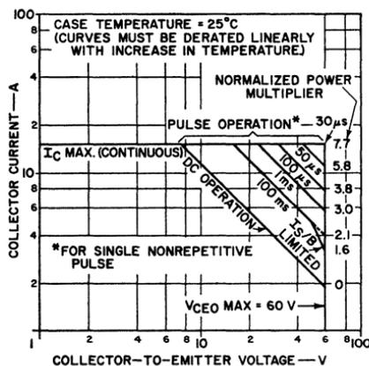
Figure 95. Maximum-operating-area curves for the 2N3055 silicon power transistor.
