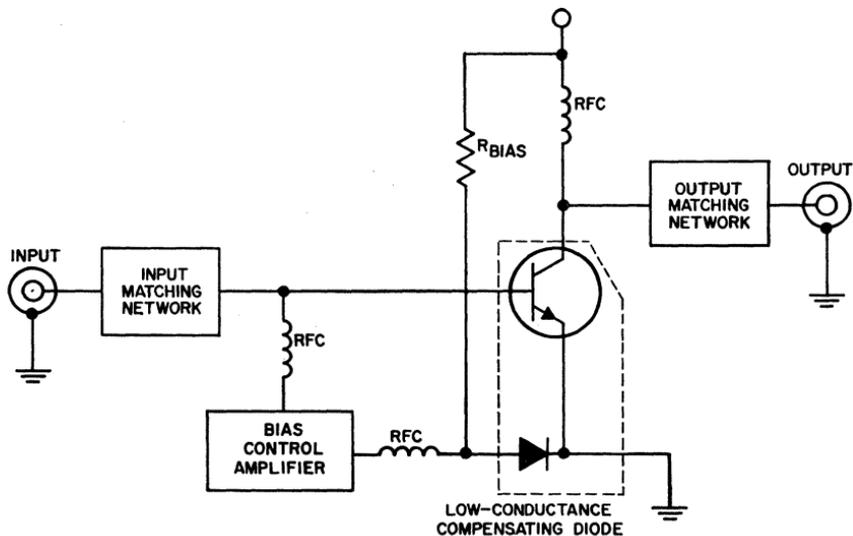
Figure 336. Block diagram of 30-MHz amplifier that uses a low-conductance diode for temperature compensation.
