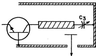
Figure 316. Capacitive-probe-coupled output cavity.
