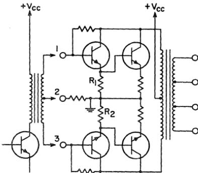
Figure 420. Class AB, push-pull, transformer-coupled audio output stage in which Darlington pairs are used to reduce drive requirements of output transistors.
