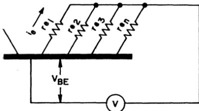
Figure 332. Schematic representation of the separate emitter sites in an "overlay" transistor with a resistor connected in series with each site.
