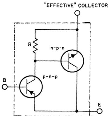
Figure 426. Connection of p-n-p driver transistor to n-p-n output transistor.
