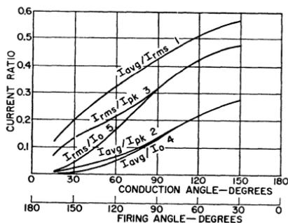
Figure 251. Ratio of SCR current as a function of conduction and firing angles for three-phase half-wave circuit having a resistive load.
