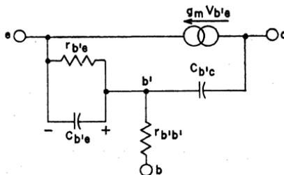
Figure 138. Hybrid-pi equivalent circuit for a transistor used in a common-base configuration (effects of base-width modulation are neglected).
