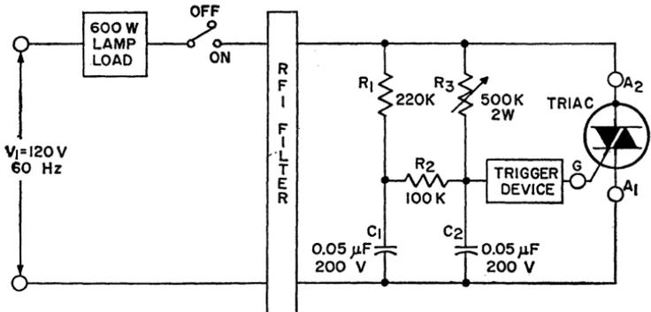
Figure 290. Double-time-constant phase-control circuit for brightness control of incandescent lamps in which a small amount of triac current flows when potentiometer is set for maximum resistance.
