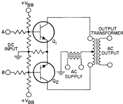
Figure 475. Phase-sensitive linear servo amplifier that develops an ac output for a dc input.
