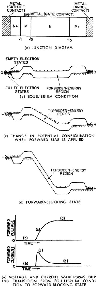
(e) VOLTAGE AND CURRENT WAVEFORMS DURING TRANSITION FROM EQUILIBRIUM CONDITION TO FORWARD-BLOCKING STATE
