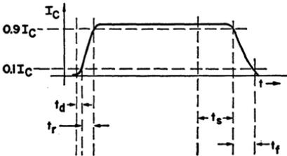
Figure 161. Collector-current waveform that results from change in conducting state of a power transistor.
