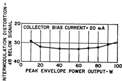
Figure 331. Typical intermodulation distortion in an RCA developmental transistor at various output power levels.
