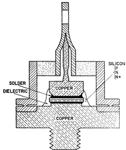
Figure 17. Cross-sectional diagram of a typical silicon rectifier.
