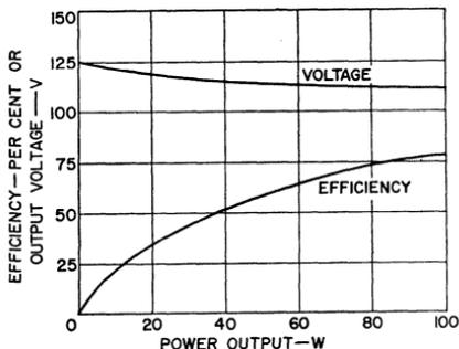
Figure 208. Output voltage and efficiency as a function of power output for the converter circuit shown in Fig. 207.
