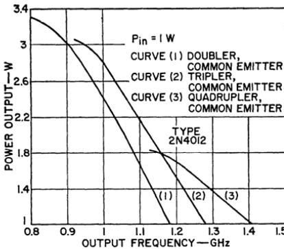
Figure 399. Power output of the RCA-2N4012 overlay transistor as a function of frequency when operated in common-emitter doubler, tripler and quadrupler circuits.
