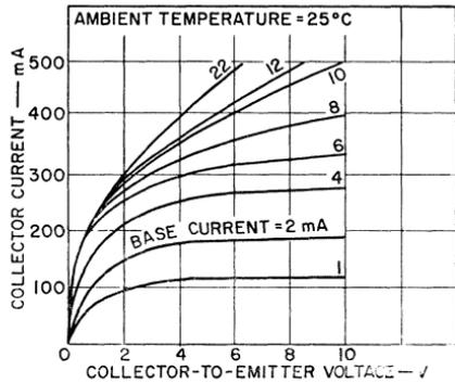
Figure 155. Typical output characteristics for the 2N3053 silicon power transistor.
