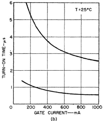
Figure 60. Turn-on time distribution among RCA SCR's: (a) low-current types, (b) high-current types.
