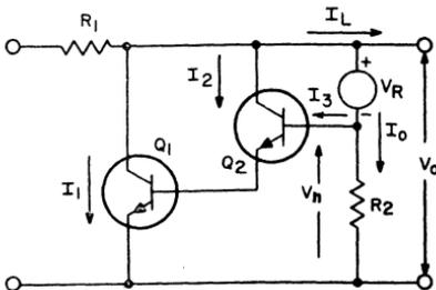
Figure 237. Shunt regulator circuit using two transistors as the shunt pass element.
