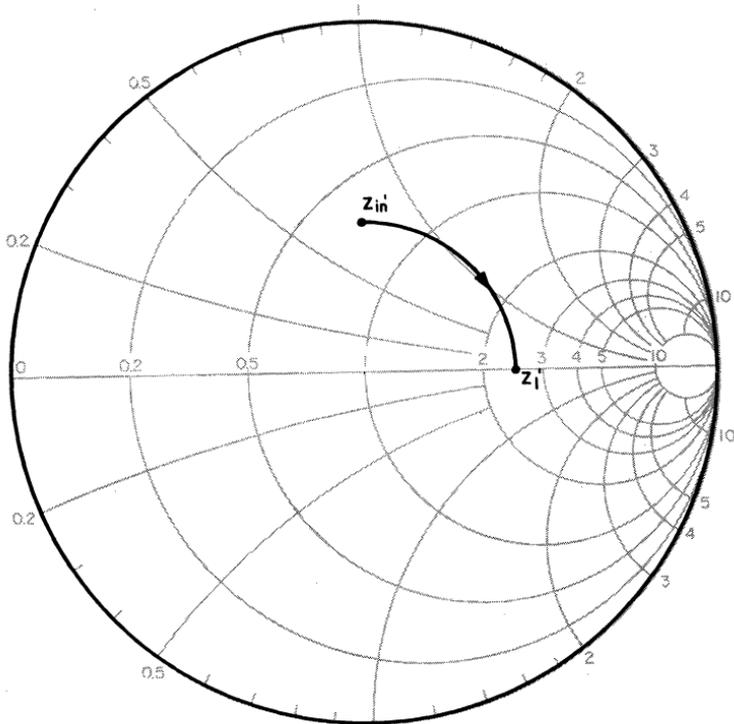
Figure 319. Smith-chart admittance plot used for design of input transmission-line matching sections.
