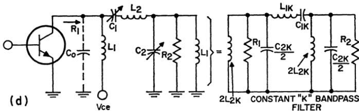
LET  $C_{2K} = 2 C_{OUT}; R_1 = R_2; f_1 = \text{LOW FREQ. CUTOFF}; f_2 = \text{HI-FREQ. CUTOFF}$
