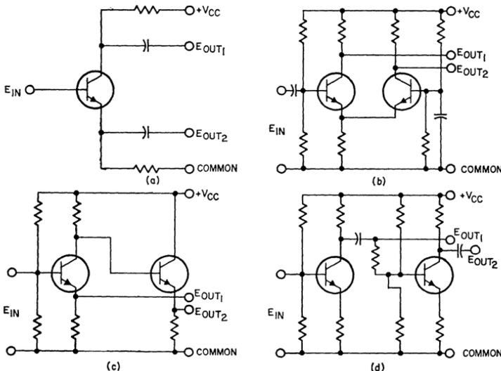
Figure 417. Basic phase-inverter circuits: (a) single stage phase-splitter type (b) two-stage emitter coupled type; (c) two-stage low impedance type; (d) two-stage similar-amplifier type.
