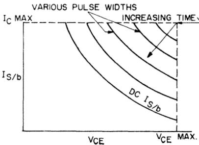
Figure 100. Variation in forward-bias second-breakdown energy level as a function of pulse width.
