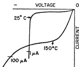
Figure 19. Typical reverse characteristics of a silicon rectifier.
