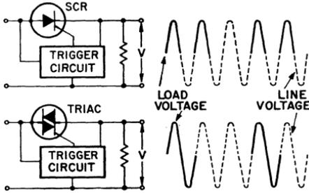
Figure 246. Integral-cycle thyristor power control circuits.
