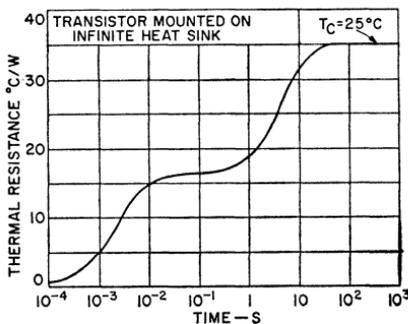
Figure 87. Graphical representation of transient thermal resistance curve.
