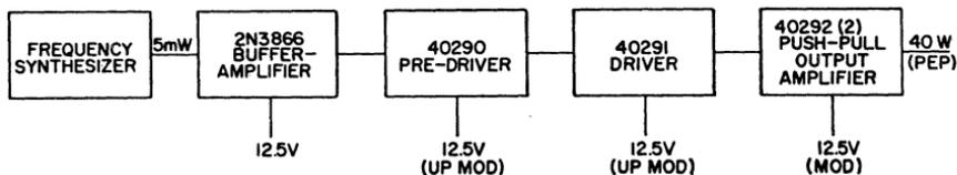
Figure 343. Block diagram of broadband 118-to-136-MHz Aircraft Transmitter.
