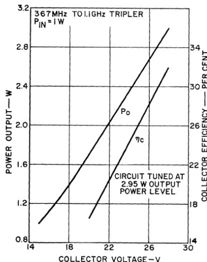
Figure 405. Power output as a function of collector supply voltage for the 367-MHz-to-1.1-GHz frequency tripler.
