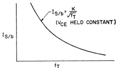
Figure 98. Variation in forward-bias second-breakdown energy level as a function of transistor frequency capability.
