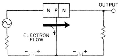
Figure 9. N-P-N structure biased for power gain.
