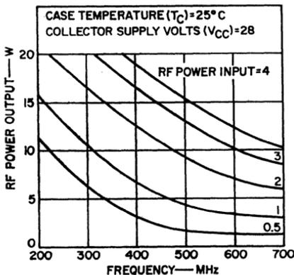
Figure 374. Typical power output as a function of frequency.
