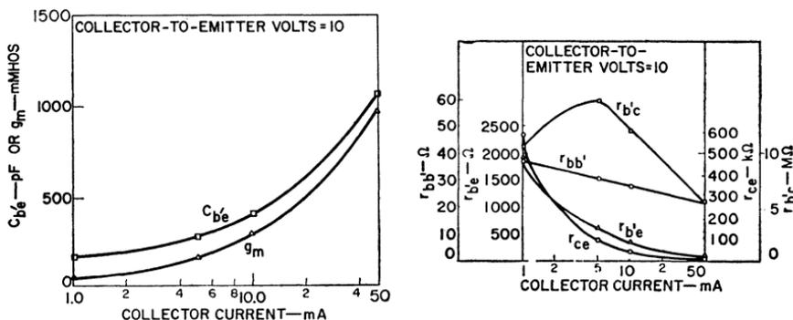
Figure 148. Hybrid-pi parameters as a function of collector current for the 2N2102 silicon power transistor.
