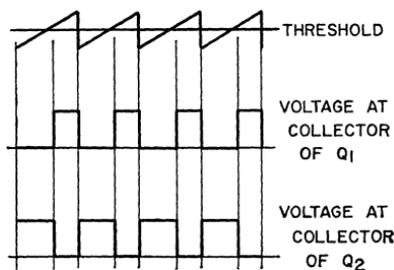
Figure 480. Waveforms showing the threshold switching control for the control amplifier shown in Fig. 479.
