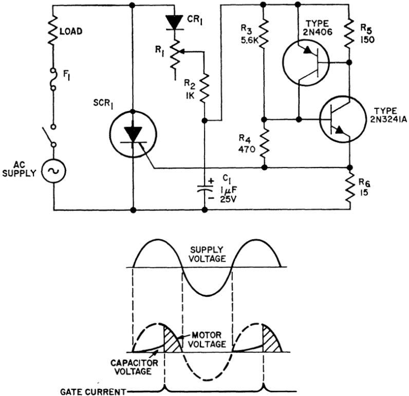
Figure 272. Half-wave SCR motor control circuit, without regulation.
