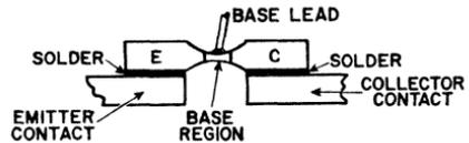
Figure 66. Cross-section of grown-junction transistor.
