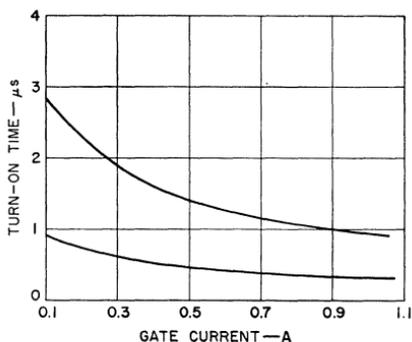
Figure 49. Turn-on time characteristics for the RCA-2N3873 SCR.
