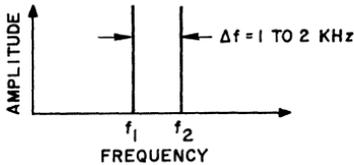
Figure 329. Frequency spectrum for a typical two-tone signal without distortion.
