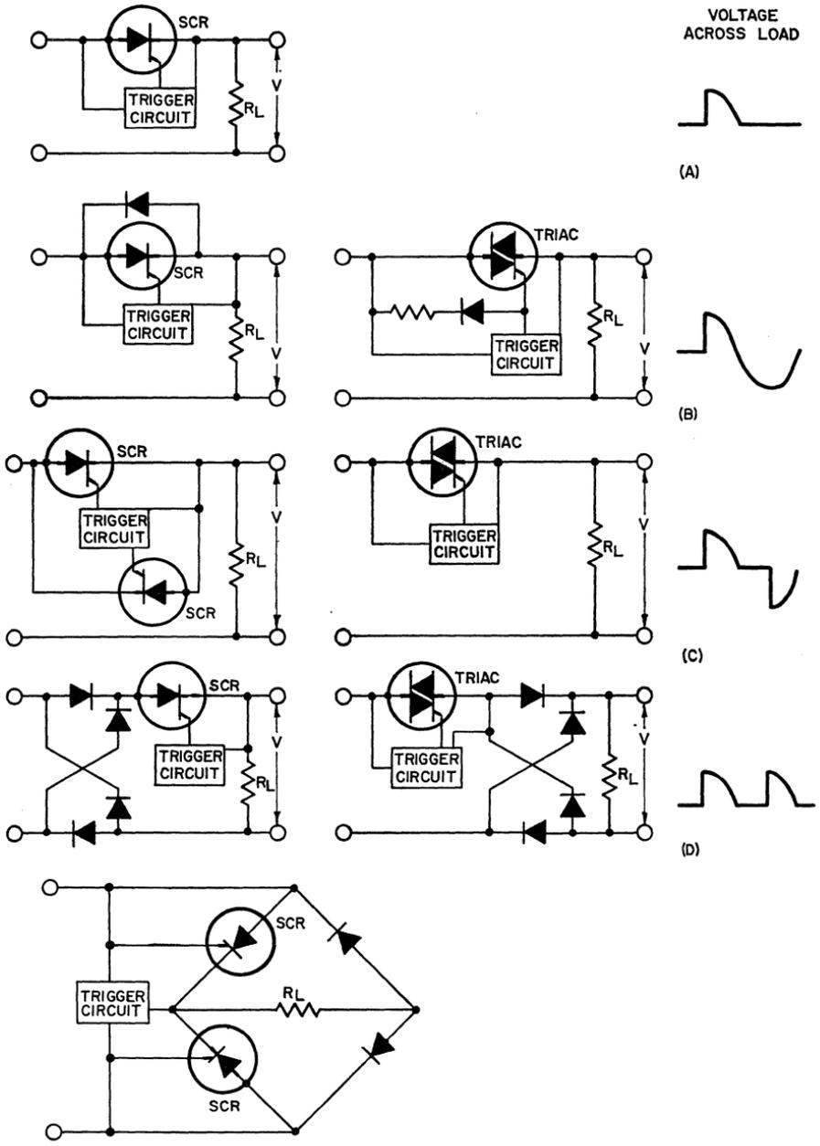
Figure 248. Basic circuit configurations for thyristor power controls and voltage waveform across the load for two complete cycles of operation.
