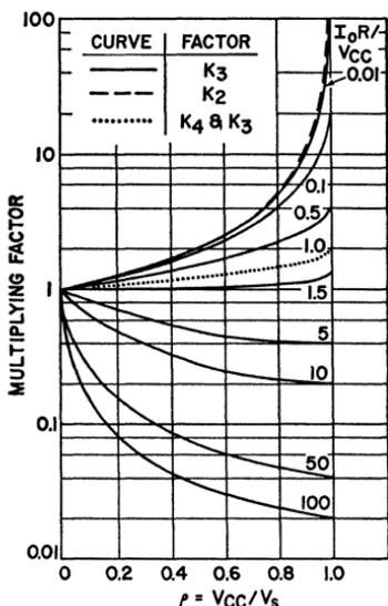
Figure 173. Multiplying factors ( $k_2$ ,  $k_3$ ,  $k_4$ ) as a function of the ratio  $V_{CC}/V_s$ .
