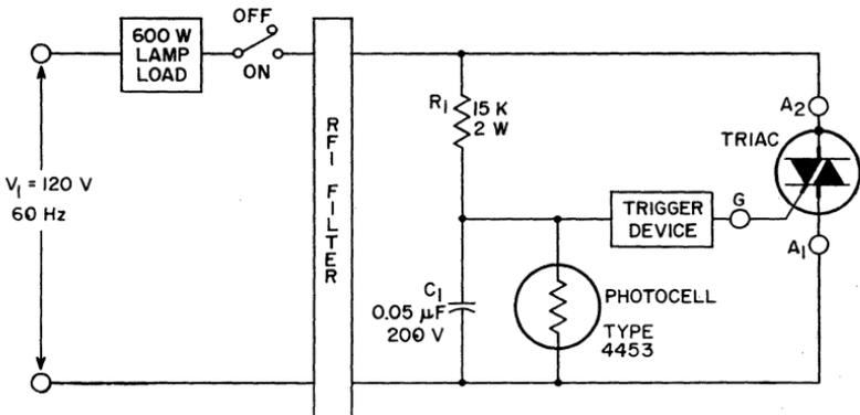
Figure 294. Photocell-operated lamp control circuit that energizes lamp load when photocell is not illuminated.
