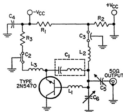
$C_1 = 0.82 \text{ pF}$ , "gimmick" capacitor (manufactured by Quality Components, Inc. St. Mary's, Pa.)
