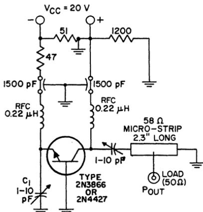
Figure 364. 1-watt, 500-MHz microstripline oscillator using the RCA 2N3866 or 2N4427 transistor.
