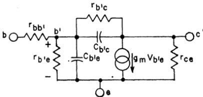
Figure 128 Conventional form of the complete hybrid-pi equivalent circuit shown in Fig. 125.
