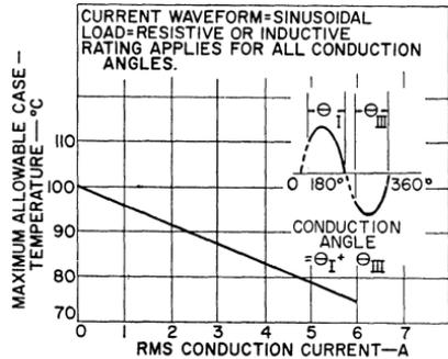
Figure 41. Current rating curve for a typical RCA triac.
