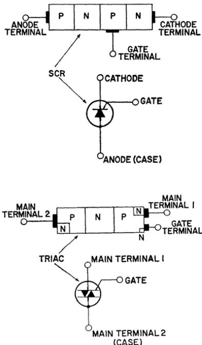
Figure 12. Junction diagrams and schematic symbols for SCR's and triacs.
