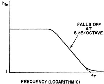
Figure 79. Transistor current-gain parameter  $h_{fe}$  as a function of frequency.
