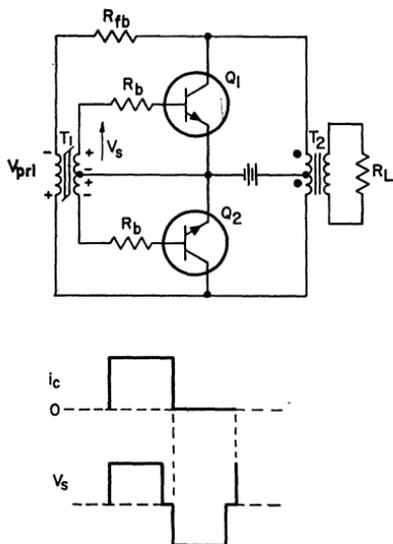
Figure 209. Two-transistor, two-transformer push-pull switching converter.
