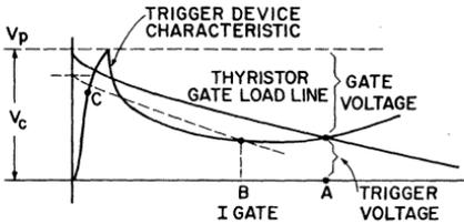
Figure 261. Load line for the circuit shown in Fig. 258.
