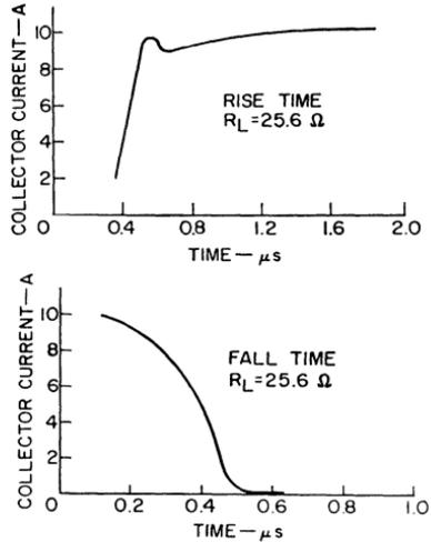
Figure 217. Collector-current rise and fall times.
