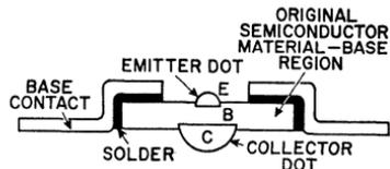
Figure 67. Cross-section of alloy-junction transistor.
