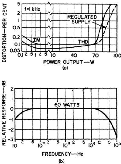
Figure 452. Performance curves for the 70-watt quasi-complementary-symmetry audio amplifier: (a) distortion as a function of power output; (b) relative response as a function of frequency. (These curves are representative of the performance provided by the universal quasi-complementary-symmetry design.)
