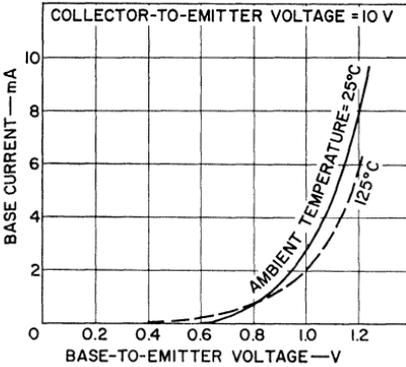
Figure 154. Typical input characteristics for the 2N3053 silicon power transistor.
