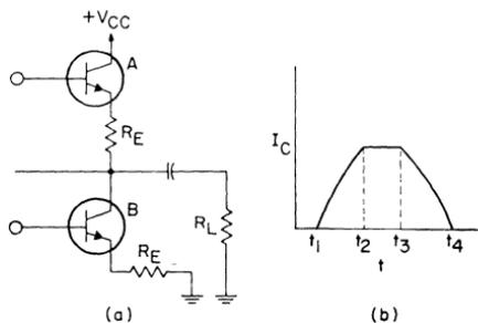
Figure 443. (a) Class B series-output stage, (b) collector-current waveform under overdrive (clipping) conditions.
