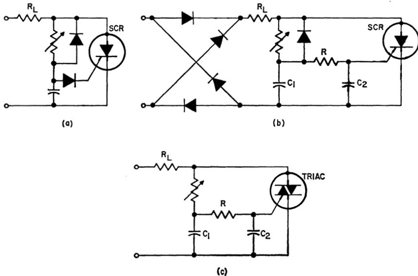
Figure 257. RC triggering networks used for phase-control triggering of thyristors: (a) series RC network and diode (for SCR); (b) RC lattice network and diode (for SCR); (c) RC lattice network without diode (for triac).
