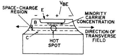
Figure 101. Cross-section of power transistor under reverse-bias conditions.
