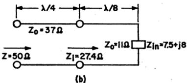
Figure 318. Input and output transmission lines with transmission-line matching sections added to provide required impedance transformation: (a) output line; (b) input line using series matching section; (c) input line using series matching section foreshortened by reactive elements.
