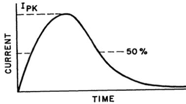
Figure 262. Typical gate-current waveform for circuit shown in Fig. 258.
