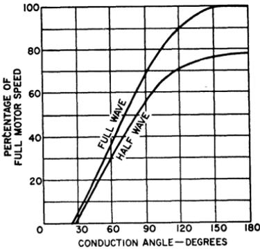
Figure 275. Typical performance curves for a universal motor with phase-angle control.
