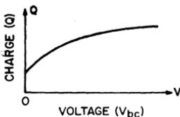
Figure 394. The charge  $Q$  in the collector-to-base junction as a function of collector-to-base voltage in an overlay transistor.
