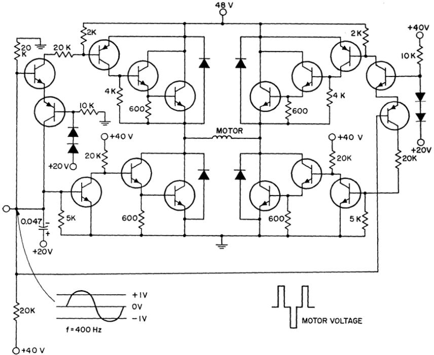
Figure 476. Pulse-width-modulated servo-motor-driver output stage.
