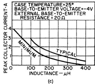
Figure 120. Reverse-bias energy of the RCA 2N3585 transistor.
