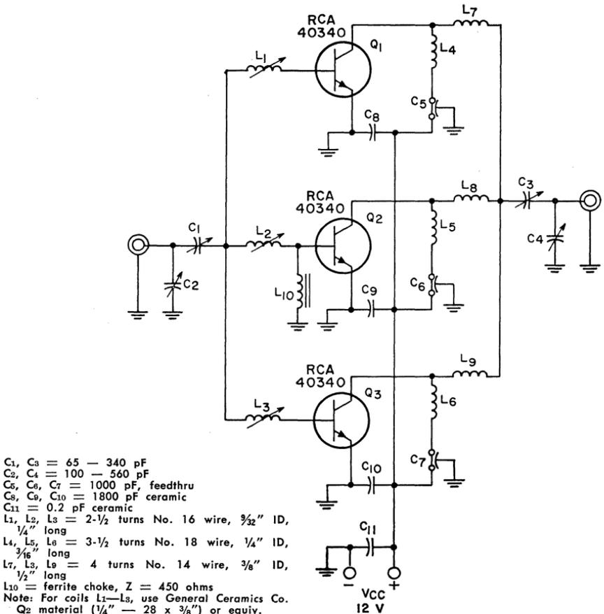
Figure 325. 50-MHz parallel-transistor power amplifier that delivers 50 watts of output power from a 12-volt dc supply.
