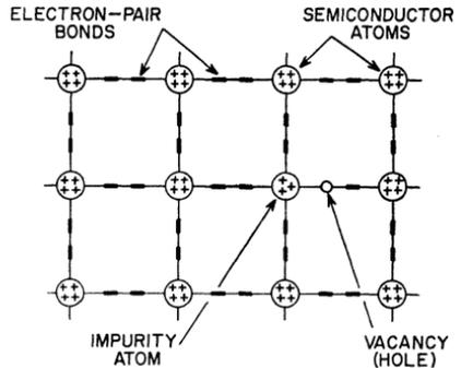
Figure 4. Lattice structure of p-type material.
