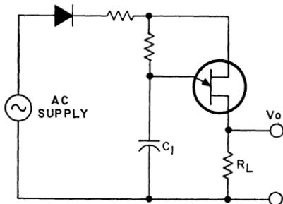
Figure 268. Pulse-triggering circuit that uses a unijunction transistor.
