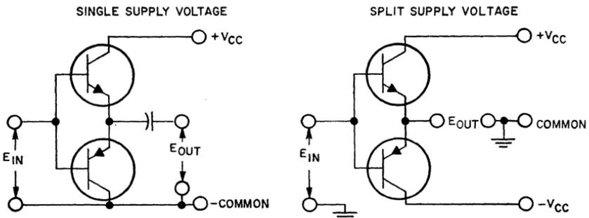
Figure 415. Circuit arrangements for operation of complementary output stages (a) from single dc supply; (b) from symmetrical dual (positive and negative) supplies.
