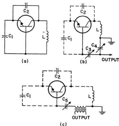
Figure 385. Colpitts oscillator for use at microwave frequencies: (a) basic ac circuit configuration; (b) basic ac circuit with collector returned to ground through parasitic inductance  $L$  and the output taken from base through capacitive voltage divider; (c) basic ac circuit with transformer coupled output.
