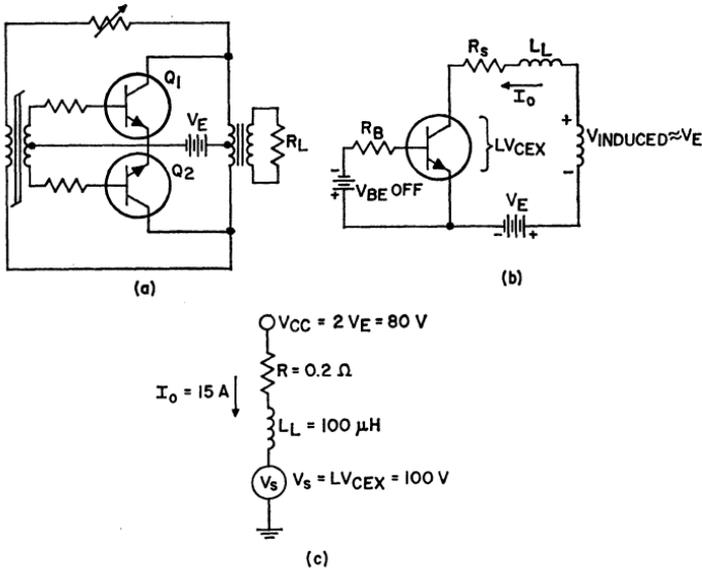
Figure 178. Typical power inverter circuit and equivalent circuits used in Example 4 as an application of case-3 equations.
