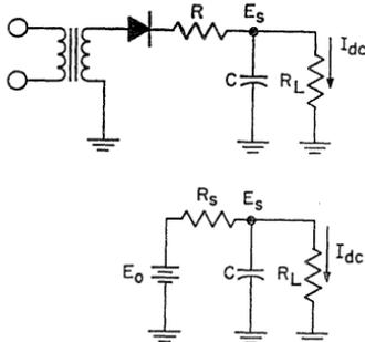
Figure 433. Equivalent circuit for single-ended capacitive-input rectifier supply.
