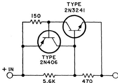
Figure 270. Two-transistor switch. Characteristics of this circuit are similar to those of a trigger diode.
