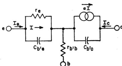
Figure 139. "T" equivalent circuit for a transistor used in a common-base configuration when the effects of base-width modulation are neglected.
