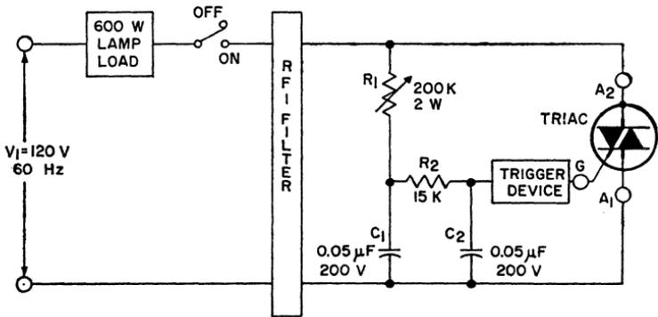
Figure 289. Double-time-constant circuit for brightness control of incandescent lamps in which triac is cut off when potentiometer is set for maximum resistance.
