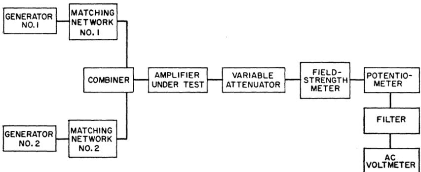
Figure 355. Block diagram of cross-modulation test setup in which a field-strength meter is used.
