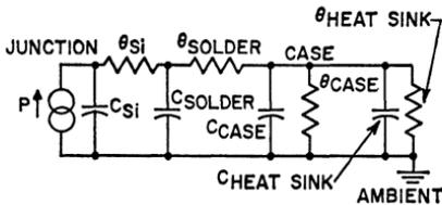
Figure 88. Thermal equivalent circuit for a transistor mounted on a heat sink.
