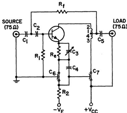
$C_1, C_2, C_5 = 0.002 \mu\text{F}$
