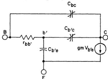
Figure 297. Simplified high-frequency equivalent circuit for an "overlay" transistor.
