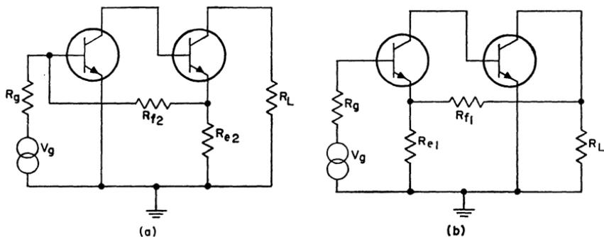
Figure 351. Two-stage wide-band rf amplifiers that use a combination of voltage and current feedback to increase circuit bandwidth: (a) Feedback is coupled from emitter of output transistor (low-impedance point) to base of input transistor (higher impedance point); (b) feedback is coupled from collector of output transistor (high-impedance point) to emitter of input transistor (low-impedance point).
