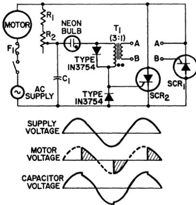
Figure 279. Full-wave SCR motor control circuit, without regulation.
