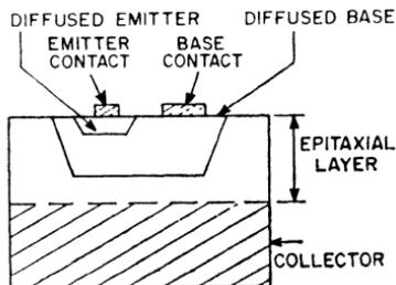
Figure 81. Structure of double-diffused epitaxial planar transistor.
