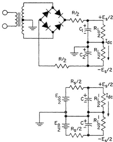
Figure 434. Equivalent circuit for split capacitive-input rectifier supply.
