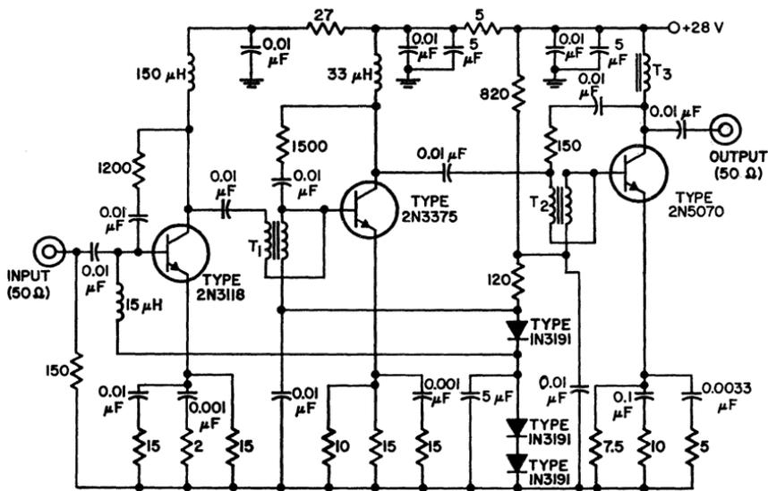
T<sub>1</sub>, T<sub>2</sub> = 18 turns twisted pair. No. 28 enamel wire on Q<sub>1</sub> CF 102 form      T<sub>3</sub> = 50 turns No. 30 enamel wire on CF 102 Q<sub>1</sub> form
