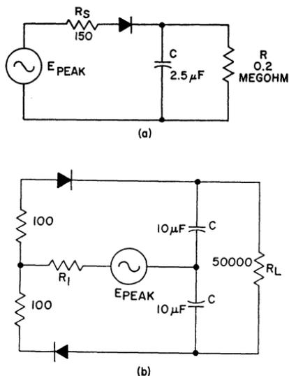
Figure 188. Typical rectifier circuits using capacitive loads: (a) half-wave rectifier circuit; (b) voltage doubler.
