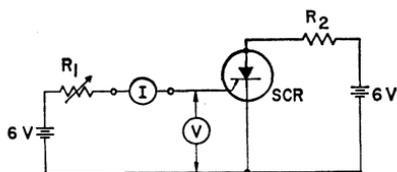
Figure 56. Test circuit used to determine gate-trigger-pulse requirements of thyristors.
