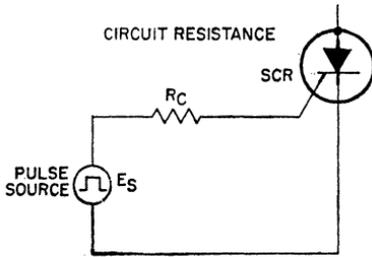
Figure 59. Equivalent diagram of the basic gate-trigger circuit for a thyristor.
