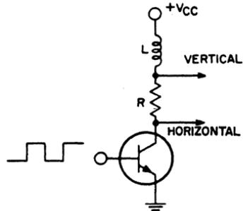
Figure 168. Test circuit used to determine transistor load lines.
