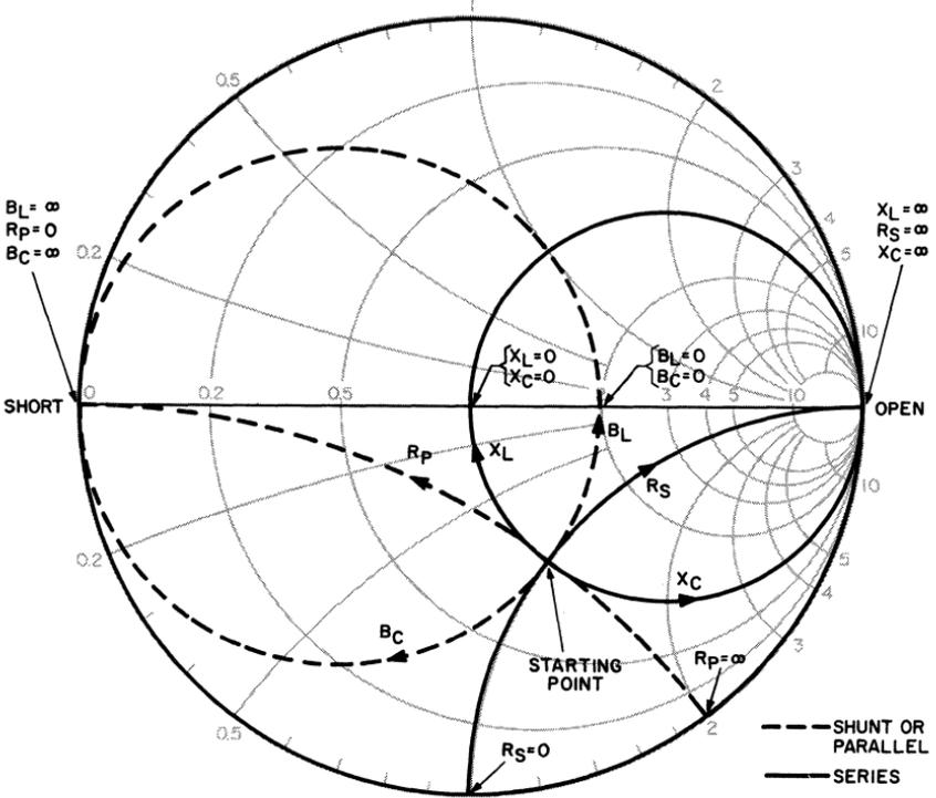
Figure 306. Method used to trace constant-parameter curves for matching-network components.
