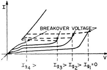
Figure 28. Curves showing breakover characteristics of a thyristor for different values of gate current.
