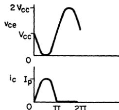
Figure 470. Collector voltage and current waveforms for an oscillator circuit that has a conduction angle of 180 degrees.
