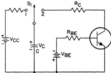
Figure 108. Capacitive-discharge test circuit used to determine reverse-bias second-breakdown energy levels in transistors.
