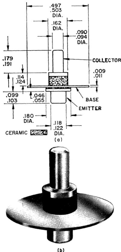
Figure 376. RCA-2N5470 coaxial transistor (a) outline; (b) external view.
