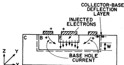
Figure 147. Model of n-p-n transistor showing transverse base field and current-crowding effect.
