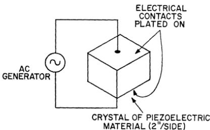
Figure 461. Application of an alternating voltage to a piezoelectric crystal to produce high-frequency sound waves.
