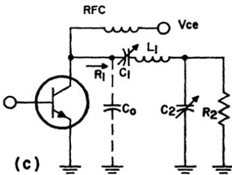
(1)  $X_{C1} = \frac{Q_L X_{C0}^2}{R_1} \left[ 1 - \frac{R_1}{Q_L X_{C0}} \right]$
