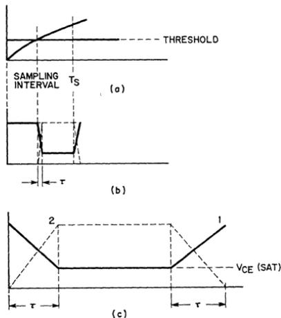
Figure 481. Approximate switching waveforms of the output transistors in the control amplifier shown in Fig. 479.
