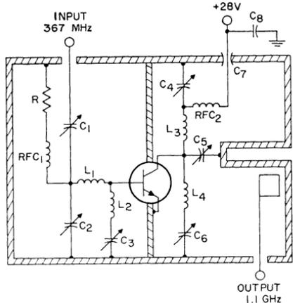
Figure 403. 367-MHz-to-1.1-GHz common-emitter transistor frequency tripler.
