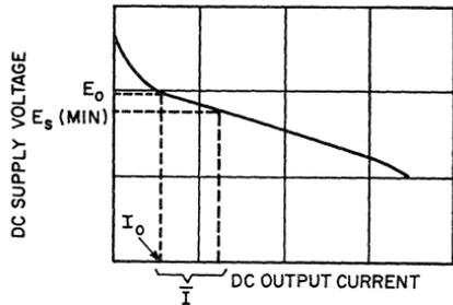
Figure 439. Power-supply regulation curve.
