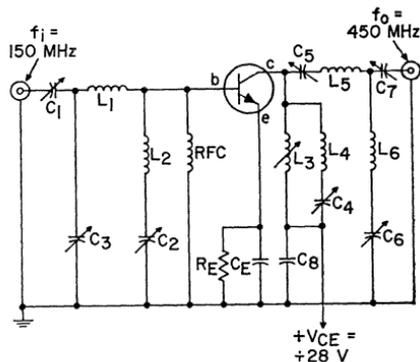
Figure 406. 150-to-450-MHz common-emitter transistor frequency tripler.
