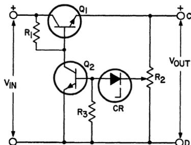
Figure 226. Series voltage regulator without current limiting.
