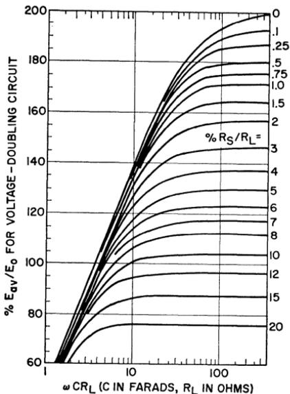
Figure 195. Relationship of applied ac peak voltage to dc output voltage in capacitor-input voltage-doubler circuit.
