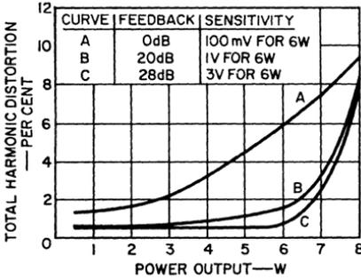
Figure 455. Total harmonic distortion (at 1 kHz) of the bridge audio amplifier as a function of power output for different values of balanced loop feedback. (Distortion performance is comparable to that of a single-ended amplifier that provides one-quarter of the power output for the same dc supply voltage.)
