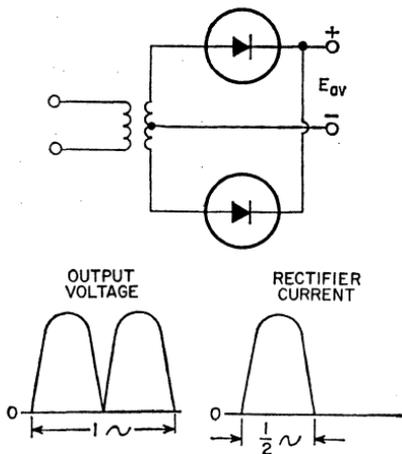
Figure 180. Single-phase full-wave circuit with center-tapped power transformer.
