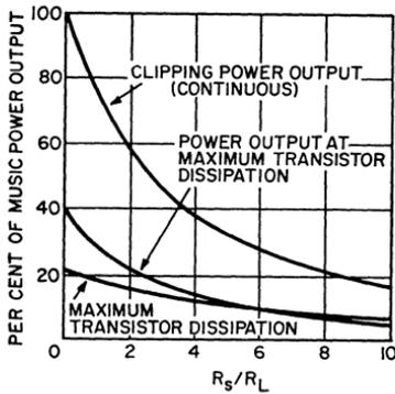
Figure 437. Power output and dissipation as functions of  $R_s$  and  $R_L$ .
