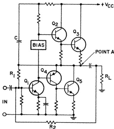
Figure 429. Quasi-complementary audio power amplifier that operates from a single dc supply.
