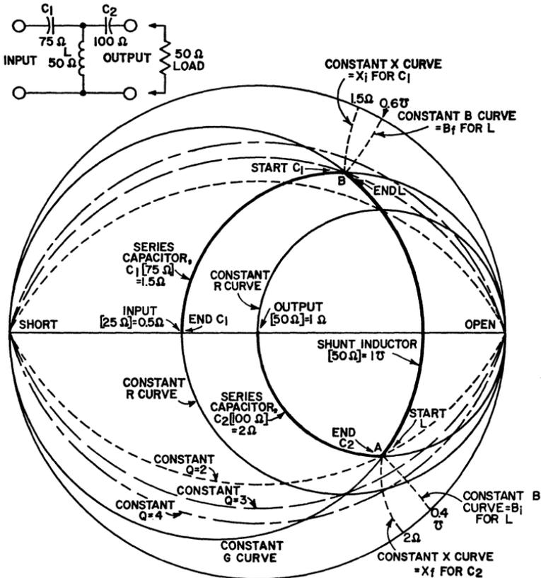
Figure 310. Typical output matching network and network map used to determine required input impedance for this network.
