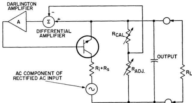
Figure 232. AC feedback circuit for a voltage-regulated power supply.
