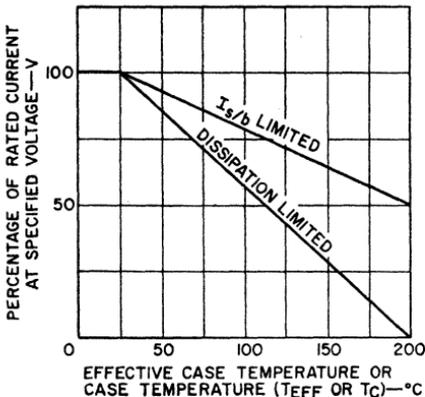
Figure 119. Temperature derating for the RCA 40411 transistor.
