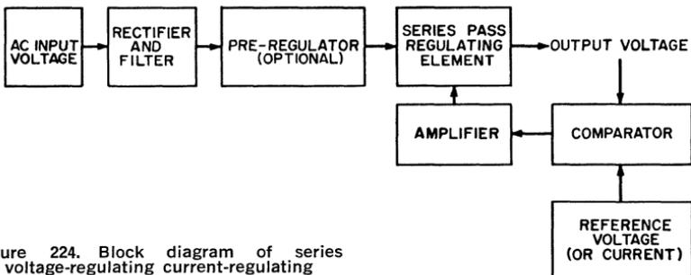
Figure 224. Block diagram of series voltage-regulating current-regulating dc power supply.
