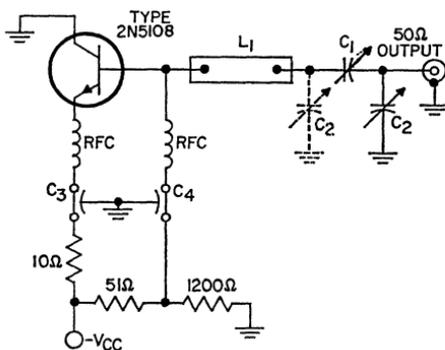
$C_1, C_2$  = Variable capacitor, 0.35 to 3.5 pF, piston type
