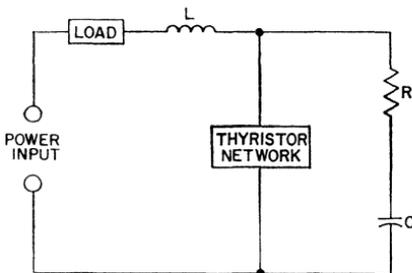
Figure 64. Diagram showing use of RC network for transient suppression and an inductance to prevent false turn-on because of transients in thyristor circuits.
