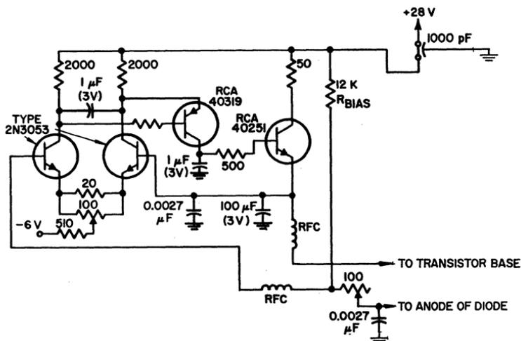
Figure 337. Linear 30-MHz amplifier with temperature-compensating circuit.
