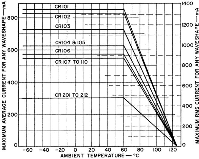
Figure 198. Current-temperature ratings for silicon stack rectifiers.
