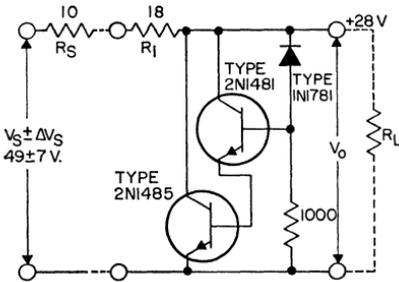
Figure 238. Schematic diagram of 28-volt shunt regulator circuit.
