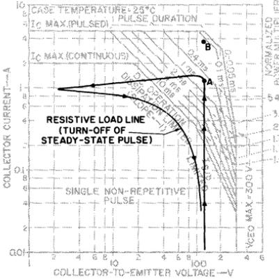
Figure 115. Inverter turn-on load line on 2N3585 safe-area curve.
