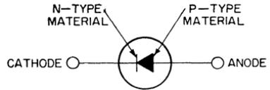
Figure 10. Schematic symbol for a semiconductor diode.
