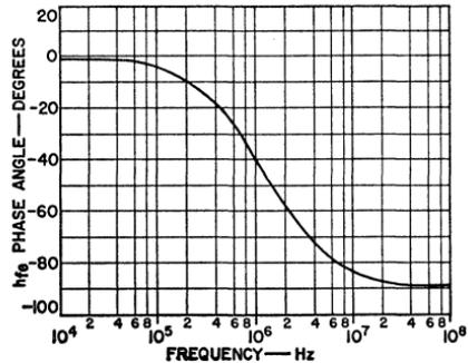
Figure 144. Phase of  $h_{fe}$  as a function of frequency for the 2N2102 silicon power transistor.
