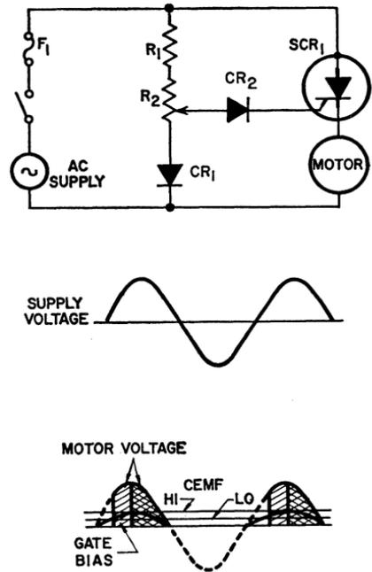
Figure 276. Half-wave SCR motor control circuit, with regulation.
