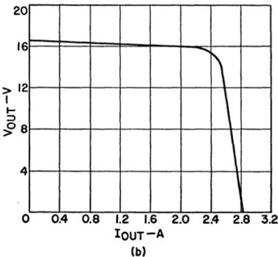
Figure 229. Series voltage regulator which uses additional transistor-diode network and series pass transistor to accomplish current-limiting function: (a) schematic diagram; (b) response characteristics.
