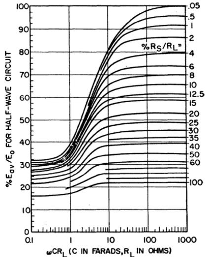
Figure 194. Relationship of applied ac peak voltage to dc output voltage in half-wave capacitor-input circuit.
