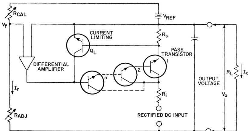
Figure 231. Voltage-regulated current-limited power supply.
