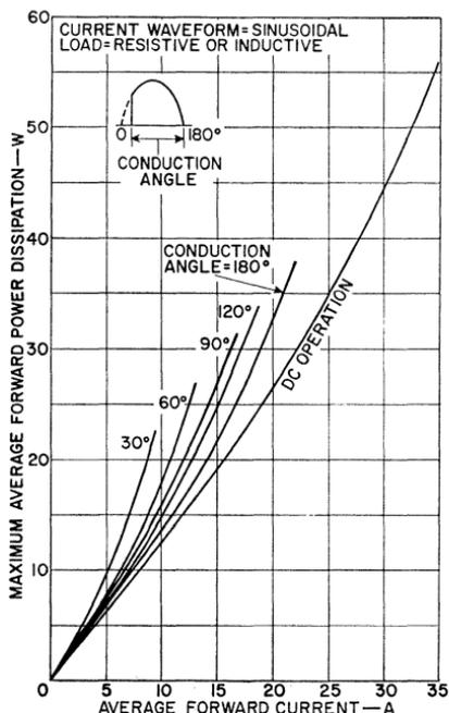
Figure 39. Power-dissipation rating chart for the RCA-2N3873 SCR.
