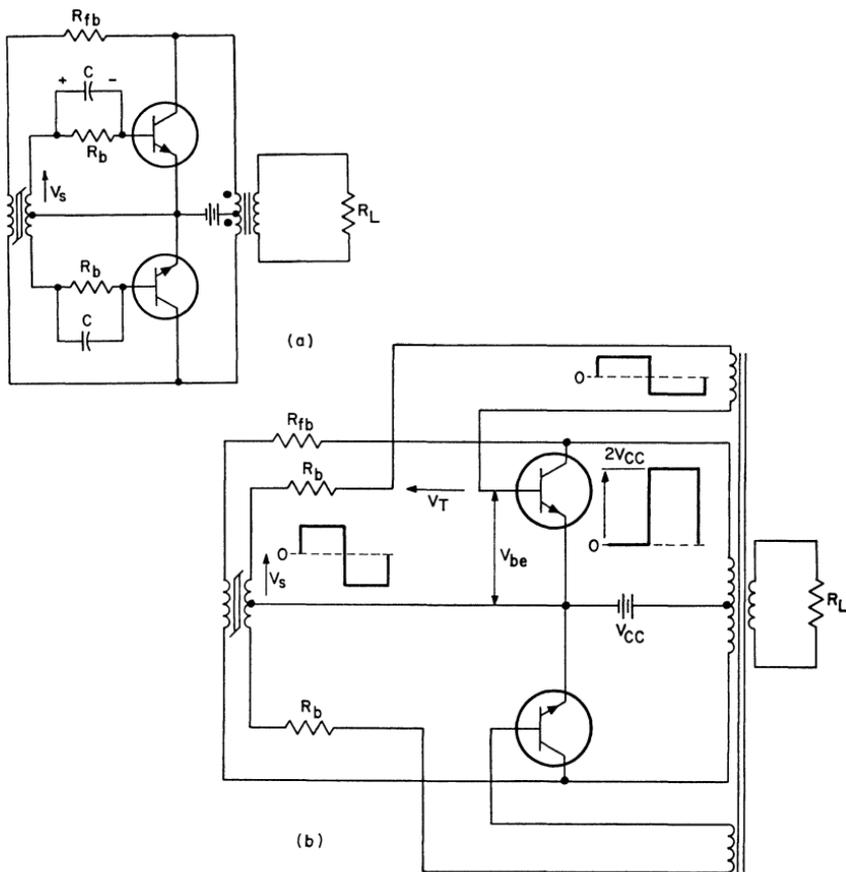
Figure 210. Two-transistor, two-transformer push-pull switching converters in which transistor-storage times are reduced: (a) Capacitor in parallel with each base resistor assures sharp turn-off of associated transistor; (b) Feedback winding from output transformer in series with base of each transistor assures sharp cutoff characteristics.
