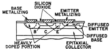
Figure 76. Cross-section of overlay transistor.
