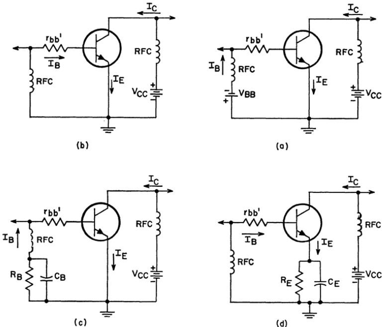
Figure 296. Methods for obtaining class C reverse bias: (a) by use of fixed dc supply  $V_{BB}$ ; (b) by use of dc base current through the base spreading resistance  $r_{bb'}$ ; (c) by use of dc base current through an external base resistance  $R_B$ ; (d) by use of self bias developed across an emitter resistor  $R_E$ .
