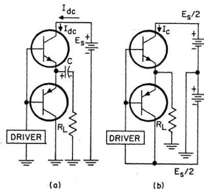
Figure 436. Typical complementary-symmetry circuits.
