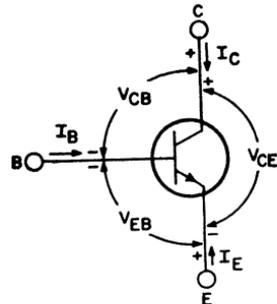
Figure 152. Terminal parameters for an n-p-n transistor.
