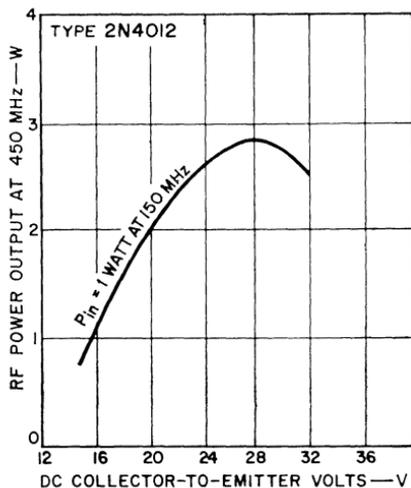
Figure 408. Power output as a function of collector supply voltage for the 150-to-450-MHz frequency tripler.
