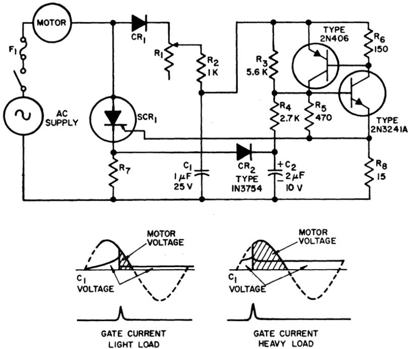
Figure 277. Half-wave SCR motor control circuit using two-transistor regenerative triggering, with regulation.
