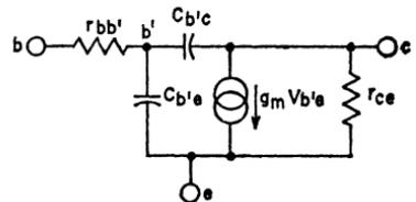
Figure 132. Simplified high-frequency hybrid-pi transistor equivalent circuit.
