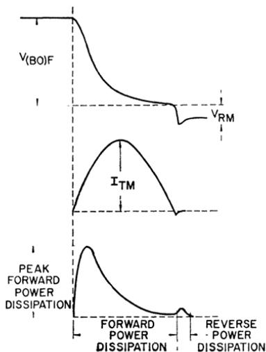
Figure 52. Instantaneous power dissipation in a thyristor during turn-on.
