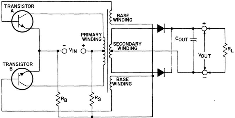
Figure 205. Two-transistor, one-transformer push-pull switching converter.
