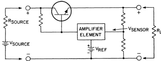
Figure 222. Basic series voltage regulator.
