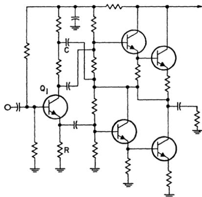
Figure 423. Push-pull series-output amplifier in which driver and output transistors are connected as Darlington pairs and drive-signal phase inversion is provided by phase-splitter stage  $Q_3$ .
