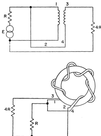
Figure 353. Wideband transformer. This transformer may be used to provide a 4:1 impedance ratio, as indicated in top diagram. The transformer is basically a twisted-pair transmission line wound about a ferrite toroid, as shown in lower diagram.
