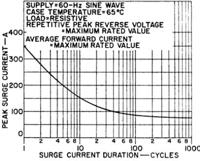
Figure 42. Surge-current rating curve for the RCA-2N3873 SCR.
