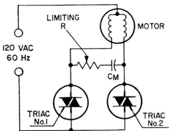
Figure 282. Motor-reversing circuit using two triacs.
