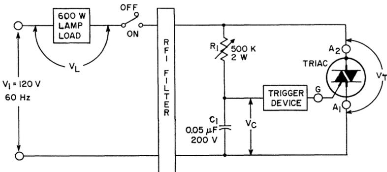
Figure 288. Single-time-constant phase-control circuit for brightness control of incandescent lamps.
