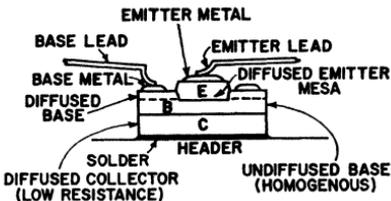
Figure 69. Cross-section of hometaxial-base silicon power transistor.
