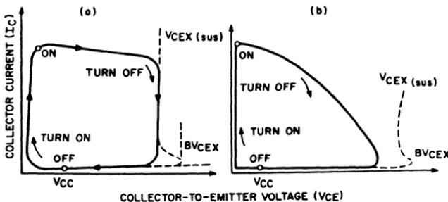
Figure 169. Inductive load line for the test circuit shown in Fig. 168; (a) typical load line; (b) load line when  $L(di/dt) < V_{CEX(sus)}$ .
