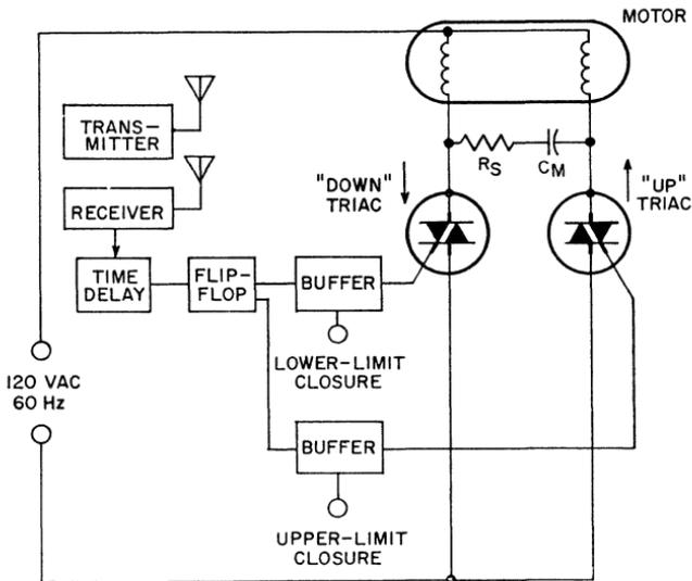
Figure 283. Block diagram of solid-state garage-door system.
