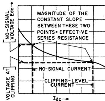
Figure 432. Regulation curve for capacitive rectifier power supply.
