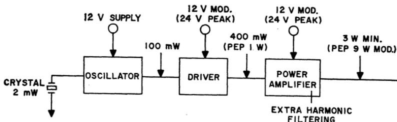
Figure 323. Block diagram of a 5-watt (dc input power to final amplifier) citizens-band transmitter.
