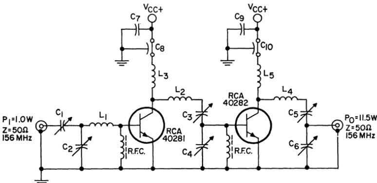
$C_1, C_2, C_3, C_4, C_5, C_6$ , = Arco 404 or equiv.
