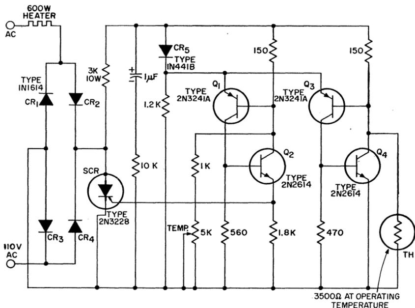
Figure 286. Half-wave SCR heater control circuit.
