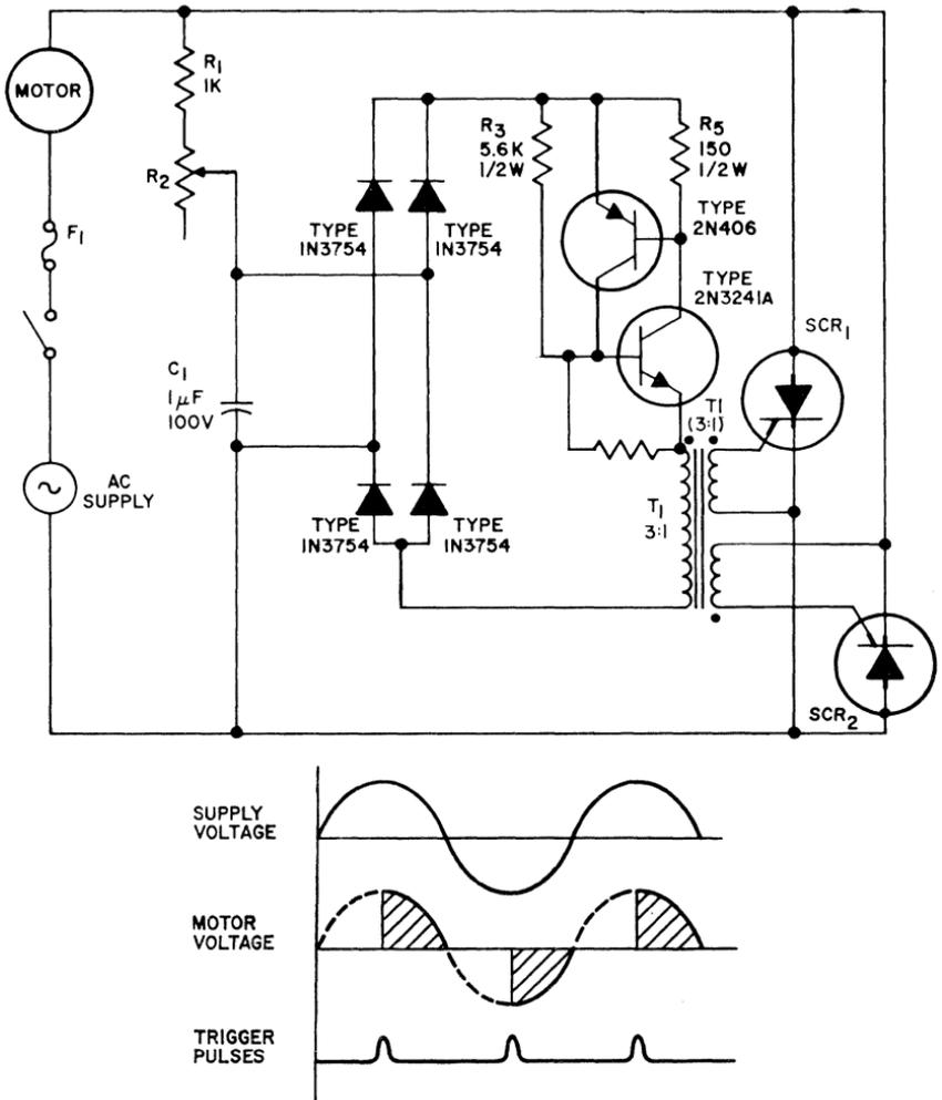
Figure 280. Full-wave SCR motor control circuit, without regulation, in which the conduction angle can be varied from 5 to 170 degrees.
