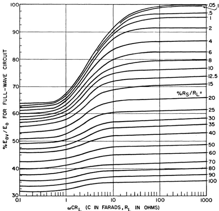
Figure 196. Relationship of applied ac peak voltage to dc output voltage in full-wave capacitor-input circuit.
