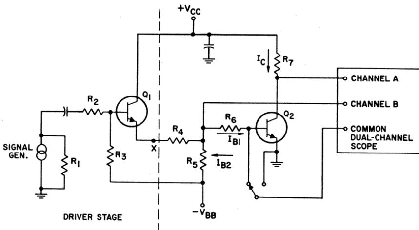
Figure 159. Test circuit used to measure switching times in power transistors.
