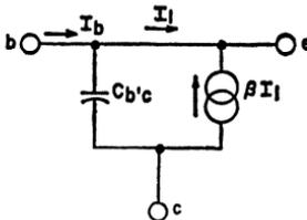
Figure 141. Simplified form of hybrid-pi equivalent circuit shown in Fig. 140.
