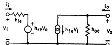
Figure 122. h-parameter equivalent circuit for a transistor used in a common-emitter configuration.
