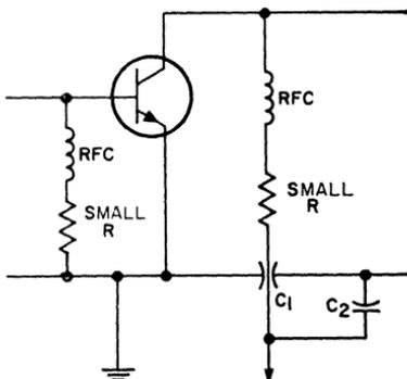
Figure 398. Circuit showing biasing techniques and bypassing capacitances used to eliminate instabilities in common-emitter frequency multipliers.
