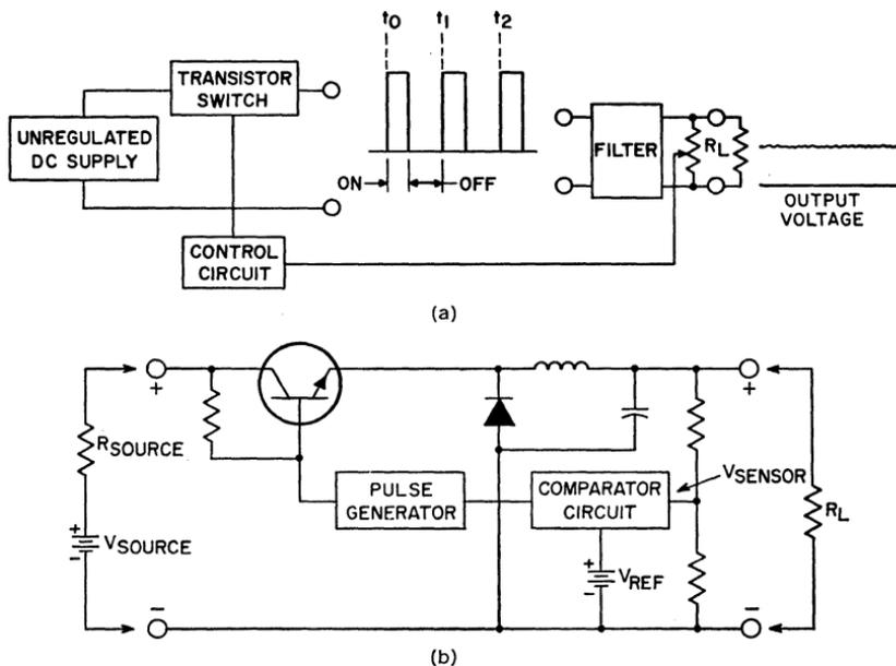
Figure 239. Basic configuration of switching type of transistor voltage regulator: (a) block diagram; (b) schematic diagram.
