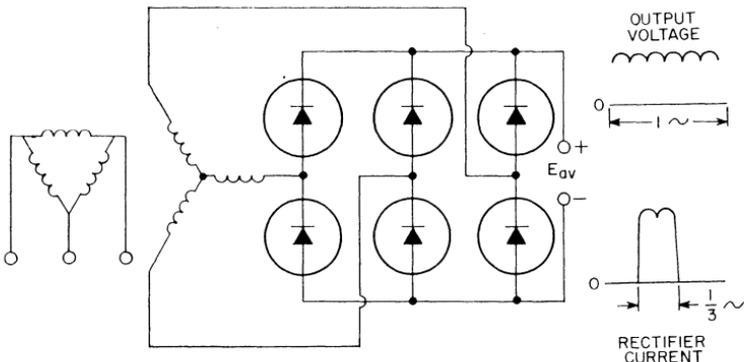
Figure 183. Three-phase "Y" full-wave circuit.
