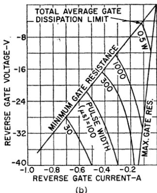
Figure 58. Reverse gate characteristics of RCA SCR's: (a) low-current types, (b) high-current types.
