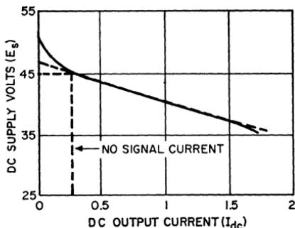
Figure 435. Typical power-supply regulation curve.
