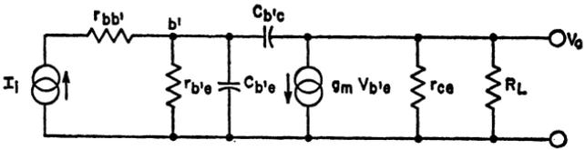
Figure 135. Equivalent circuit for common-emitter amplifier.
