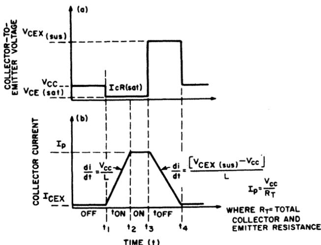
Figure 170. Voltage and current waveforms for the switching circuit shown in Fig. 168.
