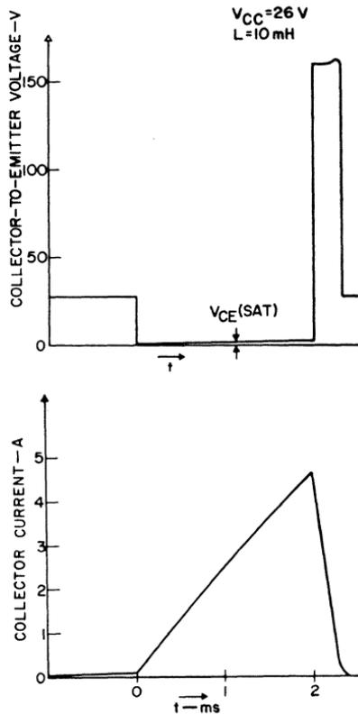
Figure 106. Test waveforms for a 2N3442 transistor subjected to  $E_{S/b}$  inductive energy test.
