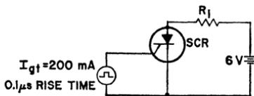
Figure 50. Test circuit used to determine turn-on time of thyristors.
