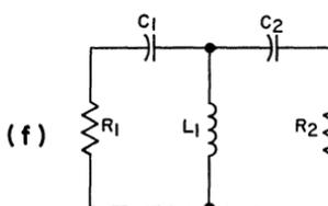
$$(1) X_{C_1} = R_1 \sqrt{\frac{R_2(Q_L^2 + 1)}{R_1}} - 1$$
