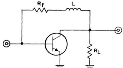
Figure 349. Common-emitter amplifier that uses shunt  $R_L$  feedback to increase circuit bandwidth.
