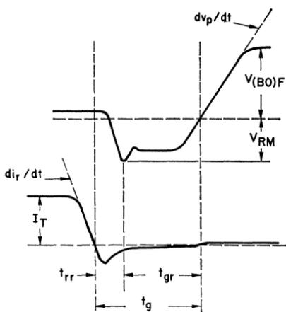
Figure 53. Circuit-commutated turn-off voltage and current waveforms for a thyristor.
