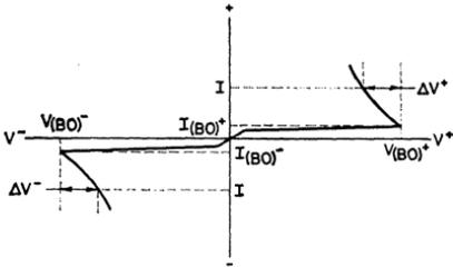
Figure 265. Typical voltage-current characteristic of a bidirectional trigger diac.
