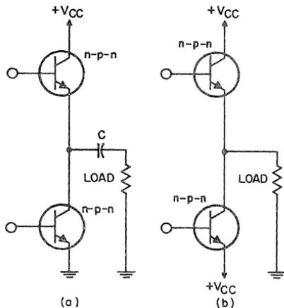
Figure 421. Circuit arrangements for operation of series output circuit from (a) a single dc supply and (b) symmetrical dual supplies.
