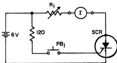
Figure 45. Test circuit used to determine holding and latching currents of thyristors.
