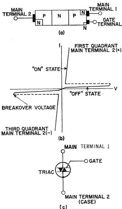
Figure 26. (a) Junction diagram, (b) principal voltage-current characteristic, and (c) schematic symbol for a triac thyristor.
