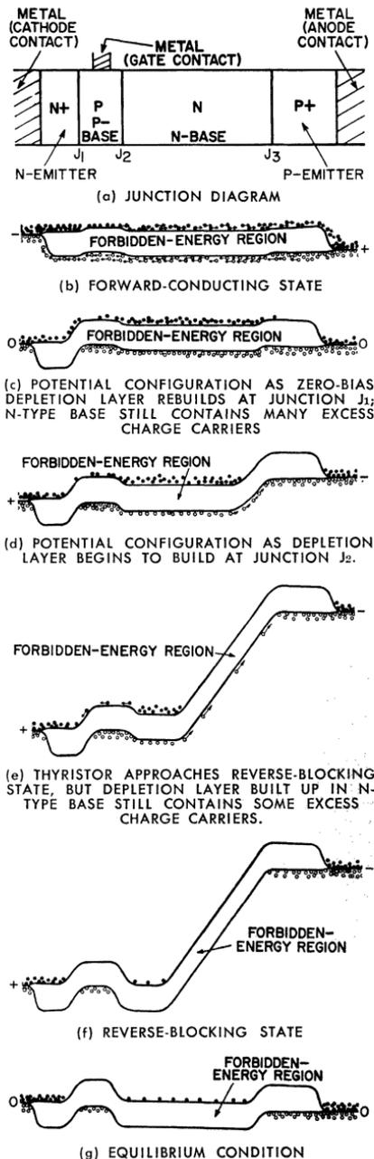
Figure 31. Potential-hill diagrams for various stages of thyristor transition from forward-conducting state to turn-off.
