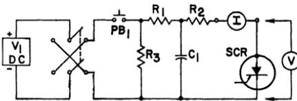
Figure 38. Test circuit used to determine dc forward- and reverse-voltage-blocking capabilities and leakage current of thyristors.
