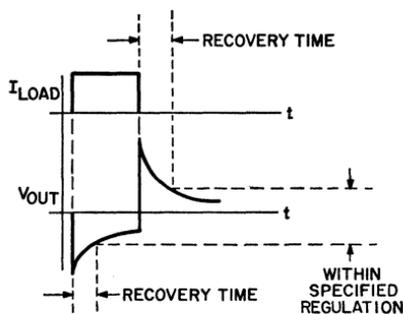
Figure 225. Typical recovery-time characteristics for regulated dc power supplies.
