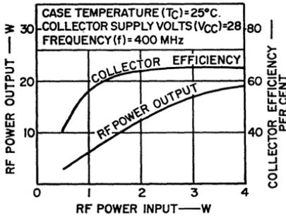
Figure 373. Typical power output or collector efficiency as a function of power input at 400 MHz.
