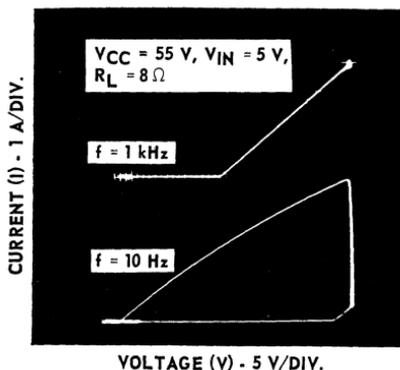
Figure 442. Effect of large signal phase shift on the load-line characteristics of a transistor at low frequencies.
