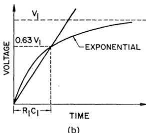
Figure 46. (a) Test circuit and (b) waveforms used to determine  $dv/dt$  capability of a thyristor.
