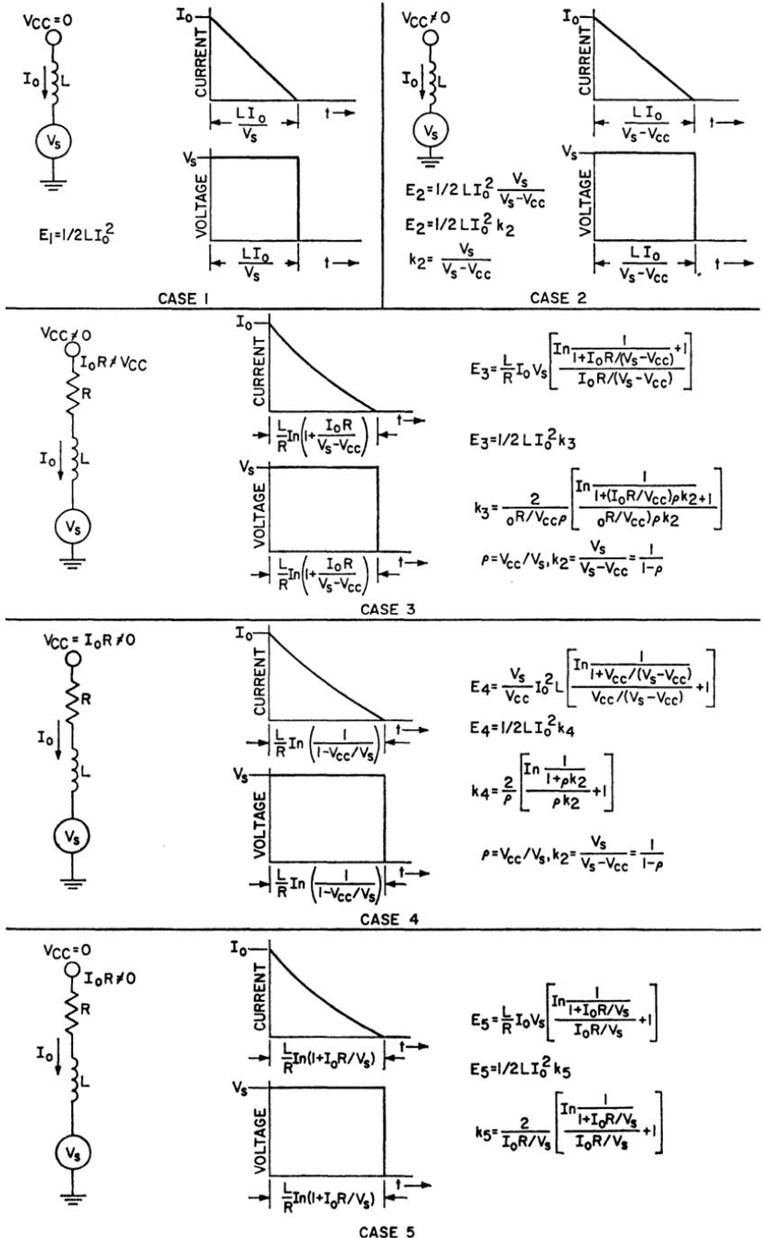
Figure 172. Equivalent circuits, energy equations, and voltage and current waveforms for the five basic circuit configurations.
