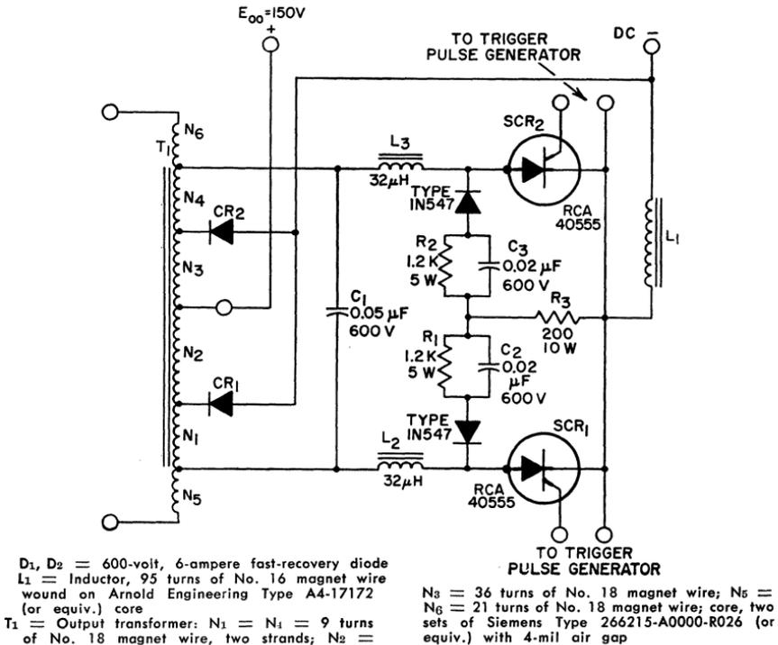
Figure 218. High-frequency (10-kHz) SCR push-pull switching inverter.
