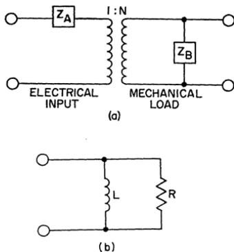
Figure 462. (a) Actual equivalent circuit and (b) simplified approximation of a magnetostrictive transducer.
