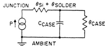
Figure 86. Simplified thermal equivalent circuit for a transistor for  $\theta_{\text{Si}} C_{\text{E}} \ll t < \theta_{\text{case}} C_{\text{case}}$ .
