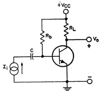
Figure 134. Common-emitter transistor amplifier.
