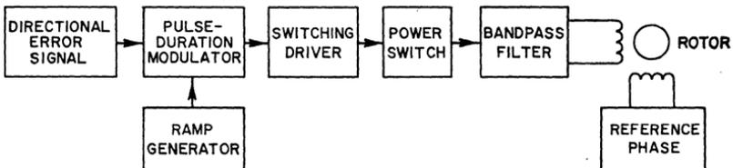
Figure 477. Block diagram of a pulse-duration-modulated switching-servo control system.
