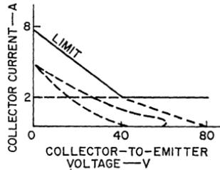
Figure 448. Load lines for the circuit of Fig. 447. Load lines showing effect of the inclusion of high-resistance diode-resistor network in the forward-biasing path of  $Q_1$  are shown dotted.
