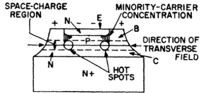
Figure 97. Cross-section of power transistor under forward-bias conditions.
