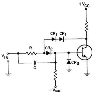
Figure 164. Practical "collector-catcher" circuit.
