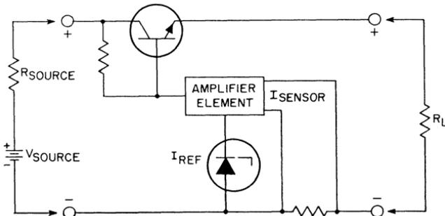
Figure 223. Basic series regulator modified for current sensing.
