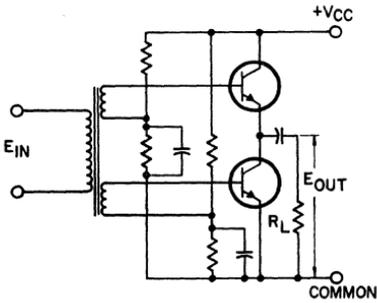
Figure 414. Class AB, push-pull amplifier with series output connection.
