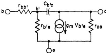
Figure 130. Simplified low-frequency hybrid-pi transistor equivalent circuit.
