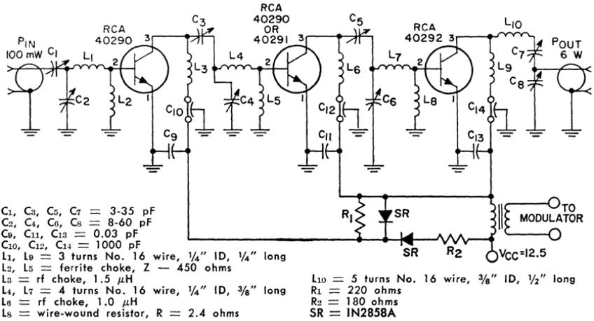
Figure 342. 35-MHz, 6-watt, narrow-band amplitude-modulated transmitter.
