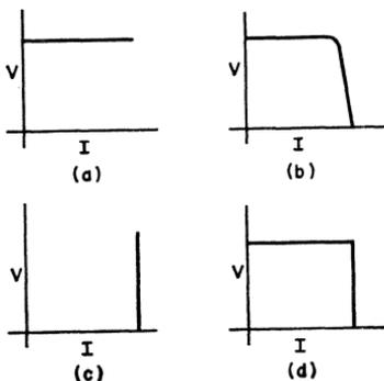
Figure 221. Typical response characteristics for series-regulated power supplies: (a) voltage-regulating types; (b) voltage-regulating current-limiting types; (c) current-regulating types; (d) voltage-regulating current-regulating types.
