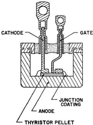
Figure 35. Cross-section of RCA press-fit thyristor package.
