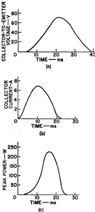
Figure 17. Audio power-amplifier waveforms.
