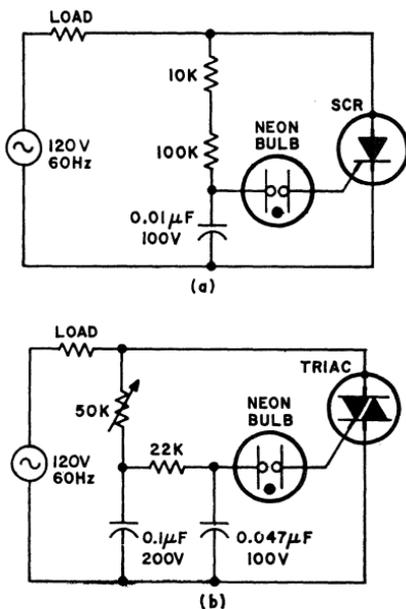
Figure 264. Circuits showing application of neon bulb as thyristor triggering device: (a) SCR power control circuit; (b) triac power control circuit.
