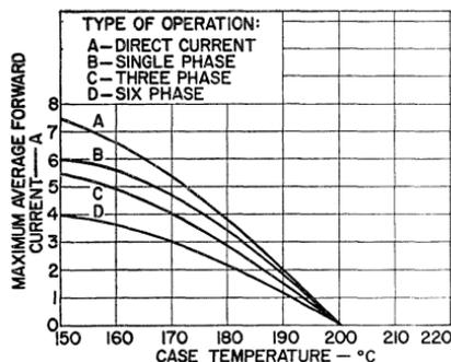
Figure 21. Current rating chart for a 12-ampere silicon rectifier.
