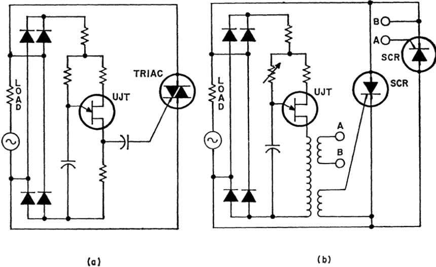
Figure 269. Circuit showing application of unijunction-transistor circuit for pulse triggering of triacs and inverse parallel SCR's: (a) triggering pulse is capacitively coupled to gate of triac; (b) triggering pulse is transformer-coupled to gate of SCR.
