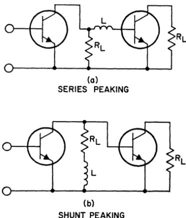
Figure 352. Circuits showing use of peaking coils to increase bandwidth: (a) series peaking; (b) shunt peaking.
