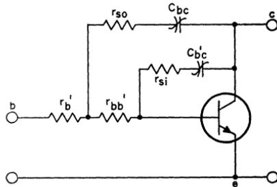
Figure 392. Circuit showing the nonlinear impedance factors that make possible frequency multiplication with overlay transistors.
