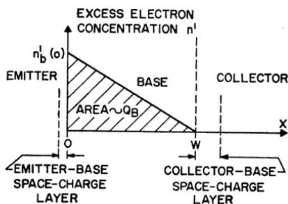
Figure 146. Excess minority-carrier concentration in the base region of a uniform-base n-p-n transistor.
