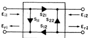
Figure 123. Scattering parameters for linear two-port network.
