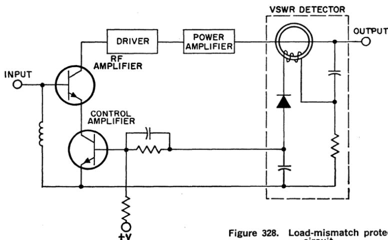
Figure 328. Load-mismatch protection circuit.
