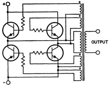
Figure 201. Basic circuit configuration of a four-transistor, single-transformer bridge inverter.
