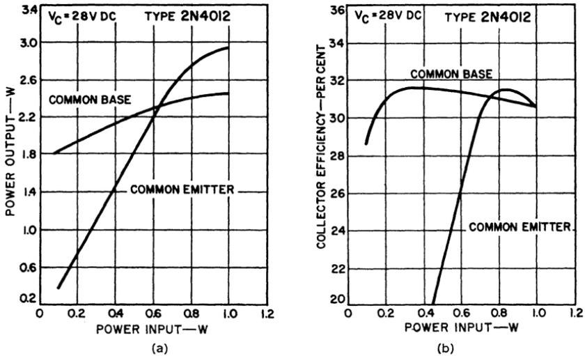
Figure 409. Comparison of performance characteristics of common-base and common-emitter tripler circuits using the RCA-2N4012 transistor: (a) Power output as a function of power input; (b) collector efficiency as a function of power input.
