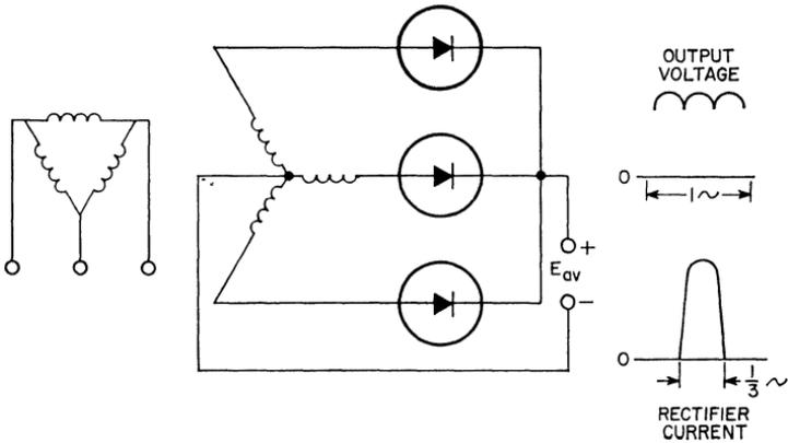
Figure 182. Three-phase "Y" half-wave circuit.
