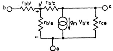
Figure 131. Simplified medium-frequency hybrid-pi transistor equivalent circuit.
