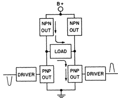
Figure 453. Block diagram of bridge type of audio-amplifier circuit.
