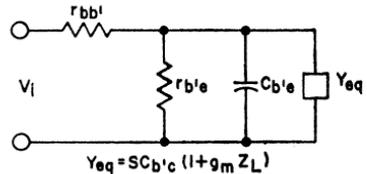
Figure 137. General equivalent input circuit for a common-emitter amplifier.
