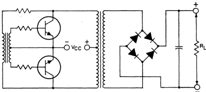
Figure 202. Basic circuit configuration of a two-transformer push-pull switching converter.
