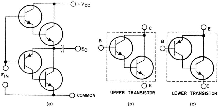
Figure 416. Compound output stage in which output transistors are driven by complementary driver transistors: (a) over-all circuit; (b) upper transistor pair; (c) lower transistor pair.
