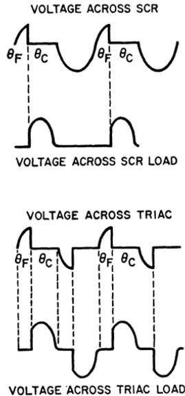
Figure 247. Voltage waveforms showing conduction angle for half-wave operation (SCR) and full-wave operation (triac) of thyristor phase-control circuits.
