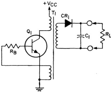
Figure 199. Basic circuit configuration for a ringing-choke dc-to-dc converter.
