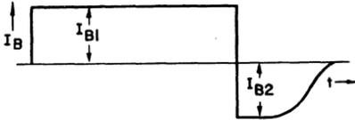
Figure 160. Base-current waveform that results from change in conducting state of a power transistor.
