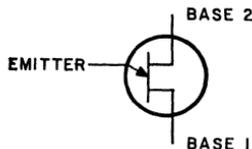
Figure 267. Schematic symbol for a unijunction transistor.
