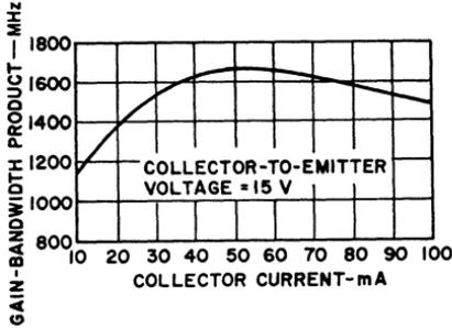
Figure 356. Gain-bandwidth product as a function of collector current for a typical RCA-2N5109 Transistor.
