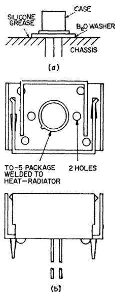
Figure 94. Suggested mounting arrangements for transistors having a JEDEC TO-5 package: (a) without heat sink; (b) with fin-type heat sink.
