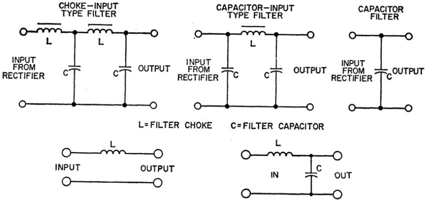
Figure 186. Typical filter circuits.
