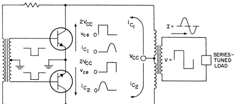
Figure 466. Use of a push-pull switching inverter to drive a transducer that forms part of a series-tuned load circuit.
