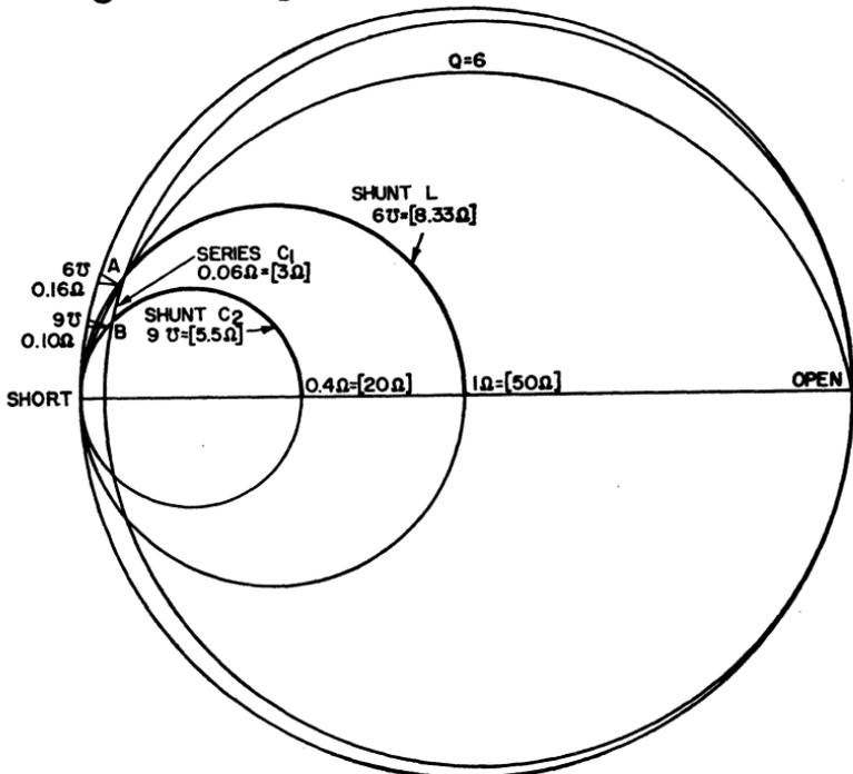
Figure 311. Circuit configuration and network map used to determine the component values for a tapped-C matching network.
