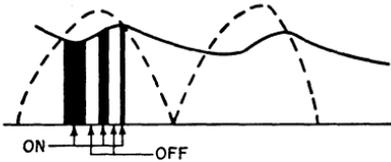
Figure 242. Effect of high-frequency switching of the switching regulator on power-supply ripple component.
