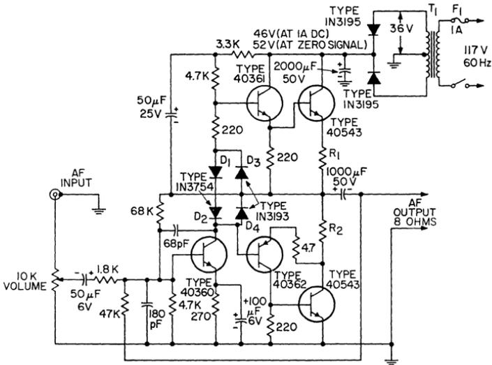
Figure 446. 25-watt (rms) quasi-complementary audio amplifier using current-limiting diodes ( $D_3$  and  $D_4$ ).
