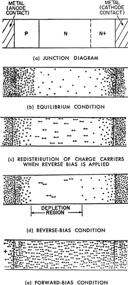
Figure 15. Concentrations of electrons (dots) and holes (circles) in a silicon rectifier.
