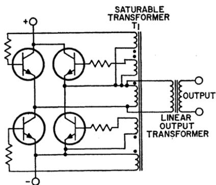
Figure 203. Basic configuration of a four-transistor bridge inverter that uses a saturable output transformer.
