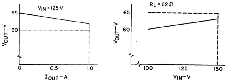
Figure 245. Performance characteristics of step-down switching regulator shown in Fig. 244.
