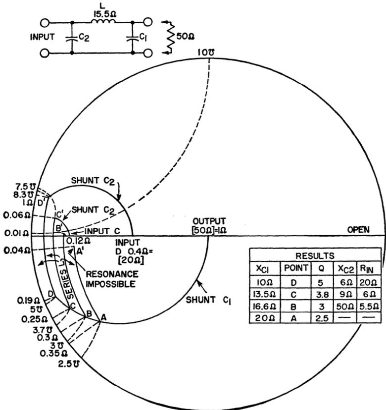
Figure 315. Circuit configuration for pi matching network and network map showing tuning range for variable components used in this type of matching network.
