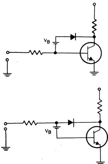
Figure 163. "Collector-catcher" circuits in which feedback is used.
