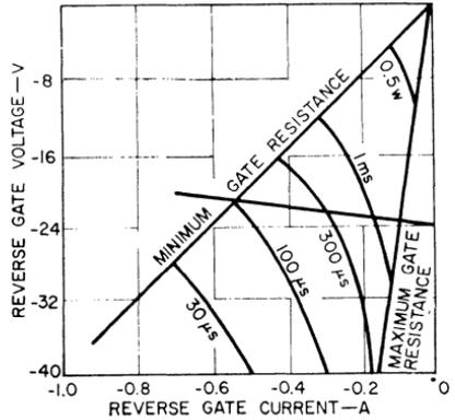
Figure 62. Reverse gate characteristics for typical RCA SCR's showing load line for a reverse gate-source voltage of 24 volts and an external circuit resistance of 5 ohms.
