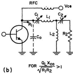
(1)  $X_{L1} = \frac{Q_L X_{C0}^2}{R_1} \left[ 1 - \frac{\sqrt{R_1 R_2}}{Q_L X_{C0}} \right]$
