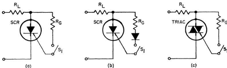
Figure 255. Simple thyristor triggering methods: (a) resistance triggering of SCR; (b) resistance-diode triggering of SCR; (c) resistance triggering of triac.
