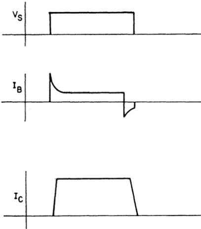
Figure 166. Waveforms for circuit shown in Fig. 165: (a) source voltage  $V_S$ ; (b) base current  $I_B$ ; (c) collector current  $I_C$ .
