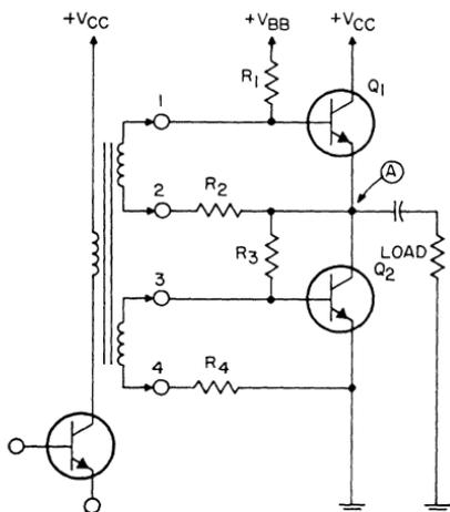
Figure 422. Circuit using a driver transformer that has split secondary windings to provide phase inversion for push-pull operation of a series-output circuit.
