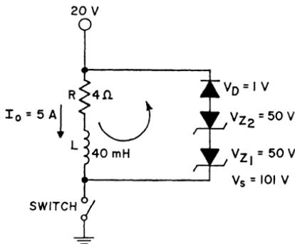
Figure 177. Circuits used in Example 3 to demonstrate the use of case-5 equations.
