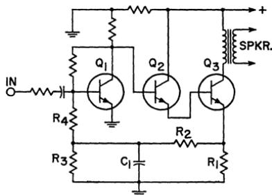
Figure 418. Three-stage, transformer-coupled, class A amplifier.
