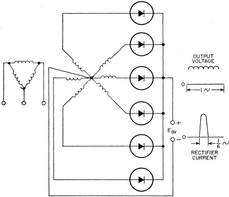
Figure 184. Six-phase "star" circuit.
