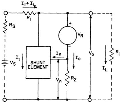
Figure 236. Basic configuration for a typical shunt regulator.
