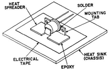
Figure 34. Typical heat-sink isolation technique for a chassis-mounted two-lead TO-5 thyristor.
