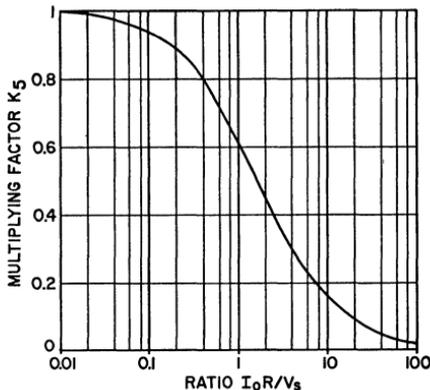
Figure 174. Multiplying factor  $k_5$  as a function of the ratio  $I_0 R / V_s$ .
