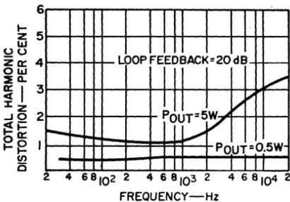
Figure 456. Total harmonic distortion of the bridge audio amplifier as a function of frequency.
