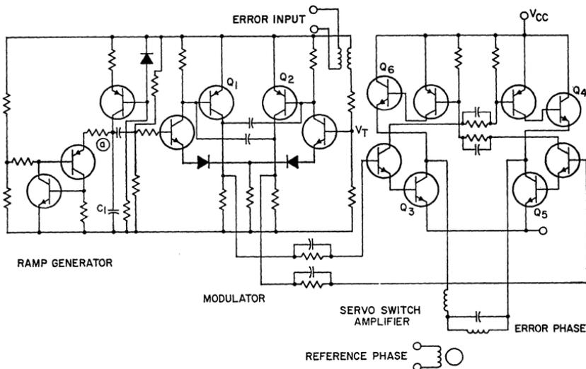
Figure 479. Switching-servo control amplifier with a pulse-width modulator.
