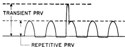
Figure 20. Typical waveform of repetitive and transient reverse voltages applied across a silicon rectifier.
