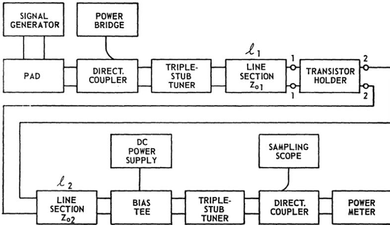
Figure 378. Block diagram of test setup used to determine input and output impedances of transistors.
