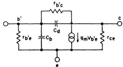
Figure 127. Elementary small-signal transistor equivalent circuit which includes components to represent effects of base-width modulation.
