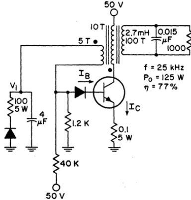
Figure 472. 125-watt, 25-kHz, class C oscillator.
