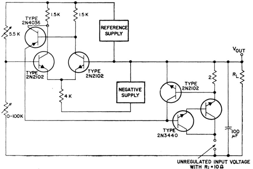
Figure 234. Schematic diagram of 100-volt series-regulated dc power supply in which output current is limited to a maximum value of 0.3 ampere.
