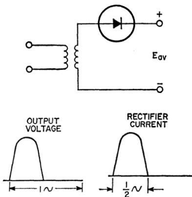
Figure 179. Single-phase half-wave circuit.
