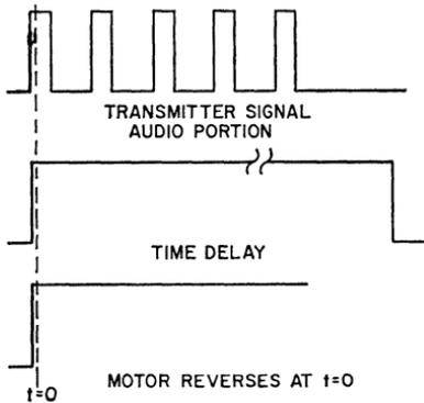
Figure 285. Timing diagram for reversing system.
