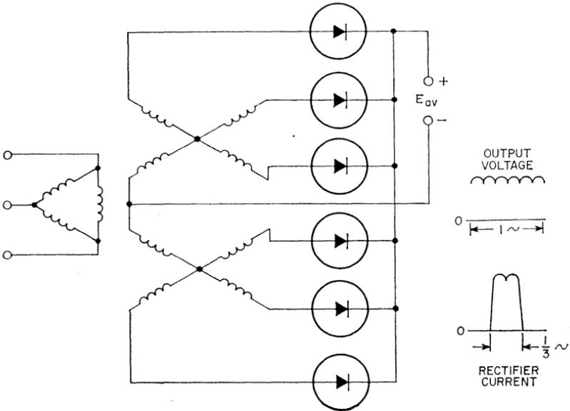
Figure 185. Three-phase "double-Y" and interphase-transformer circuit.
