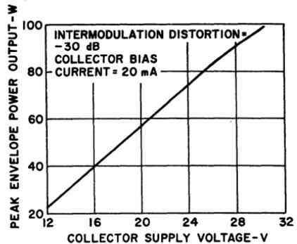
Figure 334. Peak envelope power as a function of collector supply voltage for the RCA SSB developmental transistor.
