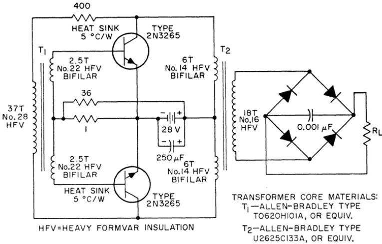
Figure 213. Schematic diagram of 250-watt, 50-kHz push-pull dc-to-dc converter.
