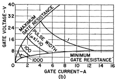
Figure 57. Forward-gate characteristics for pulse triggering of RCA SCR's: (a) low-current types, (b) high-current types.
