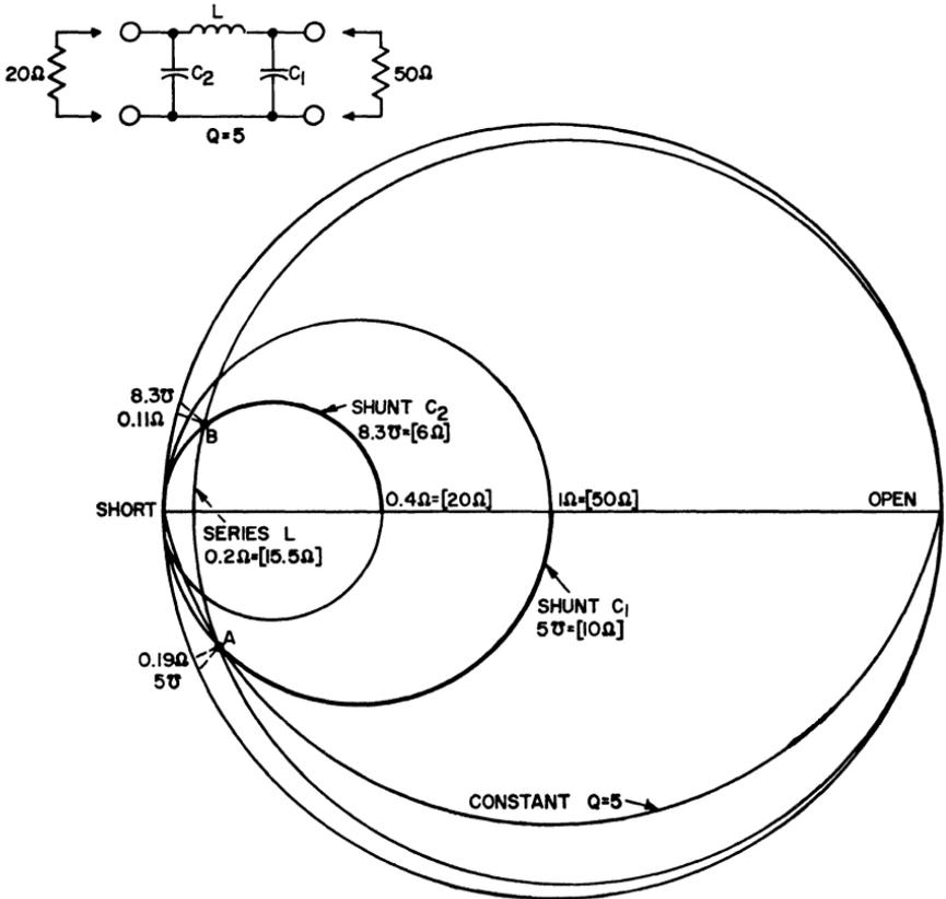
Figure 312. Circuit configuration and the network map used to determine the component value for a pi matching network.
