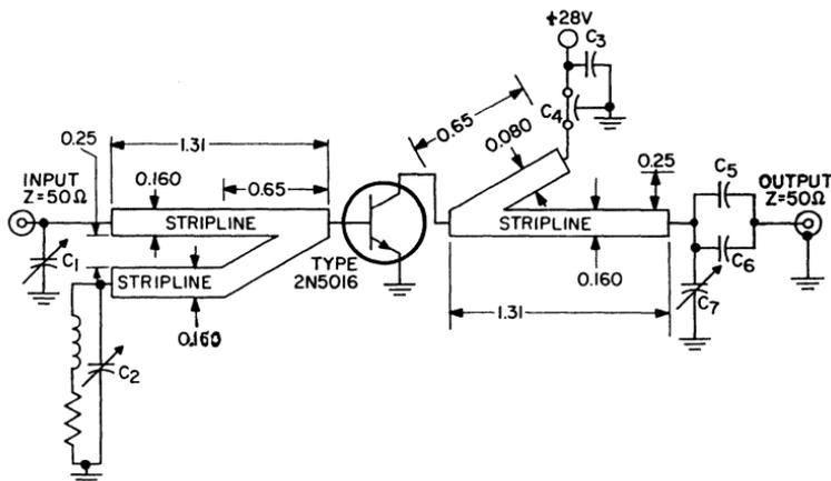
$C_1, C_2, C_7$  = trimmer capacitor, 2 to 18 pF, AmpereX HT10A/218 or equiv.
