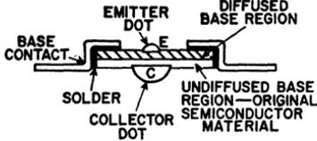
Figure 68. Cross-section of drift-field transistor.
