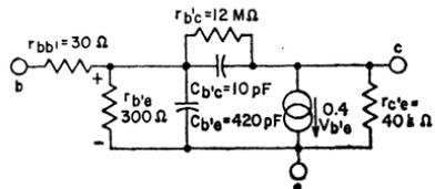
Figure 129. Hybrid-pi equivalent circuit for the 2N2102 triple-diffused silicon planar transistor.
