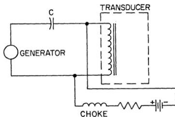
Figure 463. Circuit showing application of electrical power to a magnetostrictive transducer.
