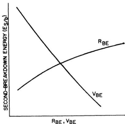
Figure 102. Variation in reverse-bias second-breakdown energy level as a function of  $V_{BE}$  and  $R_{BE}$ .
