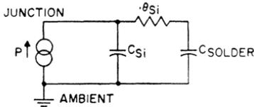
Figure 85. Simplified thermal equivalent circuit for a transistor when the duration of applied voltage and current is very short (i.e.,  $t \ll \theta_{\text{case}} C_{\text{case}}$ ).
