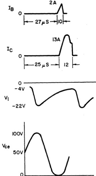
Figure 473. Current and voltage waveforms for the class C oscillator shown in Fig. 472.
