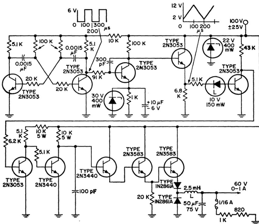
Figure 244. Typical step-down transistor switching regulator.
