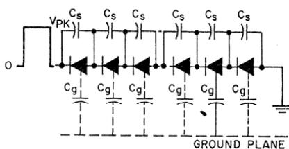
Figure 24. High-voltage rectifier assembly using shunt capacitors ( $C_s$ ) to compensate for stray capacitances ( $C_g$ ) and to equalize the reverse-recovery times of the rectifier units.
