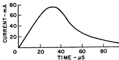
Figure 263. Typical current pulse that results from the discharge of a 0.1-microfarad capacitor through a neon bulb and a thyristor gate.
