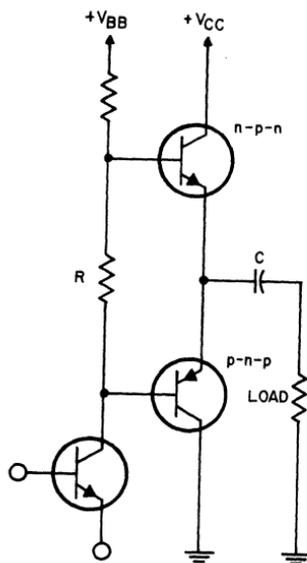
Figure 424. Basic complementary type of series-output circuit.
