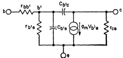
Figure 133. Simplified hybrid-pi transistor equivalent circuit for use at medium and high frequencies.
