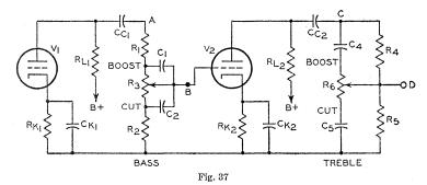
potentiometer is turned to its extreme variations (usually labeled "Boost" and "Cut"). In this network, as in the crystalequalizing network shown in Fig. 35, the parallel RC combination is the controlling factor. For bass "boost", the capacitor  $C_2$  bypasses resistor  $R_3$  so that The effect of the capacitor is negligible at low frequencies; beyond 1000 cycles, the signal voltage is attenuated at a maximum rate of 6 db per octave.
