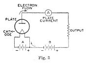
cathode, such as the 35W4, are called half-wave rectifiers, because current can flow only during one-half of the alternating-current cycle. When two plates and one or more cathodes are used in the same tube, current may be obtained on both halves of the ac cycle. The 6X4, 5Y3-GT, and 5U4-GB are examples of this type and are called full-wave rectifiers.
