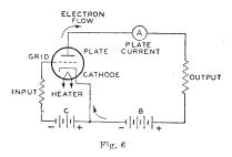
These capacitances are known as interelectrode capacitances. Generally, the capacitance between grid and plate is of the mostimportance. In high-gain radiofrequency amplifier circuits, this capacitance may act to produce undesired coupling between the input circuit, the circuit between grid and cathode, and the output circuit, the circuit between plate and cathode. This coupling is undesirable in an amplifier because it may cause instability and unsatisfactory performance.
