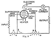
its negative potential with respect to the plate, the suppressor grid retards the flight of secondary electrons and diverts them back to the plate.
