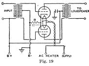
by plate-voltage-supply fluctuations are either eliminated or decidedly reduced through cancellation. Because distortion for push-pull operation is less than for single-tube operation, appreciably more than twice single-tube output can be obtained with triodes by decreasing the load resistance for the stage to a value approaching the load resistance for a single tube.
