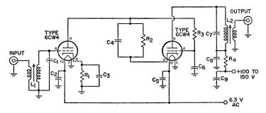
C<sub>1</sub>, C<sub>7</sub>=5  $\mu\mu$ f, 500 v., mica C<sub>2</sub>, C<sub>3</sub>, C<sub>4</sub>, C<sub>5</sub>, C<sub>6</sub>, C<sub>5</sub>, C<sub>9</sub>=0.001  $\mu$ f, 500 v., ceramic L<sub>1</sub>, L<sub>2</sub>=18 turns of No.32 Enam. copper wire wound
