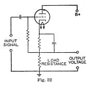
micromhos, the plate resistance is 62500 ohms, the amplification factor is 100, and the plate current is 0.0012 ampere.
