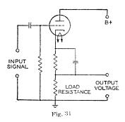
creased to make up for the voltage taken for biasing.
