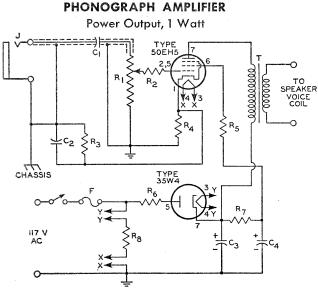
$\begin{array}{l} C_1 = 0.02 \ \mu\text{f}, \ \text{paper}, \ 400 \ \text{v}. \\ C_2 = 0.082 \ \mu\text{f}, \ \text{paper}, \ 400 \ \text{v}. \\ C_3 \ C_4 = 40 \mu\text{f}, \ \text{electrolytic}, \ 150 \ \text{v}. \\ F = F use, \ 1 \ \text{ampere} \\ J = Input \ \text{connector}, \ \text{shielded}, \\ \text{for crystal phonograph} \\ \text{pickup.} \end{array}$
