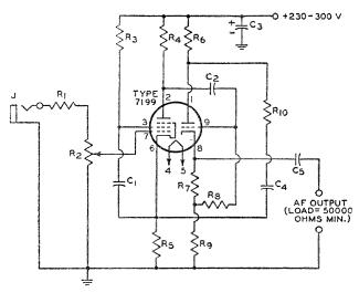
C<sub>1</sub>=0.1  $\mu$ f, paper, 400 v. C<sub>2</sub>=0.01  $\mu$ f, paper, 400 v. C<sub>3</sub>=20  $\mu$ f, electrolytic, 400 v. C<sub>4</sub>=0.25  $\mu$ f, paper, 400 v. C<sub>5</sub>=0.22  $\mu$ f, paper, 600 v. J=Input connector, shielded, for high-impedance ceramic phono pickup (0.5 v. output)  $R_1=1.8$  megohms, 0.5 watt  $R_2=$  Volume control, potentiometer, 500000 ohms, audio taper
