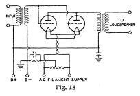
power sensitivity and efficiency than triode or conventional pentode types.
