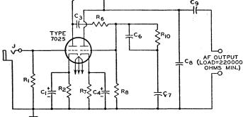
C<sub>1</sub> C<sub>4</sub>=25  $\mu$ f, electrolytic, 25 v. C<sub>2</sub> C<sub>5</sub>=20  $\mu$ f, electrolytic, 450 v. C<sub>3</sub>=0.1  $\mu$ f, paper, 600 v. C<sub>5</sub>=0.0033  $\mu$ f, paper, 600 v. C<sub>7</sub>=0.01  $\mu$ f, paper, 600 v. C<sub>7</sub>=0.01  $\mu$ f, paper, 600 v. 500 v.C<sub>1</sub>=0.22  $\mu$ f, paper, 600 v.
