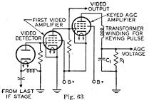
biased so that current flows only when the grid No.1 and the plate are driven positive simultaneously. The amount of current flow depends on the grid-No.1 potential during the pulse. These pulses are smoothed out in the RC network in the plate circuit ( $R_1C_1$ ). Because the dc voltage developed across  $R_1$  is negative, it is suitable for application to the grids of the rf and if tubes as an agc voltage.
