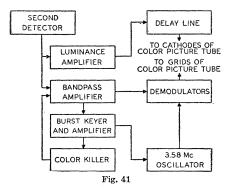
band from approximately 2.4 to 4.5 Mc is fed to a bandpass amplifier, as shown in the block diagram in Fig. 41. The color synchronizing signal, or "burst," contained in this signal may then be fed to a "burst-keyer" tube. At the same time, a delayed horizontal pulse may be applied to the keyer tube. The output of the keyer tube is applied to the burst amplifier tube and the signal is then fed to the 3.58-Mc oscillator and to the "color-killer" stage.
