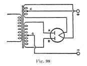
in inverse relation to that causing current flow. The peak value of this voltage is limited by the resistance and nature of the path between plate B and filament. The maximum value of this voltage at which there is no danger of breakdown of the tube is known as maximum peak inverse voltage.
