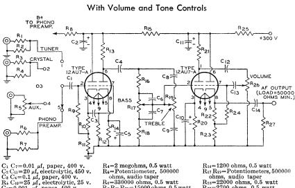
$\begin{array}{l} C_2 C_{11} = 20 \ \text{af, electrolytic, 450 v.} \\ C_3 C_4 = 0.1 \ \text{µf, paper, 400 v.} \\ C_8 = 470.001 \ \text{µf, paper, 400 v.} \\ C_8 = 470 \ \text{µf, mica, 300 v.} \\ C_9 = 4700 \ \text{µf, mica, 300 v.} \\ C_{12} C_{14} = 0.47 \ \text{µf, paper, 400 v.} \\ C_{12} = 0.033 \ \text{µf, paper, 400 v.} \\ R_1 R_2 R_7 = 270000 \ \text{ohms, 0.5 watt} \\ R_3 = 1.5 \ \text{megohms, 0.5 watt} \end{array}$
