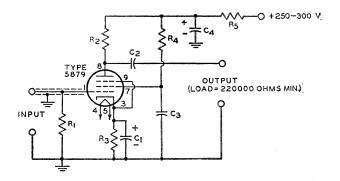
$\begin{array}{l} R_{3}{=}1000 \text{ ohms, } 0.5 \text{ watt} \\ R_{4}{=}0.47 \text{ megohm, } 0.5 \text{ watt} \\ R_{5}{=}22000 \text{ ohms, } 0.5 \text{ watt} \end{array}$
