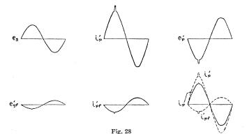
$e'_{p}$ , the feedback voltage appearing on the grid is as shown by  $e'_{gf}$ . This voltage applied to the grid produces a component of plate current  $i'_{pf}$ . It is evident that the irregularity in the waveform of this component of plate current would act to cancel the original irregularity and thus reduce distortion.
