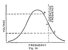
the voltage developed across the circuit varies at the modulating rate. In order that no distortion will be introduced in this circuit, the frequency swing must be restricted to the portion of the slope which is effectively straight. Since this portion is very short, the voltage developed is low. Because of these limitations, this circuit is not commonly used but it serves to illustrate the principle.
