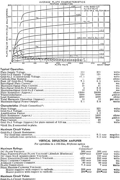
+ The duration of the voltage pulse must not exceed 15 per cent of one vertical scanning cycle. In a 525-line, 30-frame system, 15 per cent of one vertical scanning cycle is 2.5 milliseconds. • Under no circumstances should this absolute value be exceeded.
