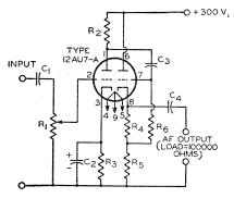
C<sub>1</sub> C<sub>3</sub>=0.1  $\mu$ f, paper, 400 v. C<sub>2</sub>=25  $\mu$ f, electrolytic, 25 v. C<sub>4</sub>=0.5  $\mu$ f, paper, 200 v.
