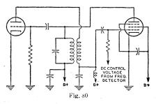
The plate current of the reactance tube is shunted across the oscillator tank circuit. Because the plate current and plate voltage of the reactance tube are almost  $90^{\circ}$  out of phase, the control tube affects the tank circuit in the same manner as a reactance. The grid bias of the tube determines the magnitude of the effective reactance and, consequently, a control of this grid bias can be used to control the oscillator frequency.
