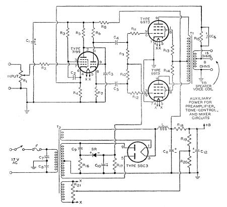
$C_1=40 \ \mu f$ , electrolytic, 450 v.  $C_2 C_4 C_5=0.25 \ \mu f$ , paper, 400 v.  $C_3=3.3 \ \mu \mu f$ , ceramic or mica,
