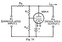
$R_1$  and  $R_2$ . This increased grid voltage causes the tube to draw an increased current from the unregulated supply. The increased current, in turn, causes a voltage drop across the high internal impedance of the unregulated supply,  $R_s$ , which tends to counteract the original rise of the voltage. If desired, the grid may be connected to a variable point on the voltage divider to allow some adjustment of the output-voltage level.
