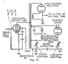
ond half of the cycle, the voltage swings below the plate supply voltage, and the damper diode conducts, damping out the oscillation. At the same time, the current through the deflecting yoke reverses and reaches its negative peak. As the damperdiode current decays exponentially to zero, the output tube begins to conduct again. The yoke current, therefore, is composed of current resulting from damper-diode conduction.
