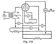
The power-output test probably gives the best correlation between test results and actual operating performance of a tube. In the case of voltage amplifiers, the power output is indicative of the amplification and output voltages obtainable from the tube. In the case of power-output tubes, the performance of the tube is closely checked. Consequently, although more complicated to set up, the power-output test will give closer correlation with actual performance than any other single test.
