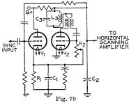
across the capacitor  $C_2$ . A portion of this sawtooth is fed back to the grid of the control tube,  $V_1$ . The positive sync pulses are also applied to the grid of  $V_1$ . The waveforms shown in Fig. 71 illustrate the sawtooth and sync pulses (A and B) and their proper "in-sync" combination (C). The sync pulse occurs partly during the portion of the sawtooth voltage in which the triode  $V_1$  draws current. Any shift in sync pulse as it is superimposed
