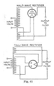
positive with respect to the cathode, and through plate No. 2 on the next halfcycle when plate No. 2 is positive with respect to the cathode.
