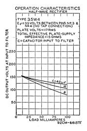
Tube requires miniature seven-contact socket and may be mounted in any position. Outline 13, OUTLINES SECTION. For heater considerations, refer to miniature type 35C5.
