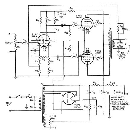
$C_1=25 \ \mu f$ , electrolytic, 50 v.  $C_2=22 \ \mu \mu f$ , ceramic or mica, 600 v.
