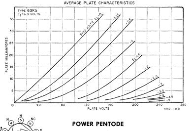
Miniature type used in the output stage of audio amplifying equipment and also in the video output stage of television receivers. Outline 18, OUT-LINES SECTION. Tube requires
