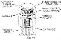
reach that portion of the target behind the electrode. Because the target does not glow where it is shielded from electrons, the control electrode casts a shadow on the glowing target. The extent of this shadow varies from approximately  $100^{\circ}$  of the target when the control electrode is much more negative than the target to  $0^{\circ}$  when the control electrode is at approximately the same potential as the target.
