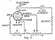
this shielding action is increased by a bypass capacitor connected between screen grid and cathode. By means of the screen grid and this bypass capacitor, the grid-plate capacitance of a tetrode is made very small. In practice, the grid-plate capacitance is reduced from several micromicrofarads ( $\mu\mu$ ) for a triode to 0.01  $\mu\mu$ f or less for a screen-grid tube.
