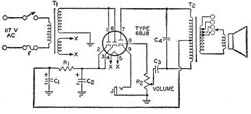
$C_1 C_2=20 \ \mu f$ , electrolytic, 150 v.  $C_3=0.001 \ \mu f$ , paper, 200 v.  $C_4=0.03 \ \mu f$ , paper, 200 v. F=1/8 ampere
