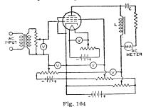
operation of tubes. The diagram illustrates the method for a pentode. The ac output voltage developed across the plate-load impedance (L) is indicated by the current meter. The current meter is isolated as far as the dc plate current is concerned by the capacitor (C). The power output can be calculated from the current reading and known load resistance. In this way, it is possible to determine the operating condition of the tube quite accurately.
