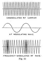
the frequency of the rf wave deviates from a mean value, at an af rate depending on the modulation, by an amount that is determined in the transmitter and is proportional to the amplitude of the af modulation signal.
