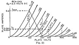
point  $I_{max}$ . Then,  $I_{max}$  is determined from the curve for use in the formula
