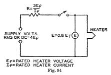
resistance having a value 3 times the nominal heater operating resistance (R = 3  $E_t/I_t$ ), and a voltage having a value 4 times the rated heater voltage (V = 4  $E_t$ ) is then applied. The warm-up time is determined when E = 0.8  $E_t$ .
