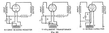
the resistor, or if the tube or tubes employ more than three electrodes, the total current determines the size of the resistor.
