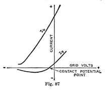
the initial velocity of emission of electrons from the cathode and an electrothermal effect due to the differences in temperature and in material composition of the grid and the cathode.
