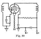
in the voltage drop across the series resistor in the screen-grid circuit; the result is a change in the power output and an increase in distortion. The screengrid voltage should be obtained from a point in the plate-voltage-supply filter system having the correct voltage, or from a separate source.
