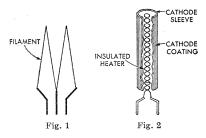
Directly heated filament-cathodes require comparatively little heating power. They are used in almost all of the tube types designed for battery operation because it is, of course, desirable to impose as small a drain as possible on the batteries. Examples of battery-operated filament types are the 1R5, 1U4, 1U5, and 3V4. AC-operated types having directly heated filament-cathodes include the 2A3 and 5Y3-GT.
