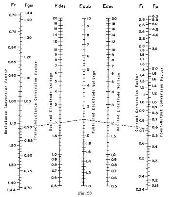
0.57,  $F_r$  is 1.12, and  $F_{cm}$  is approximately 0.892. These factors may be applied directly to operating values shown in the tube data, or to values calculated by the methods described previously.
