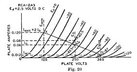
the grids run positive is inadvisable except under conditions such as those discussed in this section for class AB and class B amplifiers. the value of the load resistance. The load resistance in ohms is equal to  $(E_{max} - E_{min})$  divided by  $(I_{max} - I_{min})$ , where E is in volts and I is in amperes.
