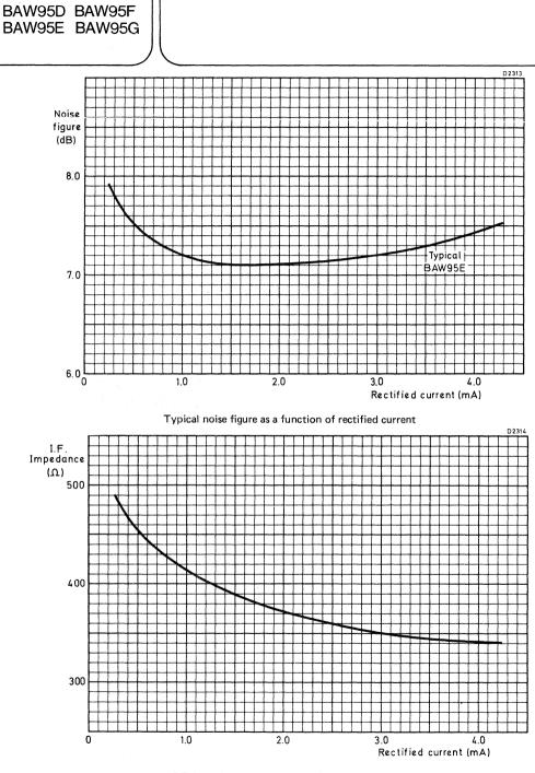
I.F. impedance as a function of rectified current
