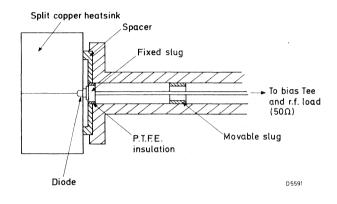
Coaxial test oscillator cavity
