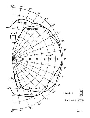
Typical polar diagram for antenna supplied
