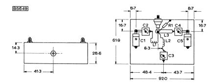
Component layout of tripler circuit
