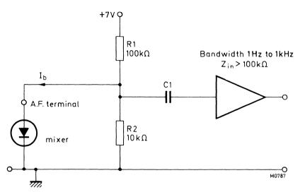
Fig.1 Circuit used to measure a.f. performance
