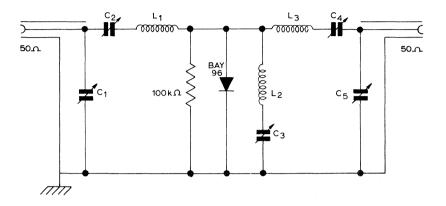
Frequency tripler circuit - 150 to 450 MHz
