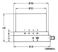
Connections: 1-2 Main coil 3-4 Fast coil 5 --V Gunn earth 6 + V Gunn
