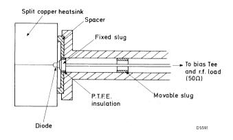
Coaxial test oscillator cavity
