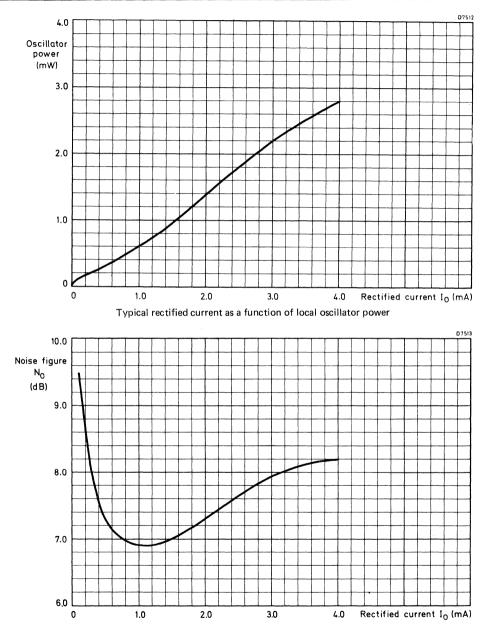
Typical noise figure as a function of rectified current
