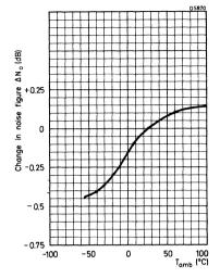
Typical change in overall noise figure as a function of temperature
