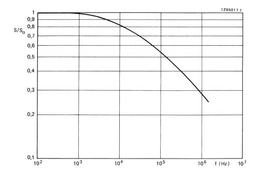
Fig. 4 Typical sensitivity variation of the fast coil versus the sweeping frequency  $S_{\rm O}$  = 320 kHz/mA.
