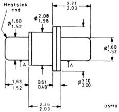
A = concentricity tolerance =  $\pm 0.13$ Normal operation with reverse bias, i.e. heatsink end positive.
