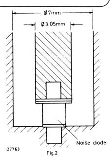
Device mounted in a 50  $\Omega$  7 mm coaxial line
