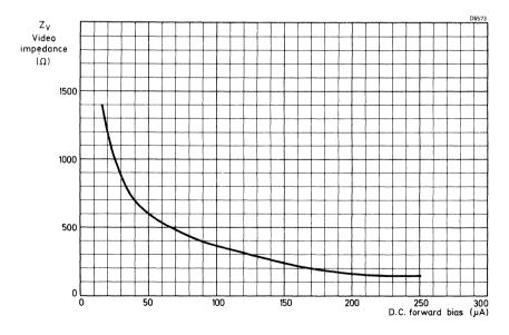
Typical video impedance as a function of d.c. forward bias current (as a detector)
