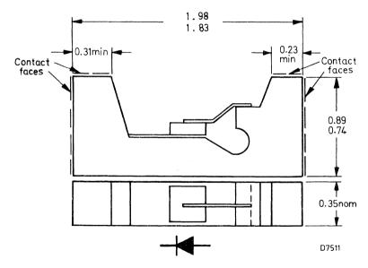
Contact faces are gold plated, 5  $\mu$ m over 1.27  $\mu$ m of nickel.
