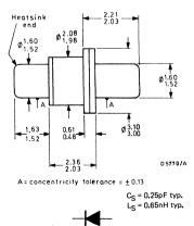
case style SOD-31 conforms to BS3934 SO-86
