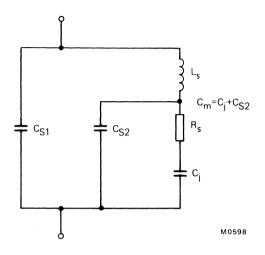
2. Measured at and about the series resonant frequency, in a suitable waveguide holder, enable the values of  $f_0$  and the diode Q factor to be determined. The effective diode capacitance and the cut-off frequency can be calculated taking  $L_s$  to be the typical value.
