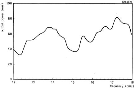
Fig. 7 Typical test curve of YG1105.
