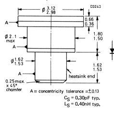
case style SOD-31 conforms to BS3934 SO-86
