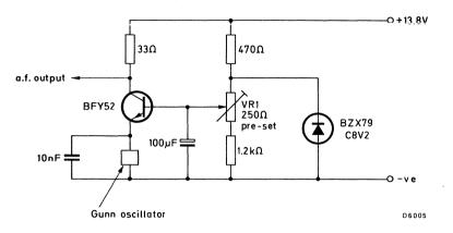
VR1 is used to set voltage at 7.0 V across Gunn oscillator.
