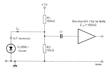
Circuit used to measure a.f. performance
