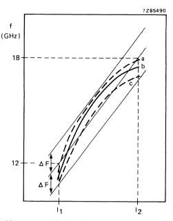
Fig. 4 Linear relation of frequency as a function of current in main coil; typical values, curve a at -40 °C; curve b at +25 °C and curve c at +85 °C.
