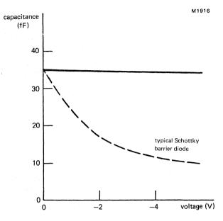
Fig.3 Typical capacitance as a function of voltage
