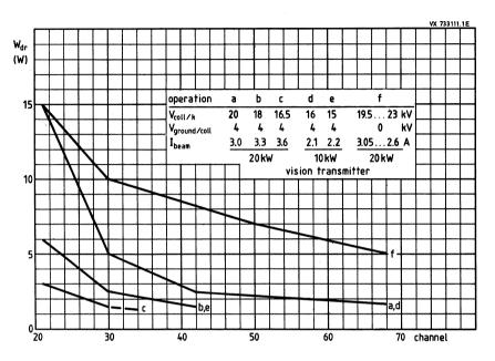
Fig. 10 Max. drive power in dependence on channel and operation mode.
