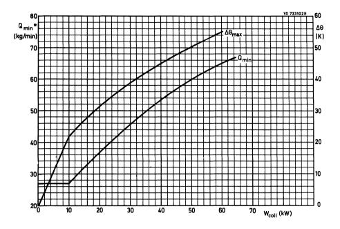
Fig. 3 Required quantity of cooling air  $\Omega_{min}$  for the inlet temperature T<sub>i</sub> = 25 °C and relative temperature difference  $\Delta\theta$  versus the collector dissipation W<sub>coll</sub>.
