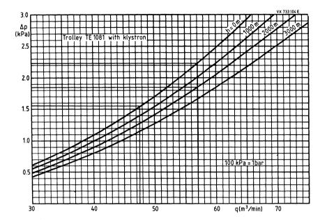
Fig. 5 Calculation of the pressure drop  $\Delta p$  between air inlet and air outlet at the trolley TE1081 as a function of cooling air volume q for selection of the correct blower.
