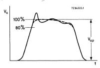
Fig. 2 Voltage pulse.
