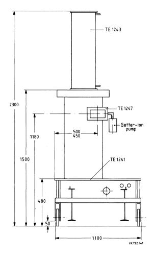
Fig. 3 Complete assembly consisting of tube, trolley, oil tank, focus mount, r.f. transition and operational lead shieldings.
