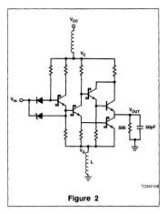
Figure 2 shows an example of a buffer connected to a test load. Probing on the ground pad, V<sub>G</sub>, shows the effect ground lead inducance has on the ground pad potential.
