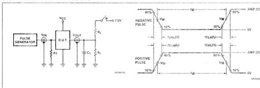
Test Circuit For 3-State Outputs
