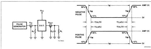
Test Circuit for Totem-Pole Outputs
