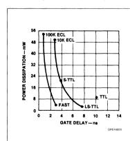
Figure 1. The Speed/Power Spectrum
