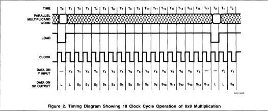
The MSB  $Y_7$  (the sign bit  $Y_S$ ) of the multiplier is first applied to the Y input during  $T_8$  and must also be applied during bit times  $T_9$  through  $T_{16}$ . This extension of the sign bit is a necessary adjunct to the implementation of Booth's algorithm and is a built-in feature of
