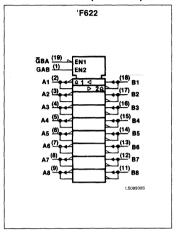
These devices allow data transmission from the A bus to the B bus or from the B bus to the A bus, depending upon the logic levels at the Enable inputs (GBA and GAB). The enable inputs can be used to disable the device so that the buses are effectively isolated
