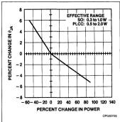
Figure 8. Average Effect of Power Dissipation on SMD  $\theta_{\rm JA}$
