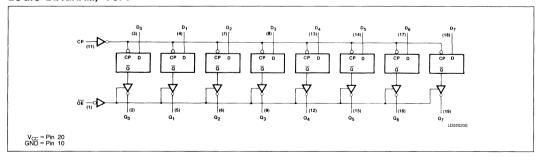
When  $\overline{\text{OE}}$  is LOW, the latched or transparent data appears at the outputs. When  $\overline{\text{OE}}$  is HIGH, the outputs are in the HIGH impedance "off" state, which means they will neither drive nor load the bus.
