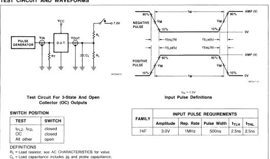
C<sub>L</sub> = Load capacitance includes jig and probe capacitance see AC CHARACTERISTICS for value.
