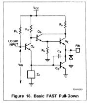
Switching to the logic I OW state occurs when  $V_{IN}$  is larger than the  $V_{BE}$  drops of  $O_{C}$  plus  $O_{C}$ , both of which are on. Part of the total emitter current available from  $O_{C}$  comes from  $O_{C}$ , which has a voltage drop of  $O_{CC} - O_{CC} - O_{CC} - O_{CC}$ . The remainder of the  $O_{C}$  emitter current is supplied through its base Schottky clamp or by other components not shown in Figure 18 but discussed in the section on
