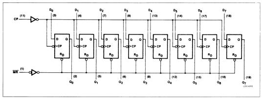
The register is fully edge-triggered. The state of each D input, one set-up time before the LOW-to-HIGH clock transition, is transferred to the corresponding flip-flop's Q output.
