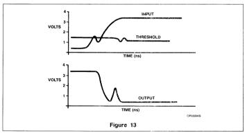
The incorporation of hysteresis circuitry into high performance TTL logic provides few user benefits and can actually create more system problems that it solves. The added circuitry consumes power, slows down logic delays and increases input loading. Input hysteresis is also very difficult to test on high-speed
