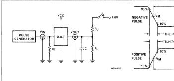
Test Circuit For 3-State Outputs
