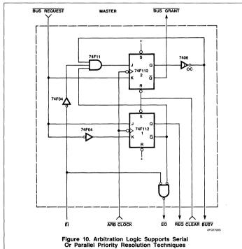
design. BUSY is generated by the master currently accessing the bus to indicate that the bus is in use. Even after a master has been granted access by the priority resolution, it must still wait for the current master to vacate the bus, i.e., BUSY going inactive. The
