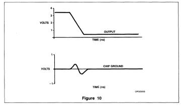
with a kink in the threshold region caused by a poorly terminated line, and/or poor decoupling at the driver. The double crossing of the input threshold has caused a glitch in the output waveform. Ideally, the incorporation of hysteresis circuitry in a receiver would improve AC noise immunity and prevent the glitched output by changing the input threshold as soon as the output begins to switch. However, Figure 13 shows that the change in input threshold occurs after the output begins to switch.
