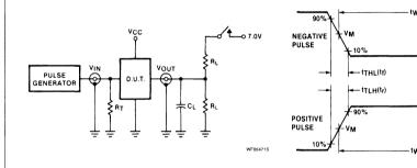
Test Circuit For 3-State Outputs
