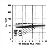
Figure 15. Results of Air Flow on  $\theta_{\rm JA}$  on SO-14 With Copper Leadframe
