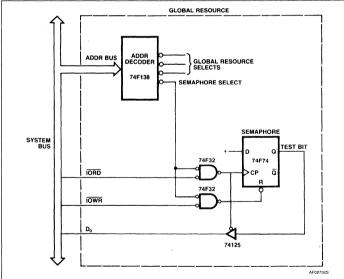
Figure 14. Semaphore (Flag) Register Permits Access To Shared Resource Without Monopolizing Shared Bus
