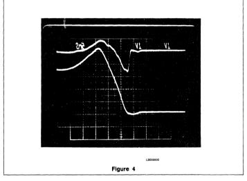
alternate 1's and 0's were clocked into seven of the eight flip-flops to obtain simultaneous output switching and worst case ground bounce. The eighth flip-flop input was held at a DC bias of 2.0V. This should result in its output being held at a constant 1 level.
