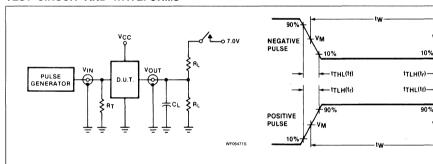
Test Circuit For 3-State Outputs
