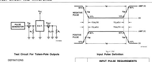
$R_L$  = Load resistor; see AC CHARACTERISTICS for value.  $C_L$  = Load capacitance includes jig and probe capacitance; see AC CHARACTERISTICS for value.
