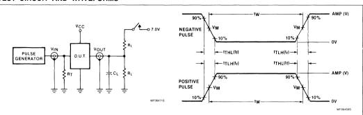
Test Circuit For 3-State Outputs
