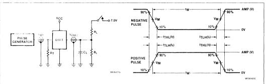
Test Circuit For 3-State Outputs
