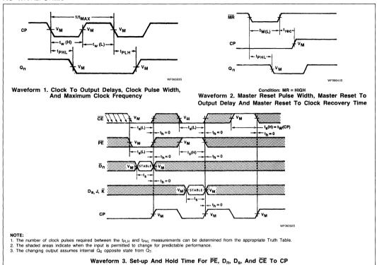
NOTE: For all waveforms, V<sub>M</sub> = 1.5V.
