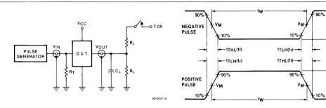
Test Circuit For 3-State Outputs
