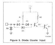
The diode cluster input (Figure 5) looks like a multiple-emitter input, except that its break-down voltage is higher because separate Schottky junctions are used instead of a transistor. It has limited use in FAST circuits.
