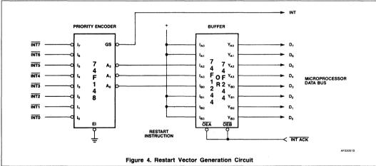
generally used for the vectors. The format of the restart instructions is 11CBA111 (binary), where CBA represents the three-bit identifier. Figure 4 illustrates a restart vector generation circuit.
