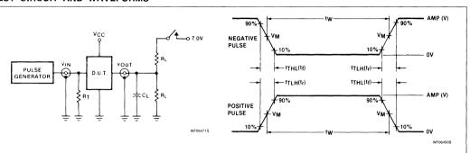
Test Circuit For 3-State Outputs
