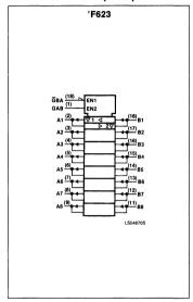
These devices allow data transmisstion from the A bus to the B bus or from the B bus to the A bus, depending upon the logic levels at the Enable inputs (GBA and GAB). The Enable inputs can be used to disable the device so that the buses are effectively isolated.
