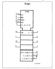
Counting is inhibited by a HIGH level on the Count Enable ( $\overline{CE}$ ) input. When  $\overline{CE}$  is LOW, internal state changes are initiated.
