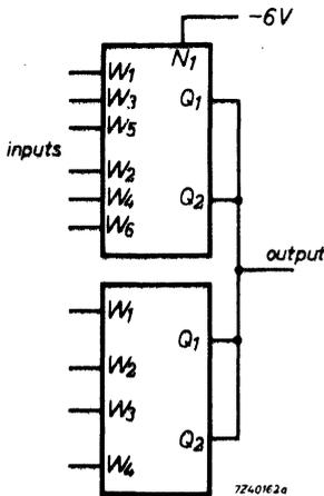
Fig.72. 10-input N-gate, composed of one 2.3N1 and one 2.2N1.
