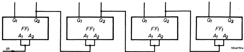
Fig.63. Scaler of 16. (Binary counter with 4 flip-flops.)
