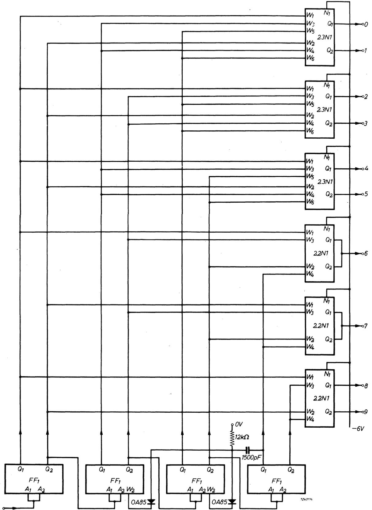
Fig.75. A count of  $n$  in the decimal counter produces a "1" signal at the output  $n$  at the right. All  $N$ ,  $E$  and  $P$  terminals of the flip-flops should be connected to the corresponding supply lines.
