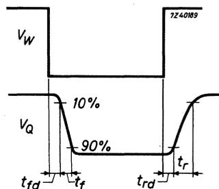
The switching and delay times are given for two values of the collector current, taken from the OC47 transistor.
