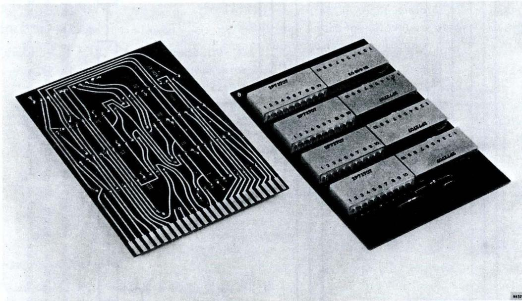
Fig.80. Circuit blocks mounted on a printed-wiring board.
