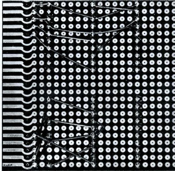
Fig.82. Rear side of an experimenter's printed wiring board with circuit blocks mounted on it.
