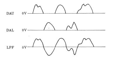
Fig. 19 Class B operation output and input waveforms
