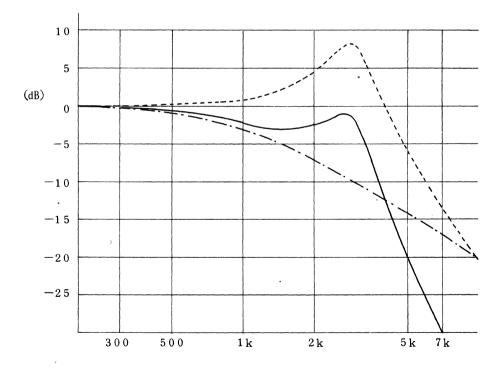
Fig. 52 Designed filter frequency response (3rd order)
