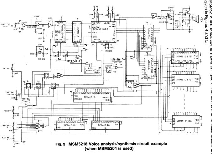
MSM5218 Voice Analysis/Synthesis Circuit Example (When MSM5204 is
