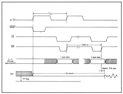
Phrase specifying input is from channel 1 to channel 4 continuously. <sup>\*1</sup> An interval of 15 Tcyc (max.) is needed between phrases.
