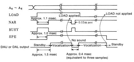
Fig. 14 MSM6243 Switch input timing diagram
