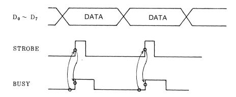
Fig. 16 Centronic interfaces in/out timing
