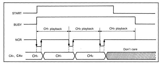
Continuous playback and repeated playback are acheived by maintaining Start terminal at "H" level. Writing to channel is done when NCR goes low, or when starts playinh back each word. So chennels will be changed, if "START" is high, when NCR goes from low to high.
