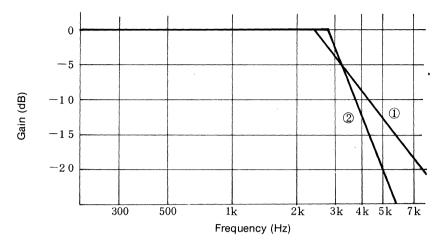
Fig. 43 f<sub>SAMPLE</sub> 8 kHz filter frequency response
