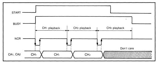
Continuous playback and repeated playback are made by maintaining start terminal at "H" level. Writing channel is done when NCR falls down, or the time when starts playbacking each word. So, changing channel is made by turning it with the time when NCR stands up.
