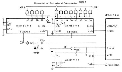
Note 1. The 12-bit output is in regular straight binary code.
