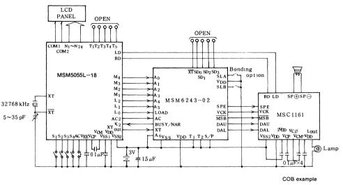
Note: If bonding on chip, make sure that MSC1161 is (begin-ind) isolated from MSM5055 and MSM6243. (See accompanying diagram.)
