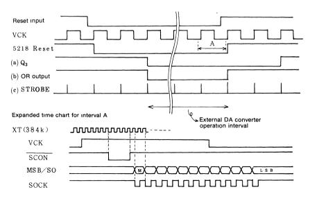
Fig. 9 MSM5218 and external DA converter time chart
