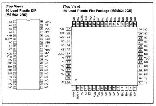
Note: Connect pin 23 (V\_DD") with V\_DD and V\_DD' externally since this pin is conducted to the substrate.
