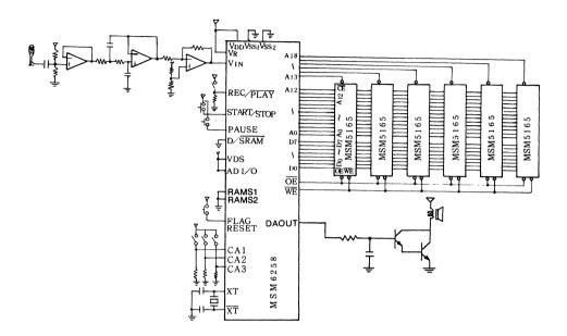
Fig. 10 MSM6258 application circuit example
