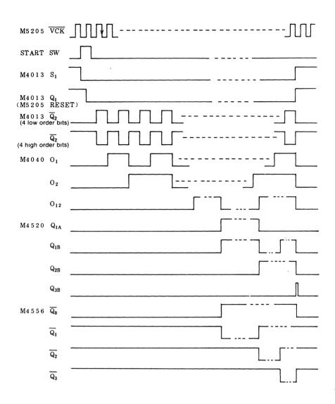
Fig. 2 MSM5205 application circuit example time chart
