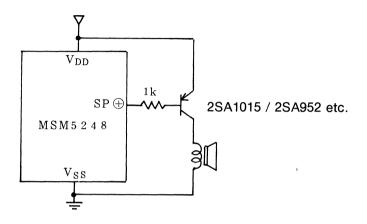
Fig. 24 Output circuit example
