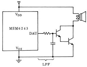
Fig. 27 MSM6243 output circuit example (for class A operation)
