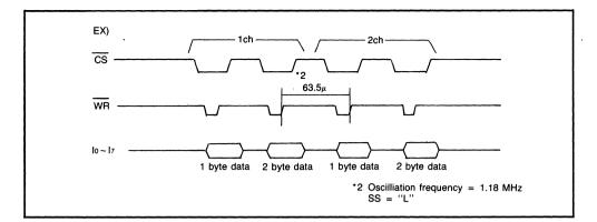
Voice synthesis operation can be started from any channel, 1 to 4. The arrangement of each channel is of no concern.
