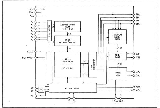
T<sub>1</sub>, T<sub>2</sub>, S/P and SD<sub>3</sub>, SD<sub>2</sub>, SD<sub>1</sub>, SD<sub>0</sub> are test pins.
