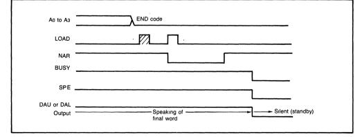
Note: t<sub>A</sub> ...... Address hold time t<sub>NL</sub> ..... Double LOAD pulse interval t<sub>L</sub> ..... LOAD pulse width t<sub>MN</sub>...... NAR "H" width
