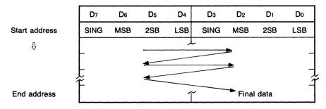
Sound source data is compatible with the data which is analyzed by MSM5218 or MSM6258. In addition, the data which is analyzed by analyzer is usable, too.
