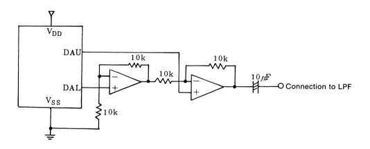
Fig. 18 MSM6212 and OP amplifier interface example 1
