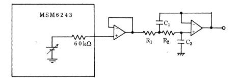
Fig. 53 MSM6243 and filter interface
