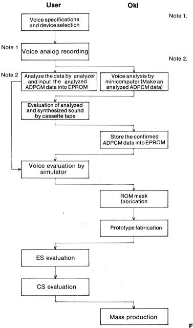
e 1. Record the source sound on an open-reel tape deck. Recording assistance
