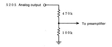
Fig. 54 Audio amplifier connection
