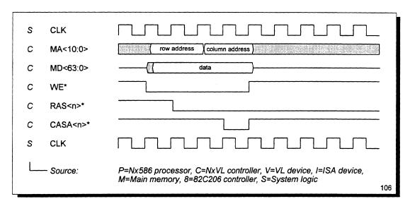
Figure 61 Fast Write to Main Memory (No Precharge)
