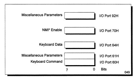
Figure 64 Configuration Registers (I/O-Mapped)
