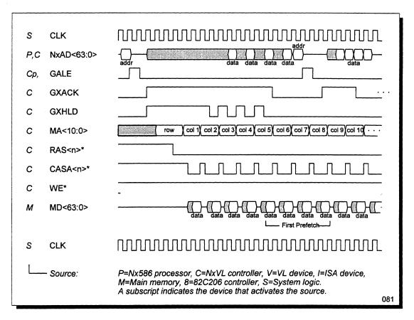
Figure 37 Processor 32-Byte Block Read from Main Memory
