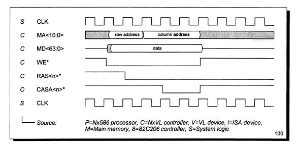
Figure 58 Slow Write to Main Memory (No Precharge)
