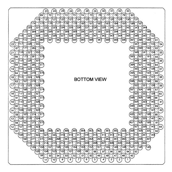
Figure 7 NxVL Pinout Diagram (Bottom View)
