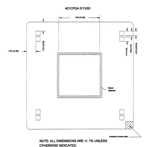
Figure 68 NxVL Package Diagram (top)
