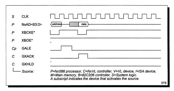
Figure 34 Processor 64-Bit Write to Main Memory (Queue Hit)
