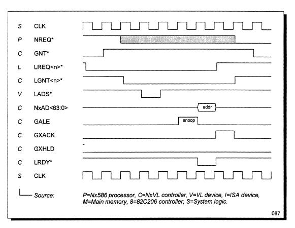
Figure 44 Bus Arbitration by VL-Bus Master
