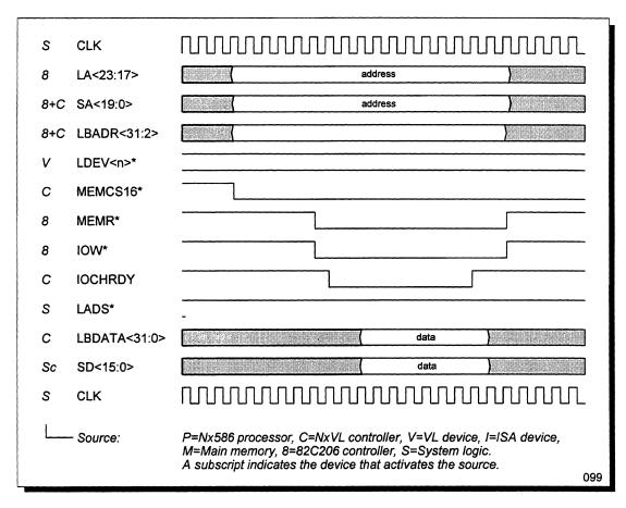
Figure 57 DMA Transfer from Main Memory to ISA-Bus 8-Bit I/O
