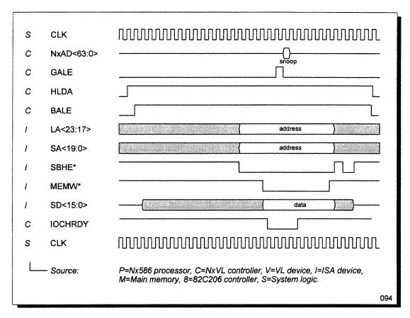
Figure 51 ISA-Master 16-Bit Write to Main Memory
