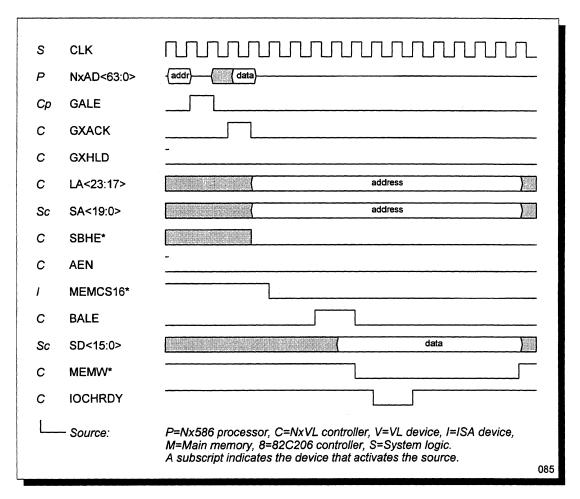
Figure 41 Processor 16-Bit Write to ISA-Bus 16-Bit Memory
