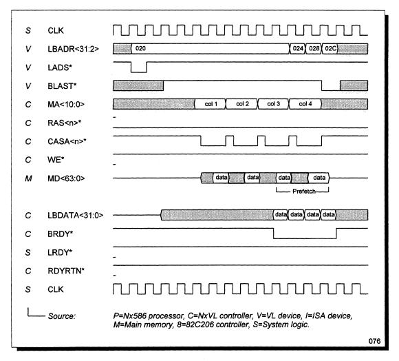
Figure 47 VL-Master 16-Byte Burst Read from Main Memory
