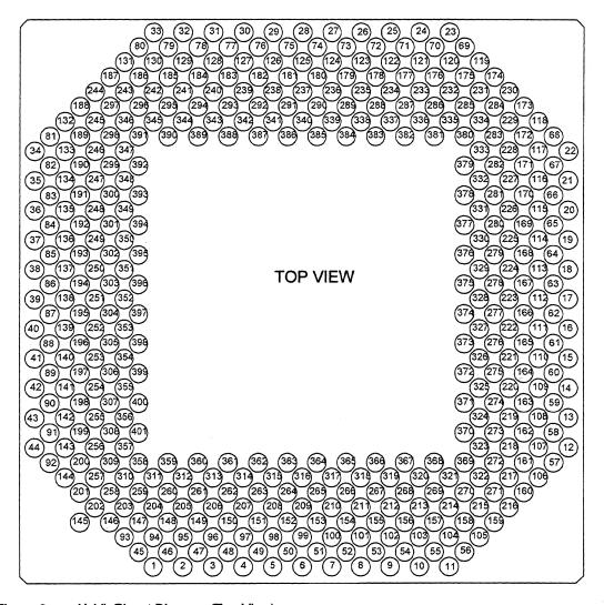
Figure 6 NxVL Pinout Diagram (Top View)
