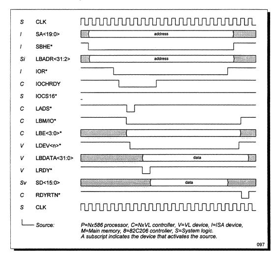
Figure 54 ISA-Master 16-Bit Read from VL-Bus I/O
