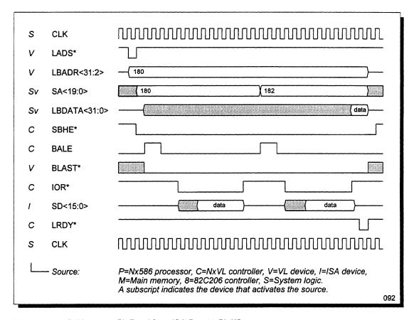
Figure 49 VL-Master 32-Bit Read from ISA-Bus 16-Bit I/O
