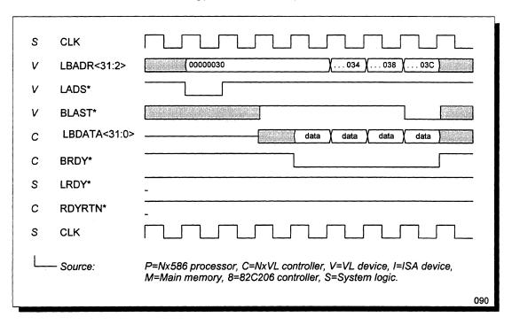
Figure 46 VL-Master 16-Byte Burst Read from Main Memory (Queue Hit)
