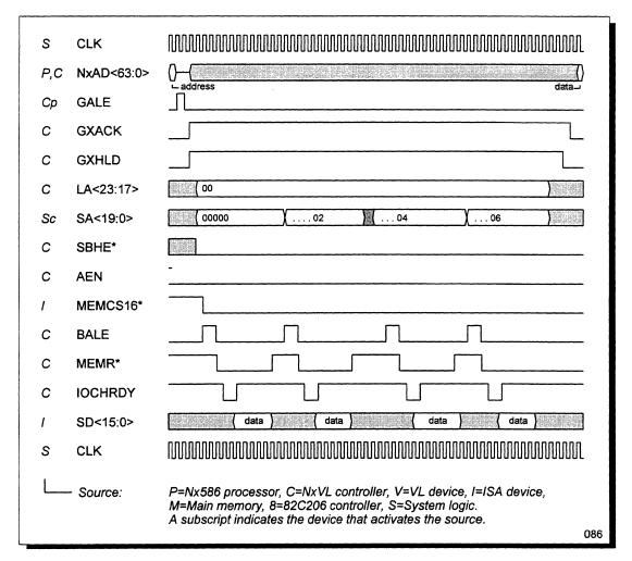
Figure 42 Processor 64-Bit Read from ISA-Bus 16-Bit Memory
