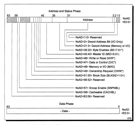
Figure 13 NexBus Address/Status and Data
