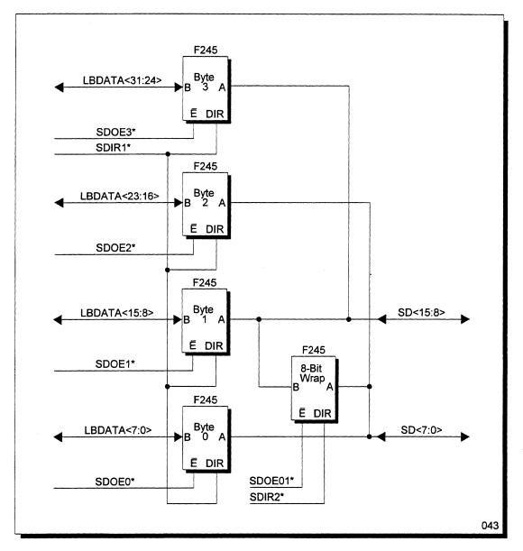
Figure 19 VL-Bus to ISA-Bus Data Transceivers
