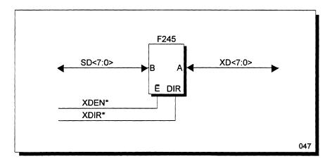
Figure 21 IPC SD-Bus to XD-Bus Data Transceiver
