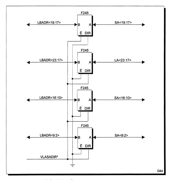
Figure 20 VL-Bus to ISA-Bus Address Transceivers
