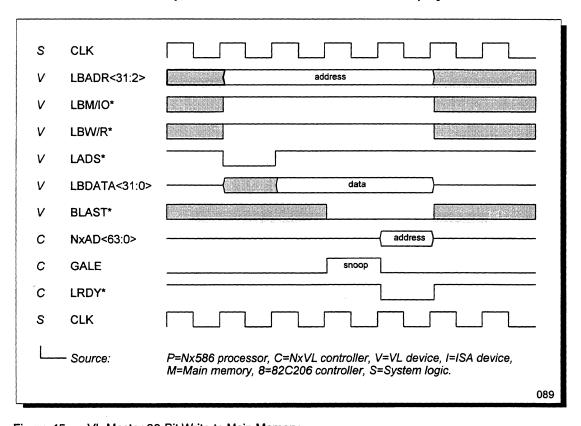
Figure 45 VL-Master 32-Bit Write to Main Memory
