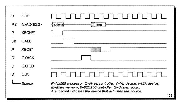
Figure 35 Processor 64-Bit Read from Main Memory (Queue Hit)
