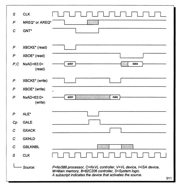
Figure 33 Bus Arbitration, Address, and Data Phase (BUFMODE = 1)
