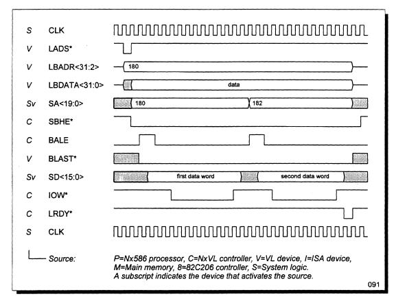
Figure 48 VL-Master 32-Bit Write to ISA-Bus 16-Bit I/O
