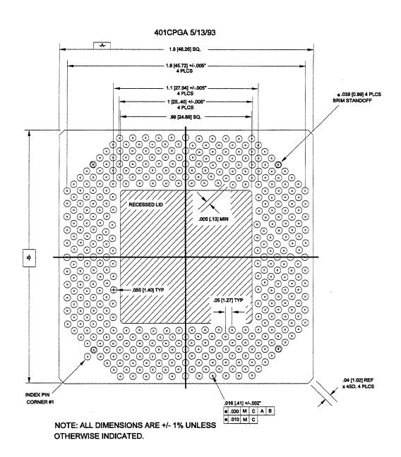
Figure 70 NxVL Package Diagram (bottom)
