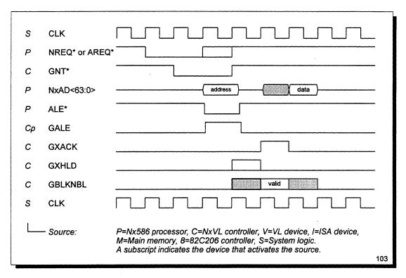
Figure 32 Bus Arbitration, Address, and Data Phase (BUFMODE = 0)
