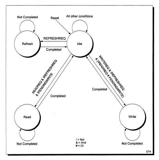
Figure 31 Main-Memory Arbitration State Diagram
