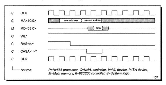
Figure 62 Fast Read from Main Memory (No Precharge)
