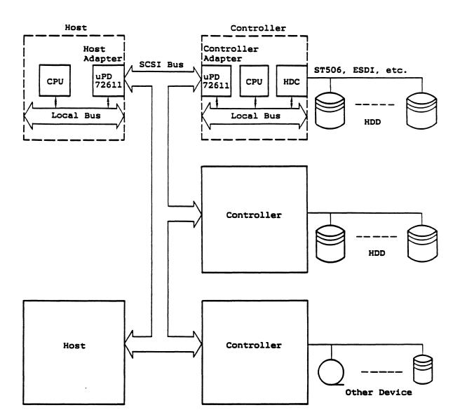
Figure 1-1 System Configuration Example
