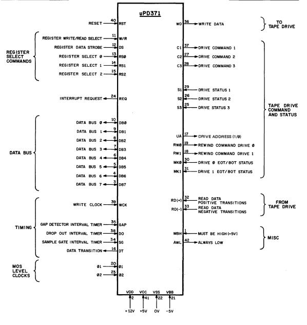
FIGURE 2 INPUT/OUTPUT SIGNALS
