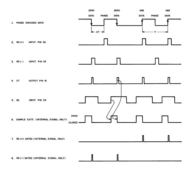
FIGURE 4 SG (SAMPLE GATE) TIMING
