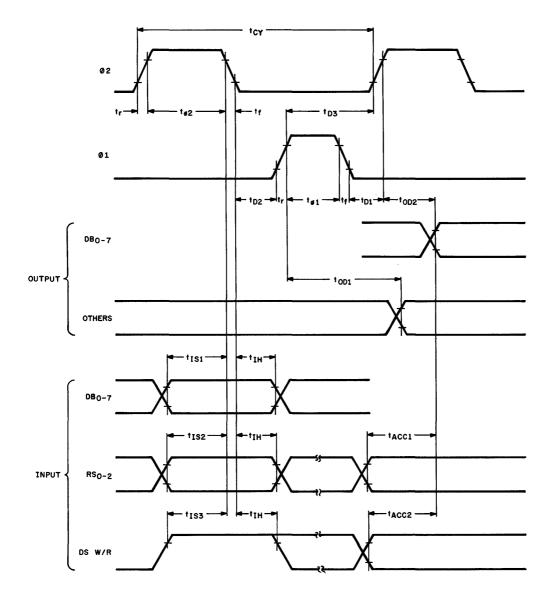
Note: Timing Measurement Levels: Clack High/Low Voltage = 9.0V/0.65V Input High/Low Voltage = 3.0V/0.8V Output High/Low Voltage = 2.0V/0.8V
