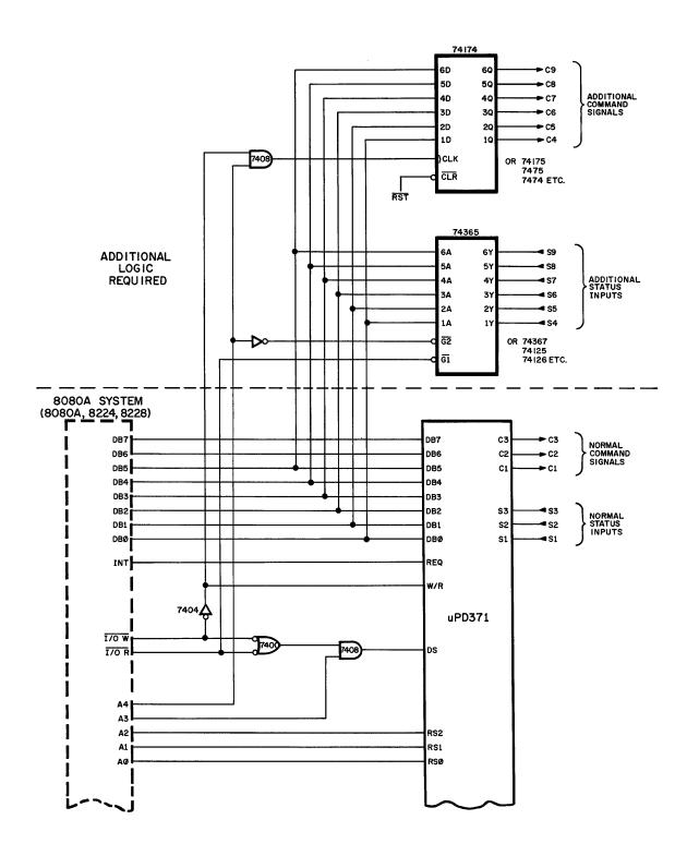
FIGURE 10 ADDITIONAL COMMAND SIGNALS AND STATUS INPUTS FOR COMPLEX DRIVES OR MULTIPLE DRIVE SYSTEMS
