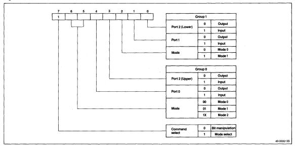
Figure 2. Bit Manipulation Command Word
