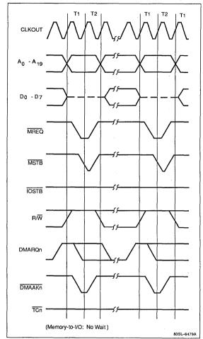
Figure 32. DMA Demand Release Timing
