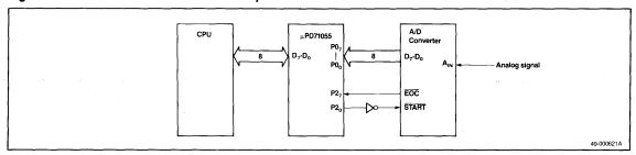
Figure 8. A/D Converter Example
