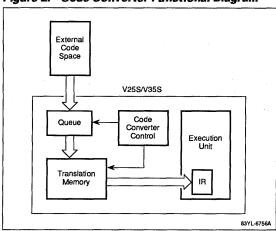
The code converter uses the encrypted opcode from the prefetch queue as an address, and provides the correct V35 opcode as data to the instruction register. An example of this is shown in figure 3. Again, only the first byte of each opcode is decoded, and subsequent bytes are passed directly from the prefetch unit to the execution unit.
