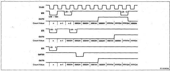
Figure 9. Mode 0 Program Example Timing Chart
