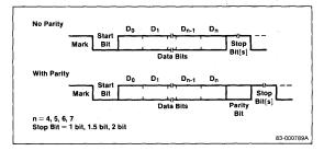
Figure 11. Asynchronous Transmitter Example
