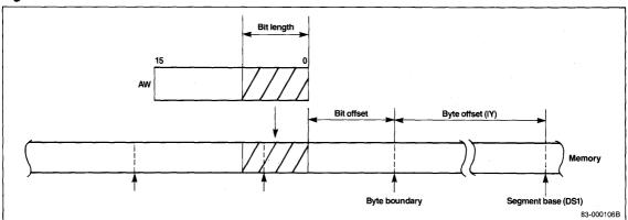
Figure 3. Bit Field Extraction
