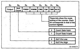
Initial OUT refers to the state of the OUT pin immediately after the mode is set.
