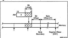
EXT reg8, reg8; EXT reg8, imm4. This instruction loads to the AW registers the bit field data whose bit length is specified by the second operand of the instruction from the memory location that is specified by the DSO segment register (segment base), the IX index register (byte offset), and the lower 4 bits of the first operand (bit offset). See figure 17.
