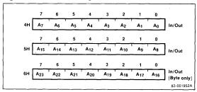
Figure 16. Device Control Register Read/Write Format
