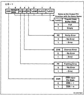
Framing, overrun, and parity errors do not disable the  $\mu$ PD71051's operations. All three error flags are cleared to 0 by a command byte that sets the ECL bit to 1.
