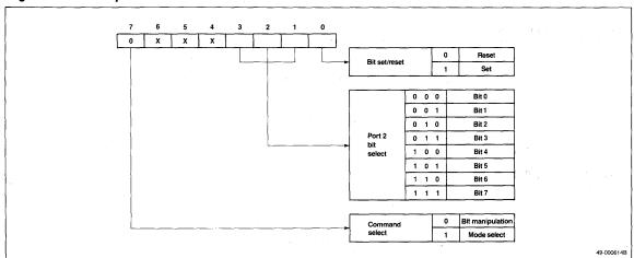
Figure 3. Bit Manipulation Command Example
