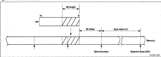
Figure 5. Bit Field Extraction
