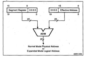
If normal addressing mode is enabled, then this 20-bit result is presented on the address bus during the bus cycle. If expanded addressing mode is enabled, this address is used as a logical address.
