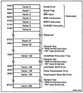
Each interrupt vector consists of four bytes. The two low bytes are loaded into the PC as the offset, and the two high bytes are loaded into the PS as the base address. See figure 42.
