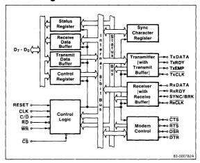
The CPU can read the current status of the  $\mu$ PD71051 and can process data after checking the status, after checking for transfer errors, and  $\mu$ PD71051 data buffer status.
