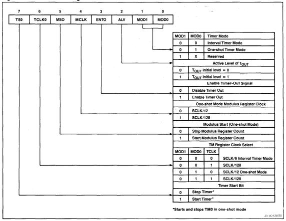
Figure 15. Timer Control Register 1
