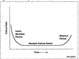
Infant mortality, as the name implies, represents the early-life failures of devices. These failures are usually associated with one or more manufacturing defects.
