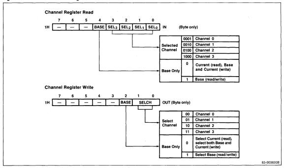
Figure 40. DMA Device Control Register
