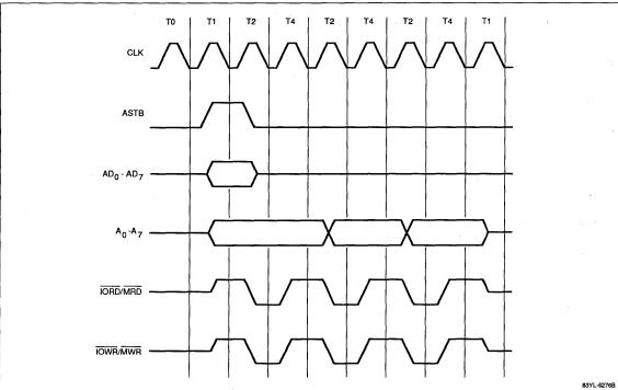
Figure 8. I/O-to-Memory Transfer, Compression Mode Timing
