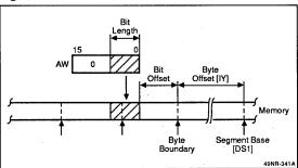
EXT reg8, reg8; EXT reg8, Imm4. This instruction loads to the AW registers the bit field data whose bit length is specified by the second operand of the instruction from the memory location that is specified by the DSO segment register (segment base), the IX index register (byte offset), and the lower 4 bits of the first operand (bit offset). See figure 115.
