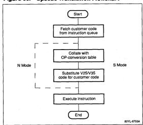
The translation table is user-defined and is inserted into each  $\mu$ PD70327 mask at the factory. The  $\mu$ PD70327 can be dynamically switched from secure mode to normal mode, thus providing an additional measure of security
