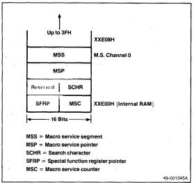
Setting the macro service mode for a given interrupt requires programming the corresponding macro service control register. Each individual interrupt, excluding INTR, NMI and TBC, has its own associated MSC register. See table 6. Format for all MSC registers is shown in figure 12.
