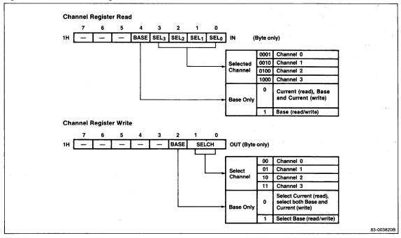
Figure 40. DMA Device Control Register
