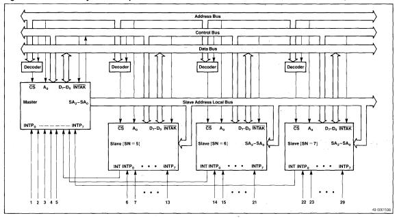
Figure 11. Extended System Example with Three Slaves
