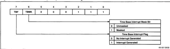
Figure 17. Processor Control Register (PRC)
