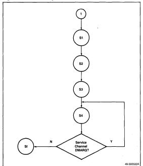
Figure 24. DMA Cycle, Single Mode
