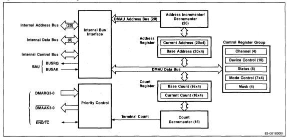
memory-to-I/O transfer, the DMA mode (DMD) register is used to select the transfer directions for each channel and activate the appropriate control signals.
