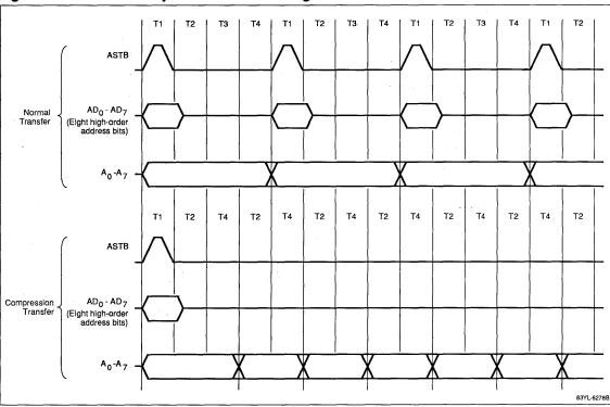
Figure 3. Normal and Compression Transfer Timing
