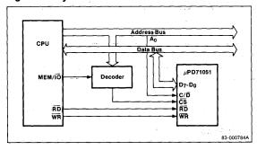
Figure 3. μPD71051 Operating Procedure
