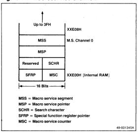
Setting the macroservice mode requires programming the corresponding macroservice control register. Each individual interrupt, excluding INT, NMI, serial error, DMA, and TBC, has its own associated register. Figure 13 shows the generic format for all MSC registers.
