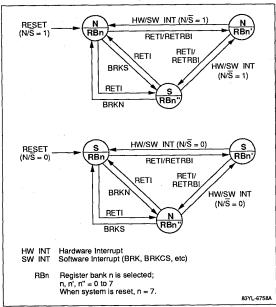
Software control of the operating mode is performed by the BRKS (Break for Secure Operation) and the BRKN (Break for Normal Operation) instructions. These opcodes are undefined codes on the standard V35 and should not be ported to standard V35 processor environments. These instructions are detailed in the instruction set section.
