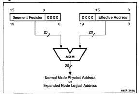
If normal addressing mode is enabled, this 20-bit result is presented on the address bus during the bus cycle. If expanded addressing mode is enabled, this address is used as a logical address.
