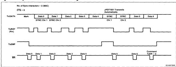
Figure 17. Issuing a Command During SYNC Character Transmission
