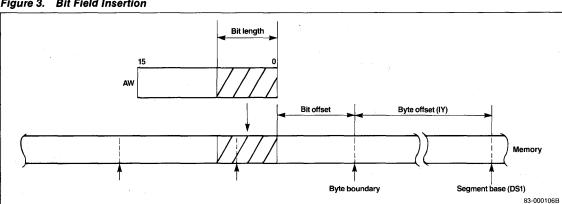
Figure 3. Bit Field Insertion
