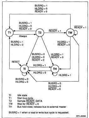
Address and bus status are output after the leading edge of T1 and are maintained until after the cycle is completed. A strobe, BCYST, is asserted during T1 to indicate the beginning of a bus cycle. BCYST is output following the leading edge of T1 and is deasserted after the leading edge of T2.
