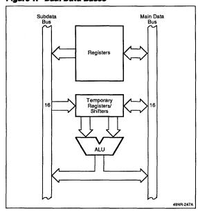
Register File. There are 12 registers in the internal RAM. Four are temporary registers used in the execution of certain instructions (LC, TA, TB, TC). The other eight are general-purpose registers (AW, BW, CW, DW, IX, IY, BP, SP) and either contain operand data or point to operand data in memory.
