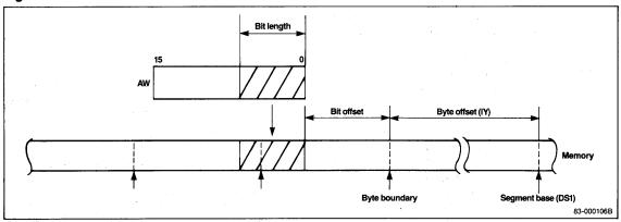
Figure 4. Bit Field Extraction
