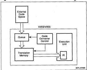
The code converter uses the encrypted opcode from the prefetch queue as an address, and provides the correct V25 opcode as data to the instruction register. An example of this is shown in figure 32. Again, only the first byte of each opcode is decoded, and subsequent bytes are passed directly from the prefetch unit to the execution unit.
