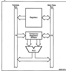
Register File. There are 12 registers in the internal RAM. Four are temporary registers used in the execution of certain instructions (LC, TA, TB, and TC). The other eight
