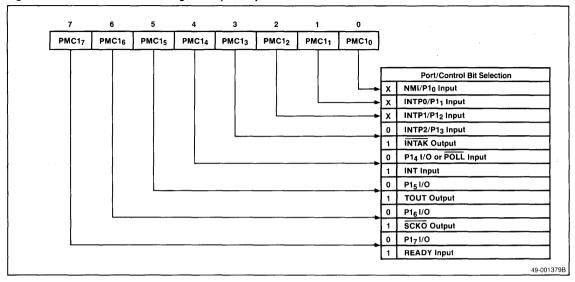
Figure 31. Port Mode Control Register 2 (PMC2)
