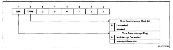
Figure 17. Processor Control Register (PRC)
