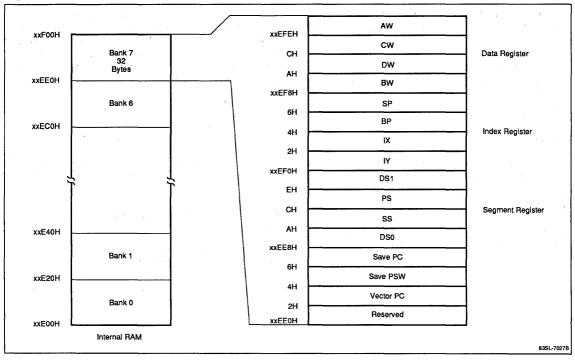
Figure 1. µPD70327 Internal RAM Register Mapping
