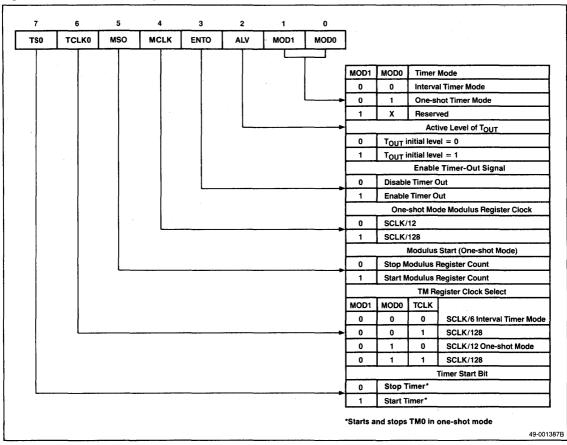
Figure 15. Timer Control Register 1
