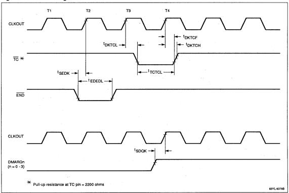
Figure 25. DMA Timing 3; Cascade Mode (Normal Operation)
