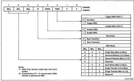
Figure 26. DMA Address Control Registers (DMAC)
