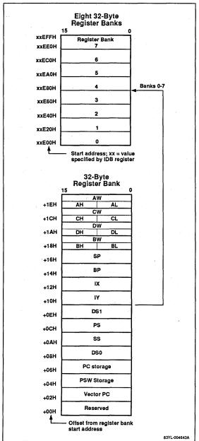
Pointers (SP, BP) and Index Registers (IX, IY). These registers are used as 16-bit base pointers or index registers in based addressing, indexed addressing, and based-indexed addressing. The registers are used as default registers under the following conditions:
