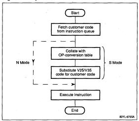
The user-defined translation table is inserted into each  $\mu$ PD70337 mask at the factory. The  $\mu$ PD70337 can be dynamically switched from secure mode to normal mode, thus providing an additional measure of security as well as compatibility with existing ROM versions of V35 software. Note, however, that the V35 Software Guard does not support internal ROM.
