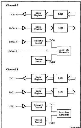
In addition to the asynchronous mode, channel 0 has a synchronous I/O interface mode. In this mode, each bit of data transferred is synchronized to a serial clock  $\overline{\text{SCKO}}$ . This is the same as the NEC  $\mu$ COM75 and  $\mu$ COM87 series, and allows easy interfacing to these devices.
