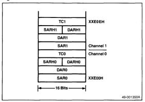
Figure 25. DMA Mode Registers (DMAM)
