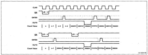
Mode 5: Hardware-Triggered Strobe [Retriggerable]. Mode 5 is similar to mode 4 except that operation is triggered by the GATE input and can be retriggered. See table 10 and figure 17.
