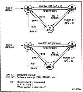
Software control of the operating mode is performed by the BRKS (Break for Secure Operation) and the BRKN (Break for Normal Operation) instructions. These opcodes are undefined codes on the standard V25, and should not be ported to standard V25 processor environments. These instructions are detailed in the instruction set section.
