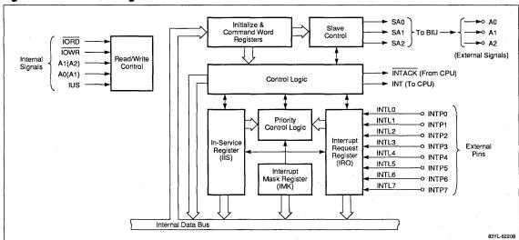
To reduce current drain in the standby modes, the V53 does not have internal pullup resistors on the INTP0-INTP7 pins. This is different from the µPD71059 and V40/V50.
