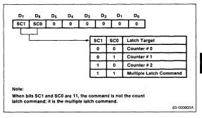
Figure 5. Control Register Format for Multiple Latch Command
