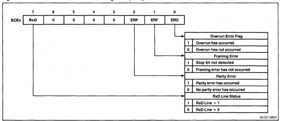
Figure 23. Serial Communication Control Register (SCC)
