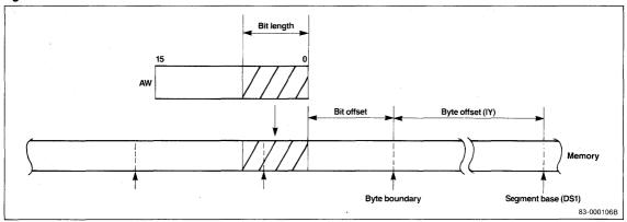
Figure 5. Bit Field Extraction.
