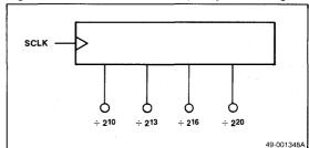
Figure 16. Time Base Interrupt Request Control Register
