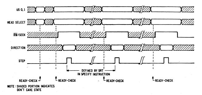
FIGURE 10 TIMING AT FDD INTERFACE SEEK AND RECALIBRATE INSTRUCTION
