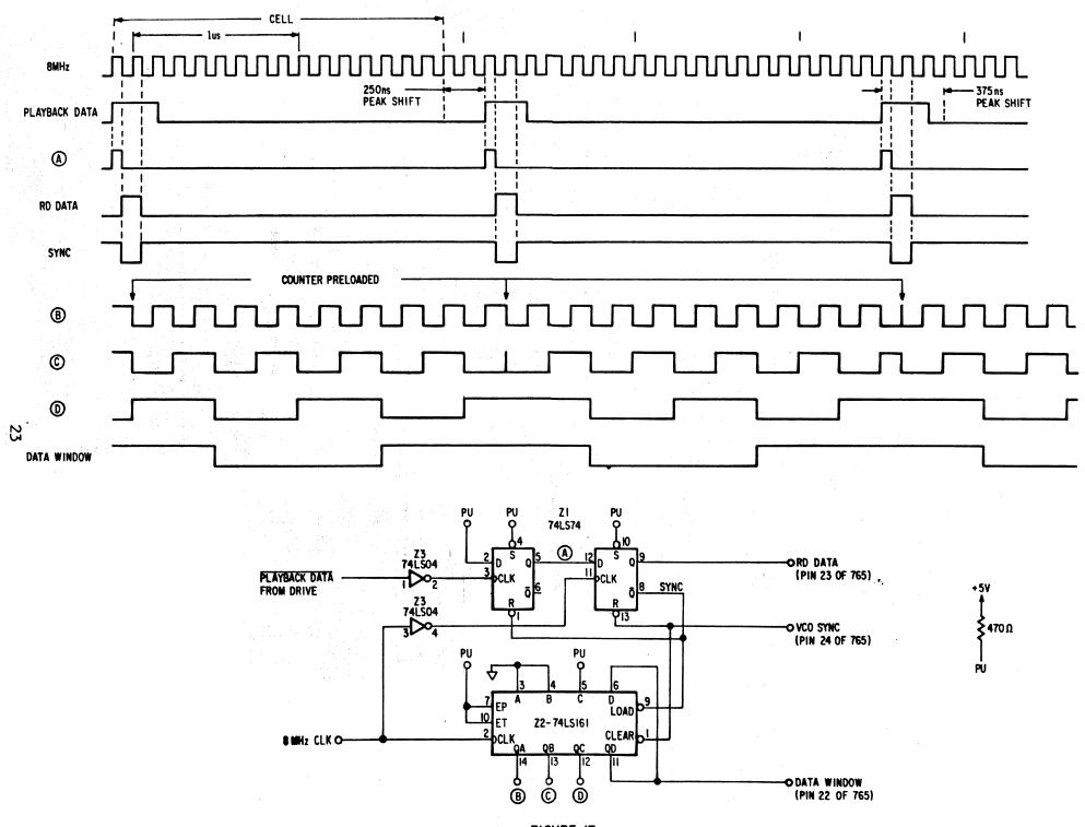
FIGURE 17 SYNCRONOUS COUNTER DATA RECOVERY CIRCUIT
