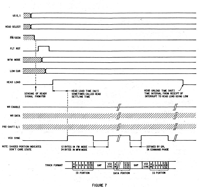
TIMING AT FDD INTERFACE READ DATA, READ DELETED DATA, READ A TRACK, SCAN, AND READ ID INSTRUCTIONS
