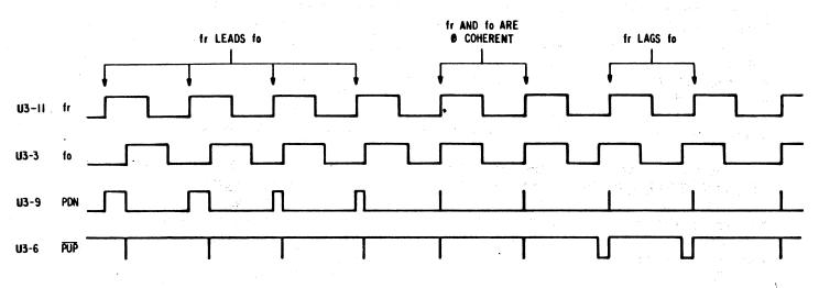
NOTE: PDN CONTROLS Q1, AND PUP CONTROLS Q2, WHICH DISCHARGE AND CHARGE CAPACTOR C1. RESISTOR CAPACTOR NETWORK R4, R7, R8 AND C1 CHANGE THE PULSE WIDTH MODULATED SIGNALS PDN AND PUP (WHICH ARE A DIRECT FUNCTION OF PHASE DIFFERENCES BETWEEN fr AND f0), INTO A D.C. LEVEL, AS SEEN AT US-2. THE LEVEL AT US-2 IS NORMINALLY -3.25V.
