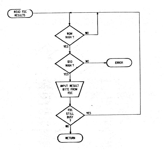
FIGURE 22 DETAIL RESULT PHASE FLOW CHART
