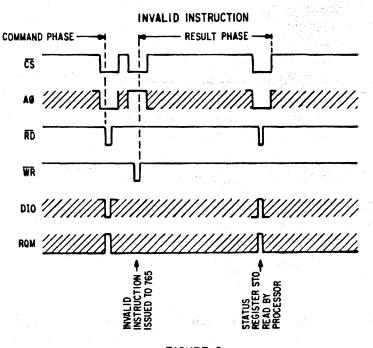
FIGURE 6 SEEK, RECALIBRATE, SENSE INTERRUPT STATUS AND INVALID INSTRUCTIONS
