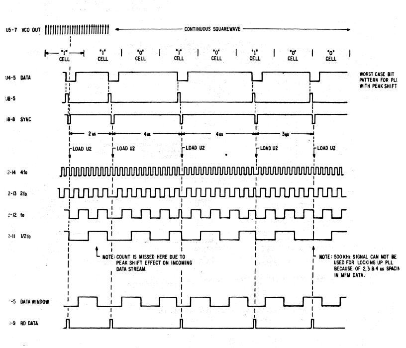
FIGURE 15 fo COUNTER SYNC WITH PEAK SHIFT
