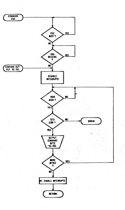
FIGURE 20 DETAIL COMMAND PHASE FLOW CHART
