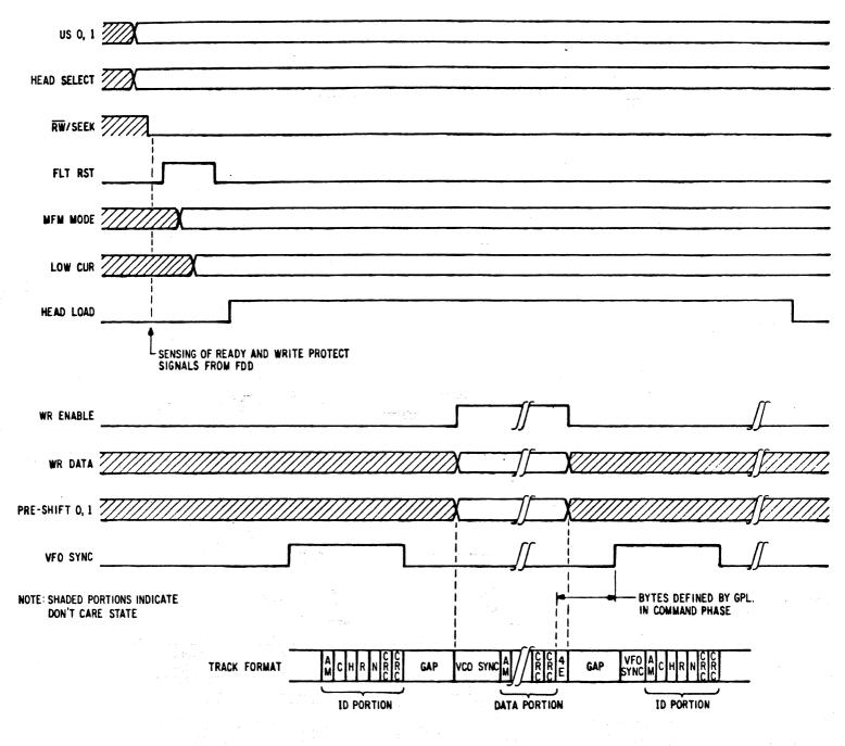
FIGURE 8 TIMING AT FDD INTERFACE WRITE DATA AND WRITE DELETED DATA INSTRUCTIONS
