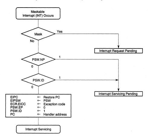
Figure 6-1 Maskable Interrupt Servicing Format
