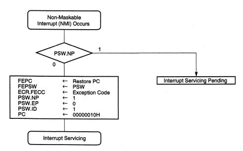
Figure 6-2 Non-maskable Interrupt Servicing Format
