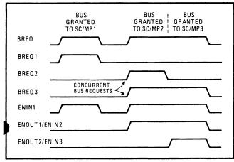
**4. Bus access.** The SC/MPs are connected in a priority arrangement for access to the common bus. SC/MP 1 has the highest priority, and even if SC/MP 3 has a concurrent request with SC/MP 2, it must wait until SC/MP 2 completes its operations.
