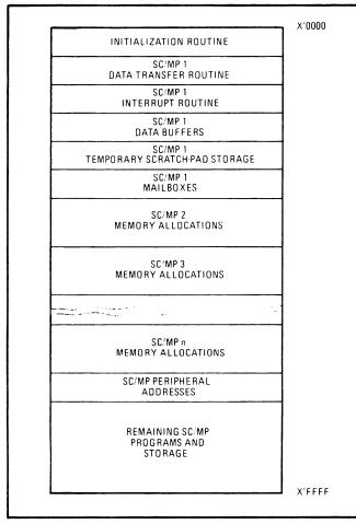
**2. Memory organization.** A common memory is used for all SC/MPs in the system. When a SC/MP requires service, it places a request in the mailbox, which is polled by the controlling device (which takes the most of the memory, since it has supervisory tasks.)
