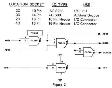
3. Wire the sockets as shown in figures 2 and 3, using the wire list in figure 4.
