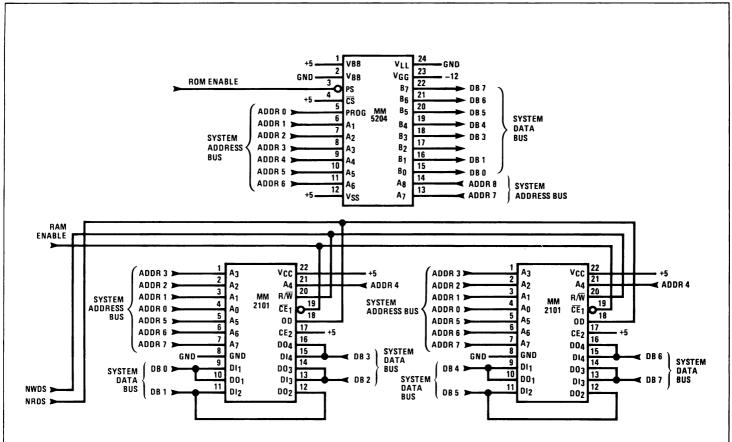
Figure 4. ROM/RAM Interconnection's Between SC/MP and Cassette Tape Recorder
