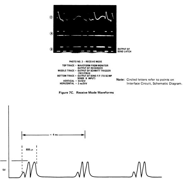
Figure 7D. Waveform at Point E of Interface Circuit
