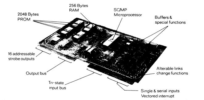
Physical Characteristics: Epoxy glass Printed Circuit Board,
