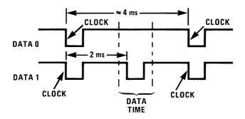
Figure 5. Data Output from Decoder
