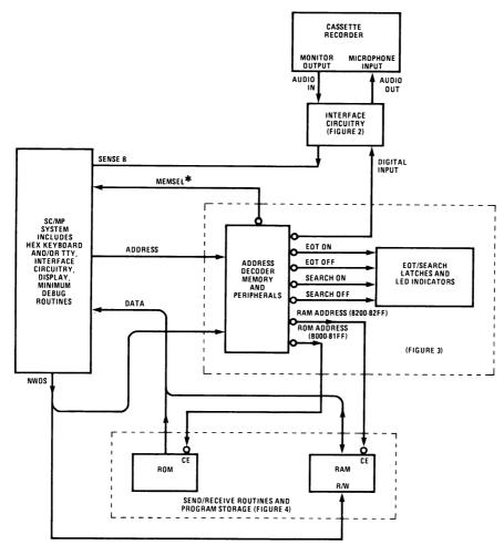
Figure 1. SC/MP-to-Cassette System Block Diagram
