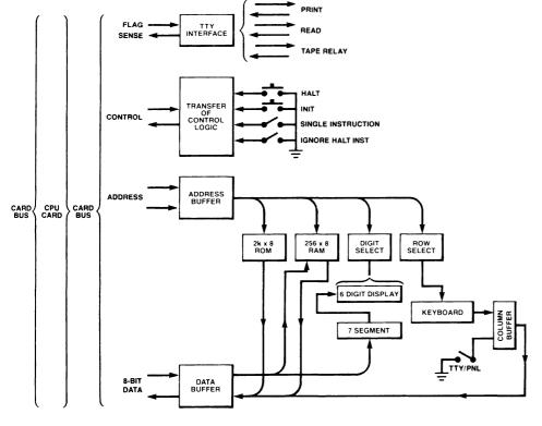
Figure 1: BLOCK DIAGRAM FOR MOTHERBOARD
