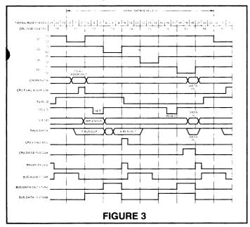
Figure 3 shows a timing diagram for the CPU, and for reference purposes, some of the bus timing signals. The most basic CPU timing signals are the 4-phase non-overlapping clocks. These are PMOS logic levels (0=+5, 1=-12) applied to all 5 IMP chips. The odd-numbered CPU states (T1, T3, T5,
