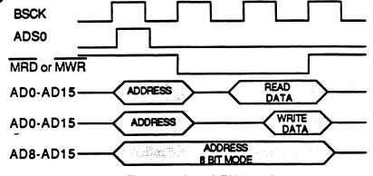
Figure 5 Local DMA cycle
