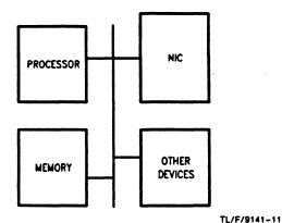
FIGURE 10. Single Bus Configuration
