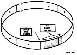
FIGURE 6. Packet Rejection
