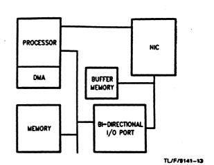
FIGURE 12. DPM Equivalent Configuration
