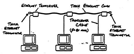
The network is constructed by first connecting two lengths of thick Ethernet coax together with an Ethernet transceiver box. Transceiver boxes are also added at each end of the coax. A terminator must be added to the ends of the thick Ethernet segment as depicted below.
