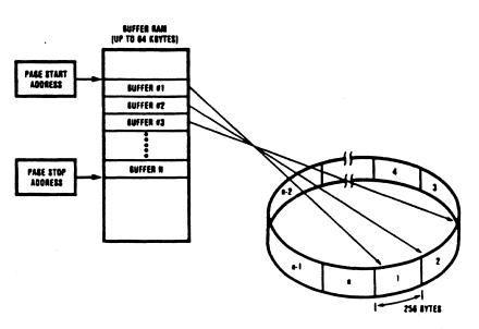
**FIGURE 4. The Receive Buffer**
