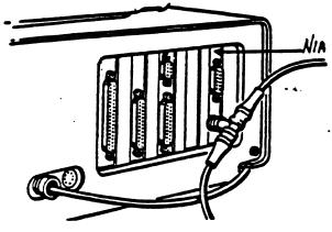
Finally the connection to the NIA board is made with the BNC-T as shown below.
