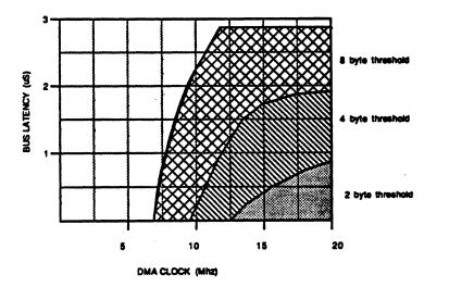
Figure 6 FIFO Threshold for Byte Mode
