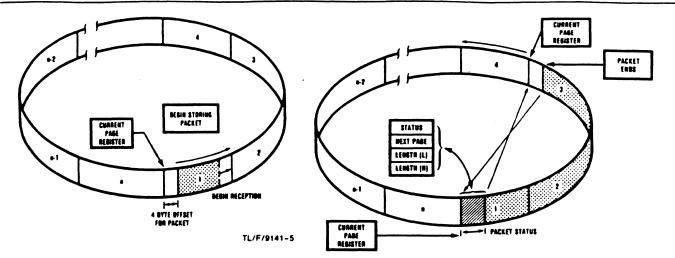
FIGURE 5. Receive Packet Buffering
