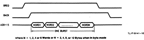
FIGURE 8. Local DMA Burst
