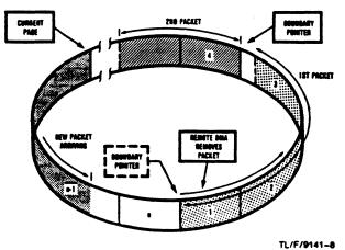
FIGURE 7. Removing Packets From Receive Buffer Ring
