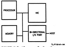
**FIGURE 13. Dual Processor Configuration**
