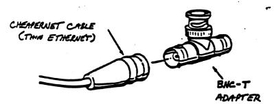
At each end of the network a BNC-T adapter and terminator are connected as depicted below.
