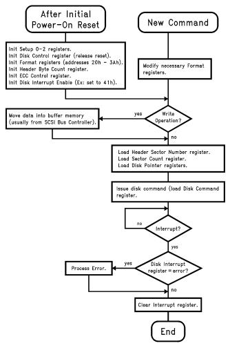
FIGURE 4.6. Software Flowchart for Simple Disk Operations
