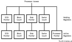
FIGURE 4.1. Holding and Active Registers
