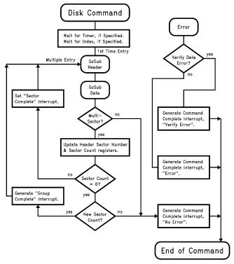
FIGURE 4.3. Disk Command Flowchart
