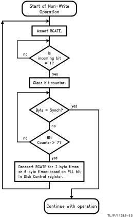
FIGURE 4.8. RGATE Operation during Search for Synch
