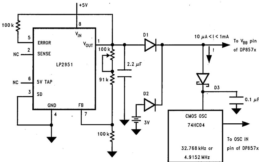
FIGURE 1. Voltage Regulator as a  $V_{CC}$  Supply for an External Oscillator
