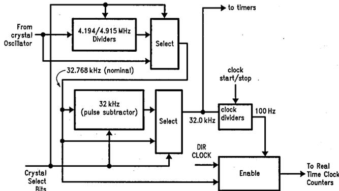
FIGURE 2. Clock Prescaler (with Test Bit)
