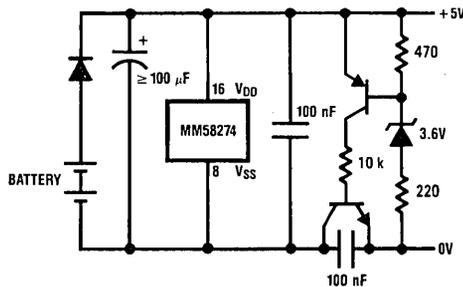
FIGURE 5. Simplified Power Supply Diagram with 100  $\mu$ F Capacitor Added
