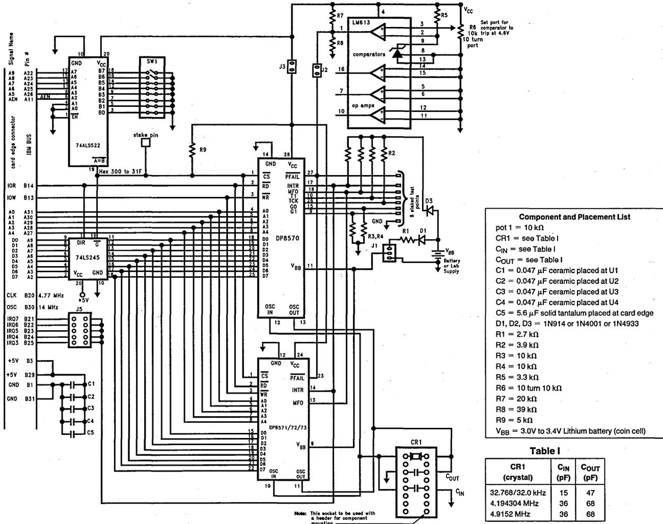
FIGURE 3. General Purpose Interface to IBM PC-XT or PC-AT for Experiments
