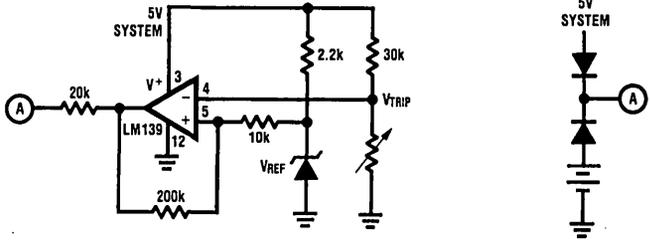
**FIGURE 18. Sensing D.C. Failure Using a Comparator**
