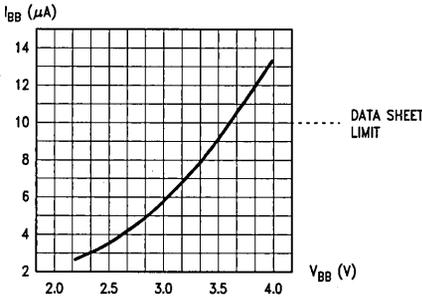
**FIGURE 3a. Standby Current against Battery Voltage  $T = 25^\circ C$  (32.768 kHz)**
