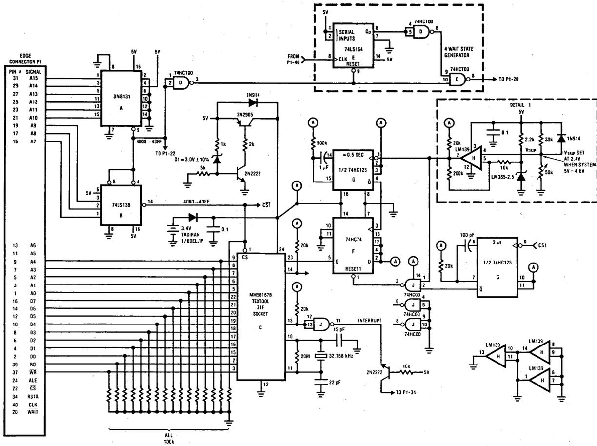
FIGURE 20. Detailed Schematic of Power Down Circuitry, and Interface to NSC888 Board
