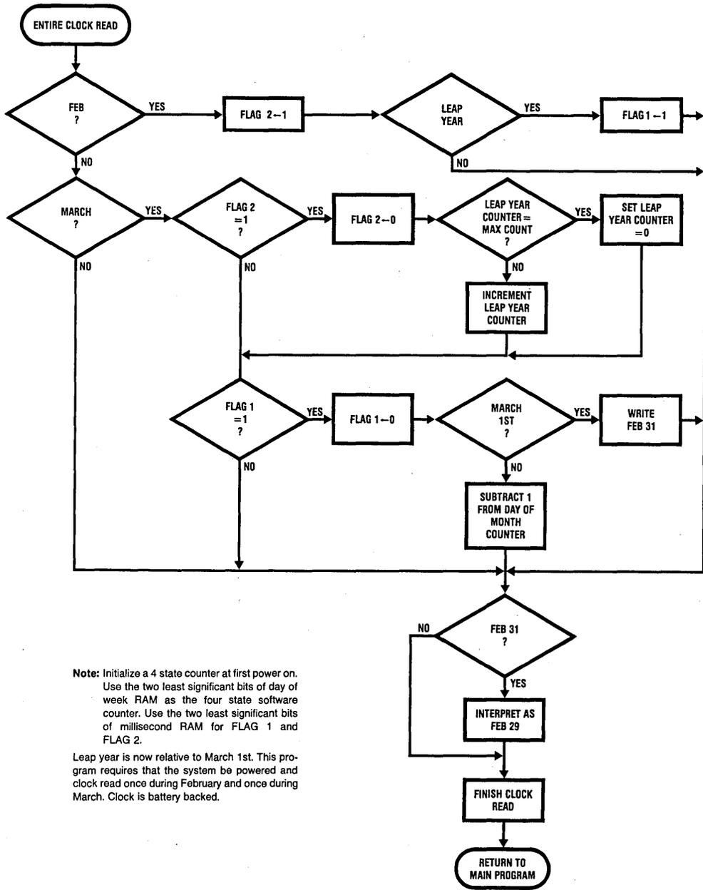
**Note:** Initialize a 4 state counter at first power on. Use the two least significant bits of day of week RAM as the four state software counter. Use the two least significant bits of millisecond RAM for FLAG 1 and FLAG 2.
