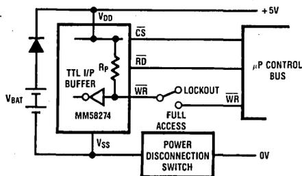
FIGURE 14. Write Protection by Manually Switching WR
