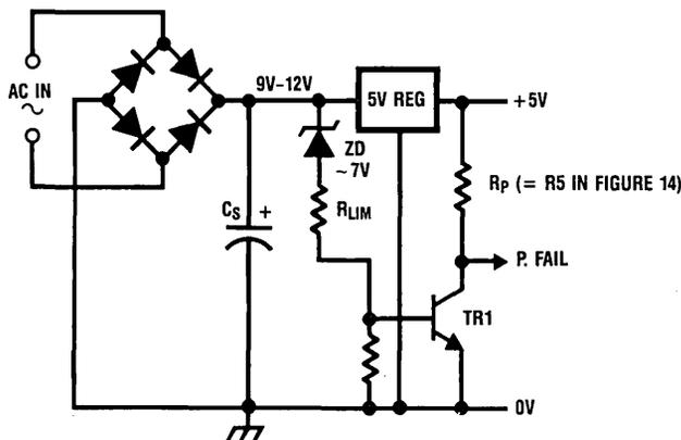
FIGURE 17. Power Fail Signal Generation from Unregulated Supplies
