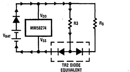
$R_S$  = System Resistance with No Power Applied
