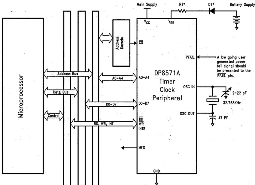
\*These components may be necessary to meet UL requirements for lithium batteries. Consult battery manufacturer.
