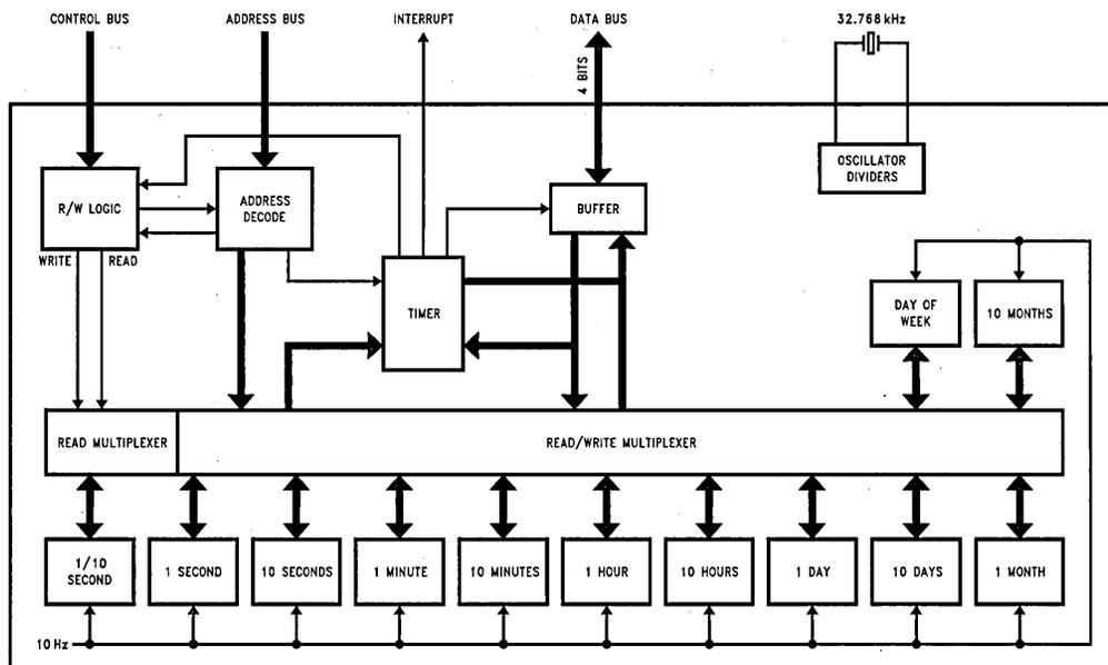
FIGURE 1. Block Diagram
