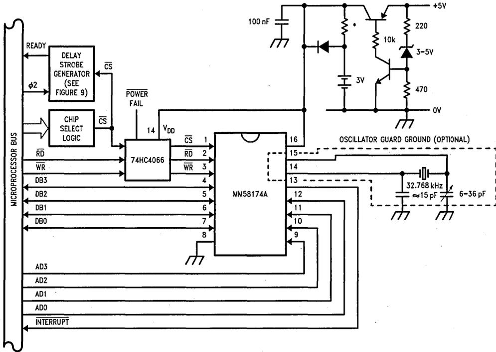
\*Use resistor with Ni-Cad cells only.
