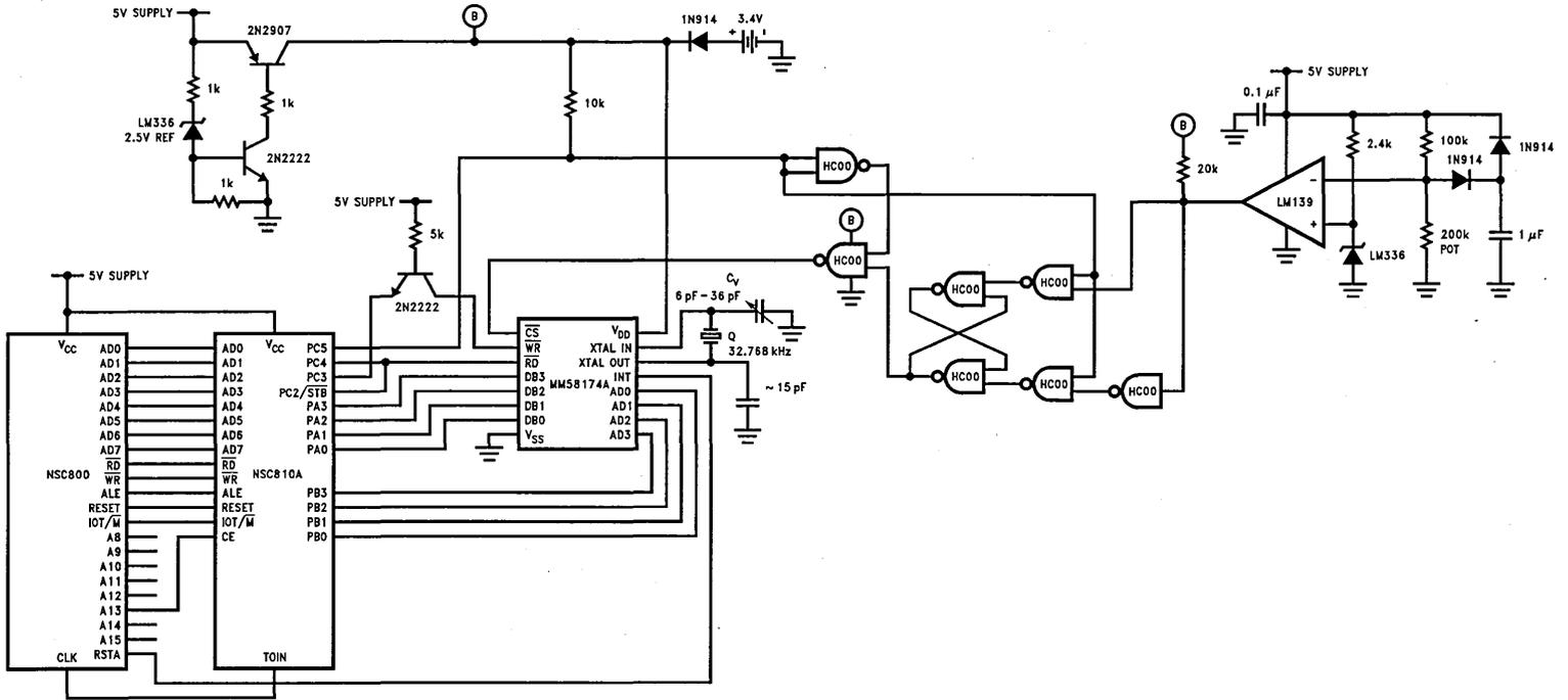
FIGURE 4. Real Time Clock Interface to NSC800™ and NSC810A without Wait States
