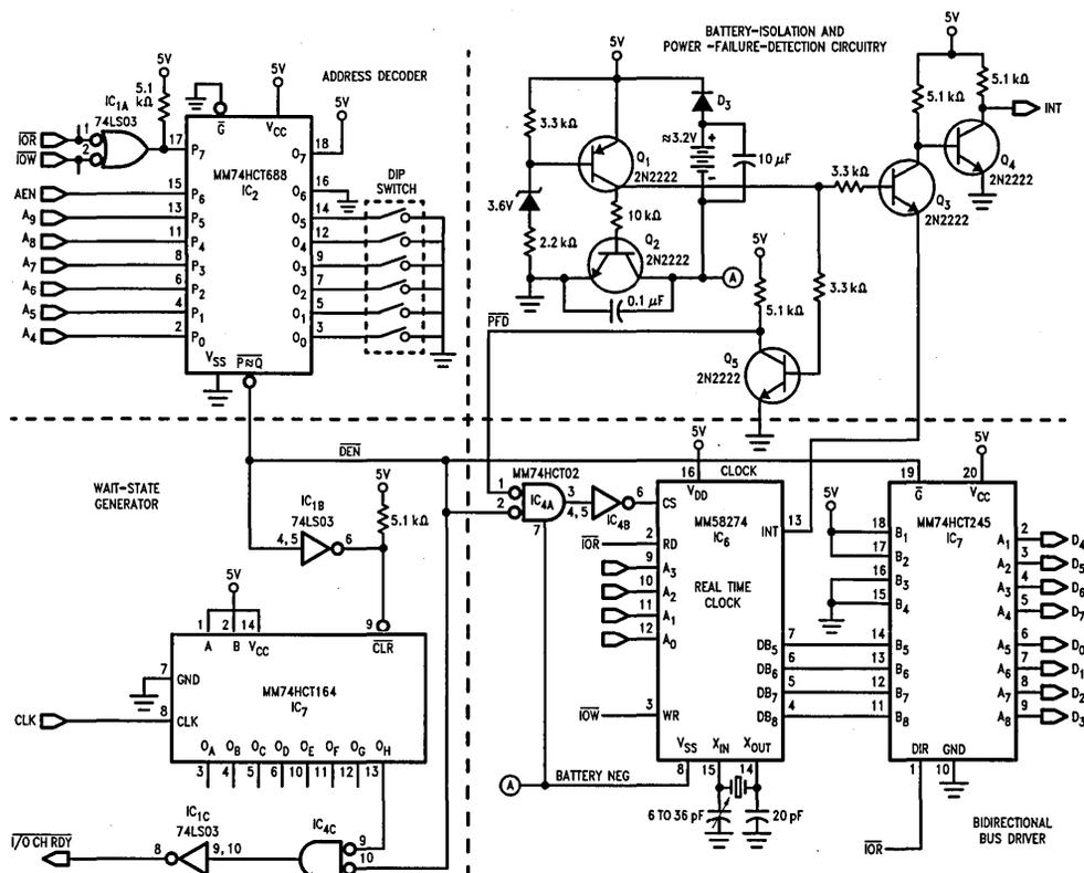
FIGURE 4. The MM58274 requires relatively few support chips: Adding a bidirectional bus driver, a wait-state generator, and an address decoder lets you implement all essential functions of the MM58274.
