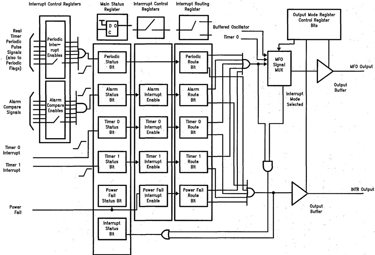
FIGURE 5. Interrupt Control Logic Overview
