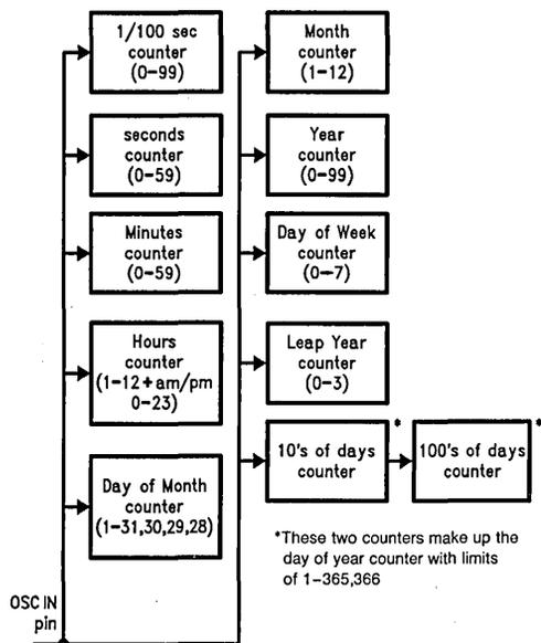
**FIGURE 3. Real Time Counters, Test Mode Configuration**
