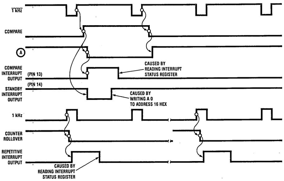
FIGURE 10. Internal Interrupt Timing
