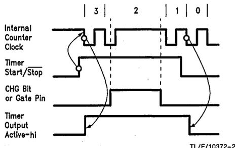
FIGURE 2. Mode 0—Single Pulse Generator
