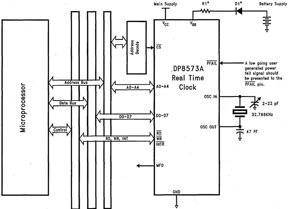
\*These components may be necessary to meet UL requirements for lithium batteries. Consult battery manufacturer.
