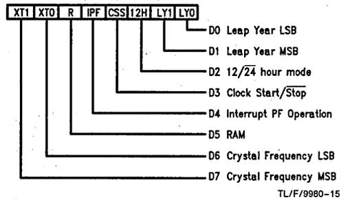
**D0-D1:** These are the leap year counter bits. These bits are written to set the number of years from the previous leap year. The leap year counter increments on December 31st and it internally enables the February 29th counter state. This method of setting the leap year allows leap year to occur whenever the user wishes to, thus providing flexibility in implementing Japanese leap year function.
