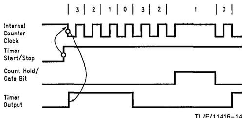
FIGURE 10. Timing Waveforms for Timer Mode 2
