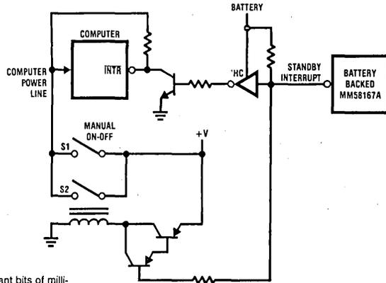
FIGURE 7B. Leap Year Flow Chart and Hardware
