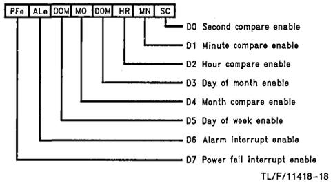
**D0-D5:** Each of these bits are enable bits which will enable a comparison between an individual clock counter and its associated compare RAM. If any bit is a zero then that clock-RAM comparator is set to the "always equal" state and the associated TIME COMPARE RAM byte can be used as general purpose RAM. However, to ensure that an alarm interrupt is not generated at bit D3 of the Main Status Register, all bits must be written to a logic zero.
