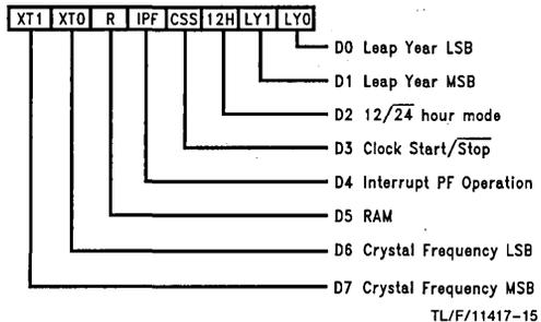
**D0-D1:** These are the leap year counter bits. These bits are written to set the number of years from the previous leap year. The leap year counter increments on December 31st and it internally enables the February 29th counter state. This method of setting the leap year allows leap year to occur whenever the user wishes to, thus providing flexibility in implementing Japanese leap year function.
