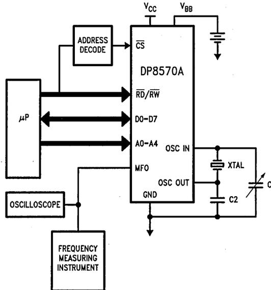
FIGURE 2. Calibration Setup
