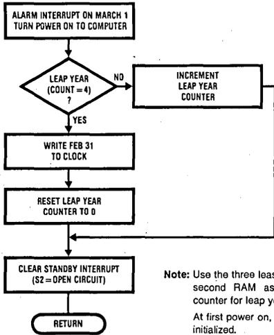
Note: Use the three least significant bits of milli-second RAM as a five-state software counter for leap year.
