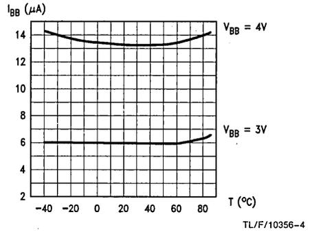
**FIGURE 3b. Standby Current against Temperature (32.768 kHz)**
