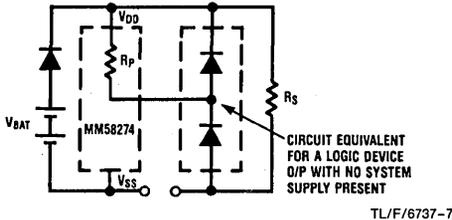
**b)  $V_{SS}$  Disconnection**
