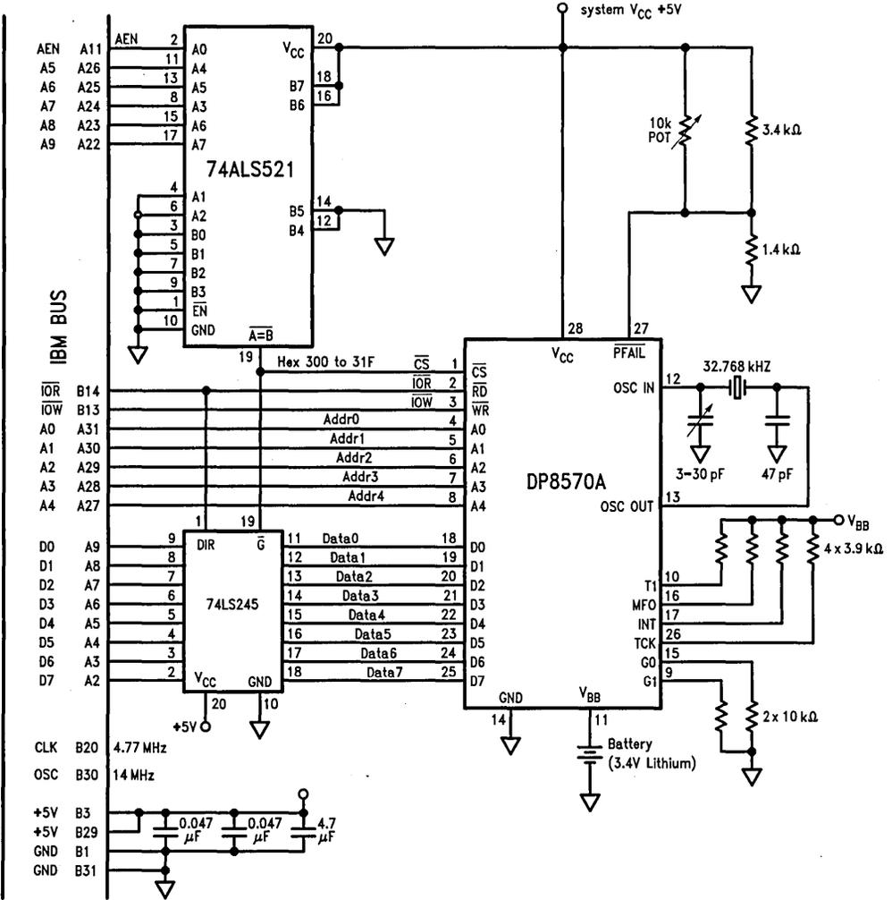
FIGURE 1. DP8570A Timer Clock Peripheral Interface to IBM/XT
