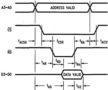
FIGURE 6. Read Cycle Waveforms
