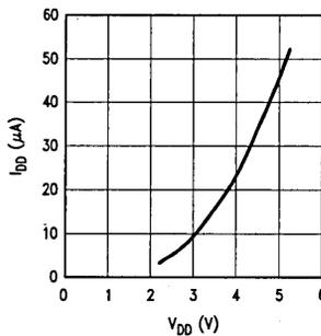
FIGURE 8. Typical Supply Current vs Supply Voltage during Power Down
