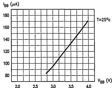
**FIGURE 3d. Standby Current against Battery Voltage (4.194304 MHz)**
