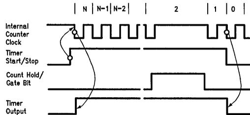
FIGURE 8. Typical Waveforms for Timer Mode 0 (Timer Output Programmed Active High)
