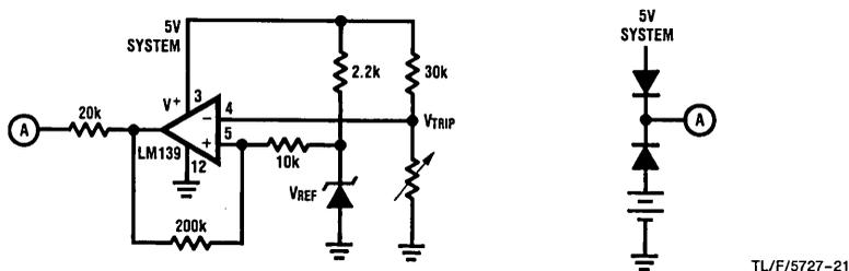
FIGURE 18. Sensing D.C. Failure Using a Comparator
