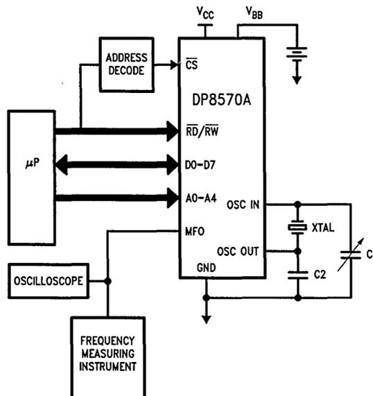
FIGURE 2. Calibration Setup
