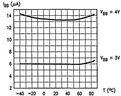
**FIGURE 3b. Standby Current against Temperature (32.768 kHz)**
