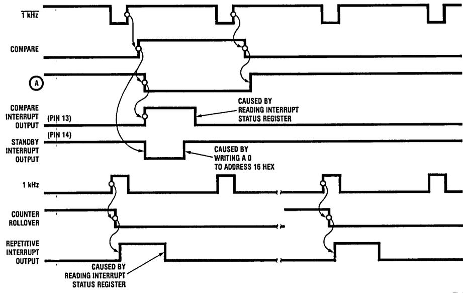
FIGURE 10. Internal Interrupt Timing
