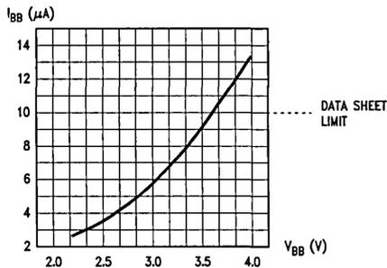
**FIGURE 3a. Standby Current against Battery Voltage T = 25°C (32.768 kHz)**
