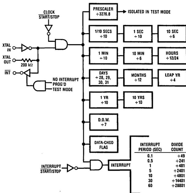
FIGURE 20. Test Mode Interconnection Diagram of Internal Counter Stages
