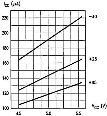
**FIGURE 3c. Operating Current against Supply Voltage (32.768 kHz)**
