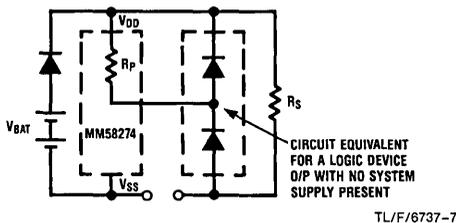
**b)  $V_{SS}$  Disconnection**
