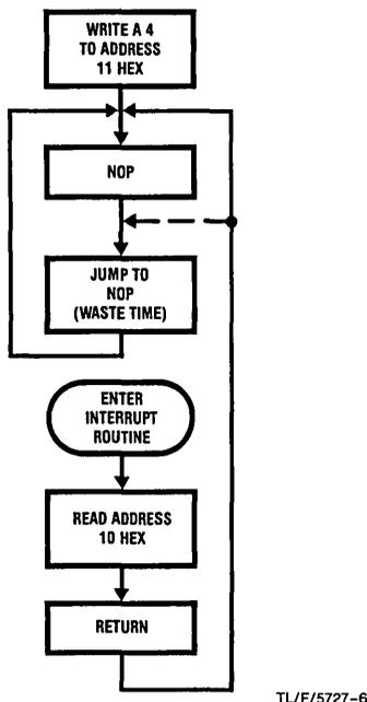
**FIGURE 5. Flow Chart for Calibration
