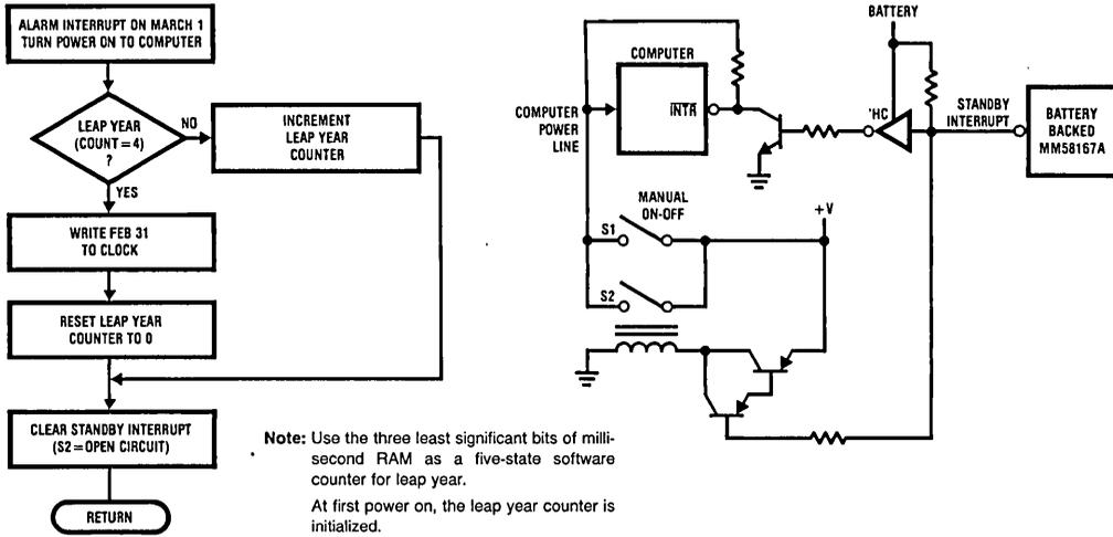
FIGURE 7B. Leap Year Flow Chart and Hardware
