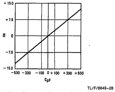
**FIGURE 10. Change in Propagation Delay relative to "true" (application) load minus AC specified data sheet load**
