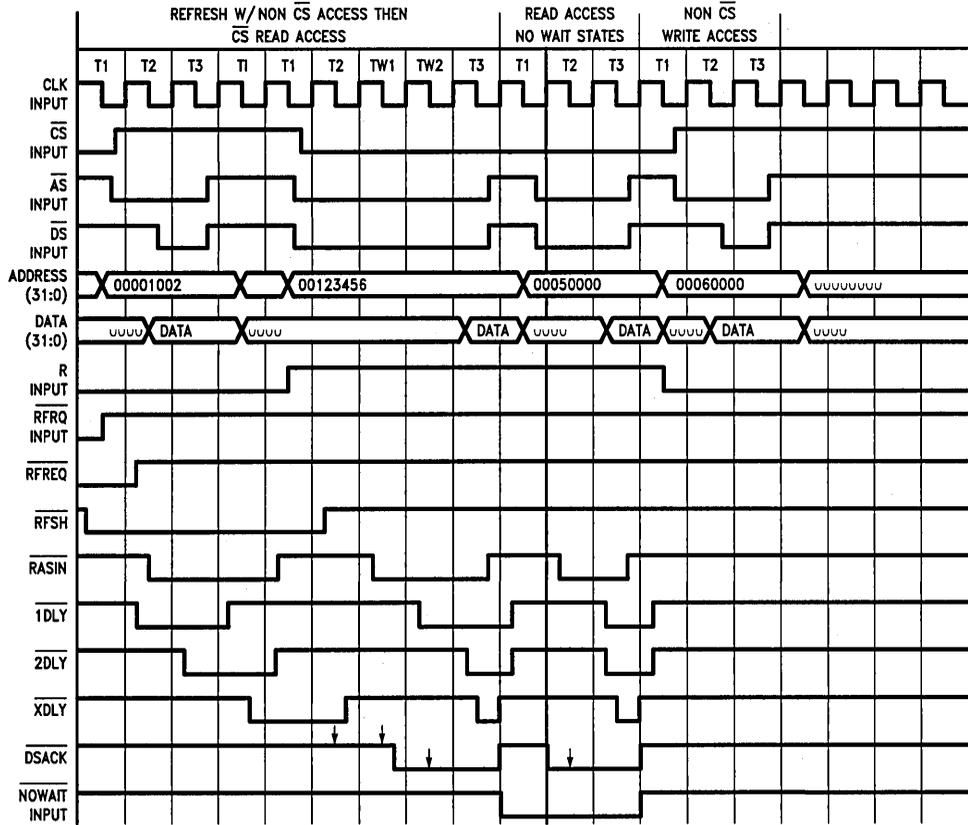
FIGURE 11. System Timing
