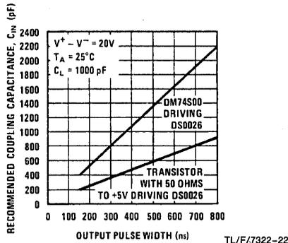
FIGURE 22. Suggested Input Capacitance vs Output Pulse Width
