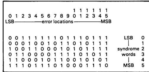
**Fig 5 Check bit generator for data words. Code used is that implemented in National Semiconductor's DP8400 ECC device**
