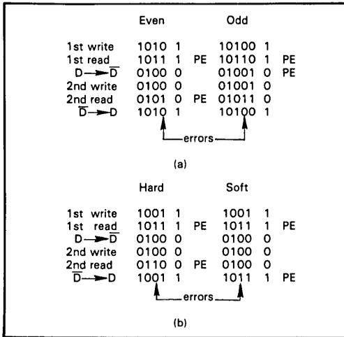
**Fig 3 Even/odd word and hard/soft parity errors. Data words with even number of bits do not yield parity error on second read (a), nor soft error (b). Hard error, however, will be corrected**
