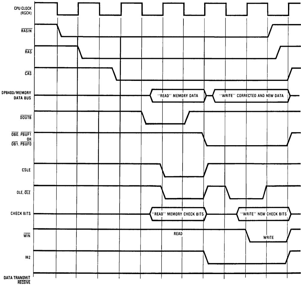
FIGURE 14b. DP8400-2 16-Bit Configuration, Byte Write Timing
