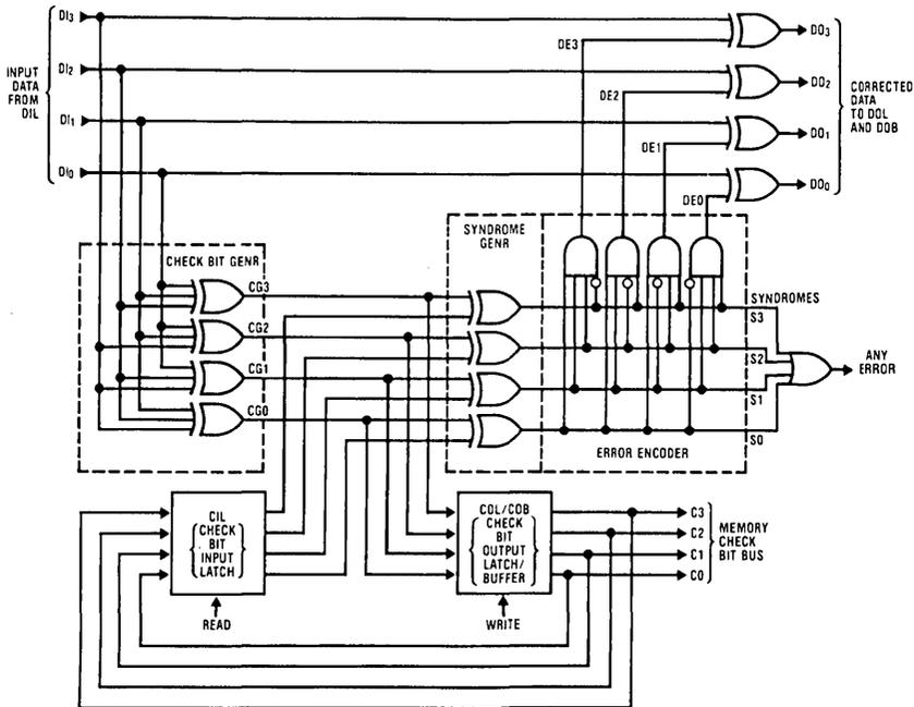
FIGURE 1a. Error Correction 4-Bit Functional Diagram
