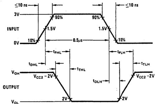
**Note 1:** The pulse generator has the following characteristics: PRR = 1 MHz,  $Z_{OUT} = 58\Omega$ .
