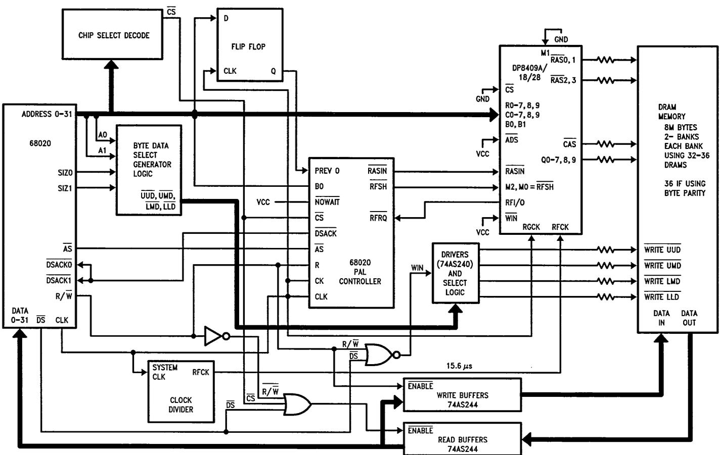
FIGURE 1. 68020 System Diagram for PAL # 1
