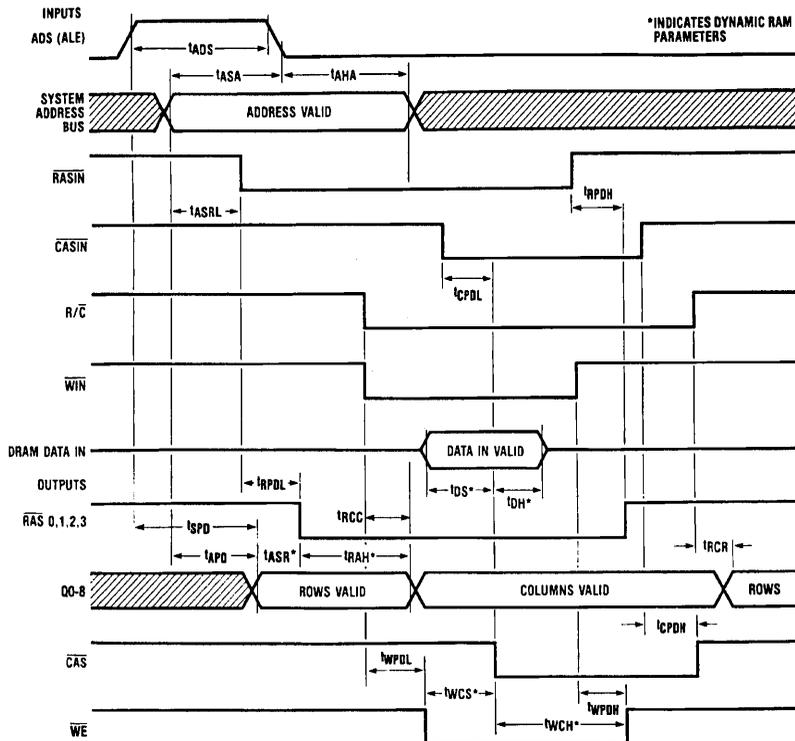
**FIGURE 5b. Write Cycle Timing (Mode 4)**
