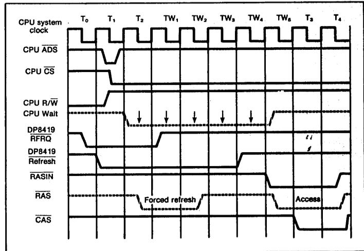
5. If the CPU in Fig. 3 requests a memory read cycle during a forced refresh cycle, the PAL senses the access request. It then adds wait states (TW<sub>x</sub>) to the CPU access cycle (upper dotted line) until the forced refresh has ended and the RAM's RAS precharge specification has been met (lower dotted line).
