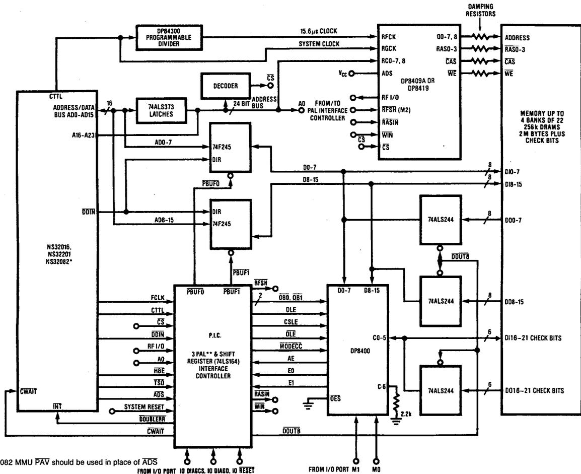
IF system contains NS32082 MMU  $\overline{FAV}$  should be used in place of  $\overline{ADS}$
