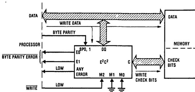
FIGURE 2a. Normal WRITE Mode with E<sup>2</sup>C<sup>2</sup>
