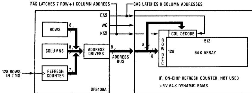
ONLY LS 7 BITS OF REFRESH COUNTER USED FOR THE 7 ROW ADDRESSES. MSB NOT USED BUT CAN TOGGLE
