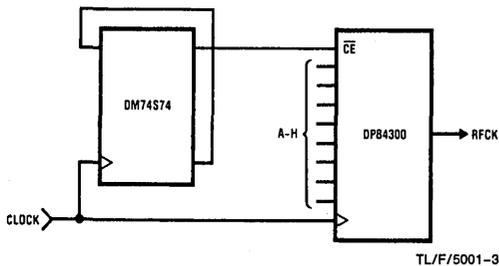
FIGURE 2a. Expansion of Clock Divisor by 2x
