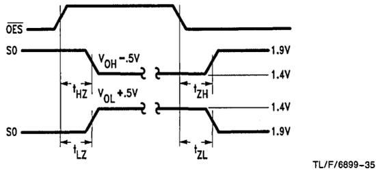
FIGURE 17. TRI-STATE Measurement
