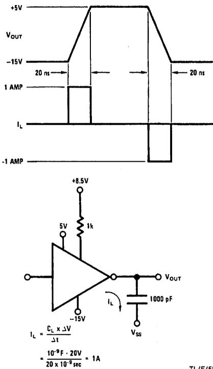
FIGURE 8. Clock Waveforms (Voltage and Current)
