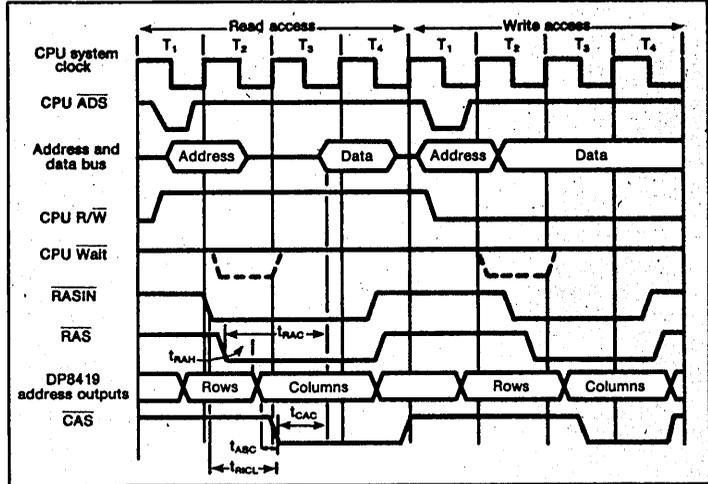
4. The interface between the CPU and the DP8419 controller chip, as shown in Fig. 3, underscores the importance of access timing. Most dynamic RAMs are characterized by  $t_{RAC}$ , their access time from RAS, but in reality  $t_{CAC}$ , the access time from CAS, is often more critical. The memory controller in fact determines which of those parameters will govern the actual access time in a system.
