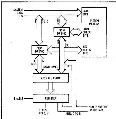
**Fig 6** A 2-bit ECC system can be implemented with two DP8400s, a 4k-byte PROM for external syndrome decoding, and a register for temporary storage of syndromes error data. Note that the altered sequence of the lines from the secondary DP8400 reflects the bit rotation needed to expand the unique matrix.
