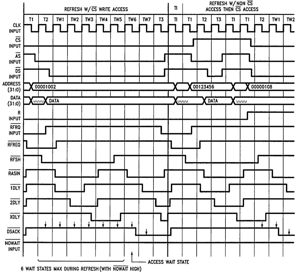
FIGURE 10. System Timing
