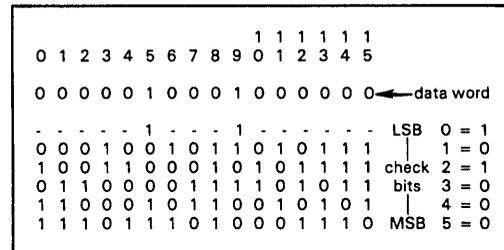
**Fig 6 Error check bits are generated by presenting the data word to ECC code matrix and noting corresponding 1s. In first row, bits 5 and 9 correspond with 1s in matrix. Thus, to maintain odd parity LSB of check bits is set to 1**
