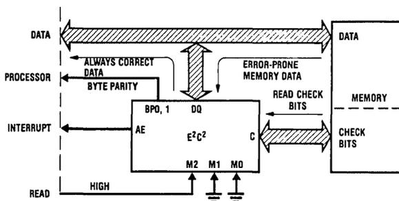
FIGURE 2c. Normal READ Mode, Always Correct Method with E<sup>2</sup>C<sup>2</sup>
