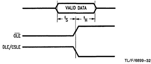
FIGURE 15. Timing Waveform for Set-Up and Hold Time
