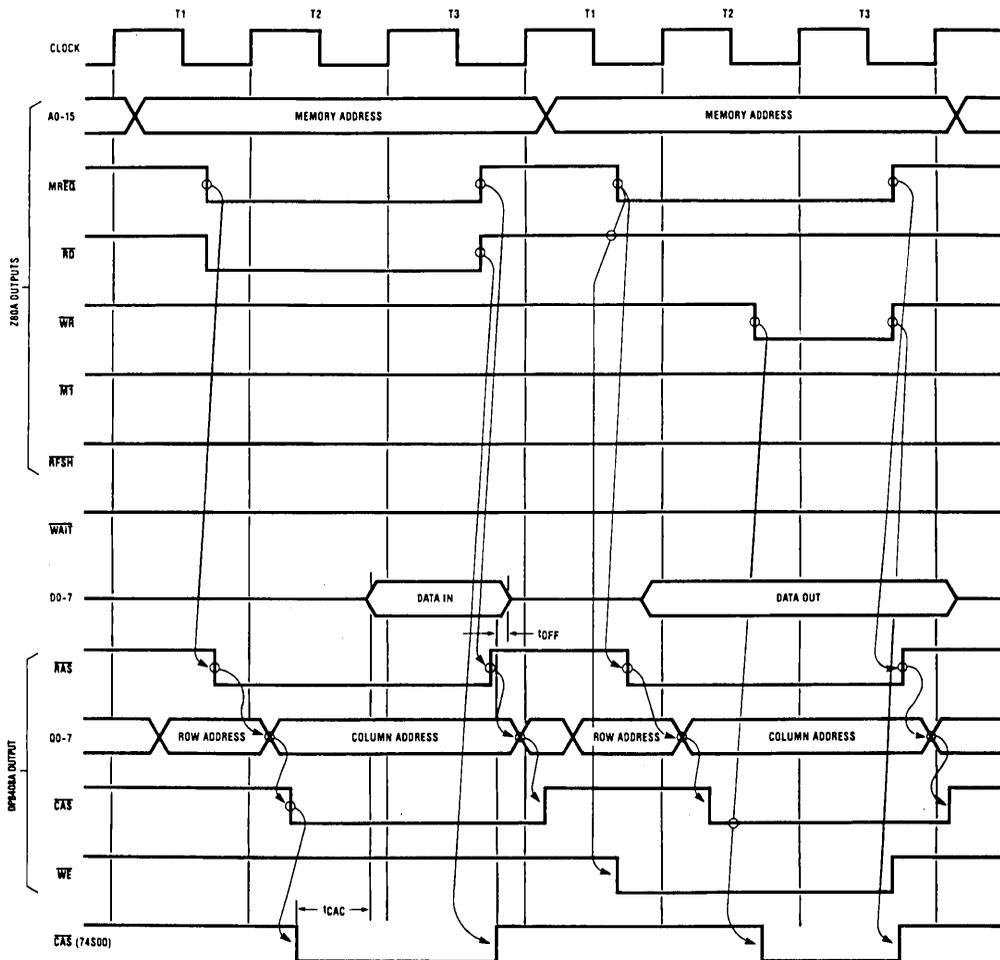
FIGURE 7. Z80A Memory Read and Memory Write Cycle
