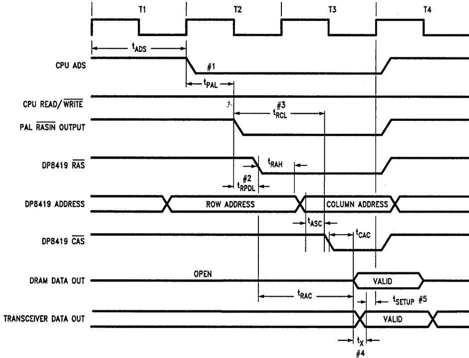
**FIGURE 2. System Access Timing (4T State Microprocessor Example)**
