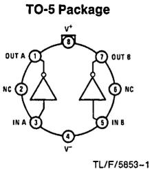
Note: Pin 4 connected to case.
