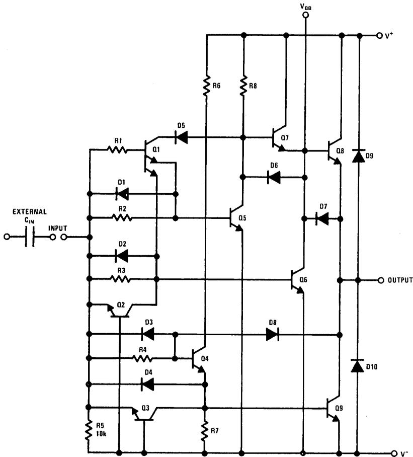
**FIGURE 7. Schematic of 1/2 DS0056**
