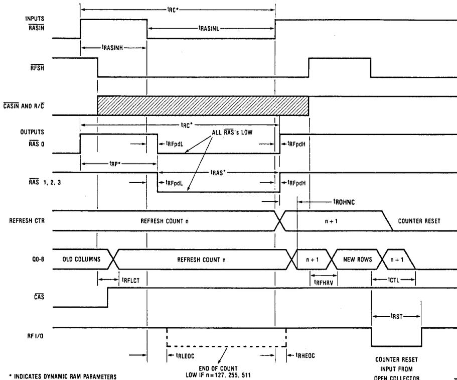
FIGURE 2. External Control Refresh Cycle (Mode 0)
