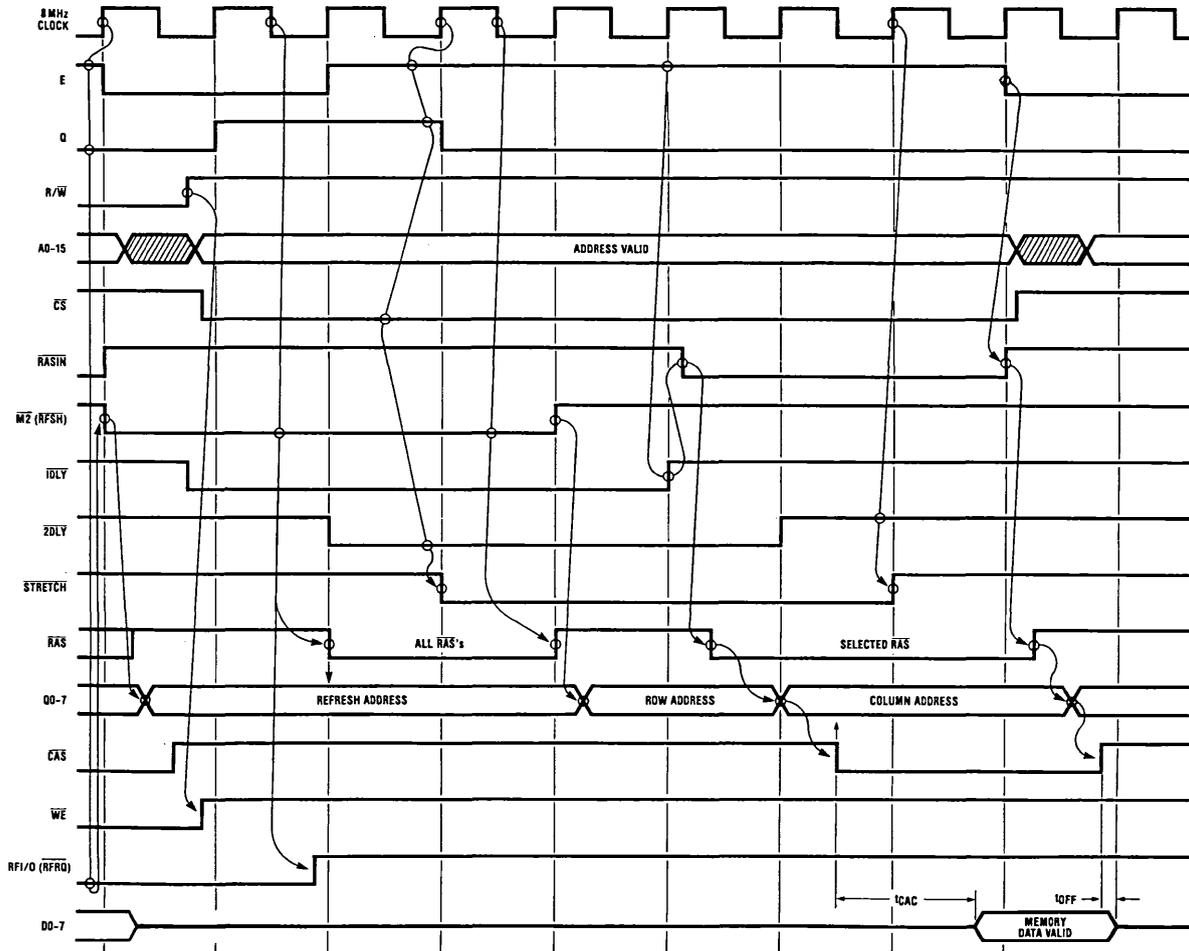
FIGURE 13. MC68B09E Forced Refresh and Memory Read Cycle
