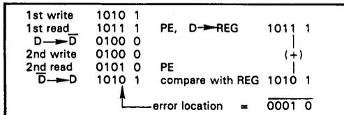
**Fig 4 Locating hard errors with parity. Use of register for temporary storage enables double complement cycle to locate single hard error**
