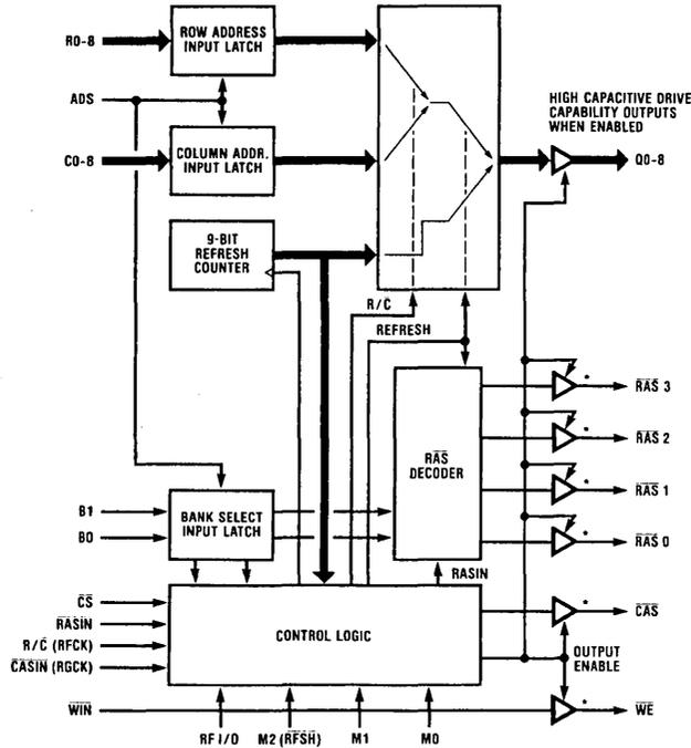
FIGURE 1. DP8409A Block Diagram
