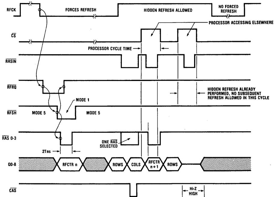
FIGURE 4. Hidden and Forced Refresh Timing of the DP8409A
