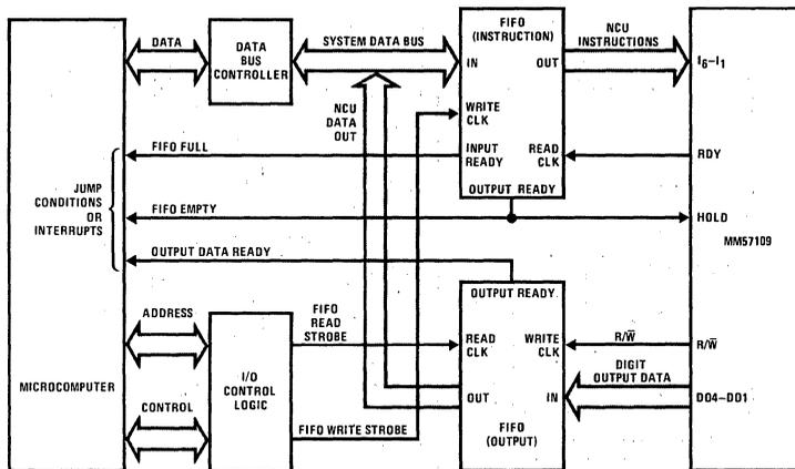
FIGURE 15. MM57109 Microcomputer Interface Using 2 FIFO's
