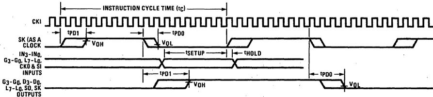
Figure 3. Input/Output Timing Diagrams (Crystal Divide-by-16 Mode)
