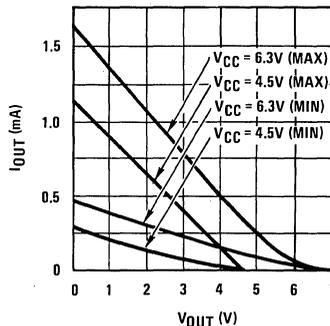
FIGURE 13. Input/Output Device Characteristics
