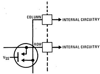
FIGURE 4a. Standard Dual Contact Telephone Key
