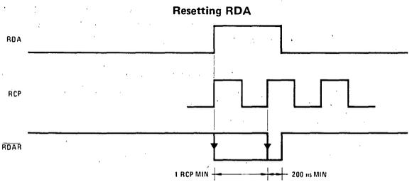
RDAR may go low any time after the RDA comes up but must stay low for at least 200 ns after the first clock pulse period. RDAR may be hard wired low, in which case RDA will go high and remain high for the duration of the positive clock pulse.
