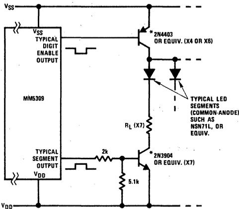
$$R_L = \frac{V_{SS} - V_{DD} - V_F - 0.6V}{N(I_F)}$$
