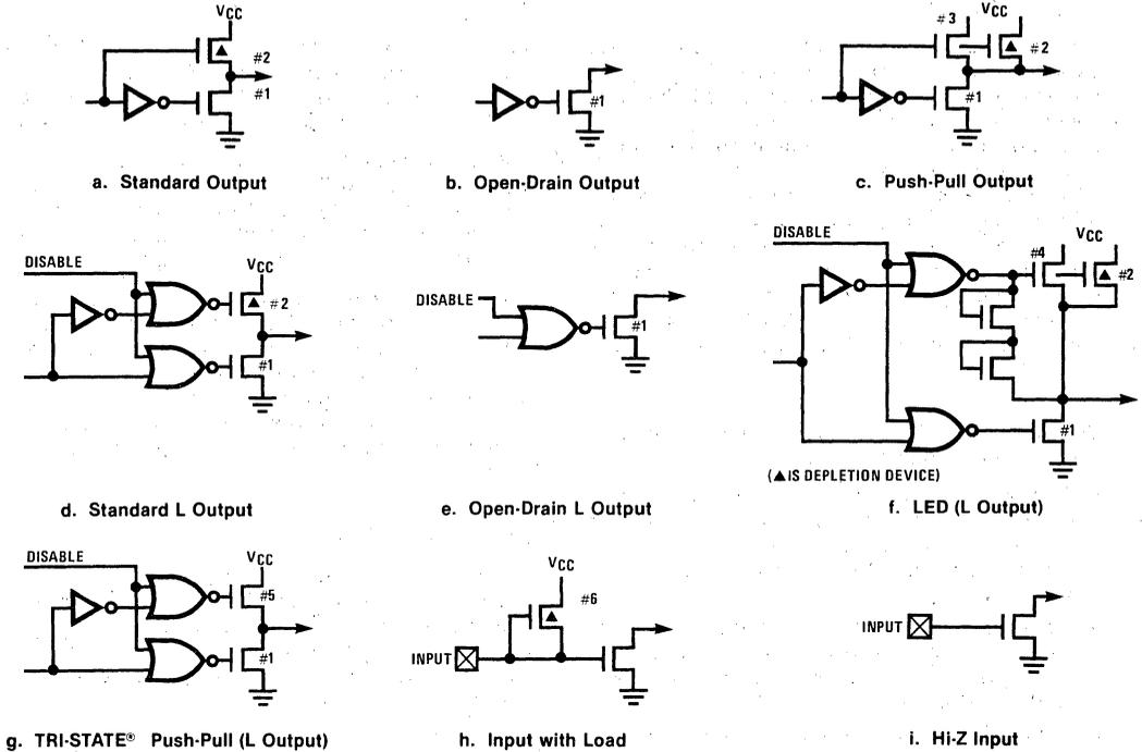
Figure 5. Output Configurations
