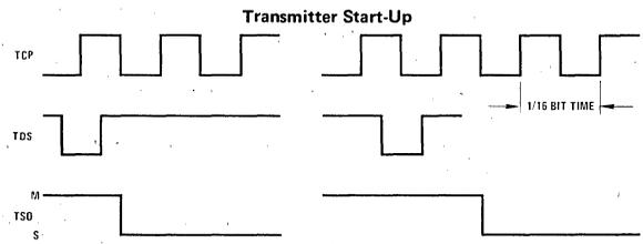
Upon data transmission initiation, or when not transmitting at 100% line utilization, the start bit will be placed on the TSO line at the high to low transition of the TCP clock following the trailing edge of TDS.
