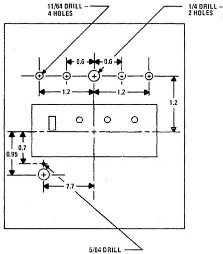
Figure 16. Drilling Guide for the Case Top if the MRC-1-10 Rotary Function Switch is Used. (Dimensions in inches.)
