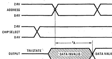
FIGURE 2. Address Follows Chip Select
