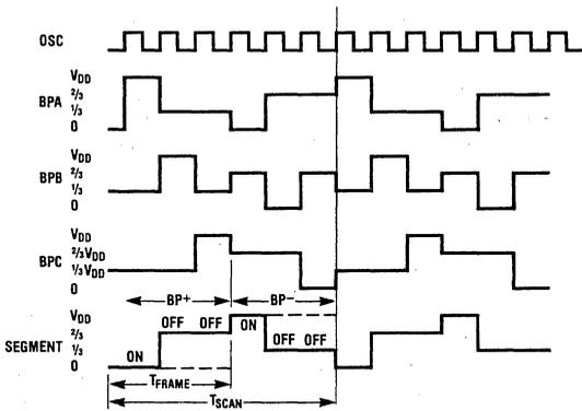
Figure 4. Backplane and Segment Waveforms
