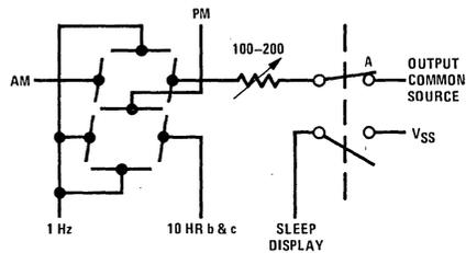
Switch A must be ganged with Sleep display as shown.
