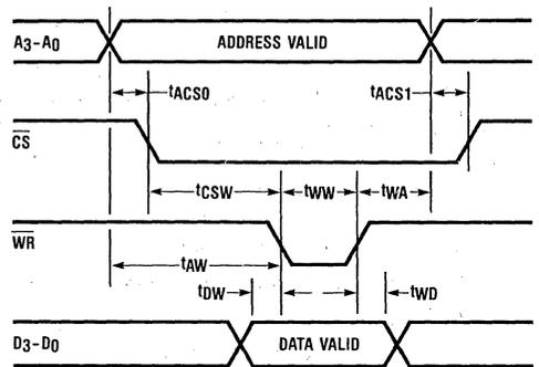
Figure 6. Write Cycle Waveforms
