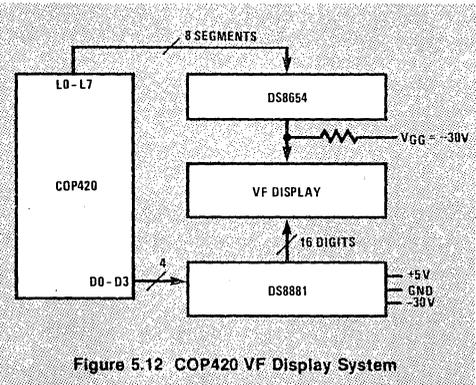
Figure 5.12 COP420 VF Display System
