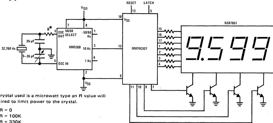
\*If the crystal used is a microwatt type an R value will be required to limit power to the crystal.
