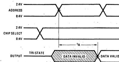
FIGURE 2. Address Follows Chip Select
