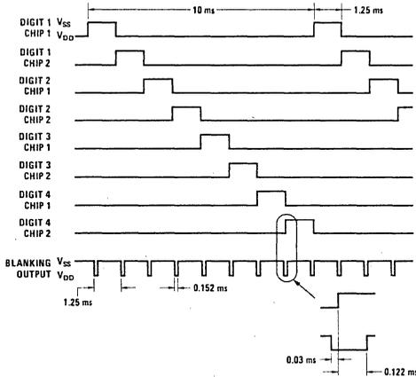
FIGURE 3. Blanking Output
