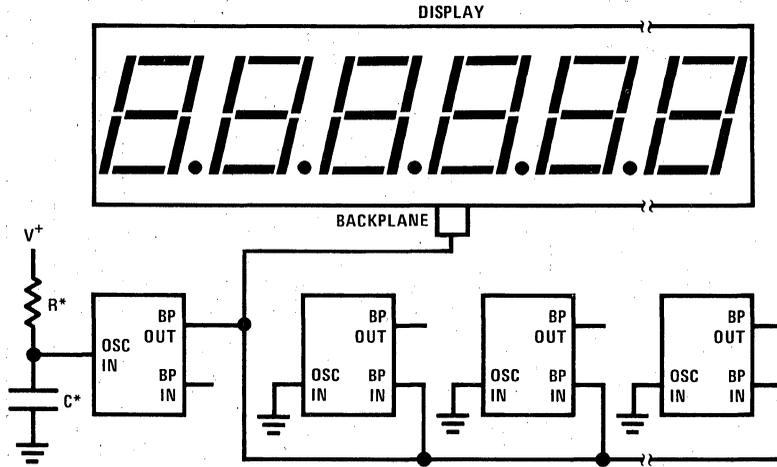
\* The minimum recommended value for R for the oscillator input is 9 kΩ. An RC time constant of approximately  $4.91 \times 10^{-4}$  should produce a backplane frequency between 30 Hz and 150 Hz.
