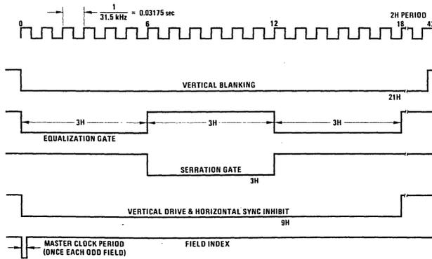
FIGURE 4. Vertical Timing
