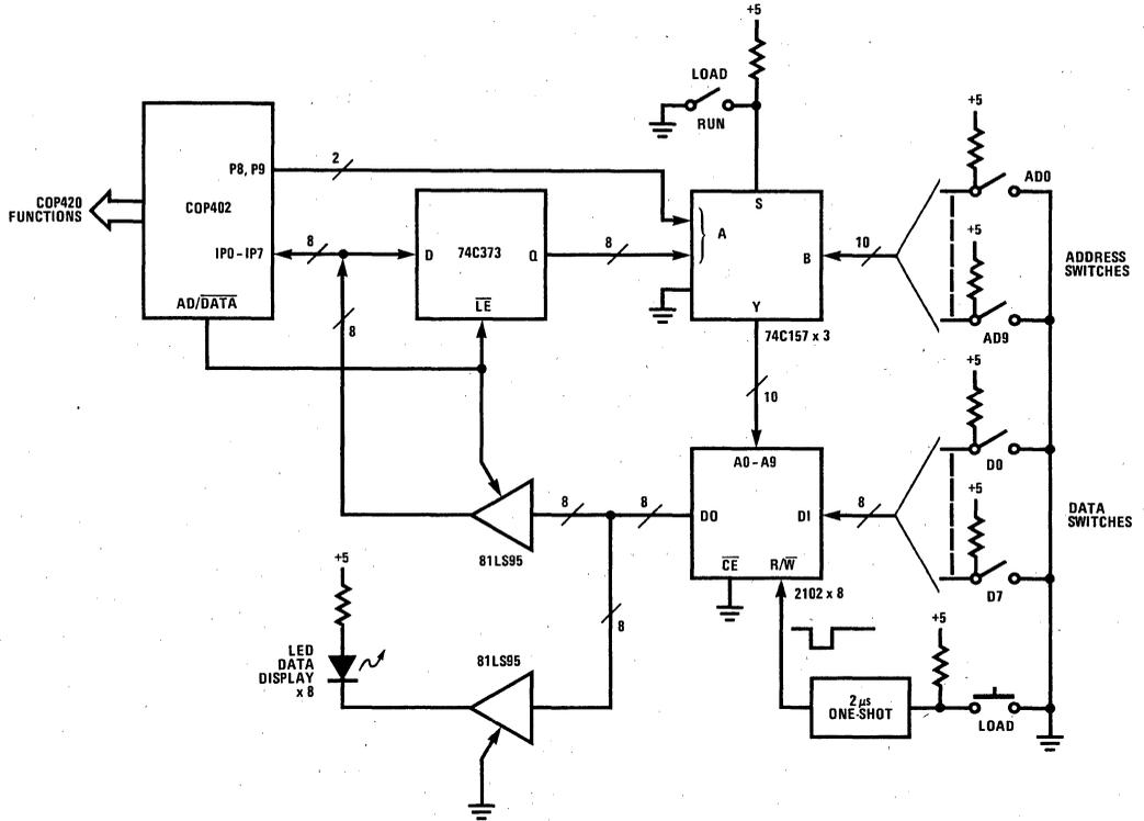
Figure 14. RAM-Based External Memory for COP402
