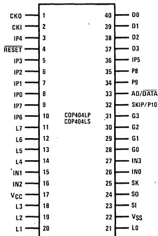
Figure 2. Connection Diagram
