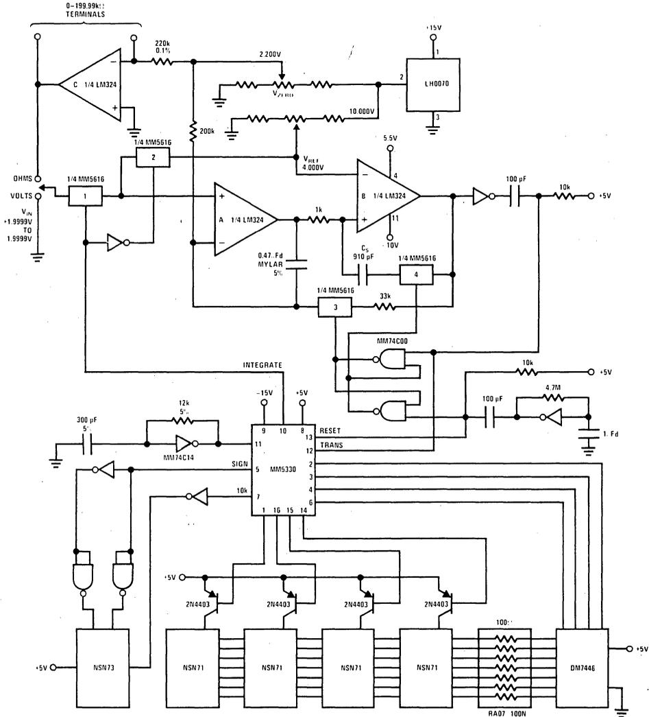
FIGURE 2. Typical Application Low Cost 4 1/2 Digit Volt-Ohm Meter
