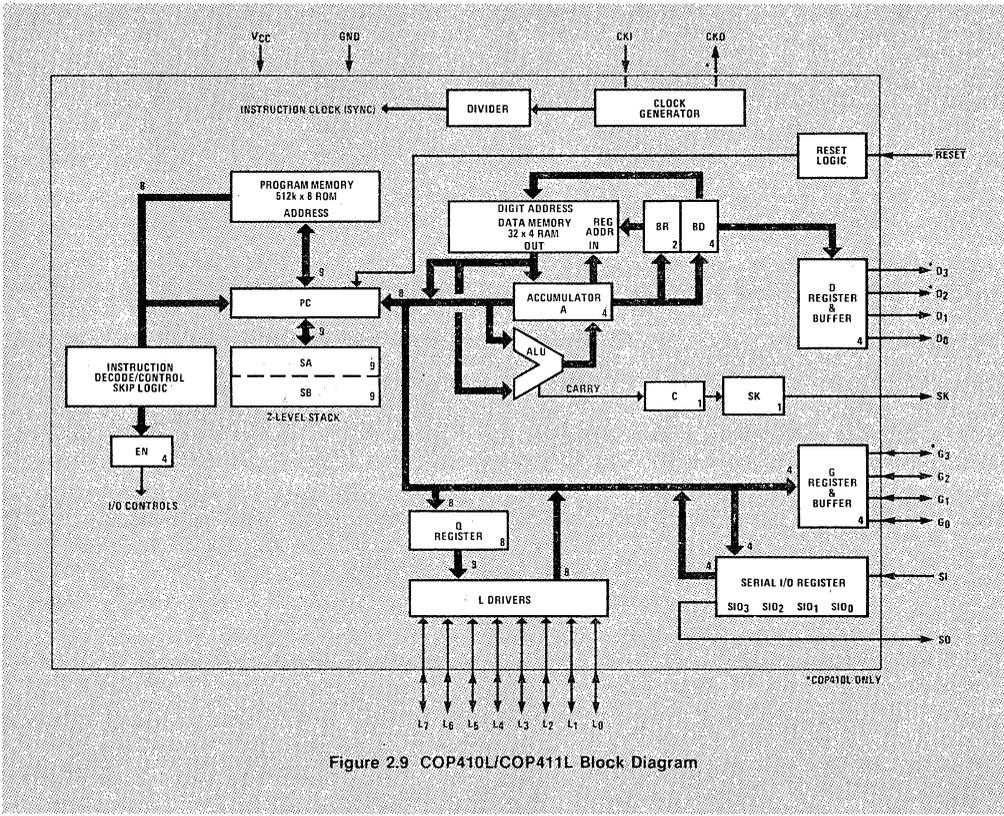
Figure 2.9 COP410L/COP411L Block Diagram
