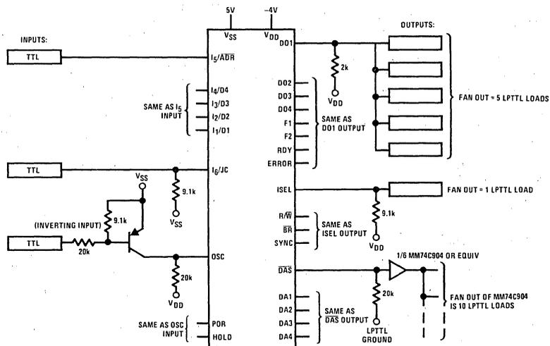
Note 1:  $I_5-I_1$  have an internal resistor to  $V_{SS}$ .  $I_6$  has an internal resistor to  $V_{DD}$ .
