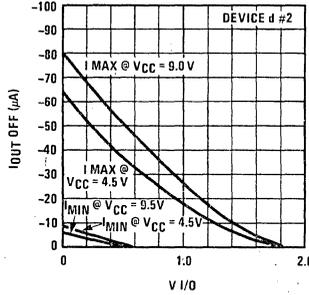
Source current for Standard Output Configuration
