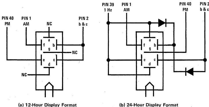
FIGURE 5. Wiring Ten's-of-Hours Digit
