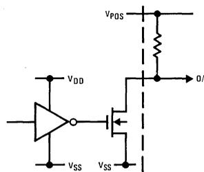
FIGURE 4b. BCD Outputs, MM53105
