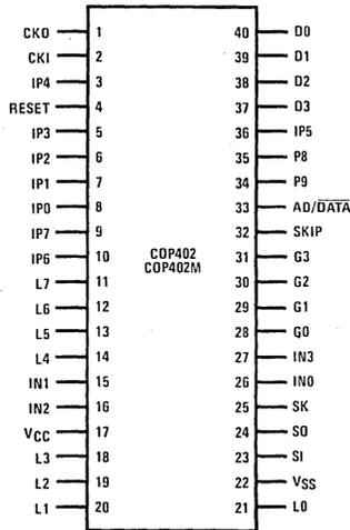
Figure 2. Connection Diagram
