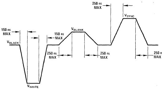
FIGURE 3. Composite Video Rise and Fall Times
