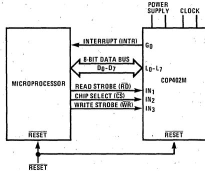
Figure 6. MICROBUS™ Optlon Interconnect
