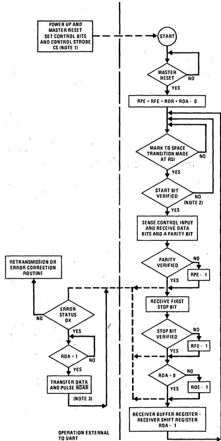
**Note 1:** Control Strobe should be made only at the beginning of transmission and remain inactive during transmission. It may be tied high if no change is necessary.
