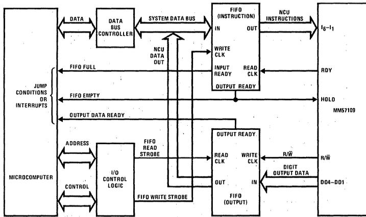
FIGURE 15. MM57109 Microcomputer Interface Using 2 FIFO's
