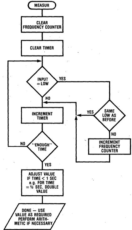
Figure 19B. V to F By Counting Pulses
