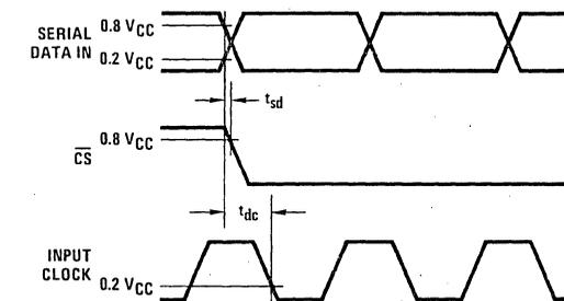
$t_{sd}$  = Delay time between active chip select command and initial data input.
