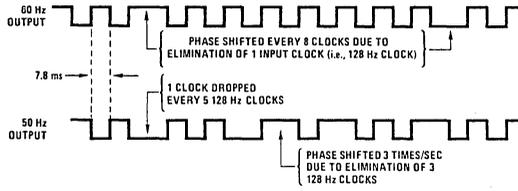
FIGURE 3. 50/60 Hz Output
