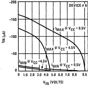
Input Current for L<sub>0</sub> through L<sub>7</sub> when Output Programmed Off by Software
