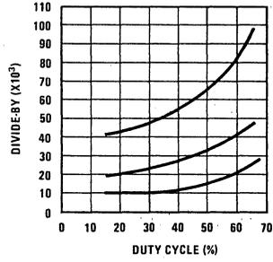
FIGURE 4. Plot of Divide-By vs Duty Cycle
