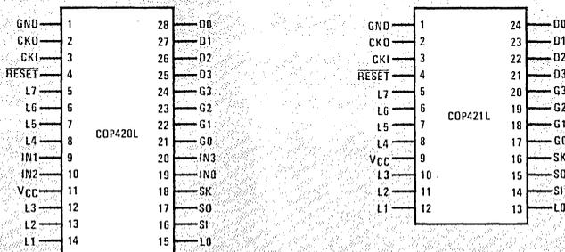
Figure 2.2 COP420/COP421 Connection Diagrams
