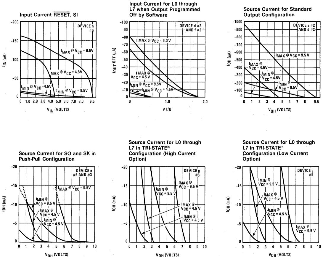
Figure 8. I/O DC Current Characteristics
