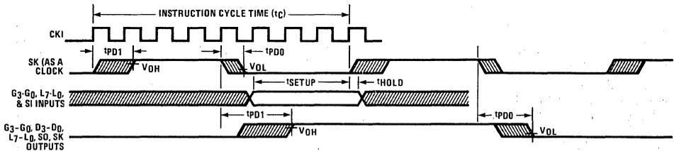
Figure 3. Input/Output Timing Diagrams (divide by 8 mode)
