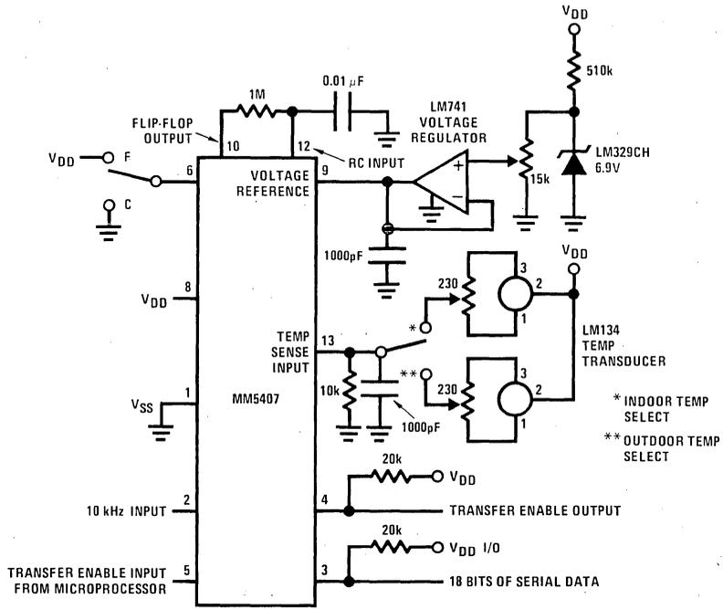
FIGURE 3A. Typical Application of MM5407 Used as a Temperature Sensor for Microprocessor
