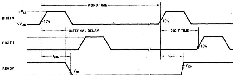
FIGURE 2. Output Timing
