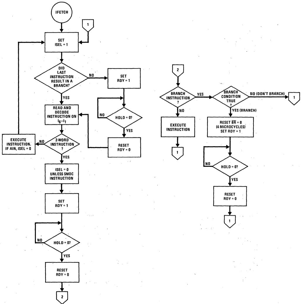
FIGURE 7. MM57109 Instruction Fetch and Execution Flowchart
