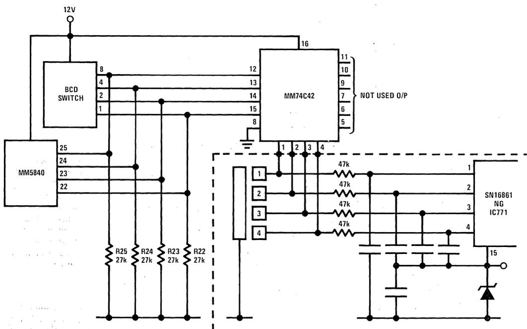
FIGURE 3. Channel Switching Interface with MM74C42
