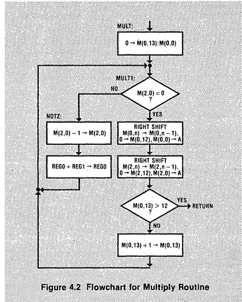
Figure 4.2 Flowchart for Multiply Routine
