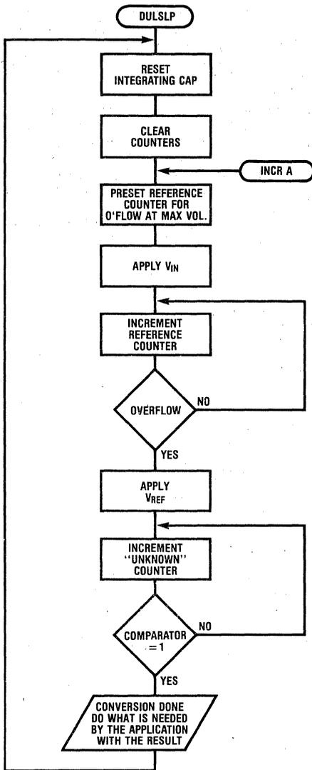
Figure 14B. Basic Dual Slope A/D Flow Chart
