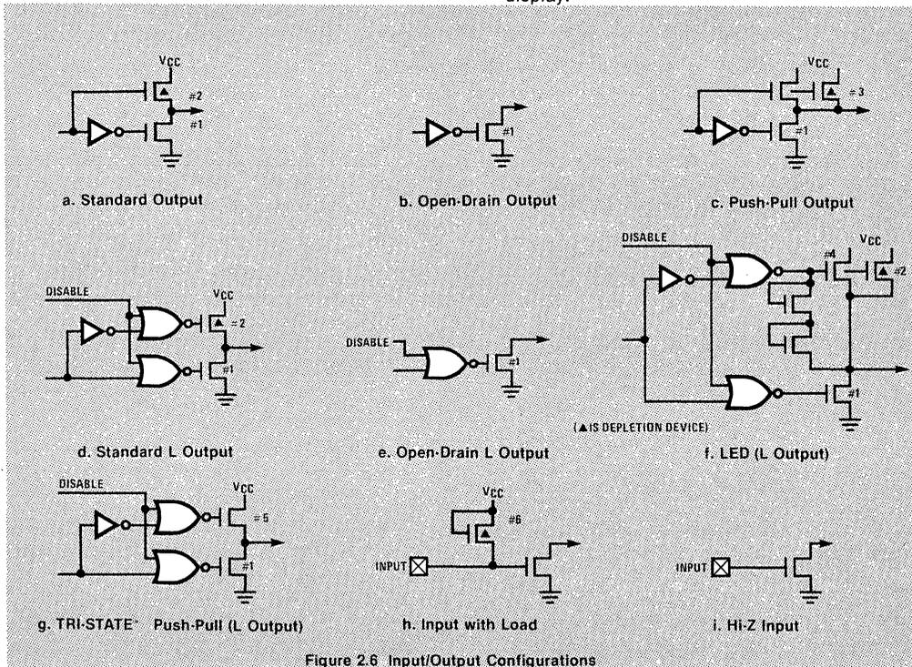
Figure 2.6 Input/Output Configurations
