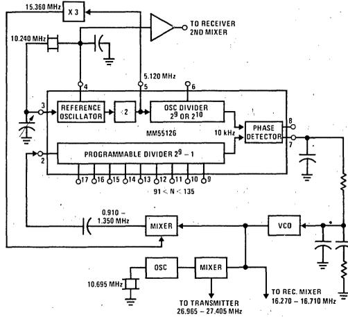
FIGURE 4b. MM55126 2-Crystal, 40-Channel Application
