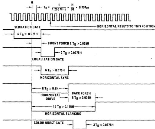
FIGURE 3. Horizontal Timing Master Clock = 1.26 MHz
