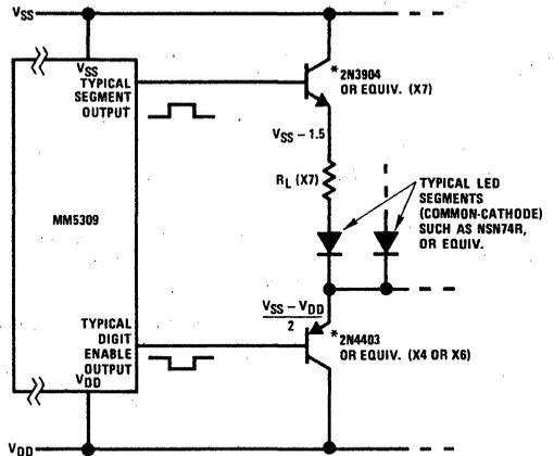
$$R_L = \frac{(V_{SS} - V_{DD})/2 - V_F - 1.5V}{N(I_F)}$$
