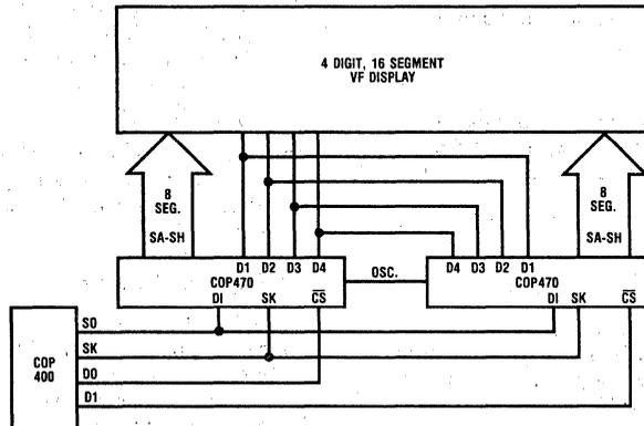
Figure 8. System Diagram for 16 Segment Display
