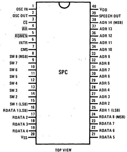
**Connection Diagrams** (Continued) ( $V_{CC} = 4.75V-5.25V$ )
