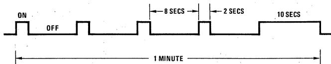
FIGURE 7. Alarm Output Waveform
