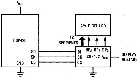
Figure 6. System Diagram — 4 1/2 Digit Display
