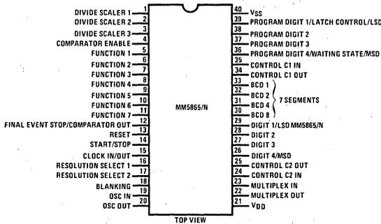
Figure 2. MM5865 connection diagram.
