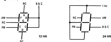
Figure 2. 10's of Hours Digit Wiring Options
