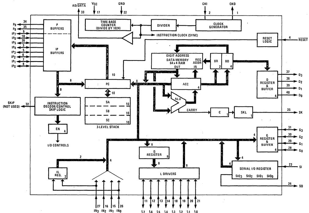
Figure 1. COP402/402M Block Diagram
