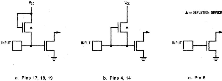
Figure 4. Input Configurations
