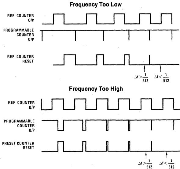
Lock signal is set after 32 cycles of REF counter output without a preset.
