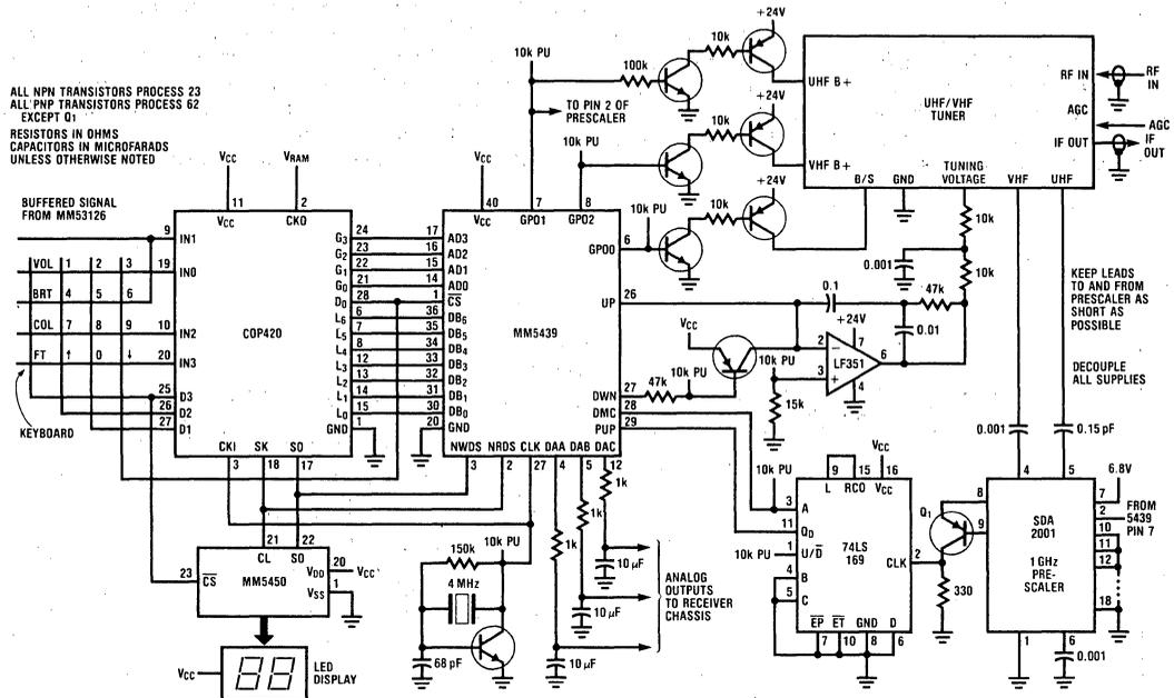
Figure 2. Low-End CTC Schematic
