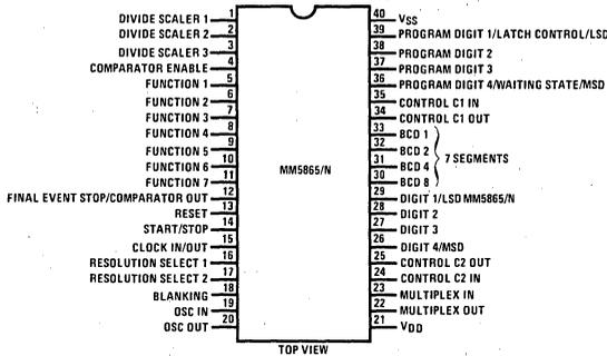
Figure 2. MM5865 connection diagram.
