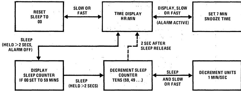
FIGURE 9. Snooze and Sleep Control State Diagram
