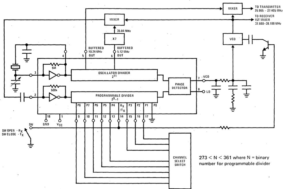
FIGURE 2. MM55108 Single Crystal 40-Channel High Side Injection
