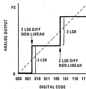
FIGURE 8.  $\pm 1$  LSB Linear,  $\pm 2$  LSB Differential Non-Linear
