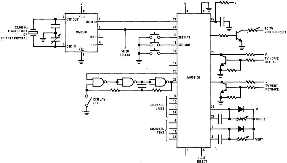
FIGURE 6. TV Time/Channel Display
