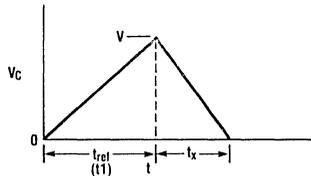
Figure 12. Dual Slope Integration — Basic Concept
