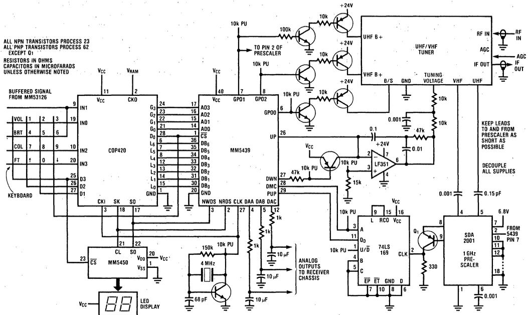
Figure 2. Low-End CTC Schematic
