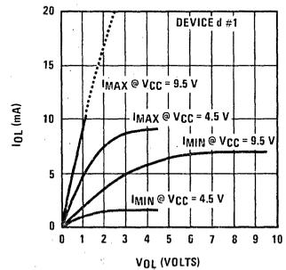
Output Sink Current G<sub>0</sub>-G<sub>3</sub> and D<sub>0</sub>-D<sub>3</sub>
