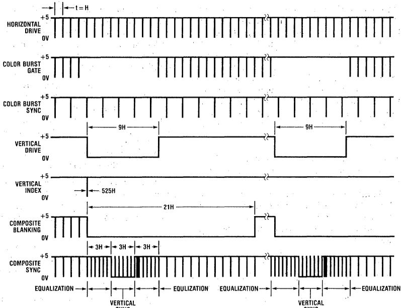
Figure 2. Sync Generator Output Waveforms
