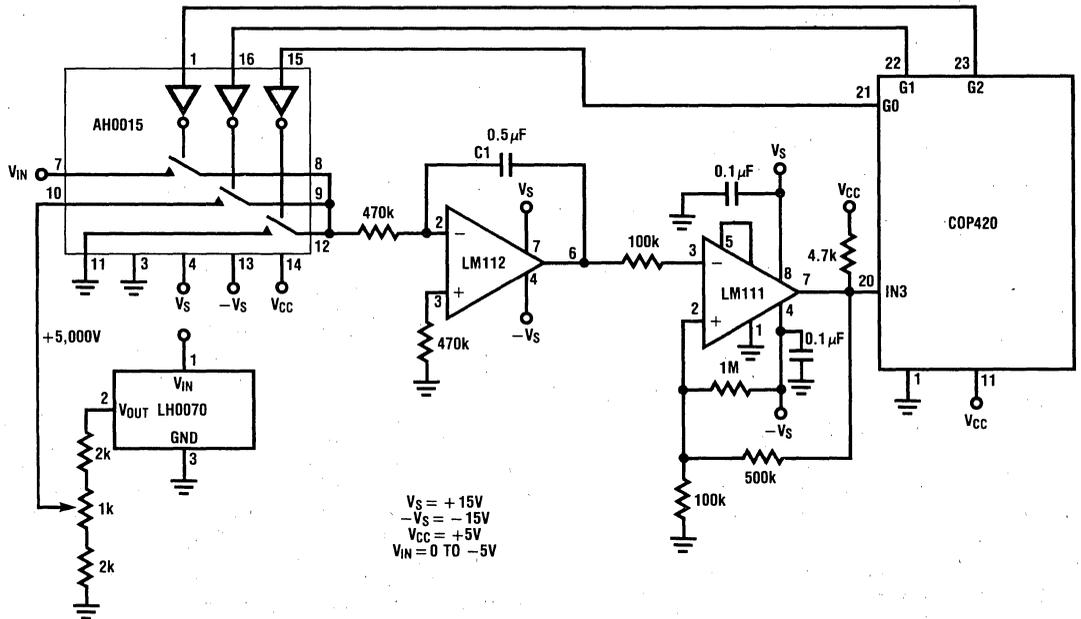
Figure 13. Basic Dual Slope Integration A/D Scheme
