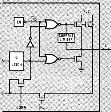
Figure 5.7 COP420 L I/O Port Characteristics
