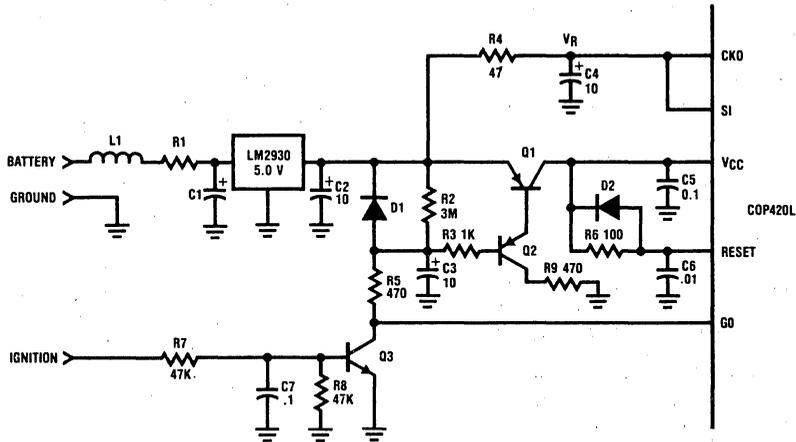
Figure 6. Power Supply Circuitry
