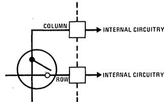
FIGURE 4b. Single Contact Key
