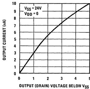
FIGURE 5. Typical Output Current Characteristics of MM5387AA, MM53108
