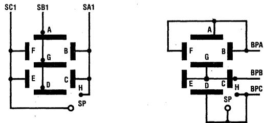
Figure 5. Typical Display Internal Connections
