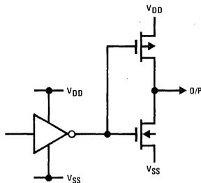
FIGURE 3. CMOS Output (TV "ON", Auto "ON", Indicator)
