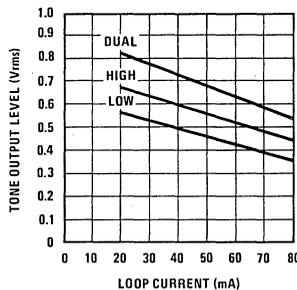
FIGURE 7. Typical Tone Output vs Loop Current
