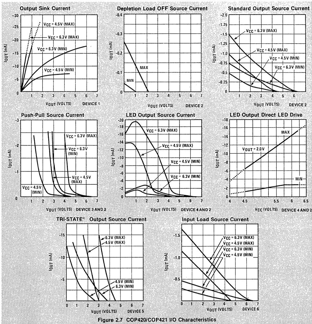
Figure 2.7 COP420/COP421 I/O Characteristics
