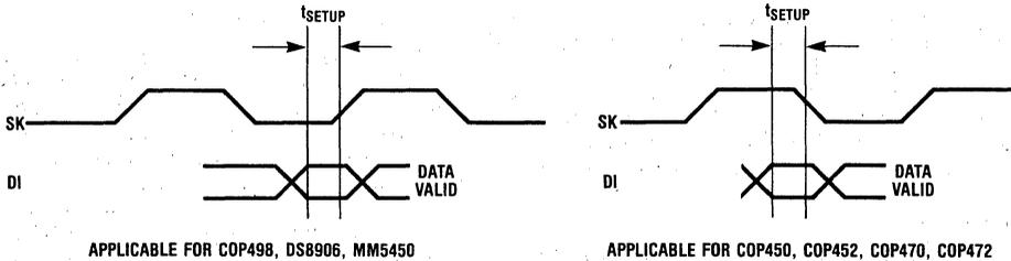
Figure 1. Serial Input Data Timing
