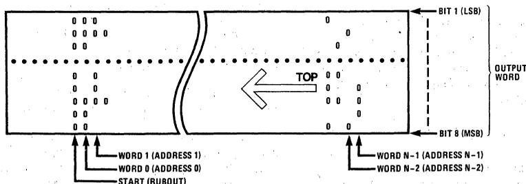
Note: Start with a RUBOUT and enter the output words in sequence from word 0 (address 0) to word N – 1 (address N – 1). There must not be any other characters on the tape. The order information must indicate whether a punch equals "0" or "1." THIS IS THE LEAST RELIABLE FORMAT. IT HAS NO ERROR CHECKING AND SHOULD BE AVOIDED IF AT ALL POSSIBLE.
