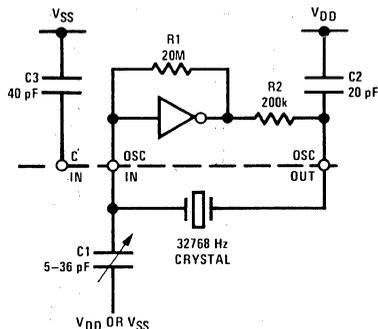
FIGURE 6. Oscillator Network
