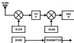
FIGURE 3. Signals Needed to Transmit and Receive Ch. 1
