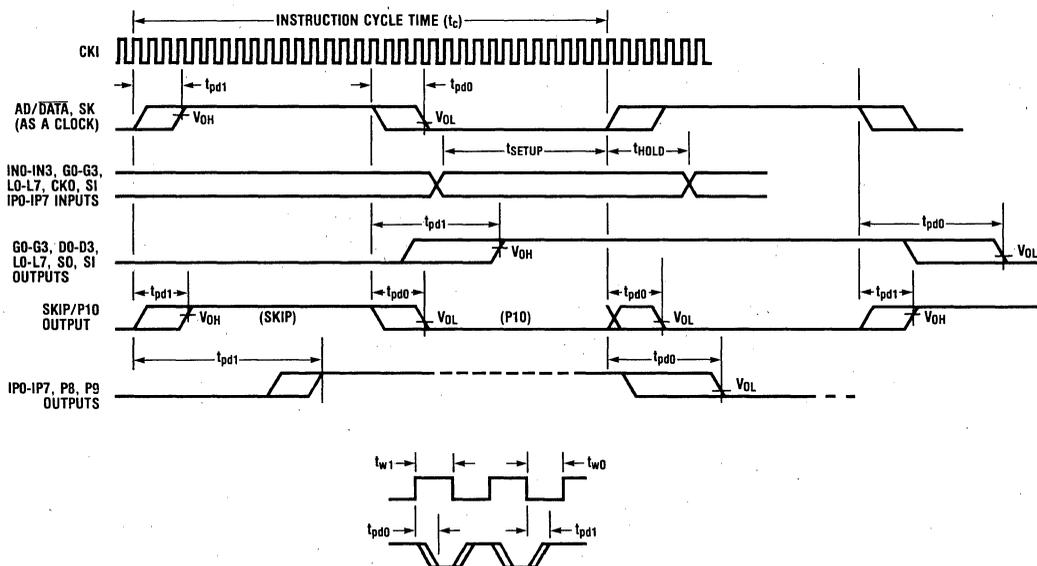
Figure 3. Input/Output Timing Diagram
