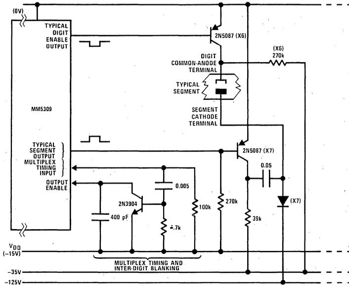
FIGURE 9. Interface Panplex II\* Neon Display Tube
