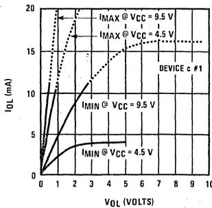
Output Sink Current for L<sub>0</sub> through L<sub>7</sub>
