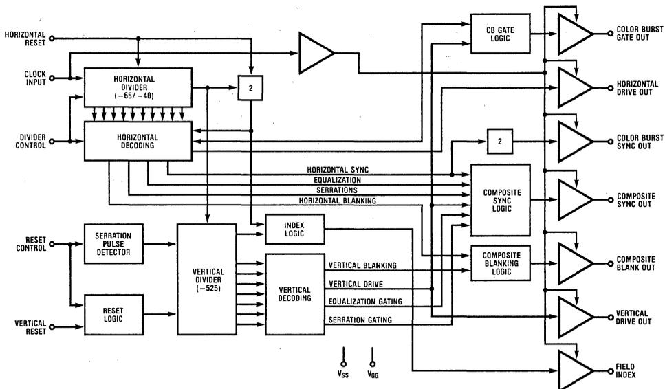
Figure 1. Block Diagram of a TV Camera Sync Generator
