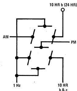
FIGURE 6. 24-Hour Operation: 10's of Hours Digit Connections
