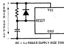
Note: If power-low failsafe option is selected, the RC and diode circuit is not used.
