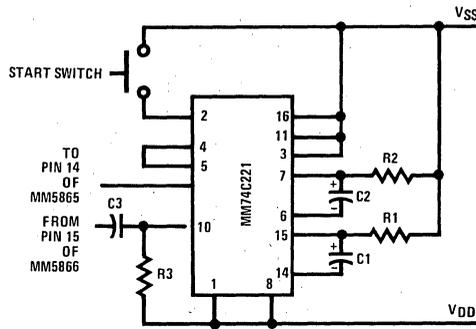
Figure 21. Start-Pulse Synchronizer. Time constant of R1 - C1 = display resolution. Time constant of R2 - C2 < display resolution. Time constant of R3 - C3 < time constant of R2 - C2.
