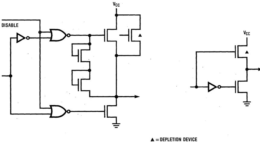
Figure 5. Output Configurations
