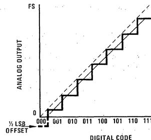
**Hysteresis Error** in an ADC causes the voltage at which a code transition occurs to be dependent upon the direction from which the transition is approached. This is usually caused by hysteresis in the comparator inside an ADC. Excessive hysteresis may be reduced by design; however, some slight hysteresis is inevitable and may be objectionable in converters if hysteresis approaches  $\frac{1}{2}$  LSB.
