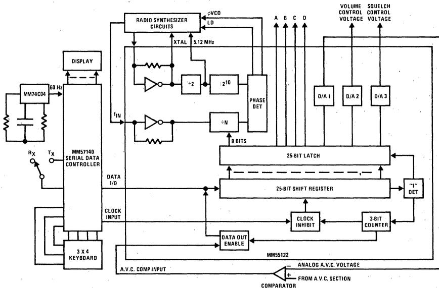
FIGURE 4. Remote Microphone Serial Data System
