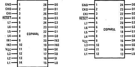
Figure 2. Connection Diagrams
