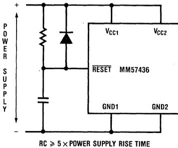
Figure 2. Power-Up Clear Circuit
