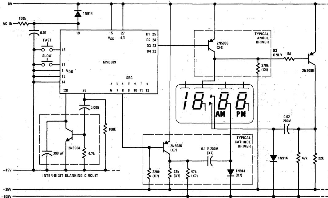
FIGURE 10. MM5309 Driving Gas Discharge Display, Typical Applications
