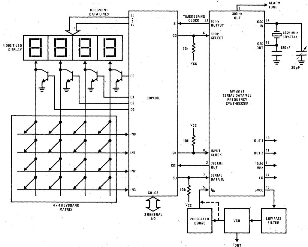
FIGURE 4. MM55121, COP420L Frequency Synthesizer/Controller
