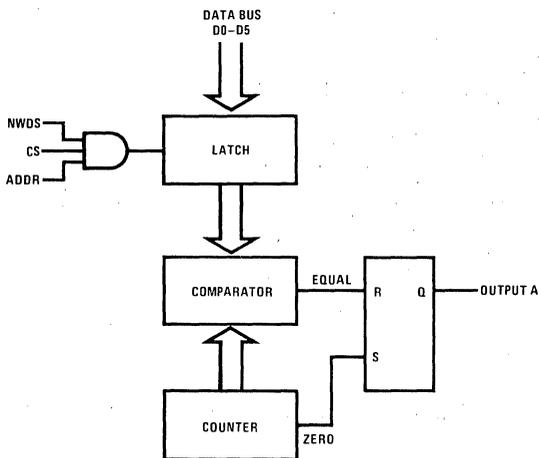
Pulse width modulated output for analog functions
