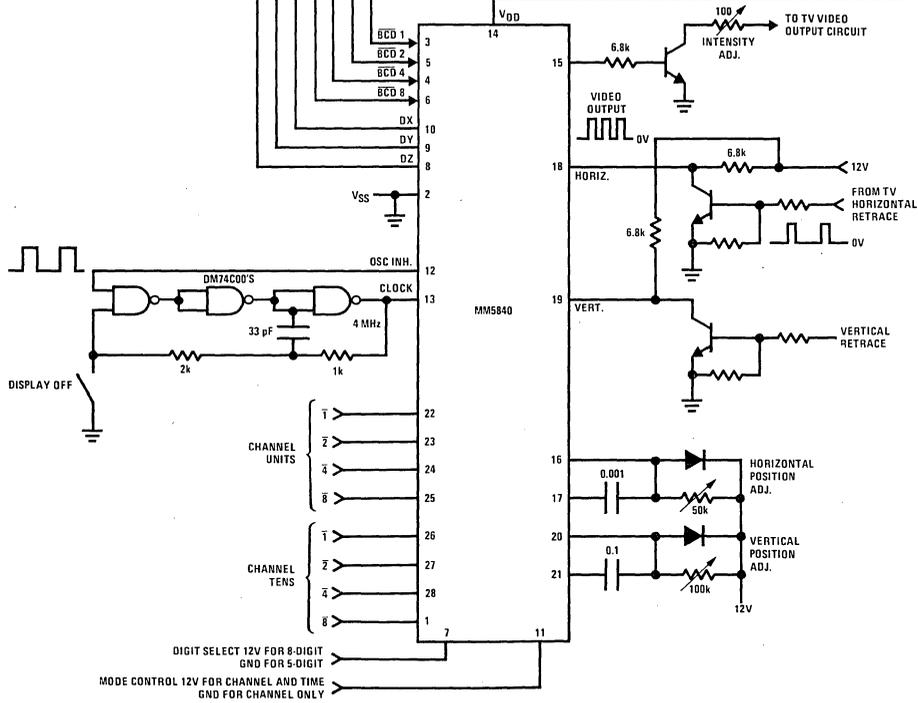
FIGURE 5. Typical Application TV Channel and Time Display
