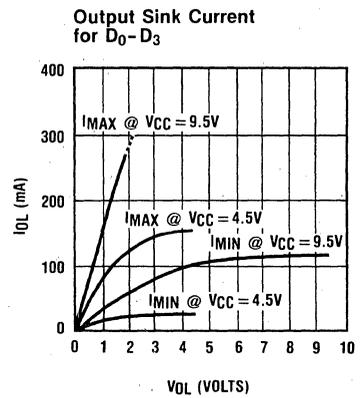
Figure 6. I/O DC Current Characteristics
