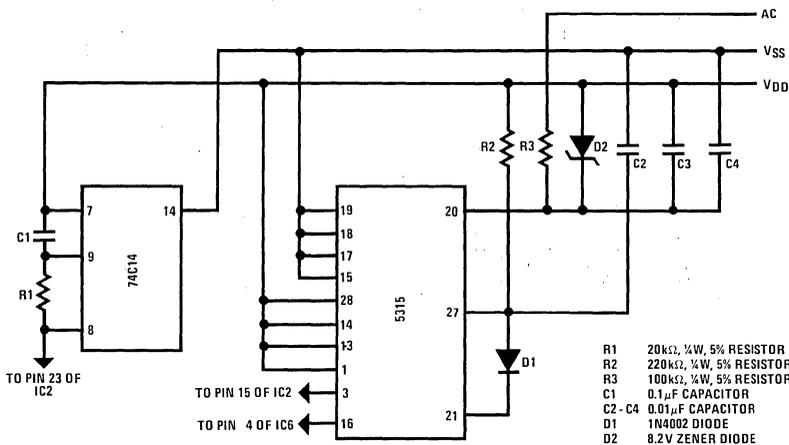
**Figure 19. Using an MM5315 Digital Clock and an External Multiplexer to Provide an External Time Base for the MM5865 to Generate a Display Resolution of 1 Minute.**
