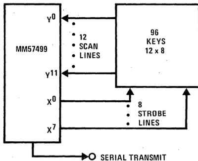
FIGURE 5. Minimal Configuration—96-Key
