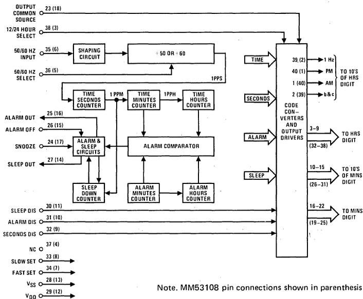
Note. MM53108 pin connections shown in parenthesis
