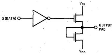
FIGURE 5. Output Circuit
