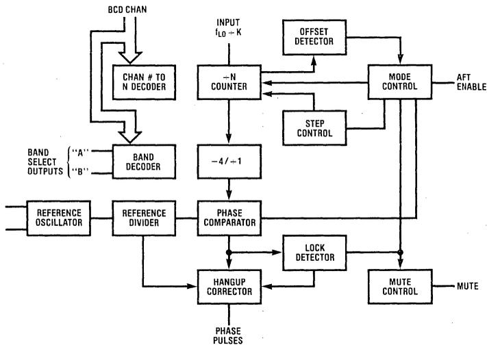
Figure 1. MM48142 TV Synthesizer with AFT Drift Simplified Block Diagram
