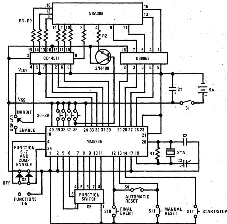
Figure 4. Stopwatch/Timer application showing the connections for a single MM5865. Two cascaded MM5865s may also be used, as described in the text.
