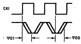
Figure 3B. CKO Output Timing
