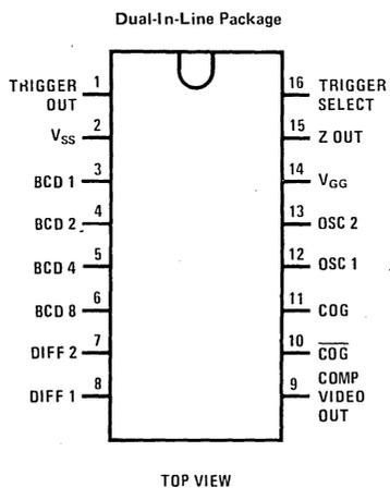
Note. Z<sub>OUT</sub> is an internal counter test point.
