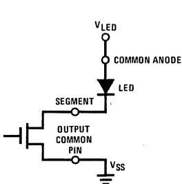
FIGURE 5(a). Common Anode Application
