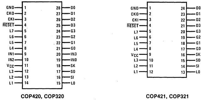
Figure 2. Connection Diagrams
