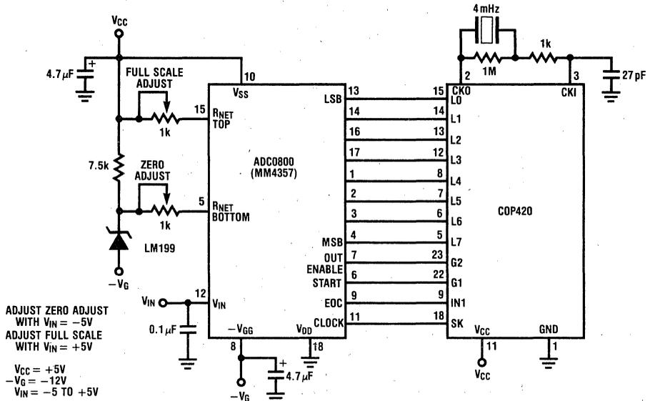
Figure 29. Simple A/D with ADC0800
