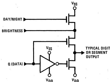
FIGURE 4. Output Circuit
