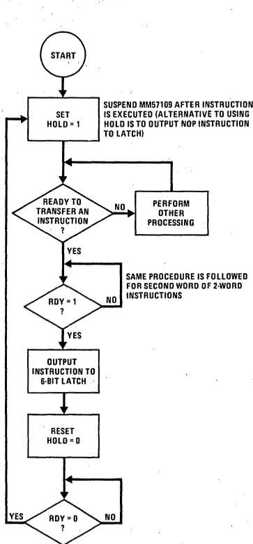
FIGURE 13(b). Microcomputer Software for MM57109 Peripheral Interface
