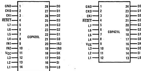
Figure 2. Connection Diagrams
