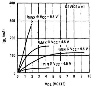
Output Sink Current IP<sub>0</sub>-IP<sub>7</sub>, P<sub>8</sub>, P<sub>9</sub>, SKIP/P10
