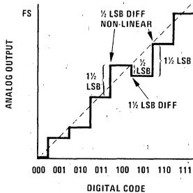
FIGURE 9. Non-Monotonic (Must be  $> \frac{1}{2}$  LSB Non-Linear)
