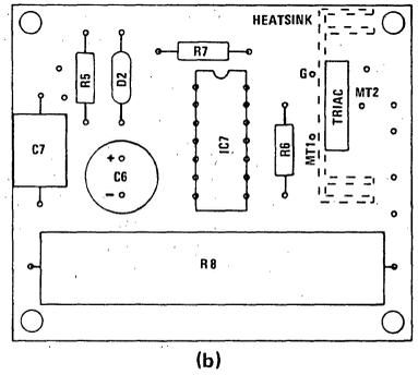
Figure 11. Printed Circuit Board Component Layouts. a) Layout for the Stopwatch/Timer PC board. b) Layout for the Appliance Control PC board.
