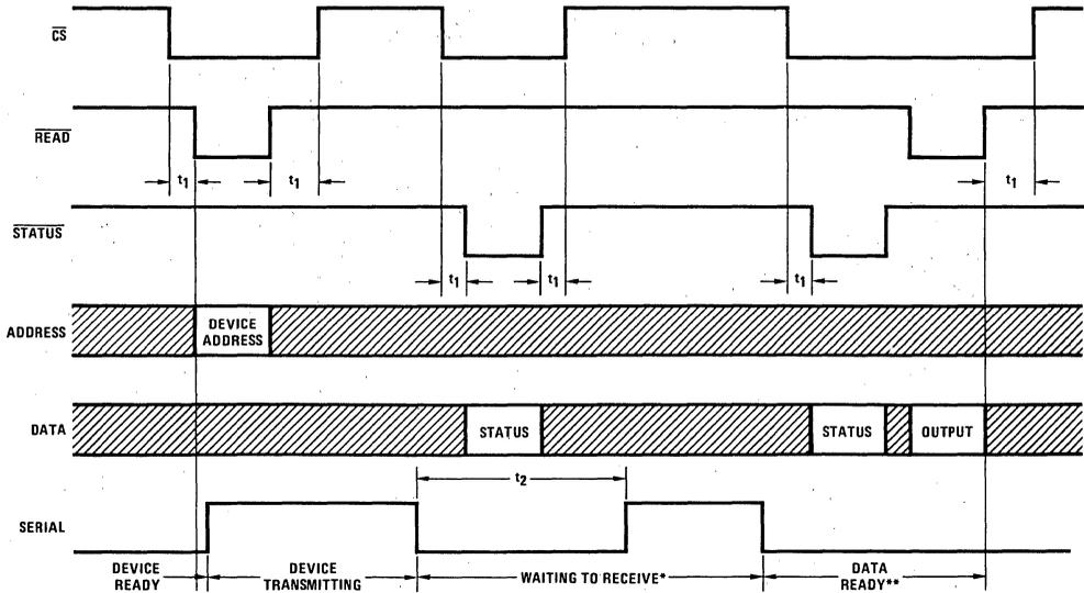
\* During "waiting to receive" state,  $\overline{CS}$  coupled with  $\overline{R}/C1$  will force device into the device ready state
