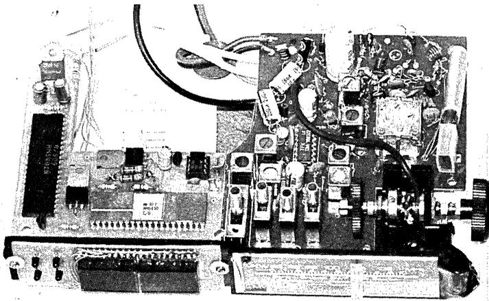
**The MM5430, MM5402 Circuit Applied to an Existing Clock Radio Chassis; Note that the Original Dial Pointer is Still Used.**
