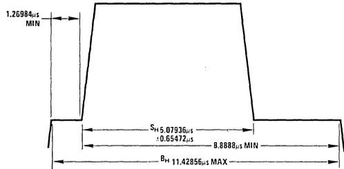
FIGURE 4. Composite Video Pulse Timing, Horizontal Sync
