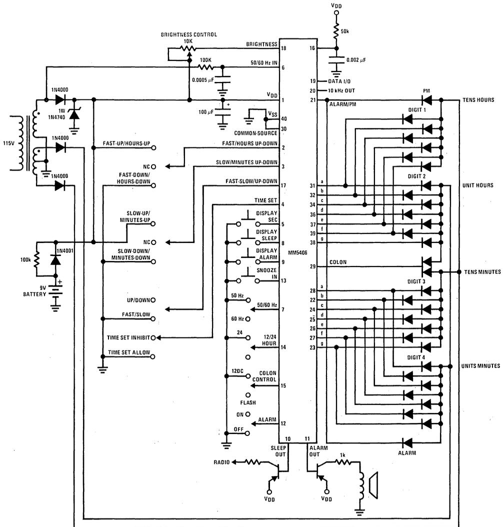
FIGURE 4 Typical Application for MM5406
