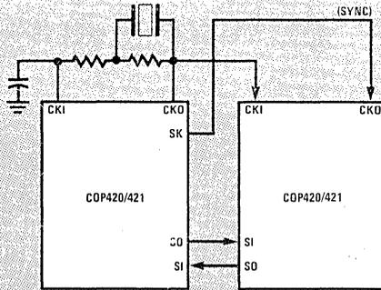
d. Externally Synchronized Oscillator
