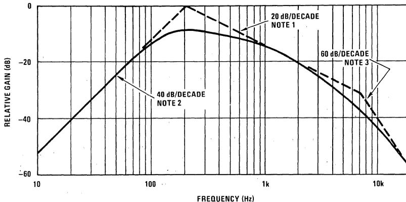
**Note 1:** This curve is the desired response of the entire audio system including speaker. Minimum response is a low pass filter with a cutoff frequency of 200 Hz. For an audio system with a natural cutoff frequency around 200 Hz, this filter can be eliminated. This cutoff frequency may be tuned for the particular voice being synthesized. For a low pitched male voice it may be 100 Hz, while for a high pitched female or child's voice it might be 300 Hz.
