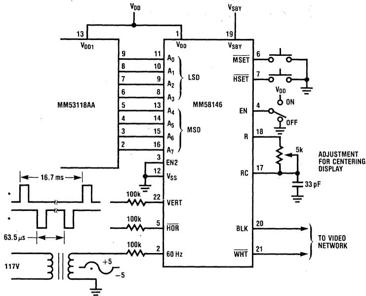
TV Channel and Time Display Interfacing with MM53118AA
