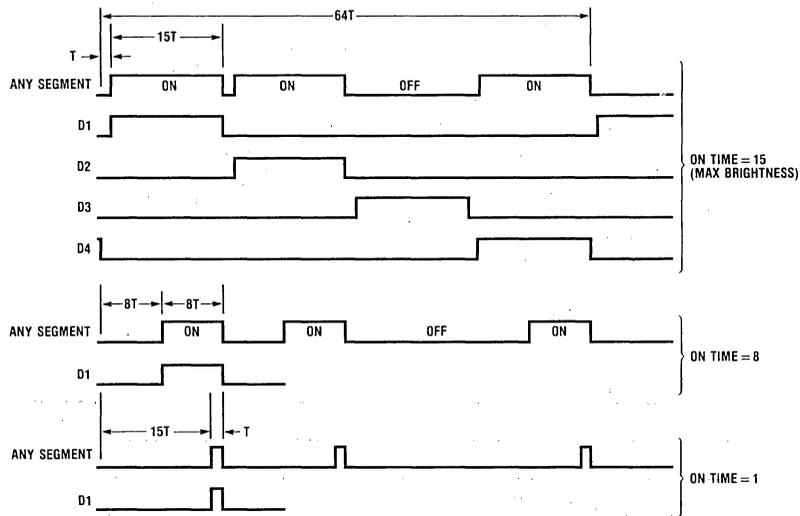
Figure 5. Segment and Digit Output Timing Diagram
