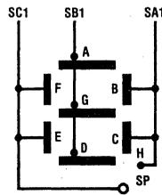
Figure 5. Typical Display Internal Connections
