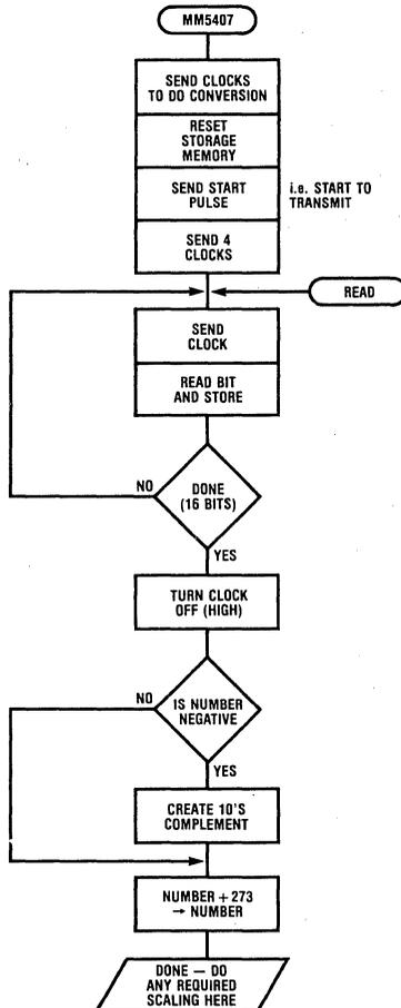
Figure 34B. MM5407 as A/D Converter Flow Chart
