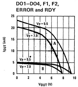
**Note 1:** Curves "A" represent a maximum current device at 0°C. Curves "B" represent a minimum current device at +70°C.
