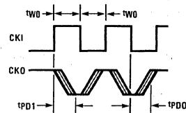
Figure 3B. CKO Output Timing
