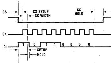
Figure 3. Serial Load Timing Diagram
