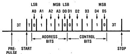
Figure 5. Format of Remote Control Signal 0111001110
