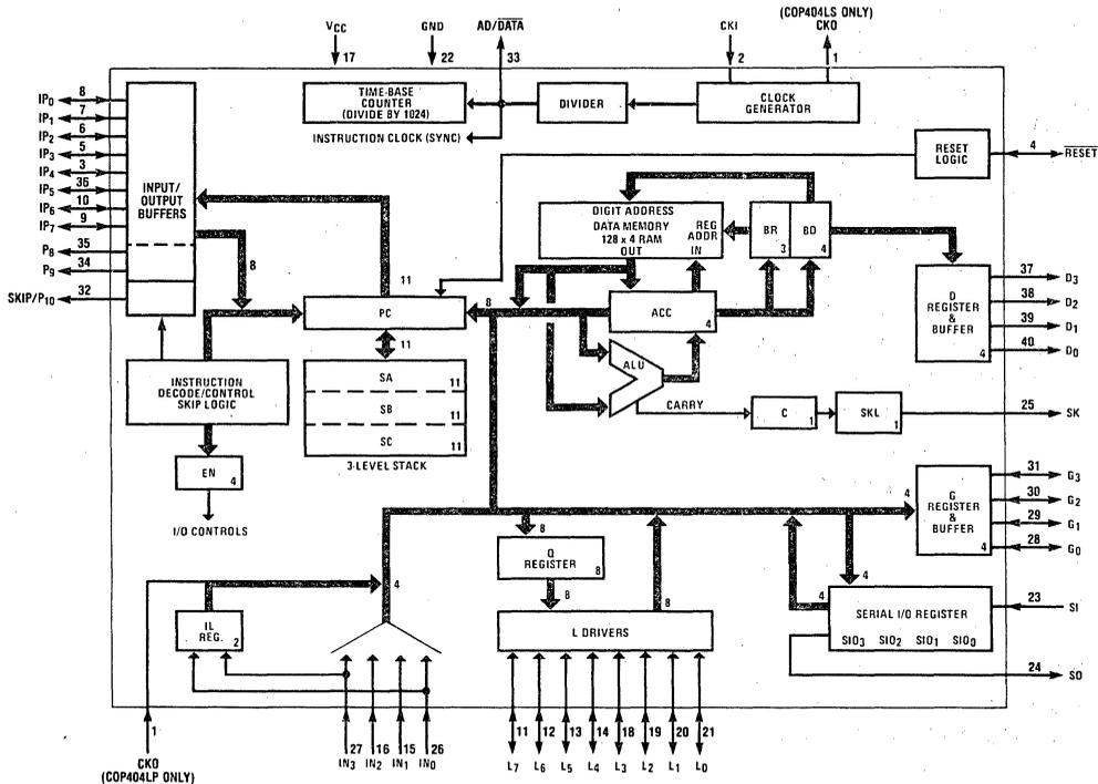
Figure 1. COP404L Block Diagram
