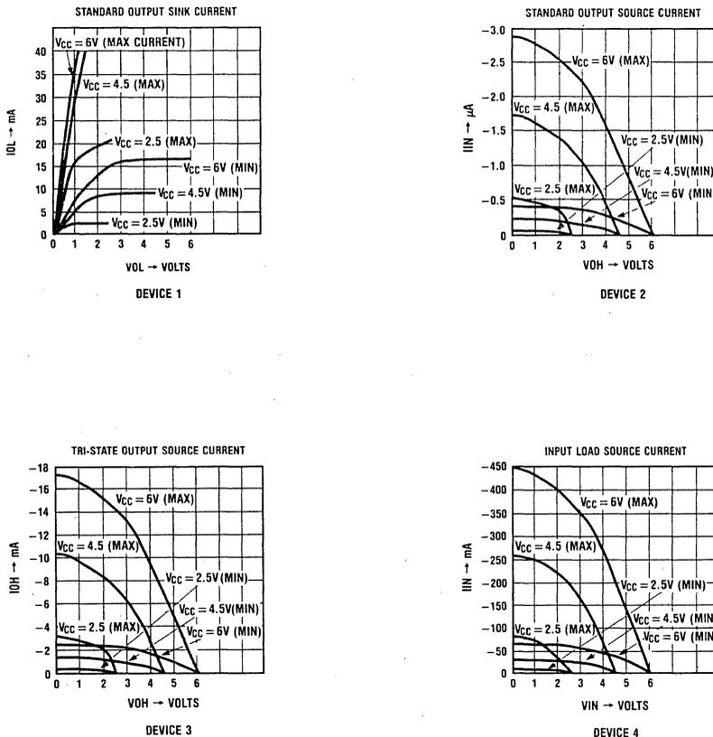
Figure 12. I/O Characteristics
