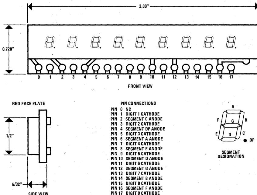
Figure 5. Physical dimensions and pin connections of the NSA398.
