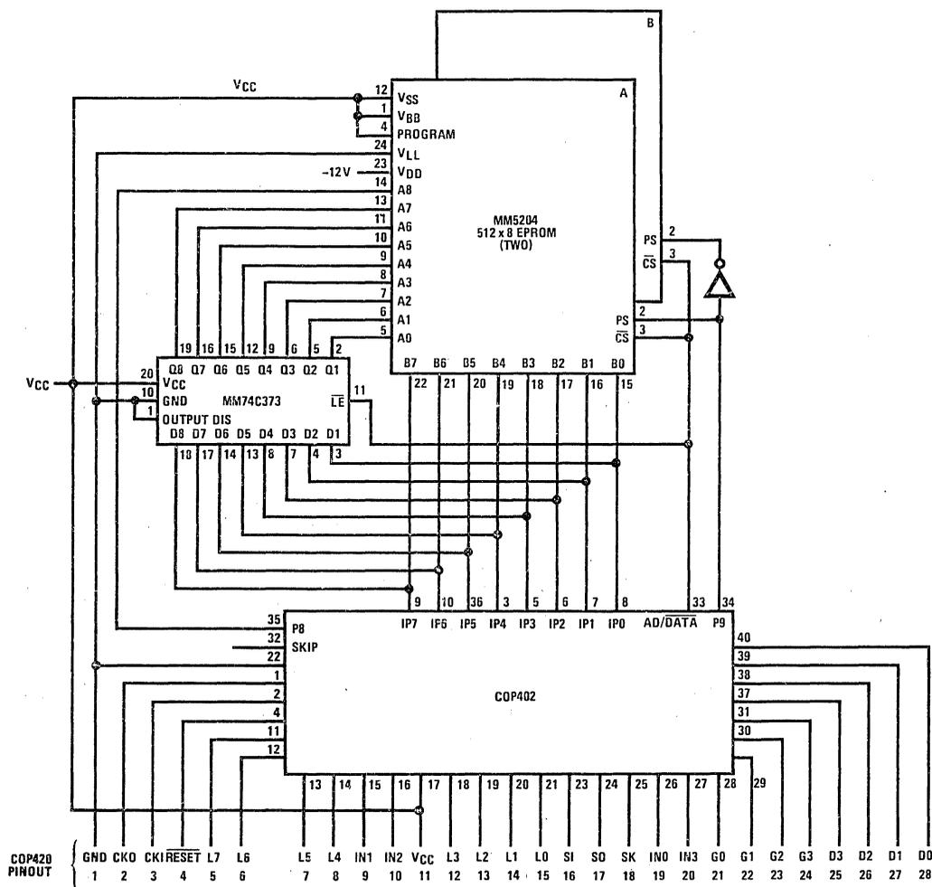
Figure 13. COP402 Used to Emulate a COP420
