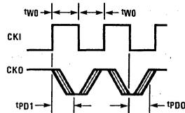
Figure 3B. CKO Output Timing
