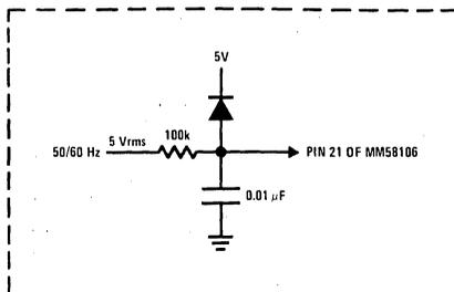
\* Optional Input Circuit Utilizing 50/60 Hz AC
