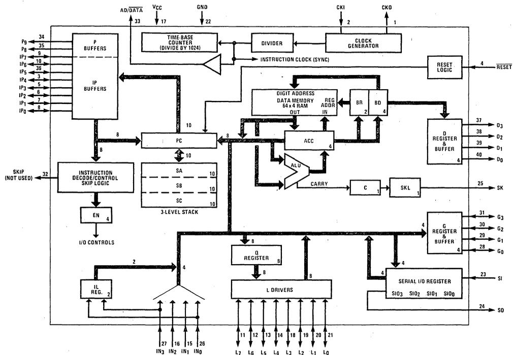
Figure 1. COP402/402M Block Diagram
