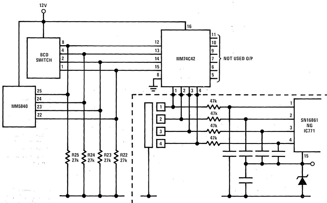
FIGURE 3. Channel Switching Interface with MM74C42
