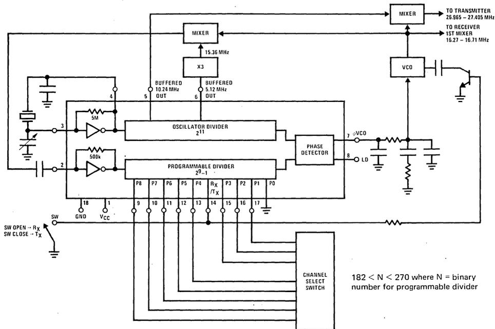
FIGURE 1. MM55108 Single Crystal 40-Channel Low Side Injection
