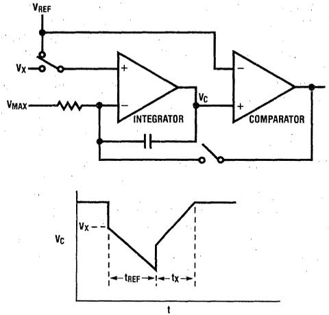
Figure 15. Modified Dual Slope — Basic Concept
