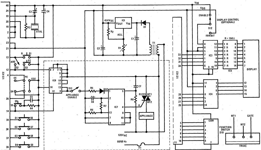
Figure 2. Schematic Diagram of the 4-Digit, 7-Function Stopwatch/Timer. As drawn, the display resolution is 1 second. A SPST switch may be included between pin 16 of IC2 and  $V_{SS}$  to provide a display resolution of 0.01 second or 1 second. Another option, shown in the figure, is the Display Control Switch, which may be used to inhibit the display.
