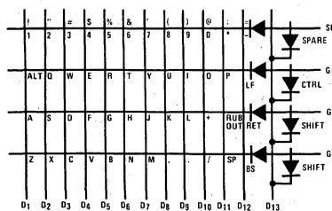
Figure 12. COP420 Keyboard/Display Interface
