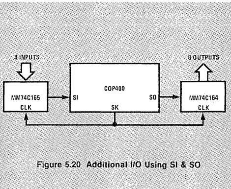
Figure 5.20 Additional I/O Using SI & SO
