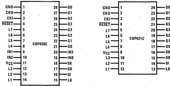
Figure 2. Connection Diagrams
