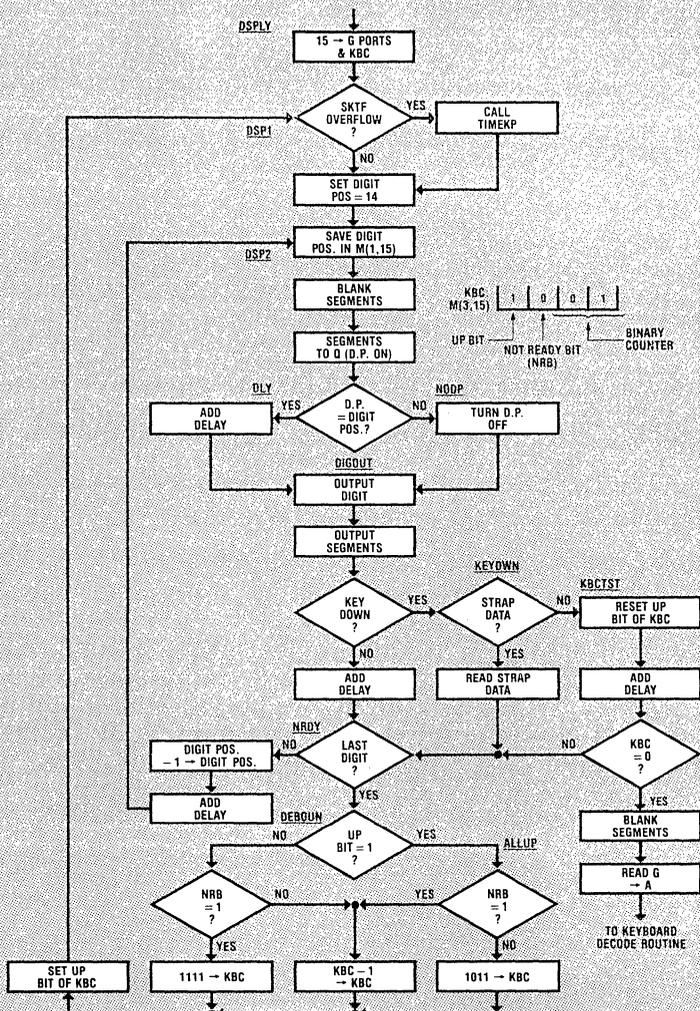
Figure 5.16 Flowchart for Display/Keyboard Debounce Routine
