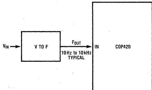
Figure 18. V to F Converter — Basic Concept
