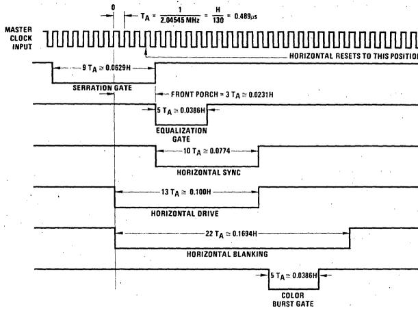
FIGURE 2. Horizontal Timing Master Clock = 2.04545 MHz
