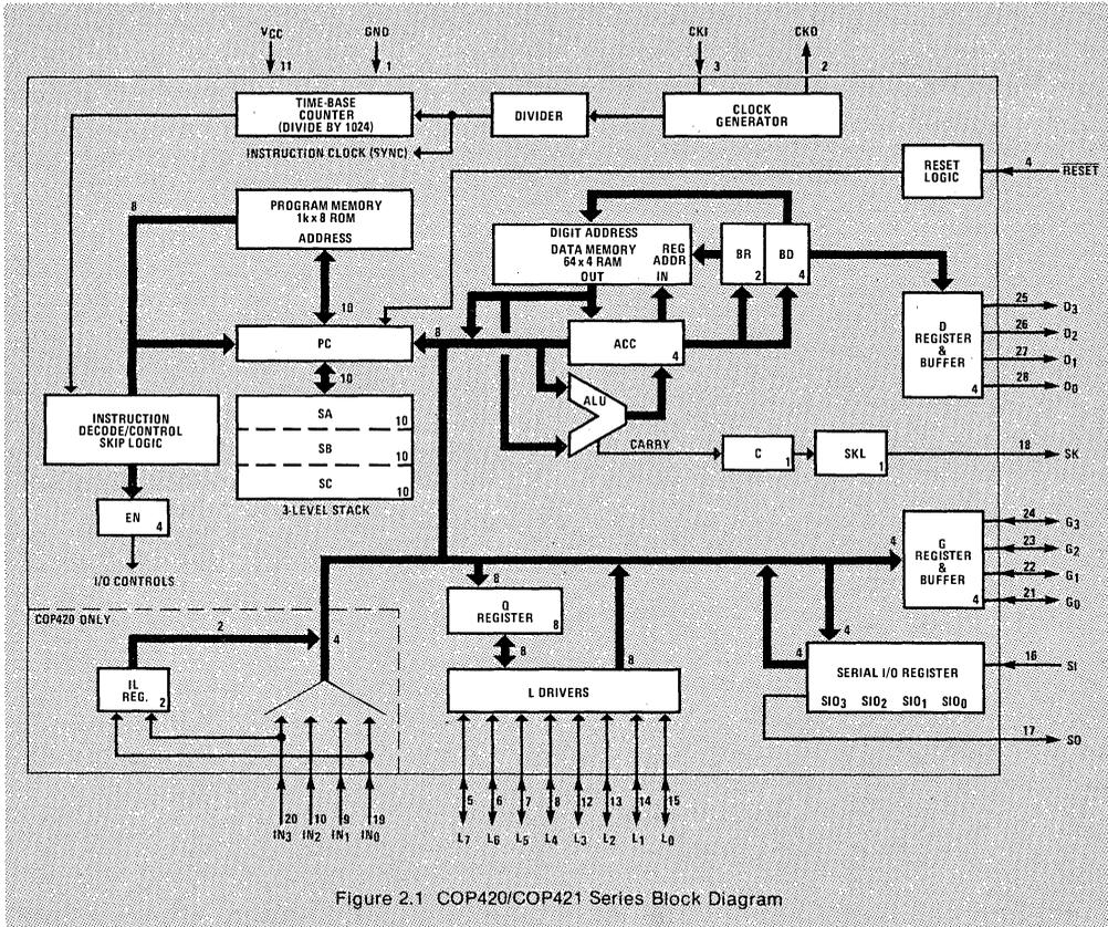
Figure 2.1 COP420/COP421 Series Block Diagram
