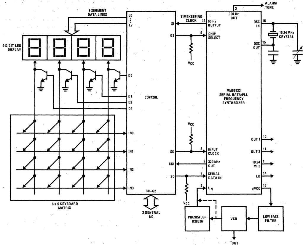
FIGURE 4. MM55123, COP420L Frequency Synthesizer/Controller
