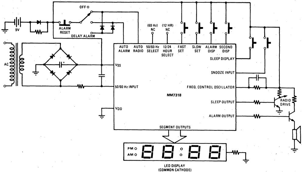
Figure 5. Typical Application (MM7318BN): Clock/Calendar with Battery Back-up
