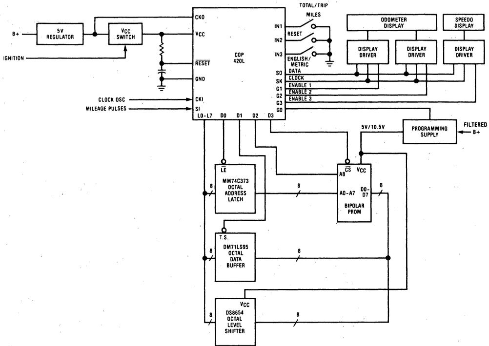
Figure 1. Electronic Speedometer/Odometer
