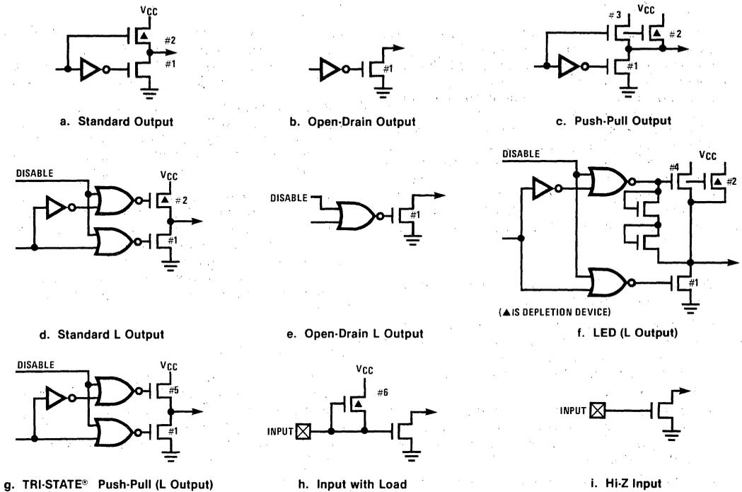
Figure 5. Output Configurations
