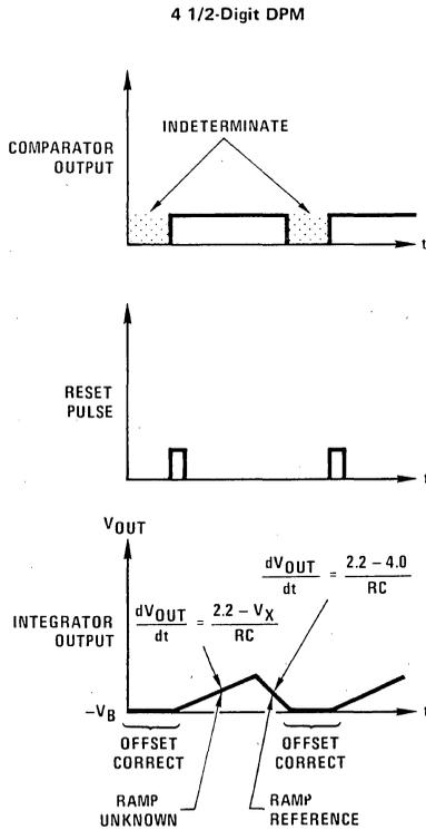
Note. Here the LF13300 always operates as an autozeroed, high input impedance inverting integrator; bipolar input voltages are handled by offsetting the analog ground by 2.2V.
