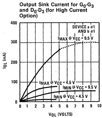
Figure 6. I/O Characteristics
