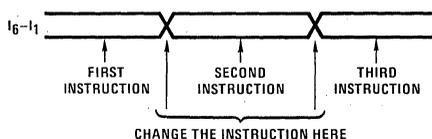
6. Minimum and/or maximum time values are sometimes specified. The interpretation of these values depends on whether the waveforms are inputs or outputs. Example:
