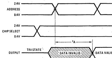
FIGURE 2. Address Follows Chip Select
