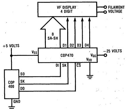
Figure 4. System Diagram - 4 Digit Display
