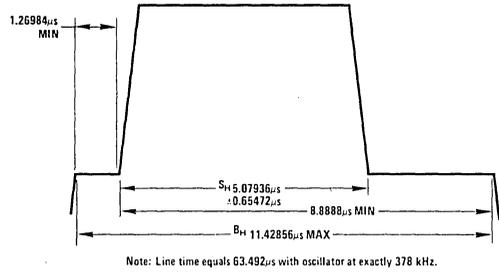
FIGURE 4. Composite Video Pulse Timing, Horizontal Sync
