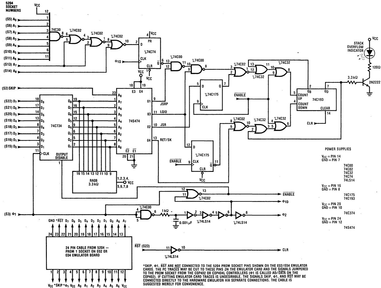
\*SKIP, ϕ1, RST ARE NOT CONNECTED TO THE 5204 PROM SOCKET PINS SHOWN ON THE E02/E04 EMULATOR CARDS. THE PC TRACES MAY BE CUT TO THESE PINS ON THE EMULATOR CARD AND THE SIGNALS JUMPERED TO THE PROM SOCKET FROM THE COP402 OR COP404L CONTROLLERS (ϕ1 IS CALLED AD/DATA ON THE COP402). IF CUTTING EMULATOR CARD TRACES IS UNDESIRABLE, THE SIGNALS SKIP, ϕ1, AND RST MAY BE CONNECTED DIRECTLY TO THE HARDWARE EMULATOR VIA SEPARATE CONNECTIONS. THE CABLE IS SUGGESTED MERELY FOR CONVENIENCE.
