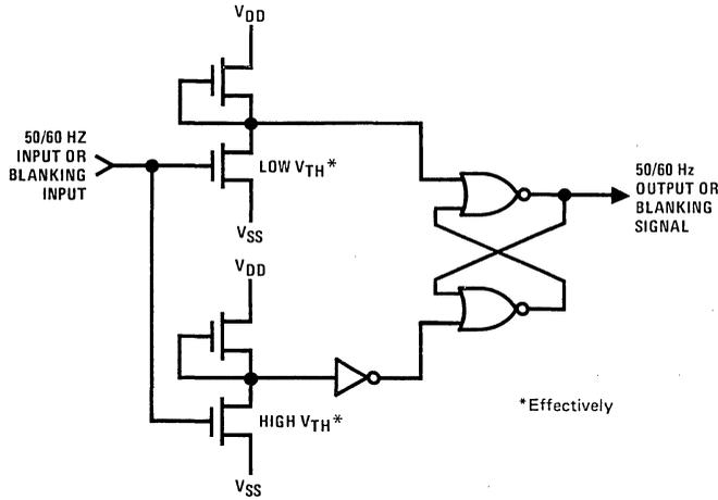
FIGURE 3. 50/60 Hz or Blanking Input Shaping Circuit
