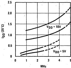
FIGURE 6. Typical Current Drain vs Oscillator Frequency
