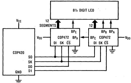
Figure 7. System Diagram — 8 1/2 Digit Display
