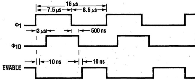
$$ENABLE = (\overline{\Phi 1} + \Phi 1D)$$
