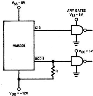
For  $V_{SS} = 5, V_{DD} = -12, R = 7.5k$
