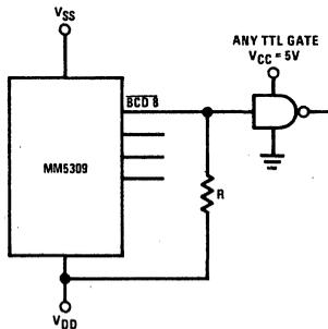
For  $V_{SS} = 5, V_{DD} = 12, R = 10k$
