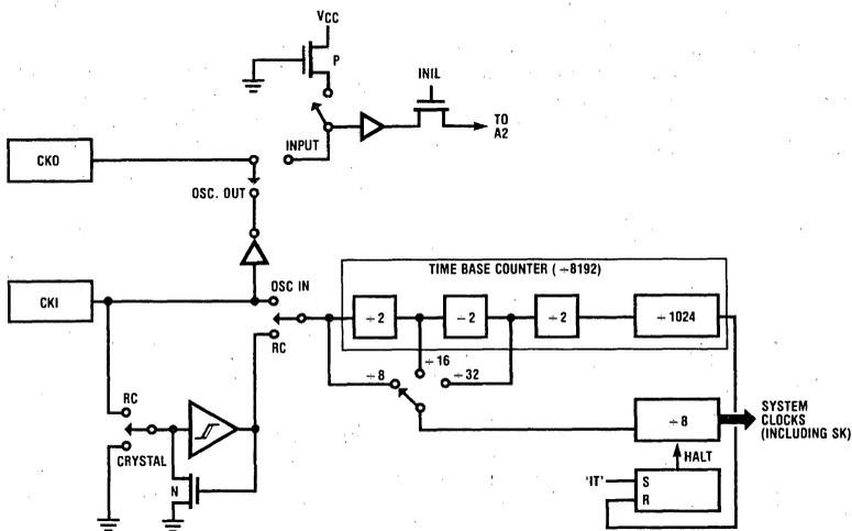
Figure 10b. Oscillator Options Block Diagram Using IT Instruction
