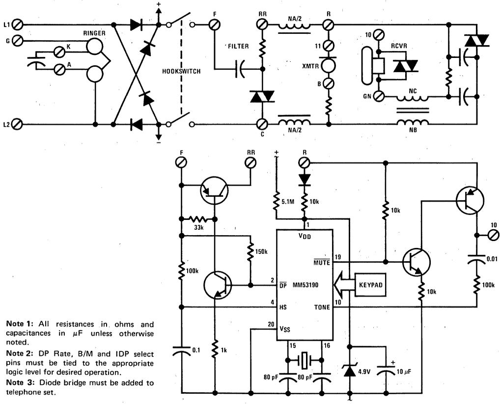
**Note 1:** All resistances in ohms and capacitances in  $\mu\text{F}$  unless otherwise noted.
