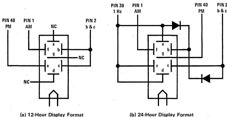
FIGURE 5. Wiring Ten's-of-Hours Digit
