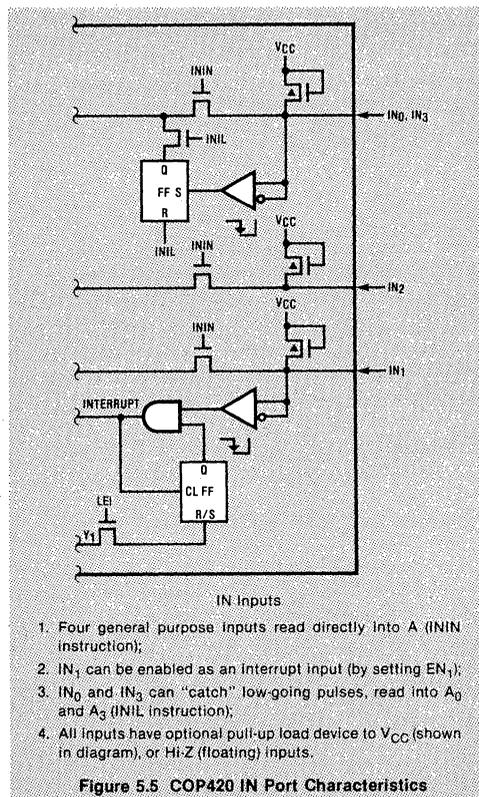
1. Four general purpose inputs read directly into A (ININ instruction);
