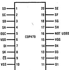
Figure 1. COP470 Pin Connection
