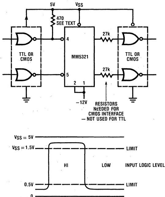
Figure 1. Input/Output Interfacing
