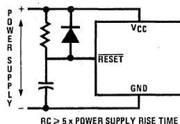
Figure 7. Power-Up Clear Circuit
