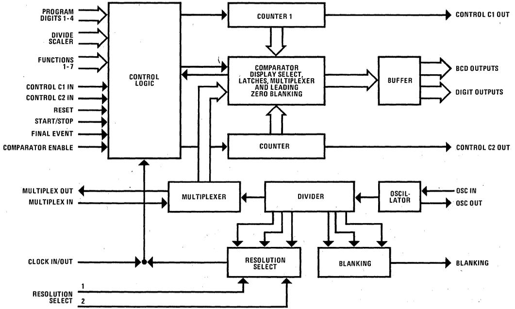
Figure 1. Internal block diagram of the MM5865 Universal Timer.
