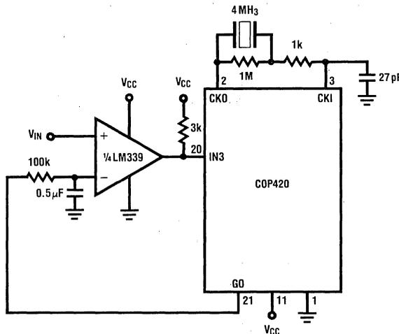
CRYSTAL OSCILLATOR VALUES CHOSEN TO GIVE  $4\mu\text{s}$  CYCLE TIME WITH DIVIDE BY 16 OPTION
