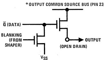
\* Alarm and sleep output sources are connected to  $V_{SS}$ ; blanking is not applied to these outputs.
