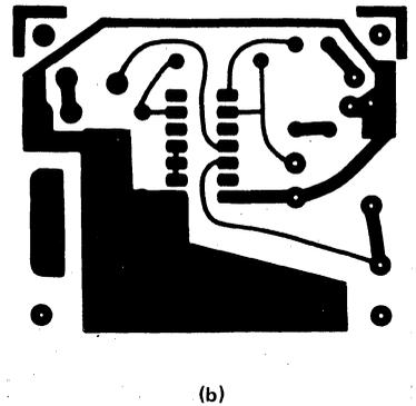
Figure 12. X1 Positives for the Printed Circuit Boards. a) Positive for the Stopwatch/Timer. b) Positive for the Appliance Control circuit.
