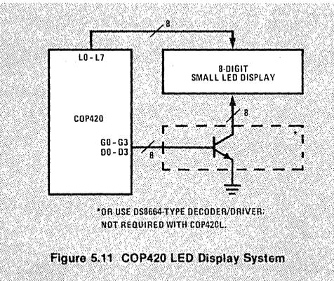
Figure 5.11 COP420 LED Display System
