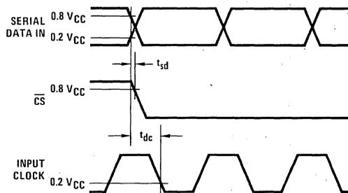
$t_{sd}$  = Delay time between active chip select command and initial data input.
