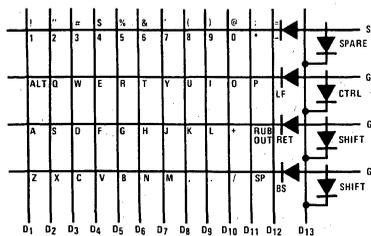
Figure 12. COP420 Keyboard/Display Interface
