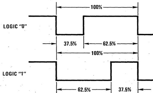
A bit is equivalent to 96 clocks of the R-C oscillator frequency i.e., when R-C frequency = 400 kHz, 1 bit = 240  $\mu$ s, 1 word = 4.32 ms.
