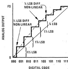
FIGURE 7.  $1\frac{1}{2}$  LSB Non-Linear,  $\frac{1}{2}$  LSB Differential Non-Linearity
