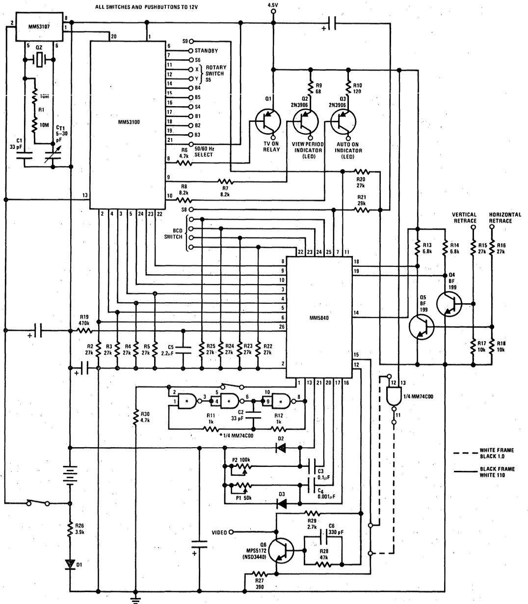
FIGURE 1. Clock Schematic
