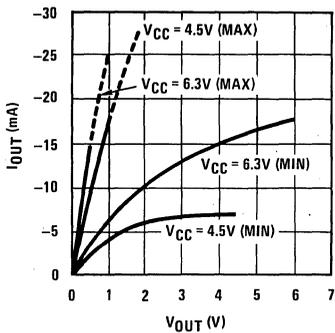
Depletion Load Off Source Current
