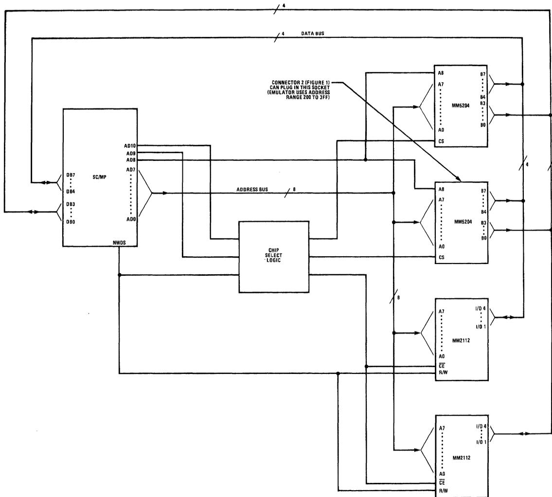
Figure 2. Memory Configuration of SC/MP Introkit Showing PROM/ROM Emulator Connection
