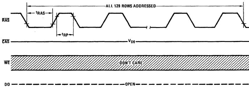
FIGURE 11.  $\overline{\text{RAS}}$  Only Refresh Cycle
