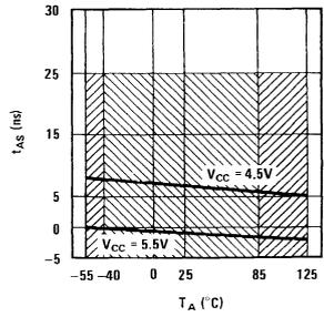
(h) Address Setup Time vs Ambient Temperature
