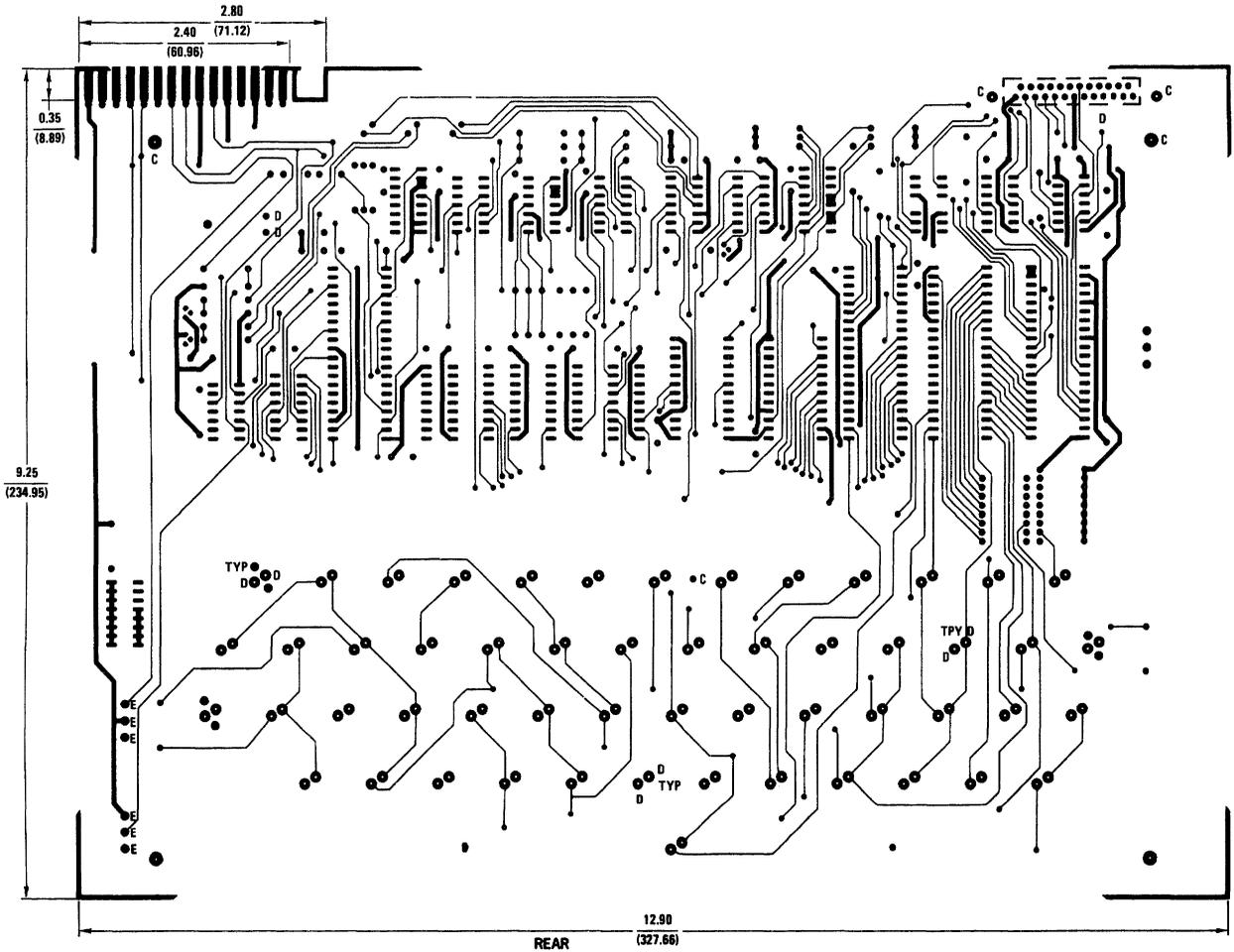
FIGURE 7B. PC Board Layout Fabrication
