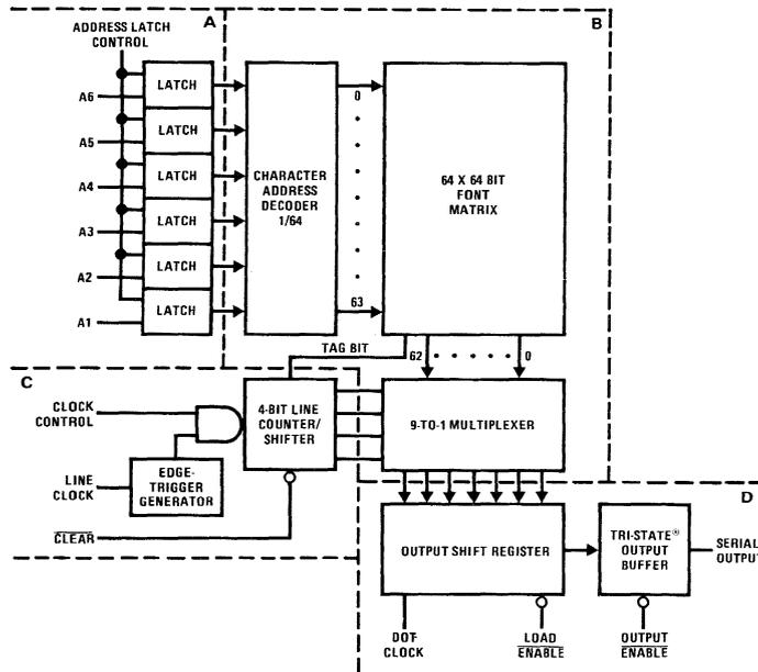
FIGURE 1. Block Diagram
