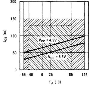
(i) Output Enable Time vs Ambient Temperature
