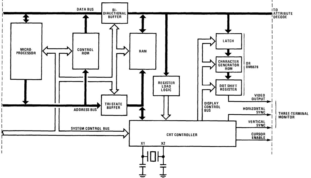
Figure 7. System Diagram with no Line Buffer
