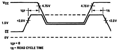
Figure 4. 4k Static Power Down Mode
