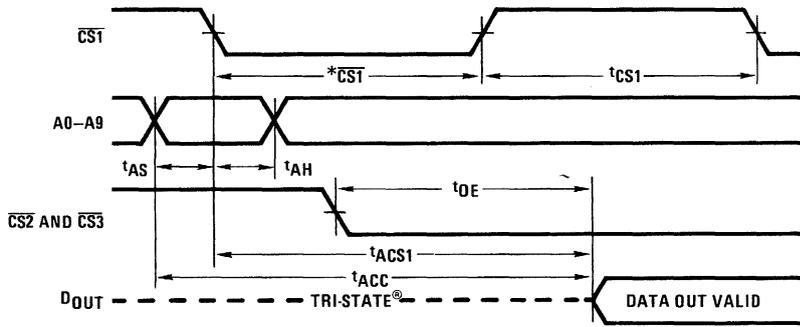
(a) Read Cycle ( $\overline{WE} = V_{IH}$ )
