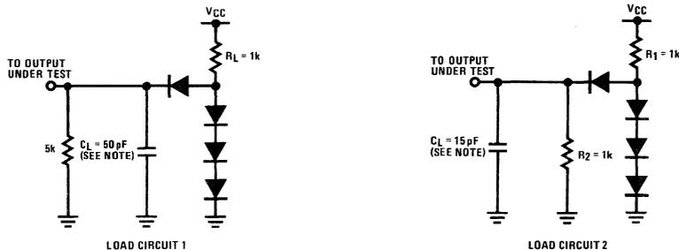
NOTE:  $C_L$  INCLUDES PROBE AND JIG CAPACITANCE
