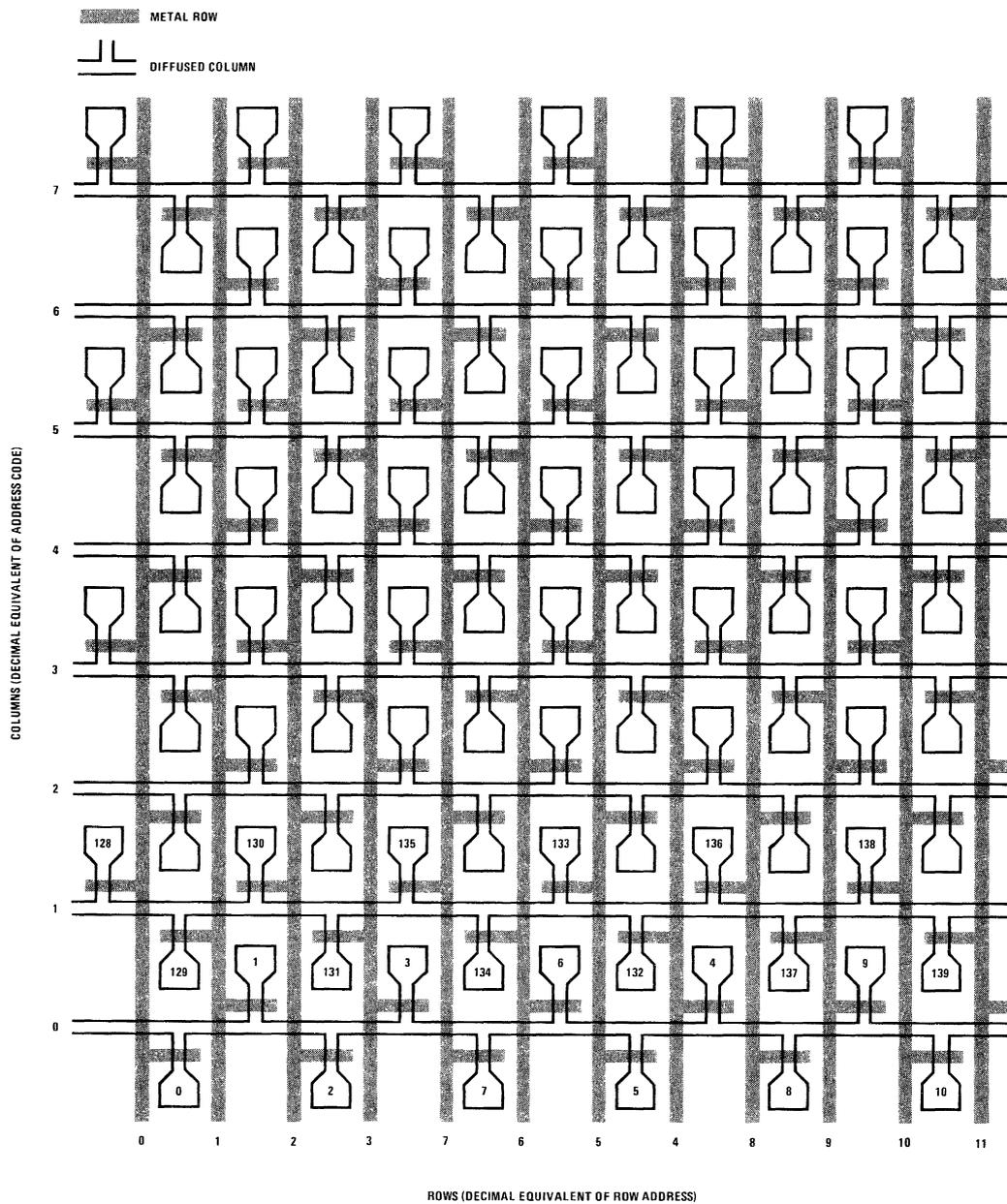
Figure 6. Simplified Topology (lower left corner of array)
