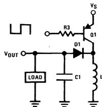
FIGURE 2. Flyback Circuit
