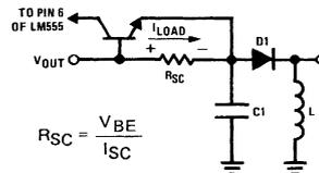
FIGURE 13. Short Circuit Protection
