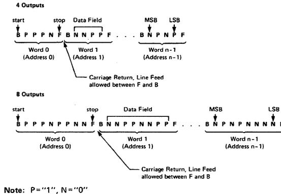
Figure 8. BPNF Paper Tape Formats
