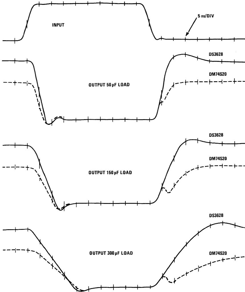
Figure 3. Switching Response with Capacitive Load
