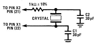
If the DP8350 series is clocked at dot rate by a system clock, pin 22 (X1 input) should be clocked directly using a Schottky series circuit. Pin 21 (X2 input) may be left open.
