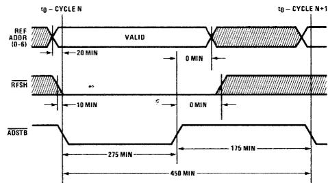
Figure 4. REFRESH Cycle Timing
