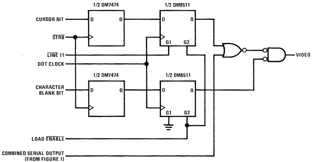
FIGURE 2. Pipelining Attribute Bits
