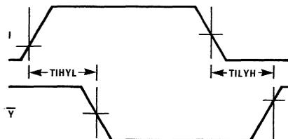
The first interval is the delay from I HIGH to Y LOW and the second from I LOW to Y HIGH.
