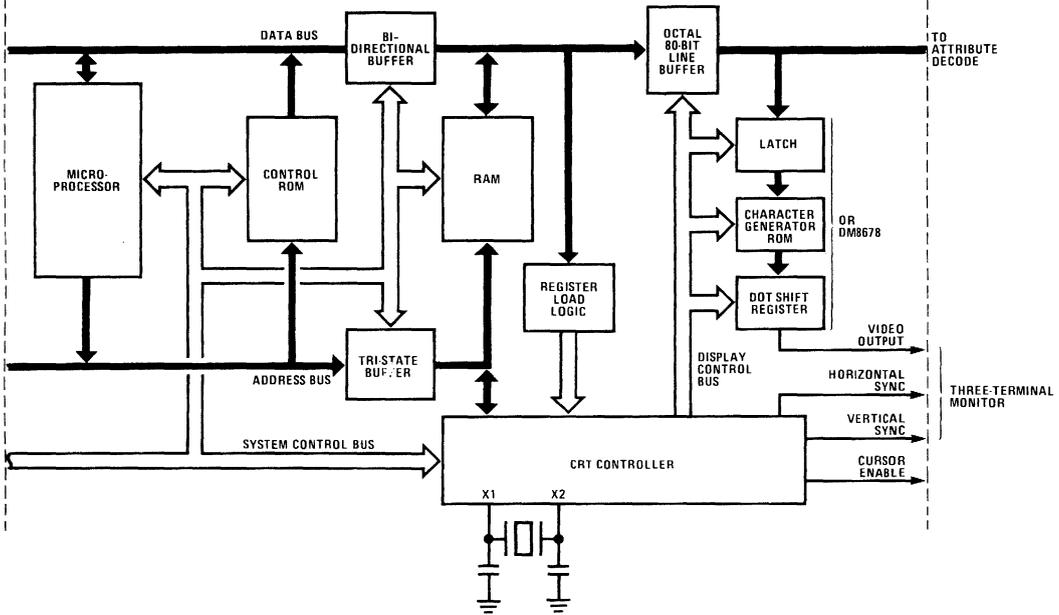
Figure 6. System Diagram Using a Line Buffer
