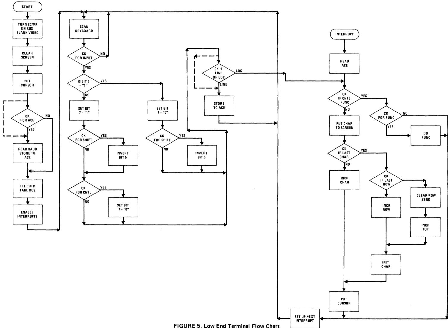
FIGURE 5. Low End Terminal Flow Chart
