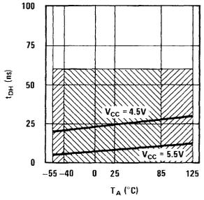
(e) Data-In Hold Time vs Ambient Temperature
