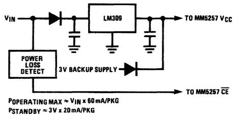
Figure 3. 4k Static Power Down 2
