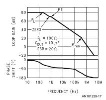
FIGURE 17. HIGH ESR CAUSES UNSTABLE LOOP
