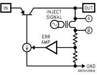
FIGURE 6. LOOP GAIN EXAMPLE
