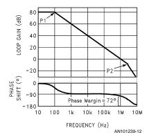
FIGURE 12. BODE PLOT FOR NPN REGULATOR
