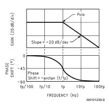
FIGURE 9. POLE GAIN/PHASE PLOT
