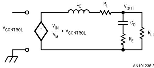
FIGURE 3. Small Signal Model of Power Stage
