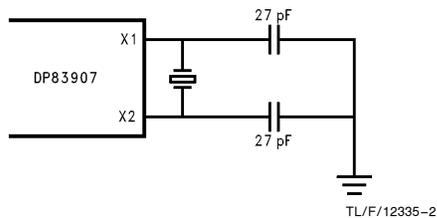
FIGURE 2. Crystal Circuit
