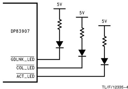
FIGURE 5. LED Circuit
