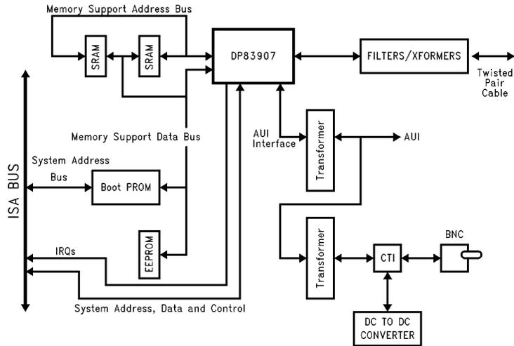
FIGURE 1. DP83907EB Block Diagram
