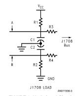
FIGURE 3. Node Load Circuit
