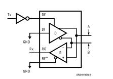
FIGURE 4. The DS75176B in a SAE J1708 Application
