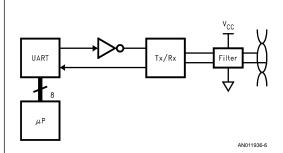
FIGURE 6. Typical SAE J1708 System Block Diagram
