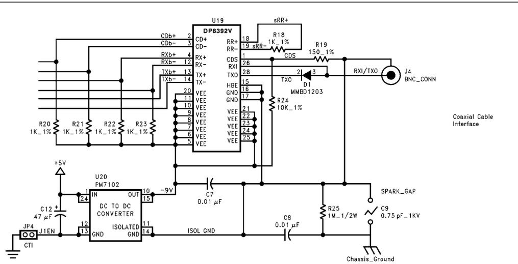
Note: CTI configured for transmit mode collision detection.
