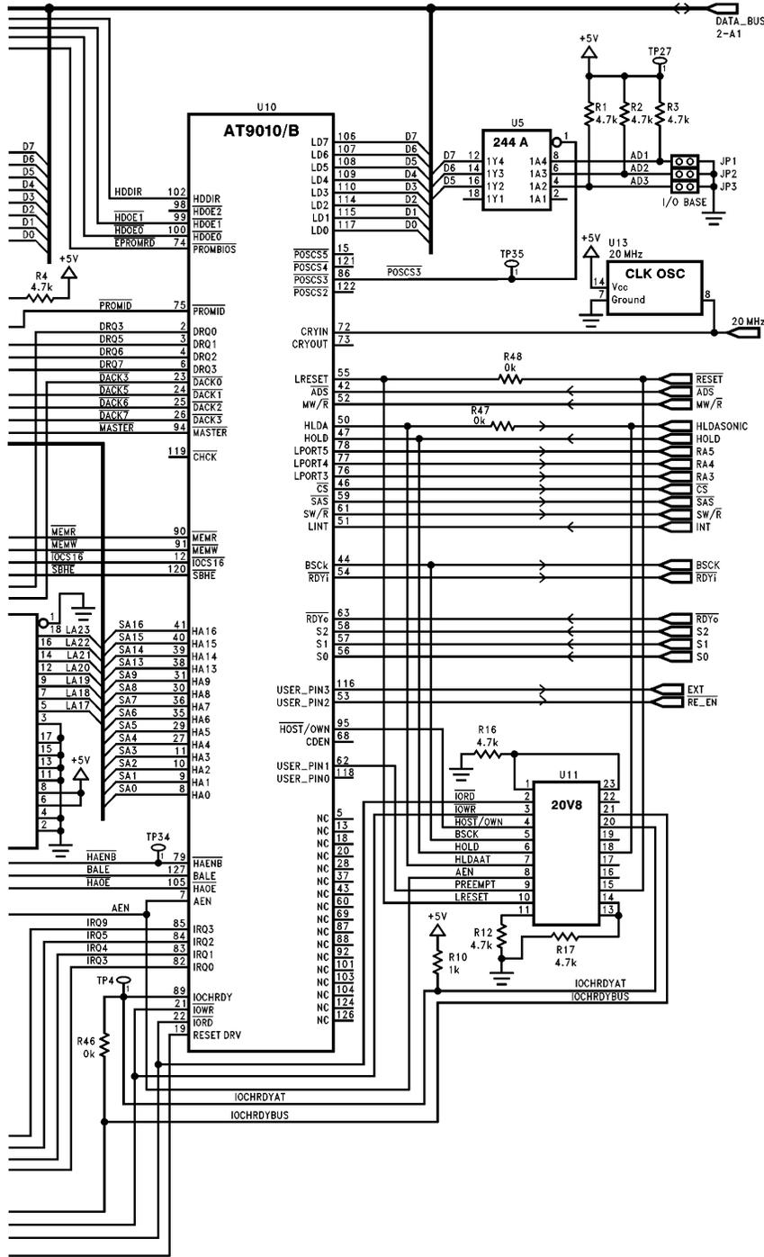
**Note:** For original AT9010, install U11 and leave R46, R47 and R48 open. For AT9010B install R46, R47 and R48 and leave U11 open.
