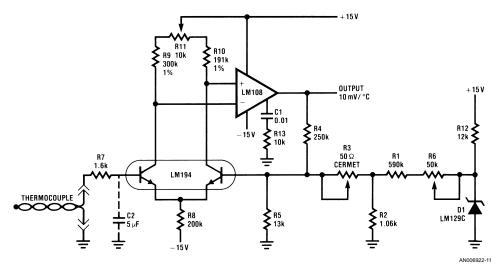
FIGURE 11. Thermocouple Amplifier with Cold-Junction Compensation
