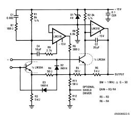
FIGURE 5. Low Drift-Low Noise Instrumentation Amplifier
