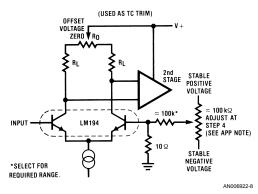
FIGURE 8. Correcting for Residual or Source Generated Drift
