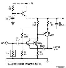
FIGURE 4. Ultra Low Noise Preamplifier
