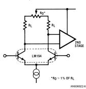
FIGURE 6. Zeroing Offset and Drift
