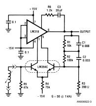
NOTE: Cartridge is assumed to have less than 5  $k\Omega$  DC resistance. Do not capacitor couple the cartridge. R1, R2, and R3 should be low noise metal film resistors.
