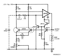
FIGURE 9. Micropower Reference
