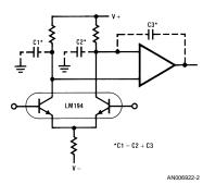
FIGURE 2. High Frequency Power Supply Rejection
