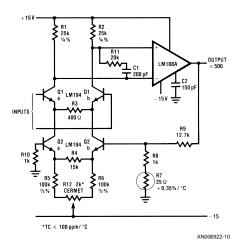
FIGURE 10. Strain Gauge Instrumentation Amplifier
