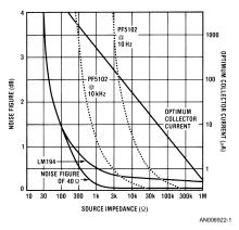
FIGURE 1. Noise Figure vs Source Impedance
