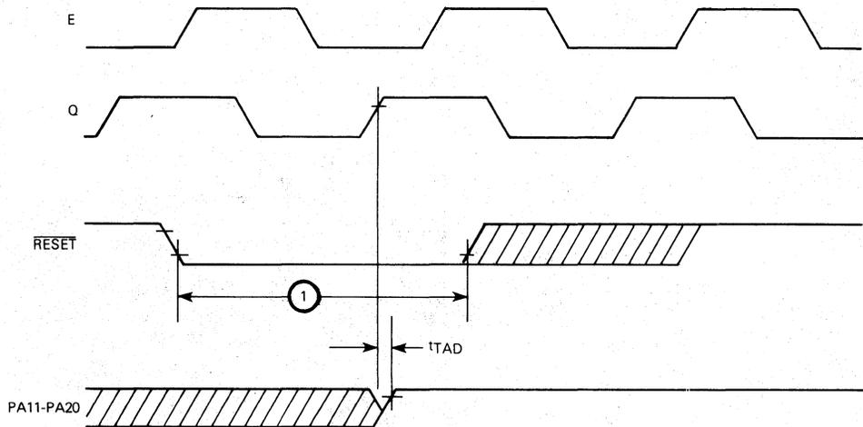
Note: Timing measurements are referenced to and from a low voltage of 0.8 volts and a high voltage of 2.0 volts, unless otherwise noted.
