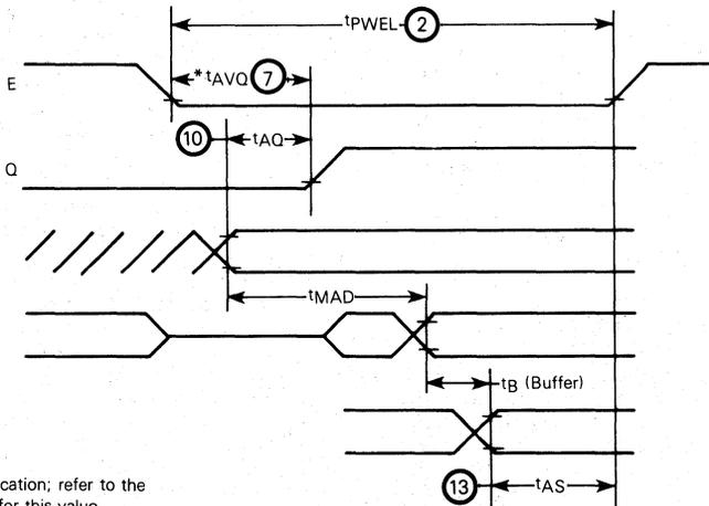
\* $t_{AQ}$  is a MPU specification; refer to the MC6809 Data Sheet for this value.
